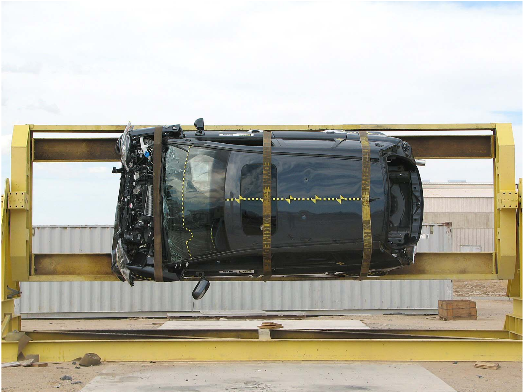
Figure A-59: Vehicle on Rollover Device (90°)
