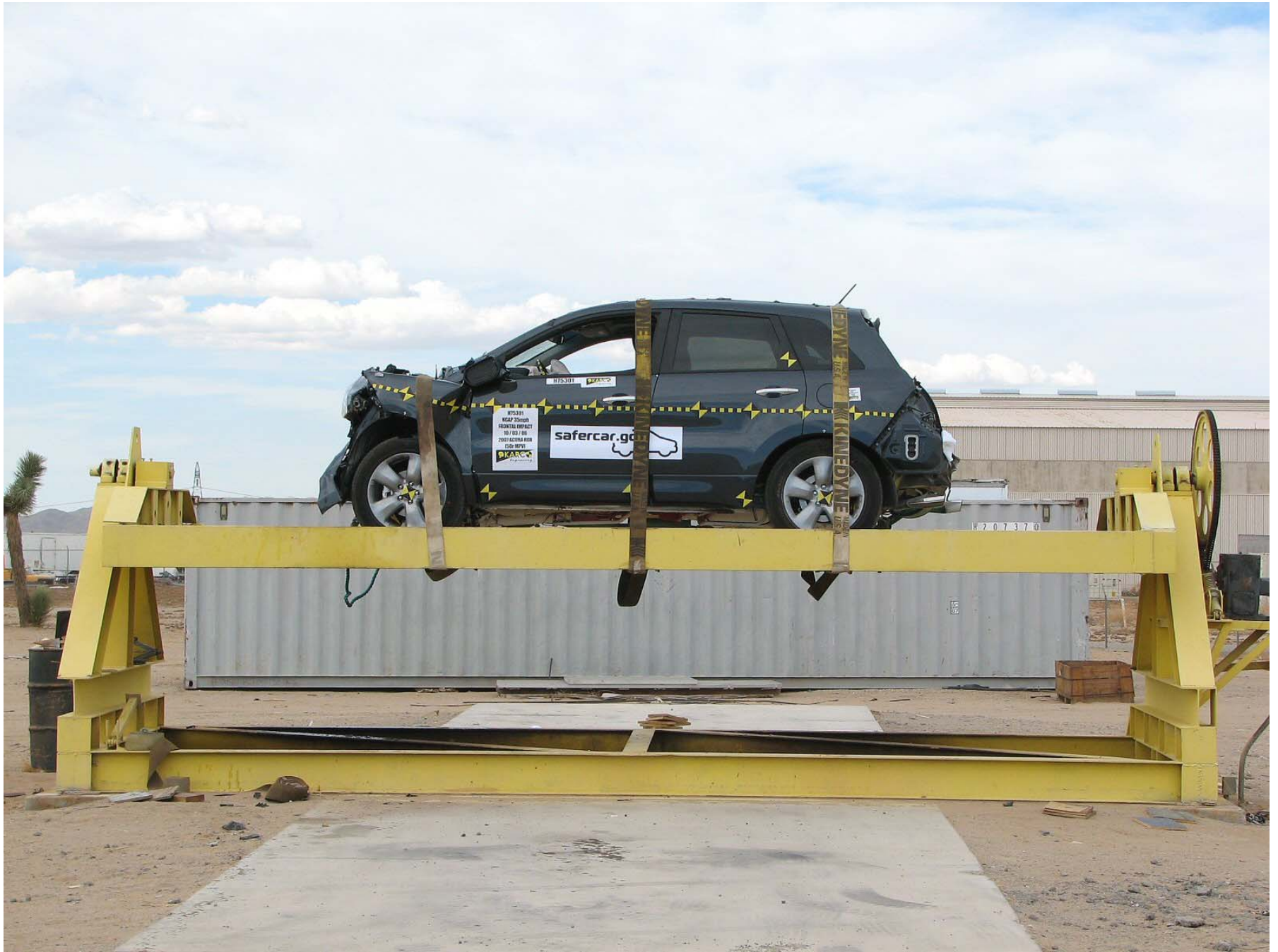
Figure A-58: Vehicle on Rollover Device (0°)
