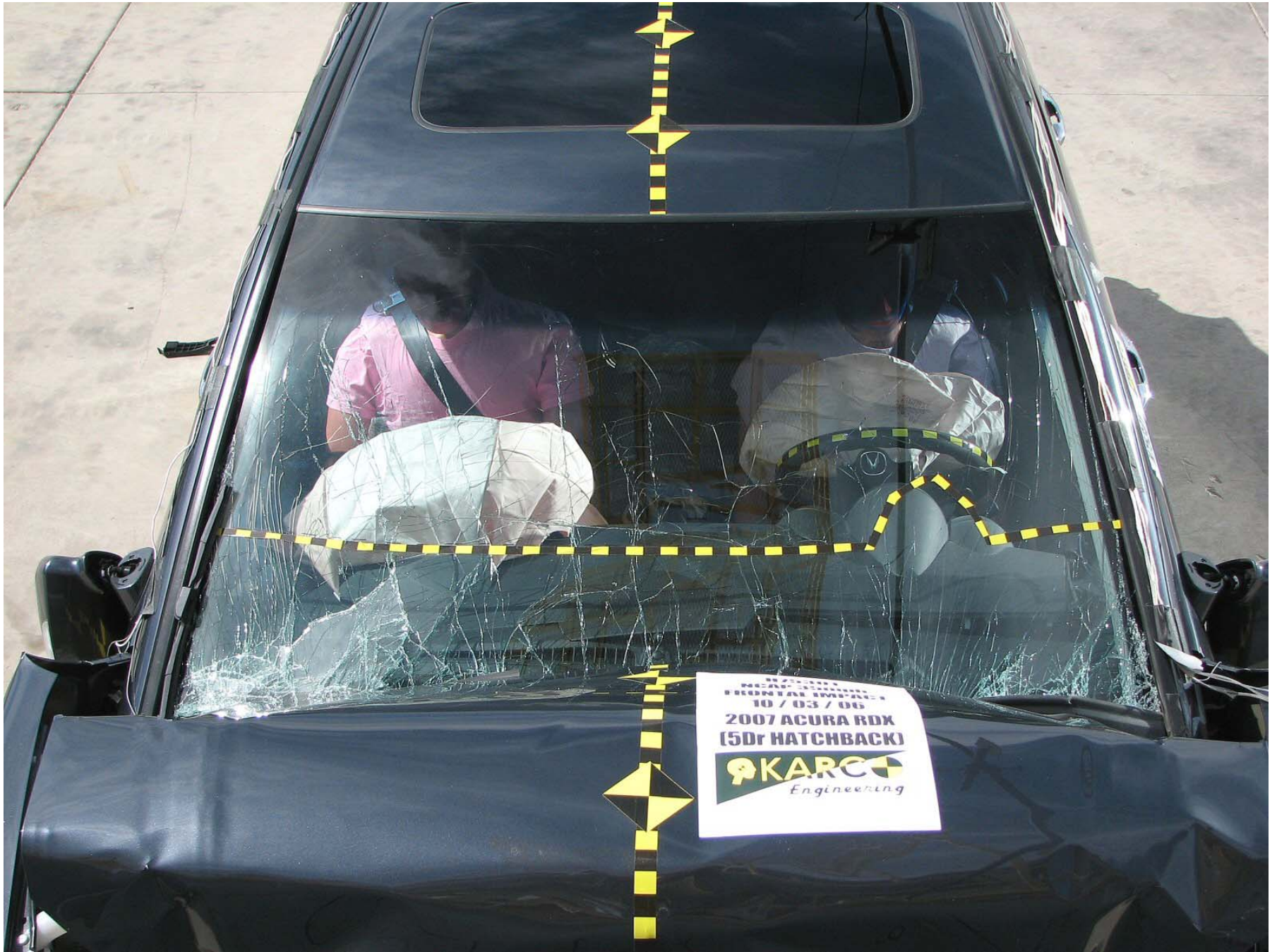
Figure A-19: Post-Test Windshield
