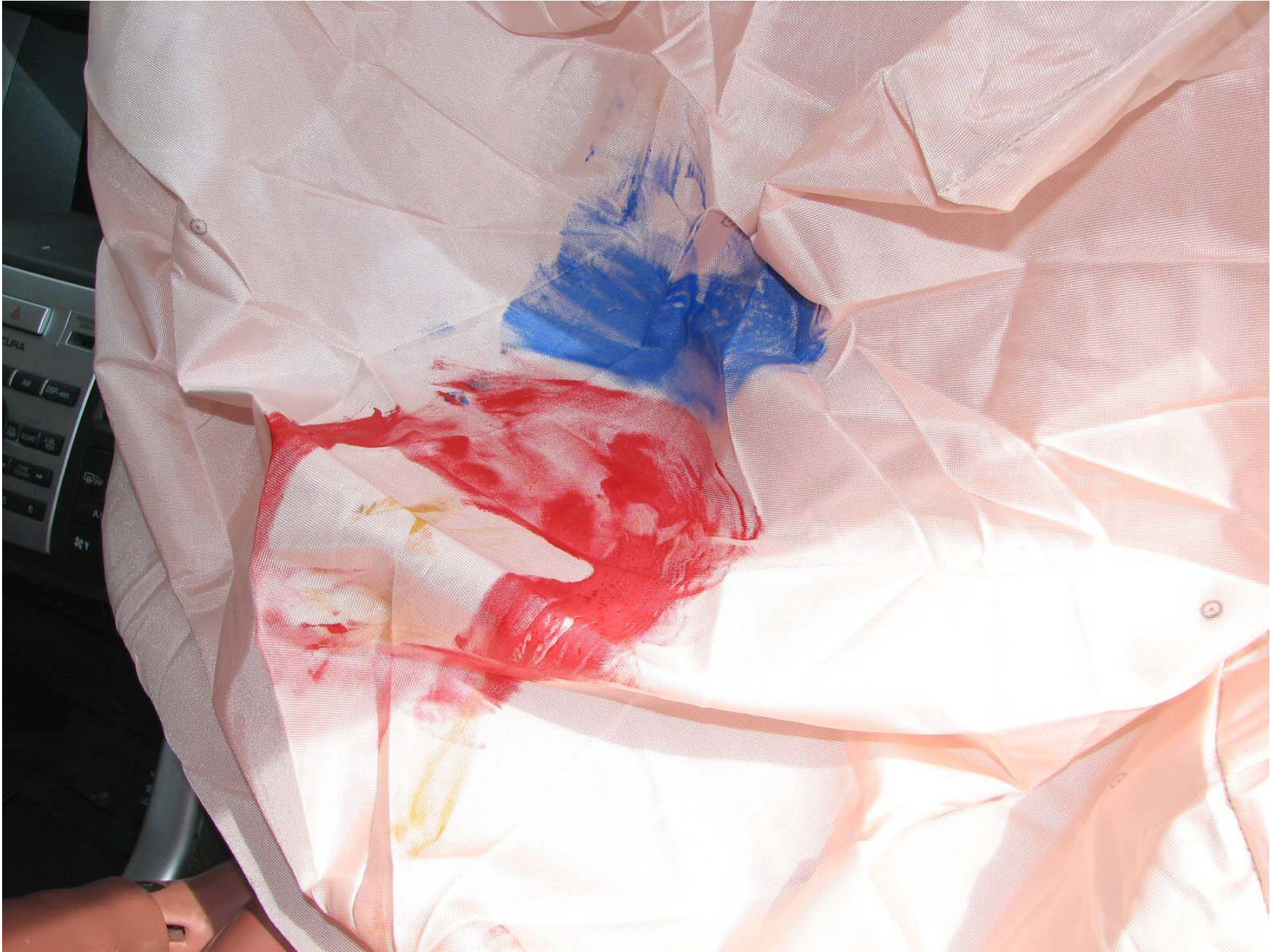
Figure A-57: Post-Test Passenger Dummy Airbag Contact
