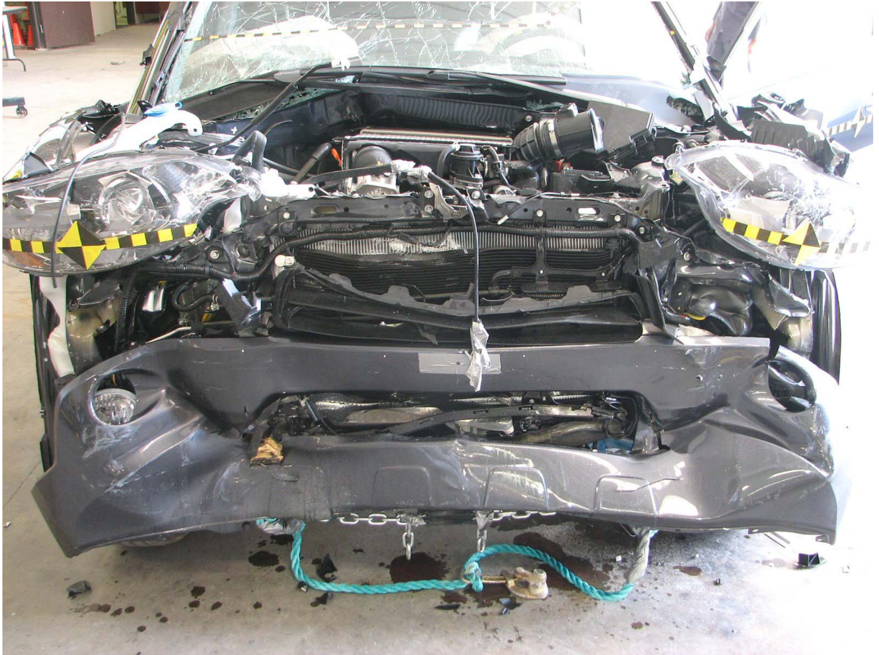
Figure A-21: Post-Test Engine Compartment (Vehicle Moved)
