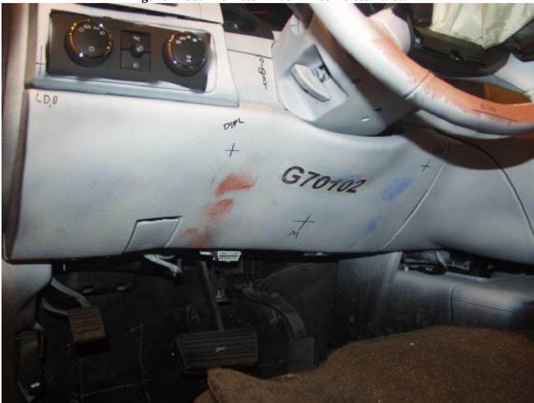
Figure A-39: Post-Test Driver Knee Bolster View
