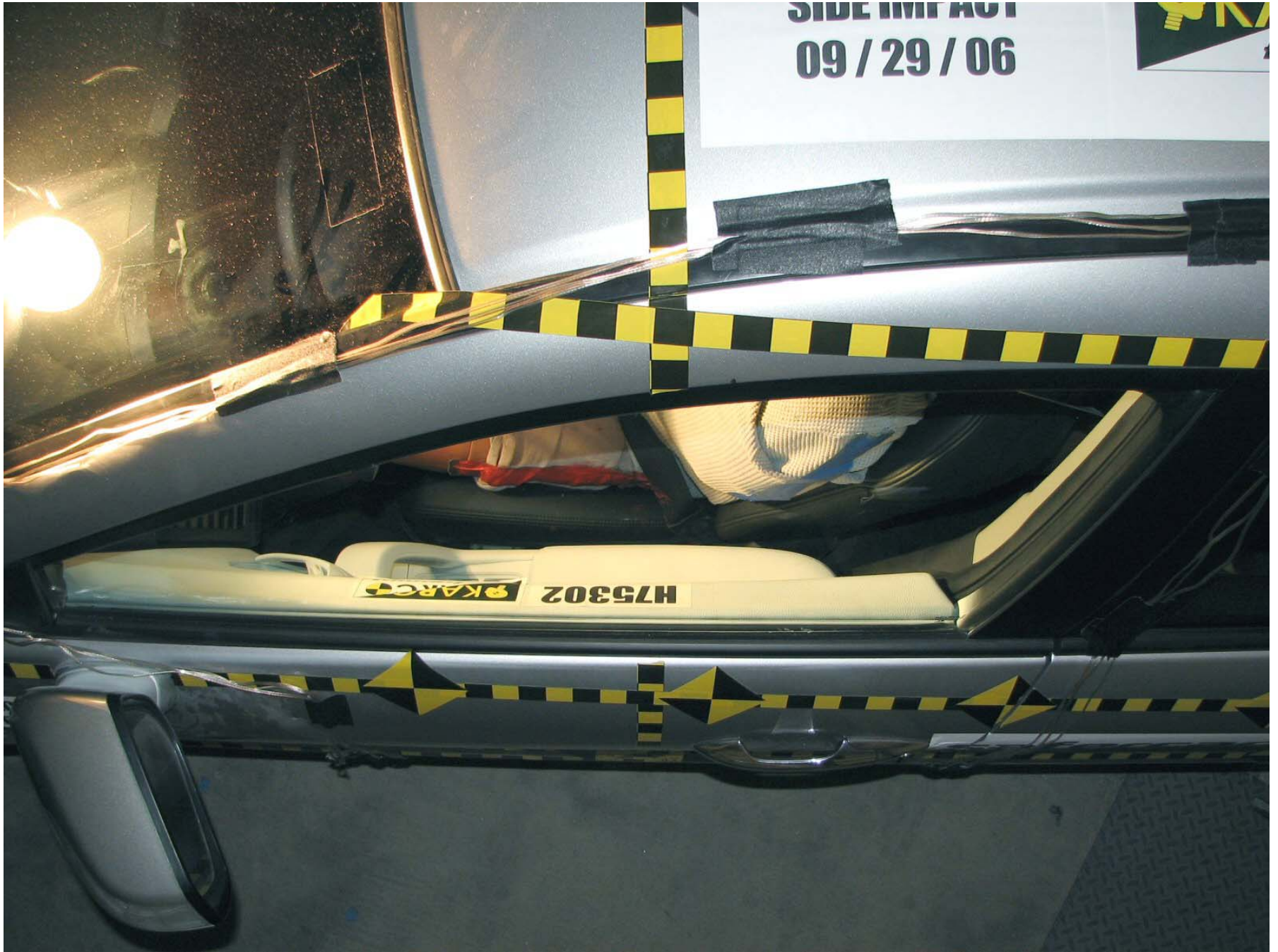
Figure A-38: Pre-Test Driver Dummy Clearance From Door
