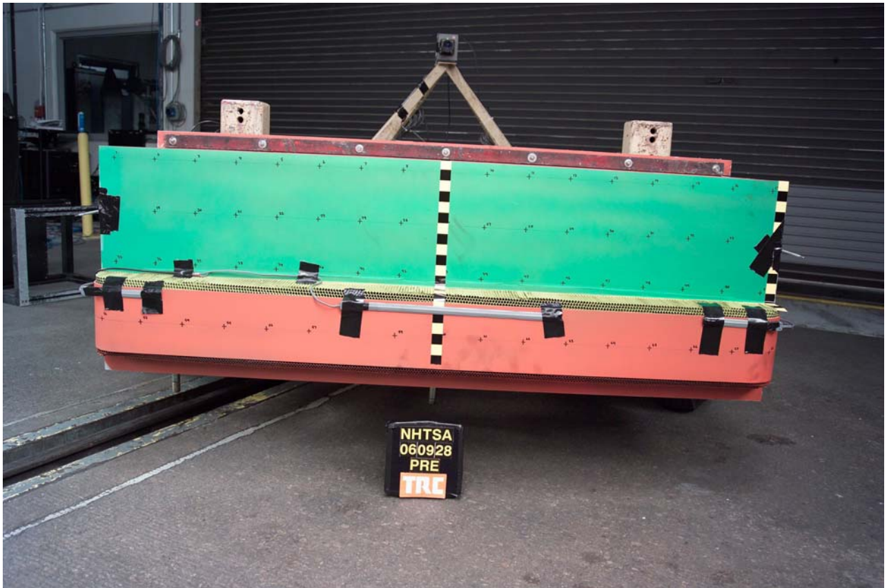
Figure A-58 Pre-Test Front View of Deformable Barrier
