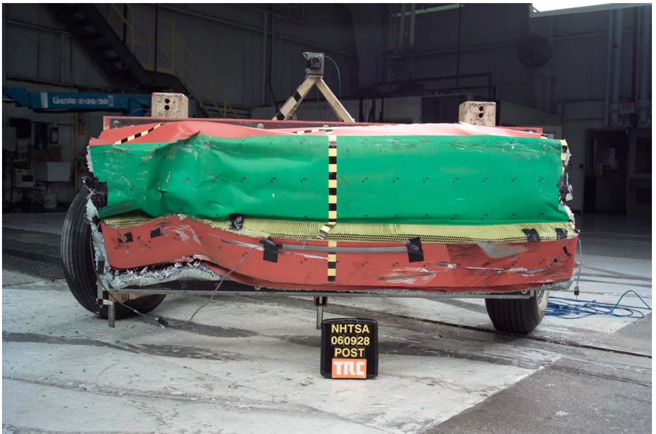
Figure A-59 Post-Test Front View of Deformable Barrier
