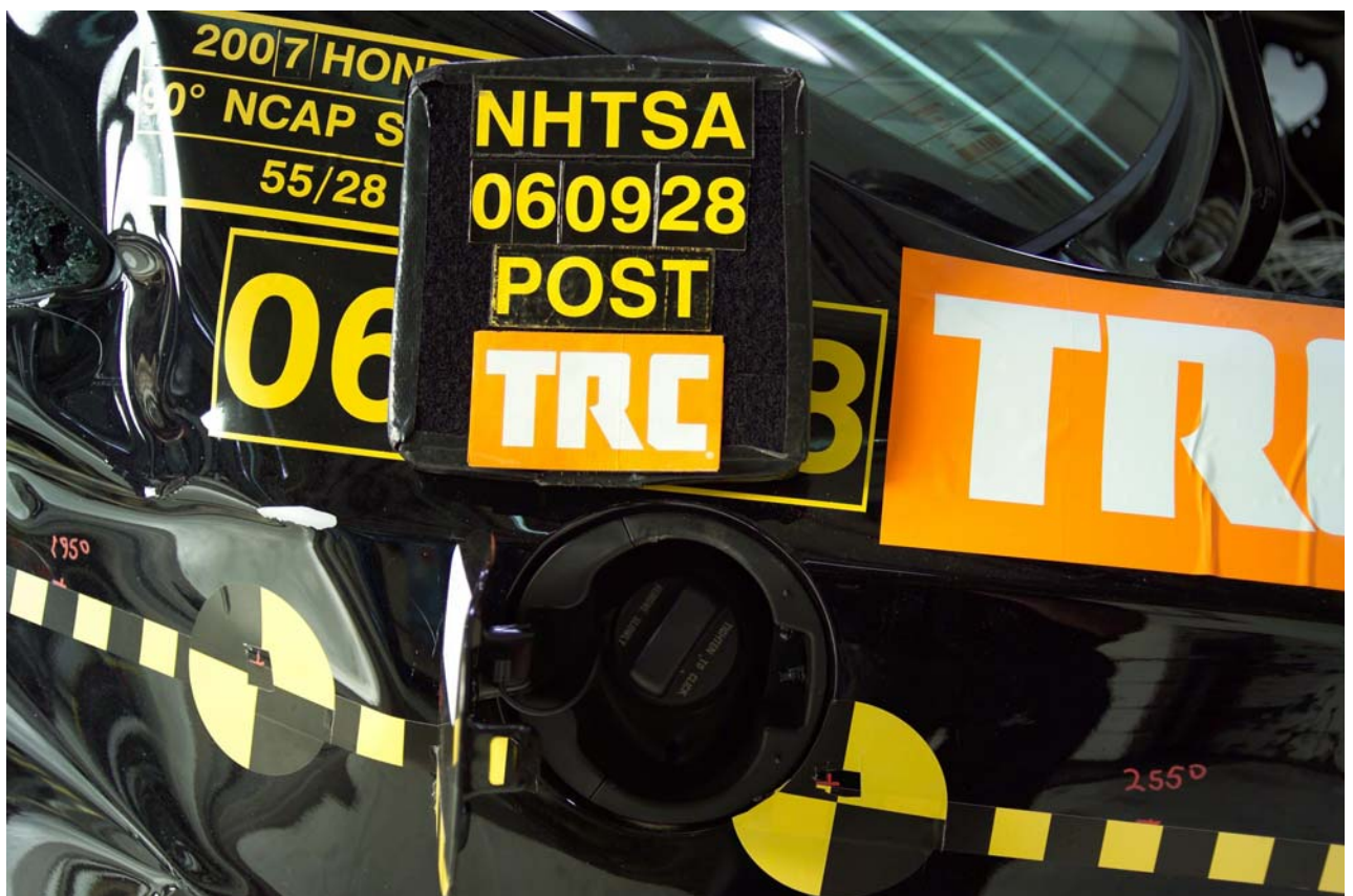
Figure A-26 Post-Test Fuel Filler Cap - View 1
