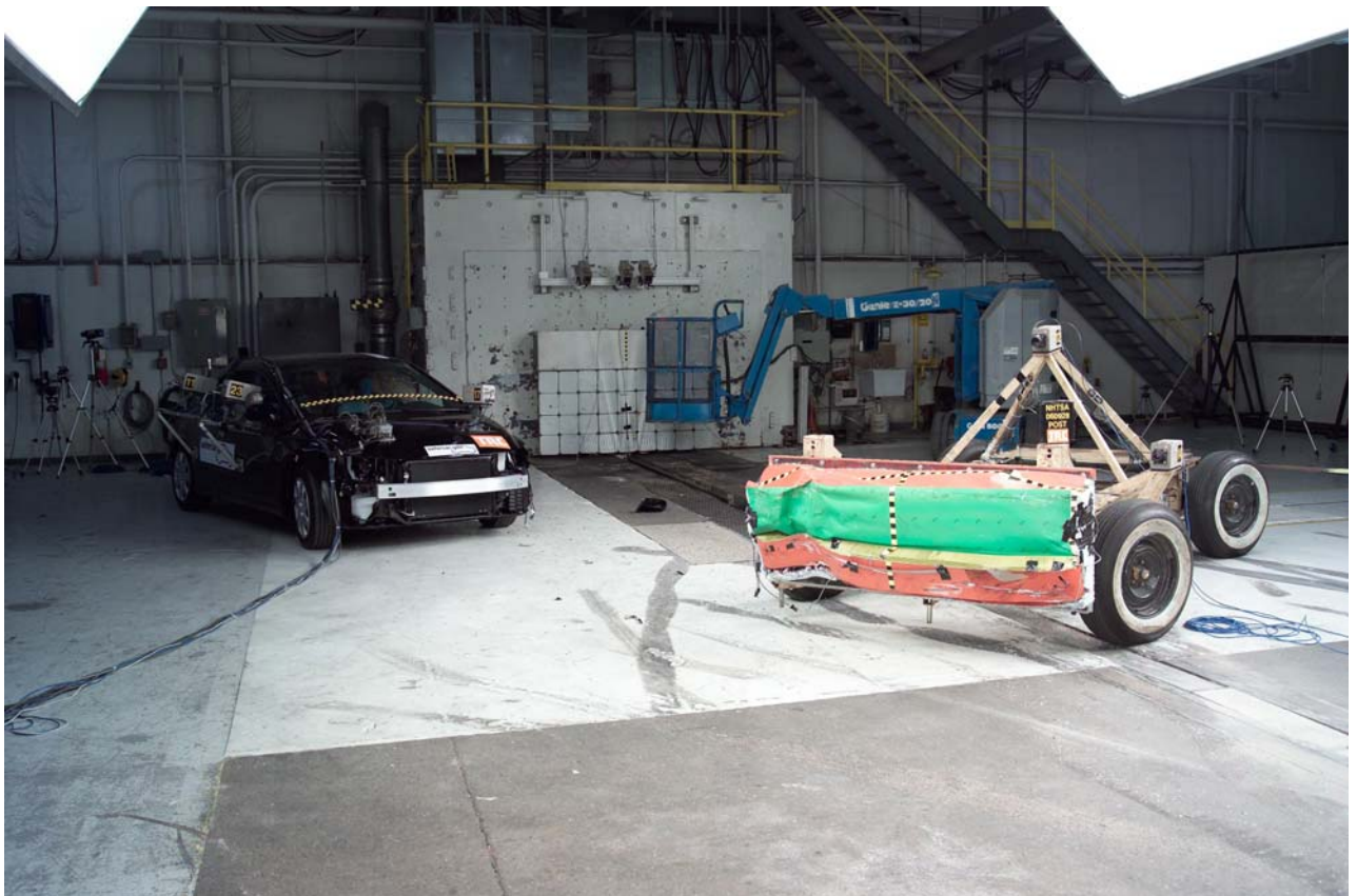
Figure A-77 Post-Test Moving Barrier and Vehicle Right Front View
