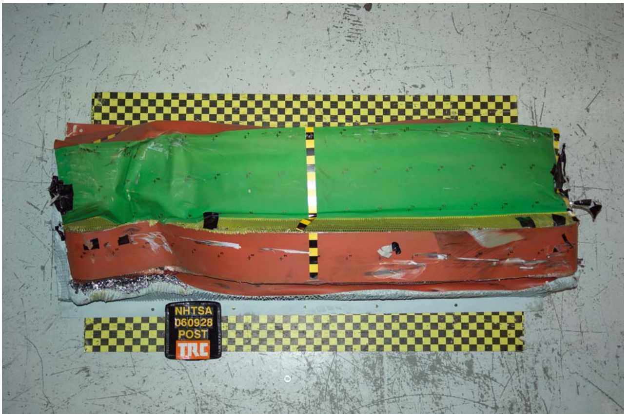
Figure A-51 Post-Test Front View of Barrier Face
