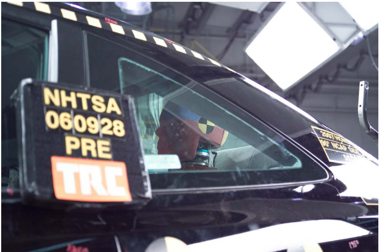
Figure A-40 Pre-Test Rear Passenger Dummy (Through Window)
