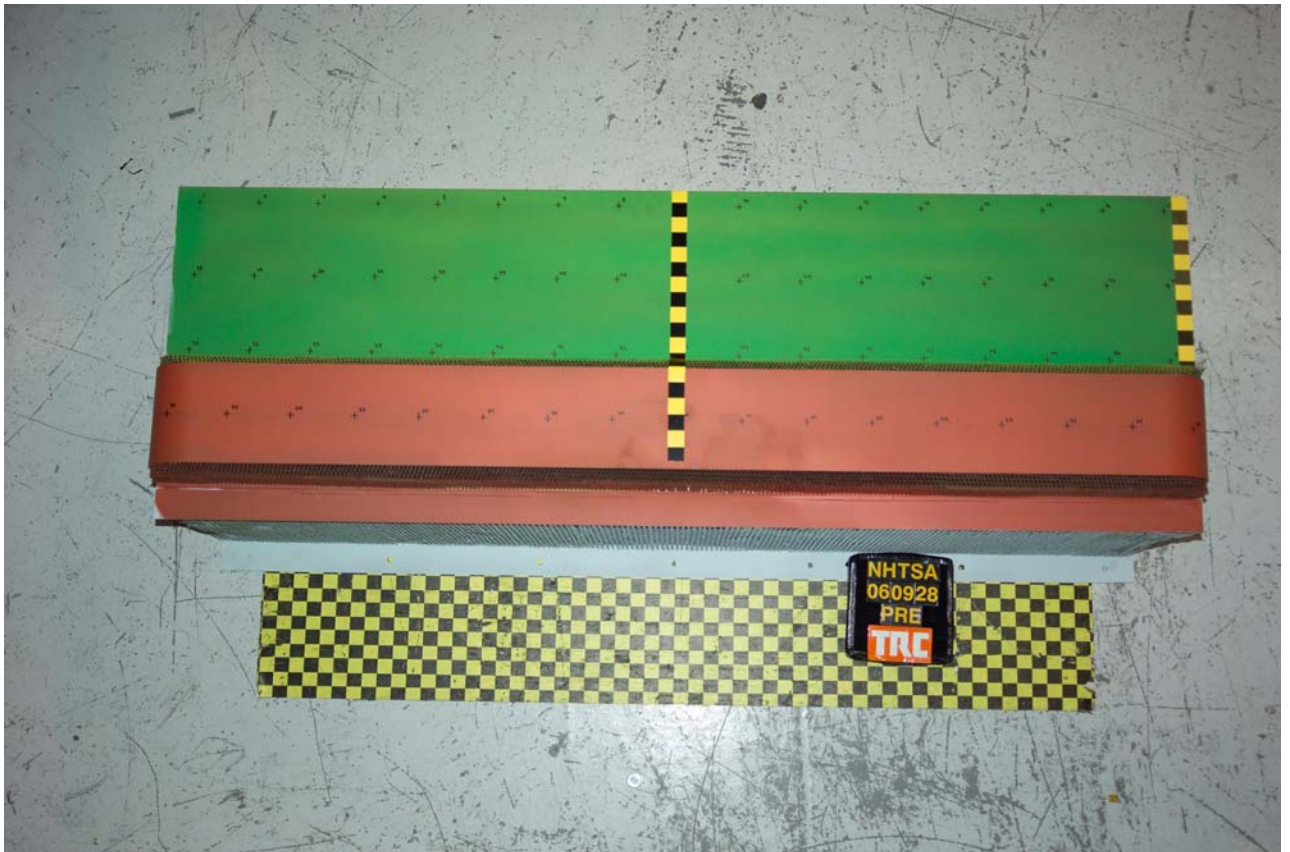
Figure A-50 Pre-Test Front View of Barrier Face
