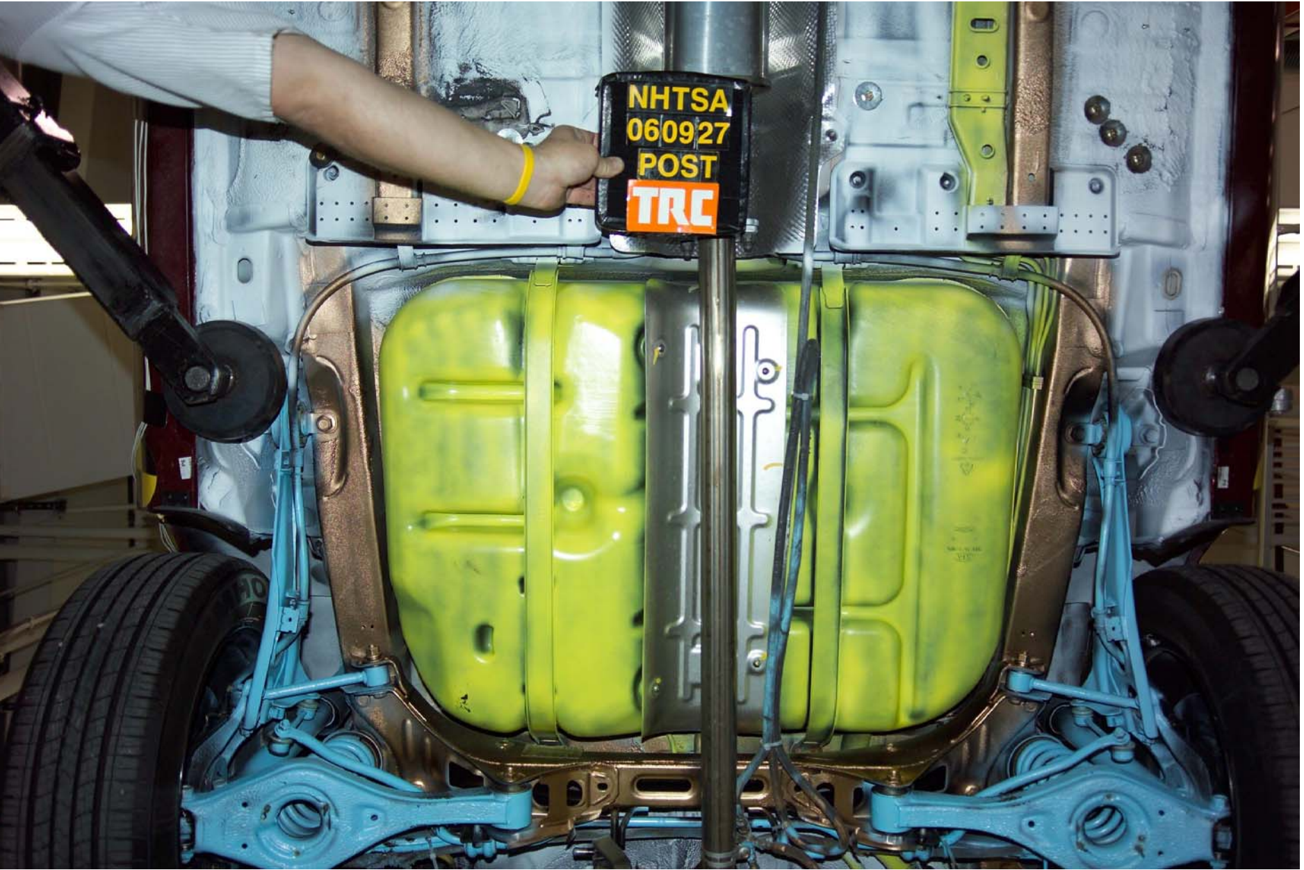
Figure A-32 Post-Test Fuel Tank View
