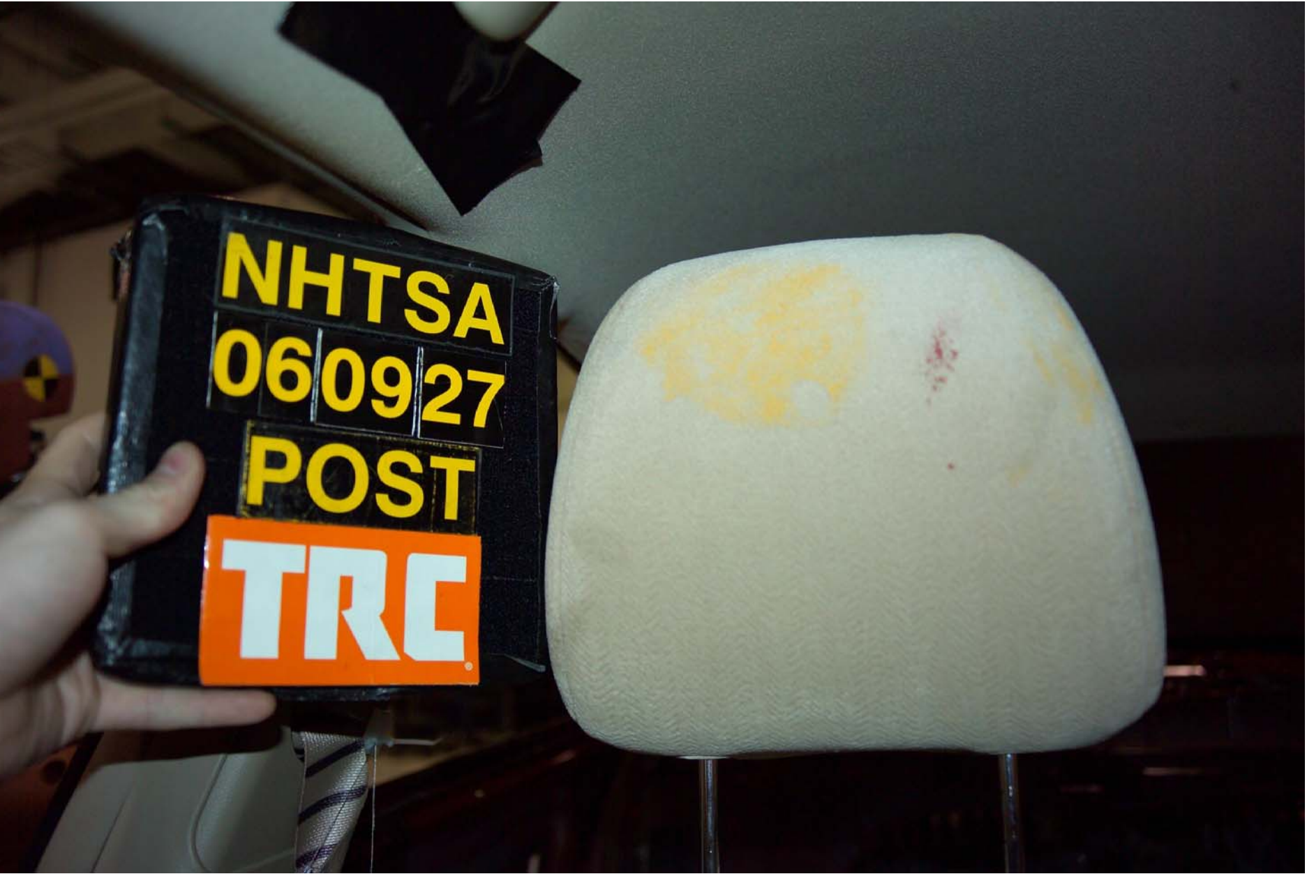
Figure A-74 Post-Test Right Front Passenger Dummy Head Contact - View 3
