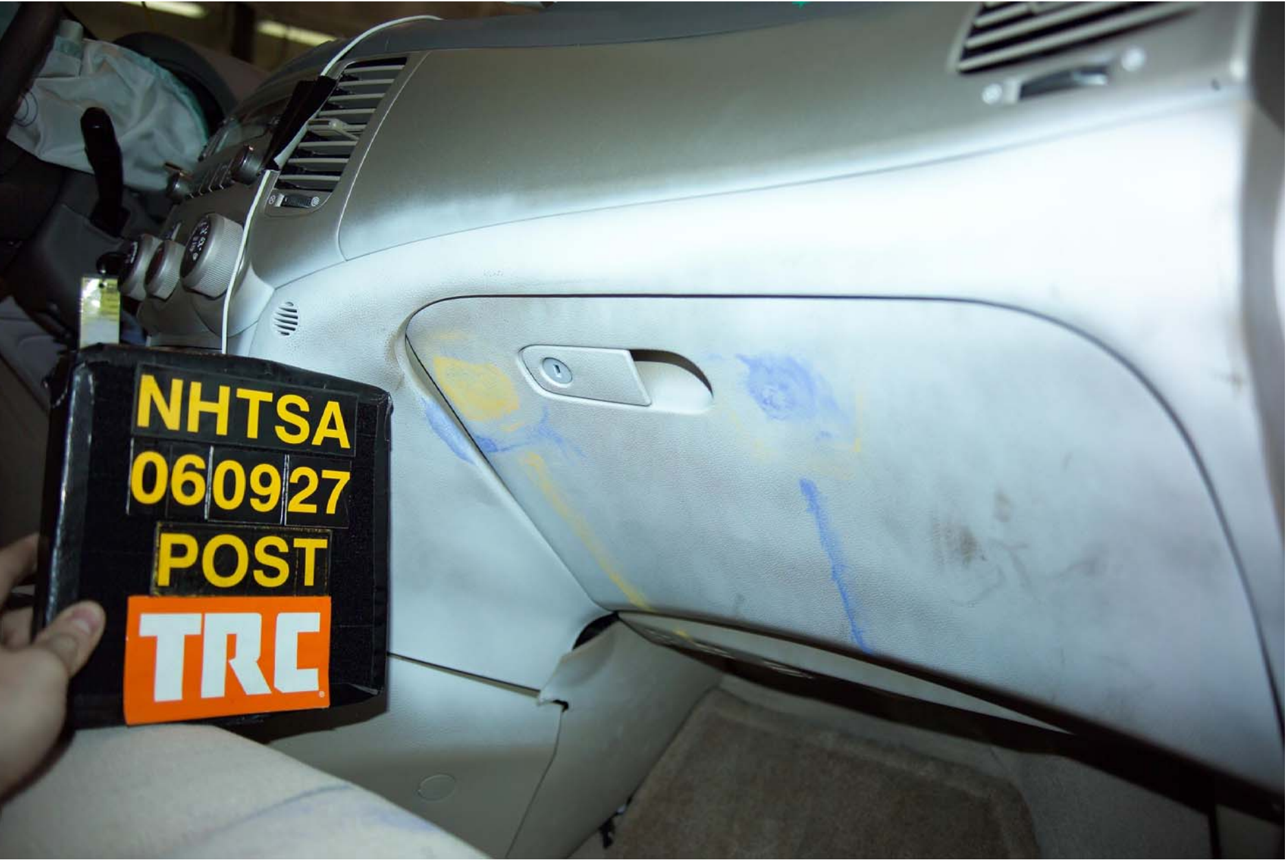
Figure A-76 Post-Test Right Front Passenger Dummy Knee Contact - View 2
