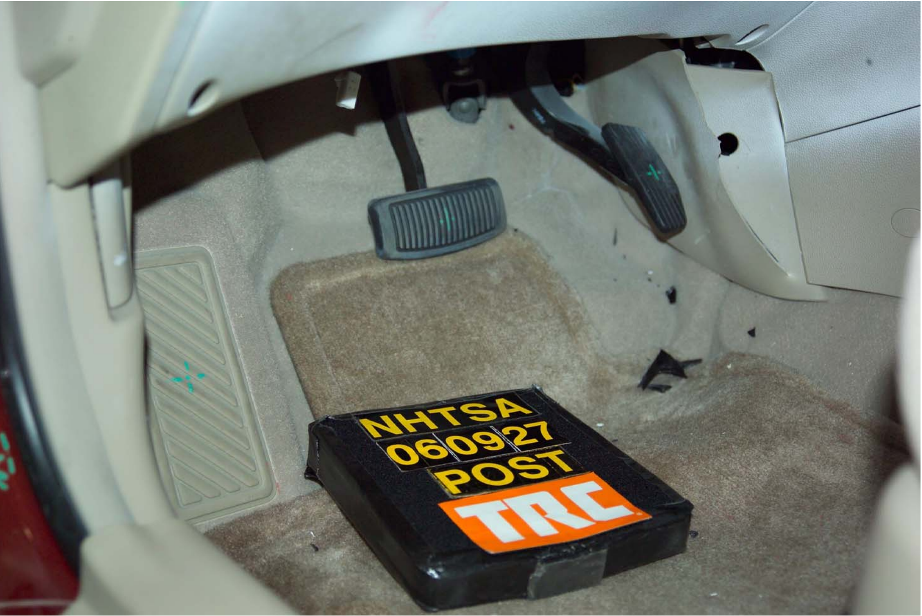
Figure A-60 Post-Test Driver Toeboard Deformation View
