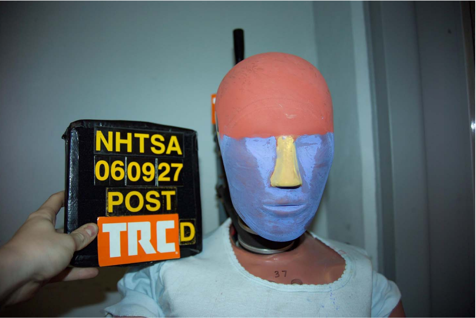
Figure A-54 Post-Test Driver Dummy Head Contact - View 1
