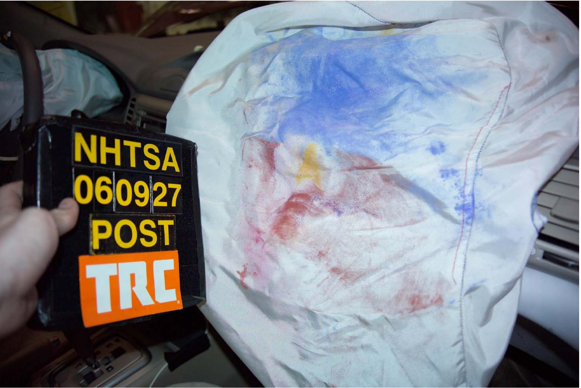
Figure A-73 Post-Test Right Front Passenger Dummy Head Contact - View 2
