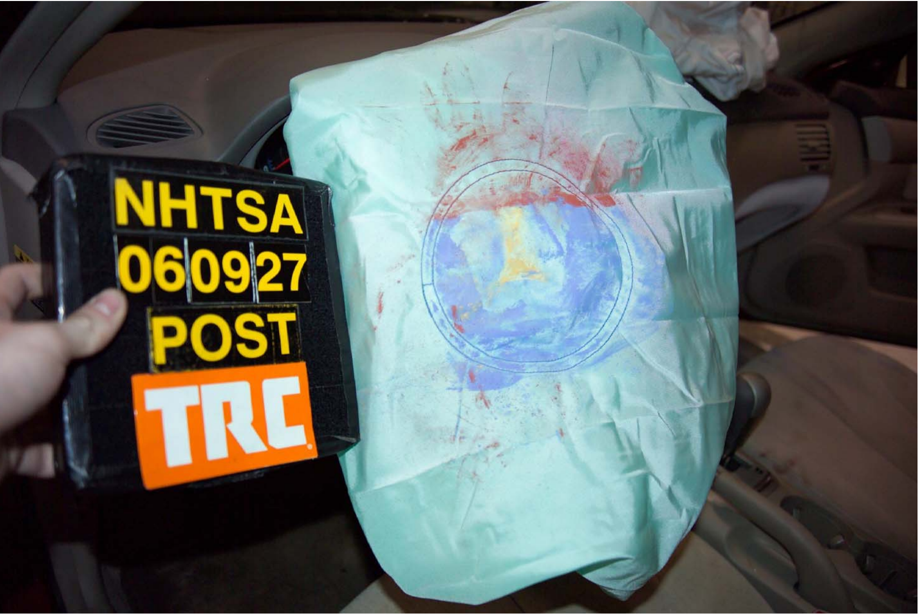
Figure A-55 Post-Test Driver Dummy Head Contact - View 2
