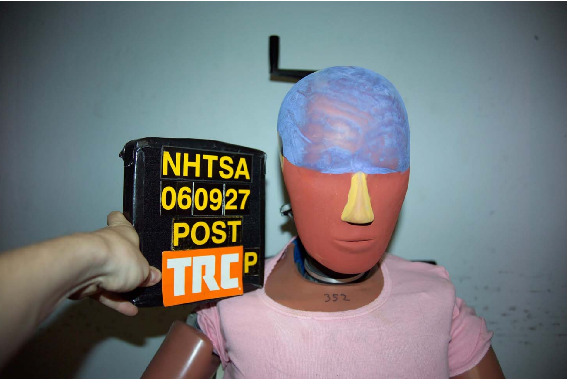
Figure A-72 Post-Test Right Front Passenger Dummy Head Contact - View 1
