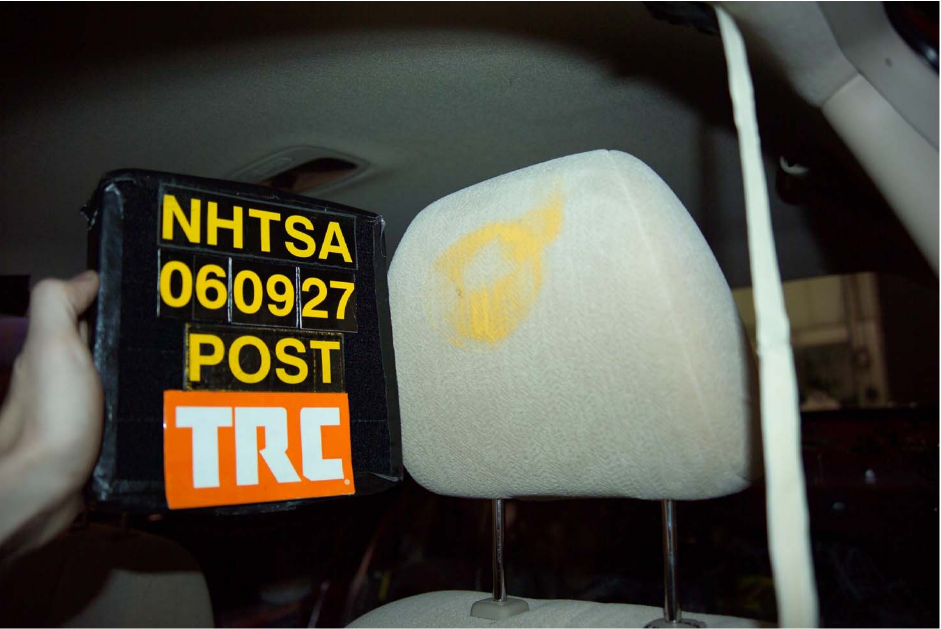
Figure A-56 Post-Test Driver Dummy Head Contact - View 3
