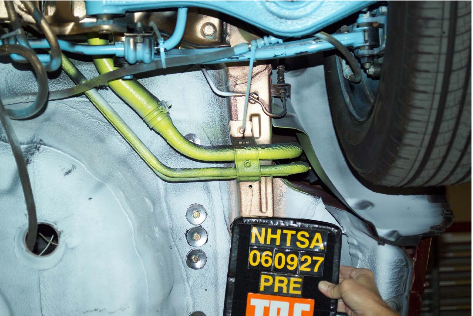
Figure A-33 Pre-Test Fuel Filler Neck View
