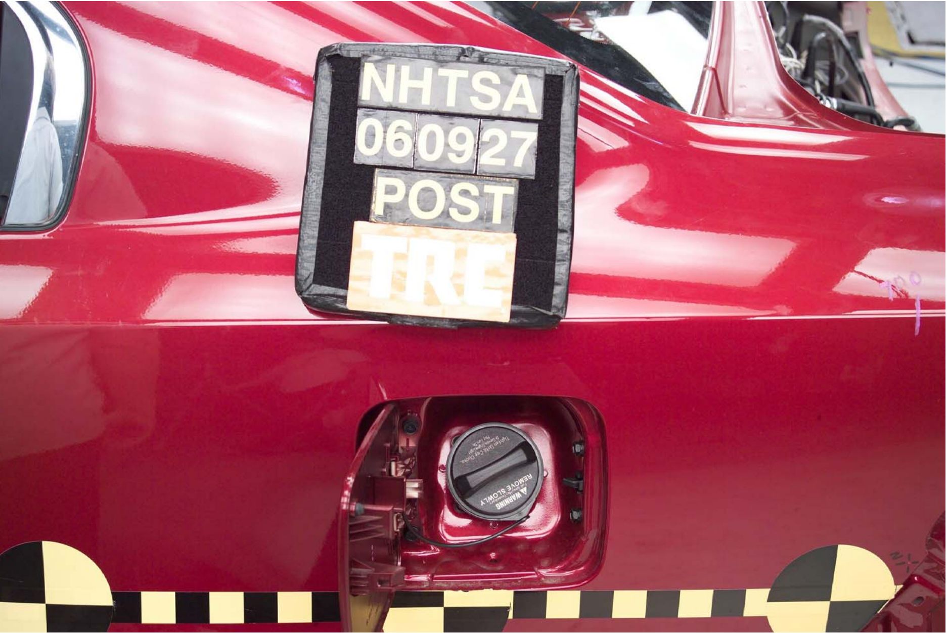
Figure A-36 Post-Test Fuel Filler Cap View
