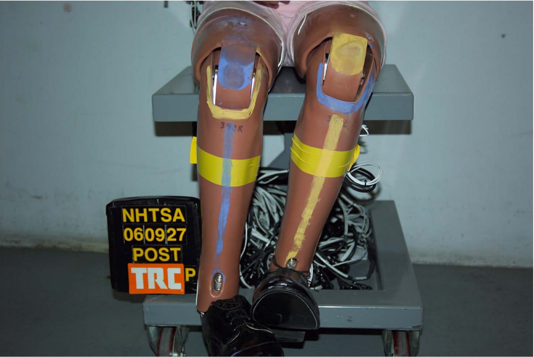
Figure A-75 Post-Test Right Front Passenger Dummy Knee Contact - View 1
