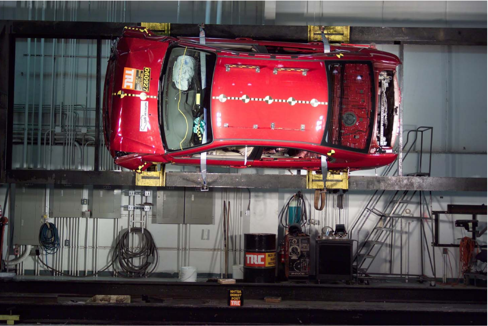
Figure A-83 FMVSS 301 Rollover View at 90°
