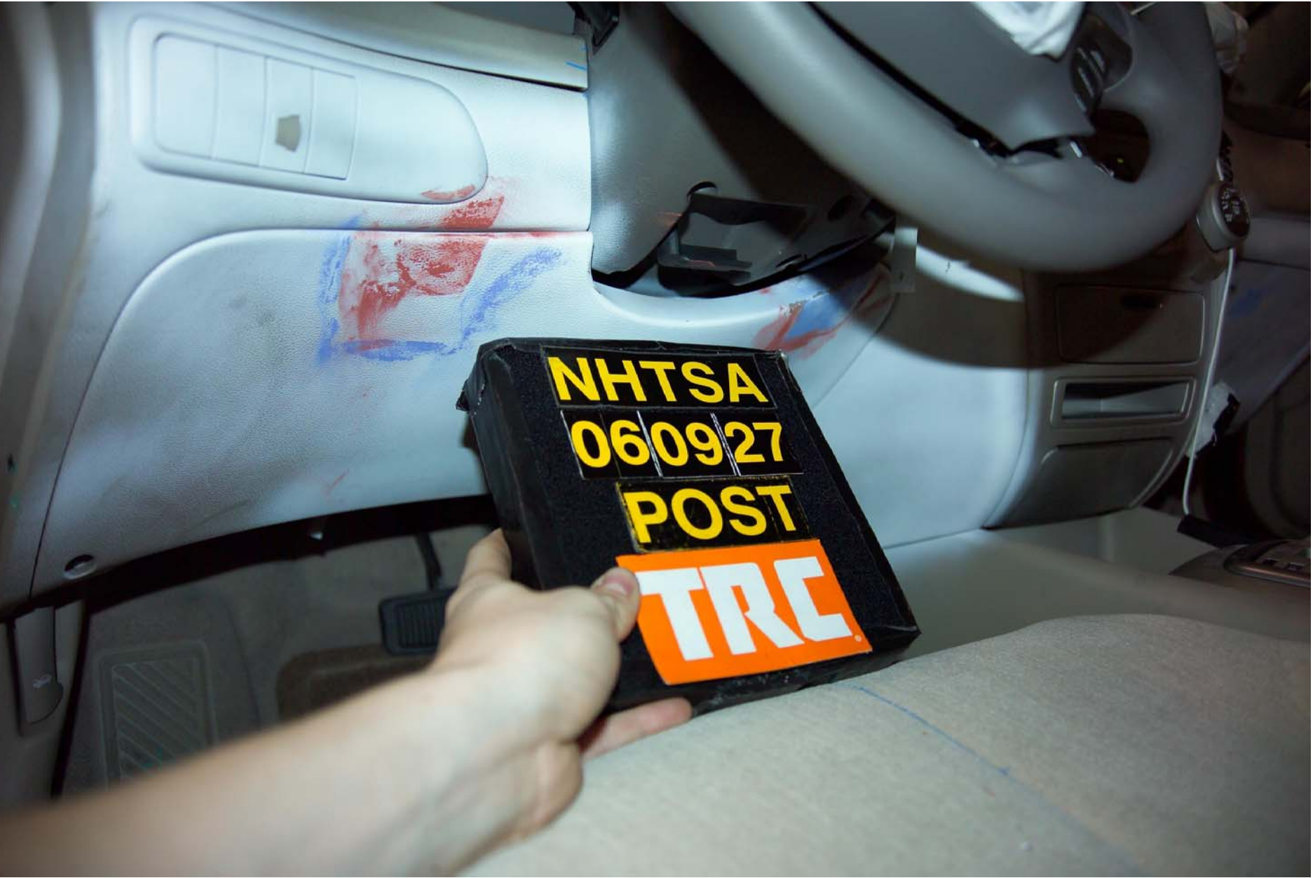
Figure A-58 Post-Test Driver Dummy Knee Contact - View 2
