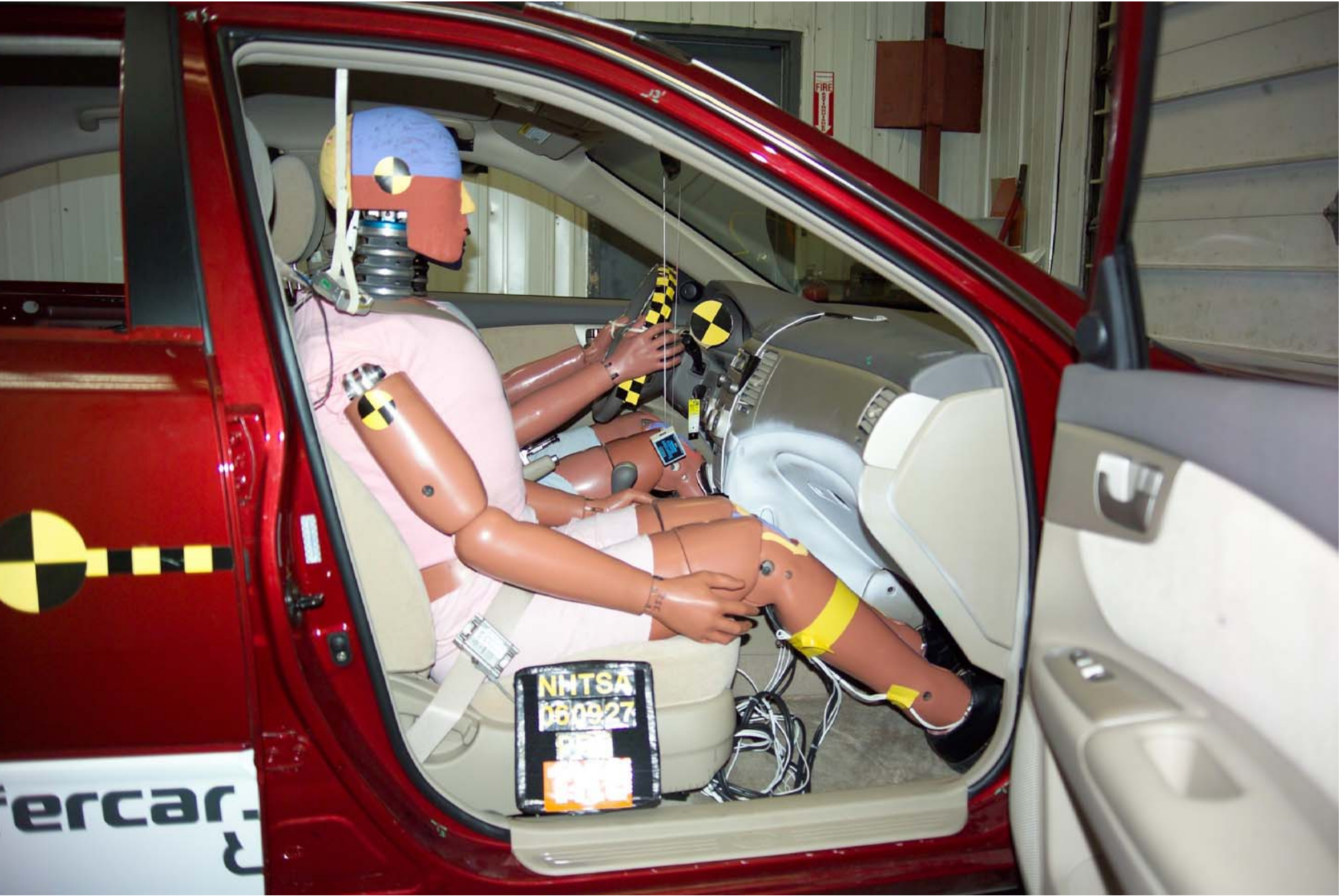
Figure A-65 Pre-Test Right Front Passenger Dummy - View 3
