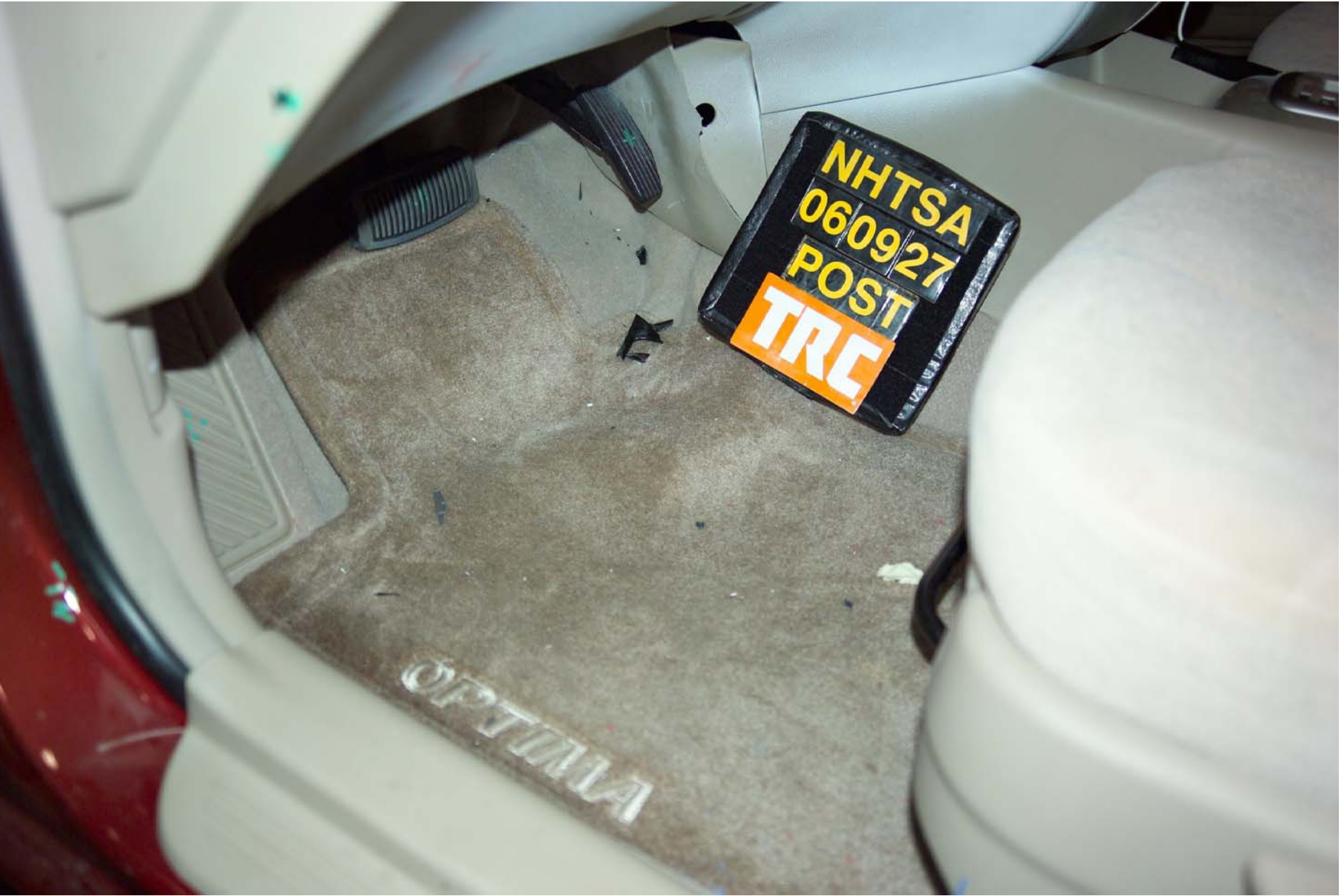
Figure A-59 Post-Test Driver Floorboard Deformation View
