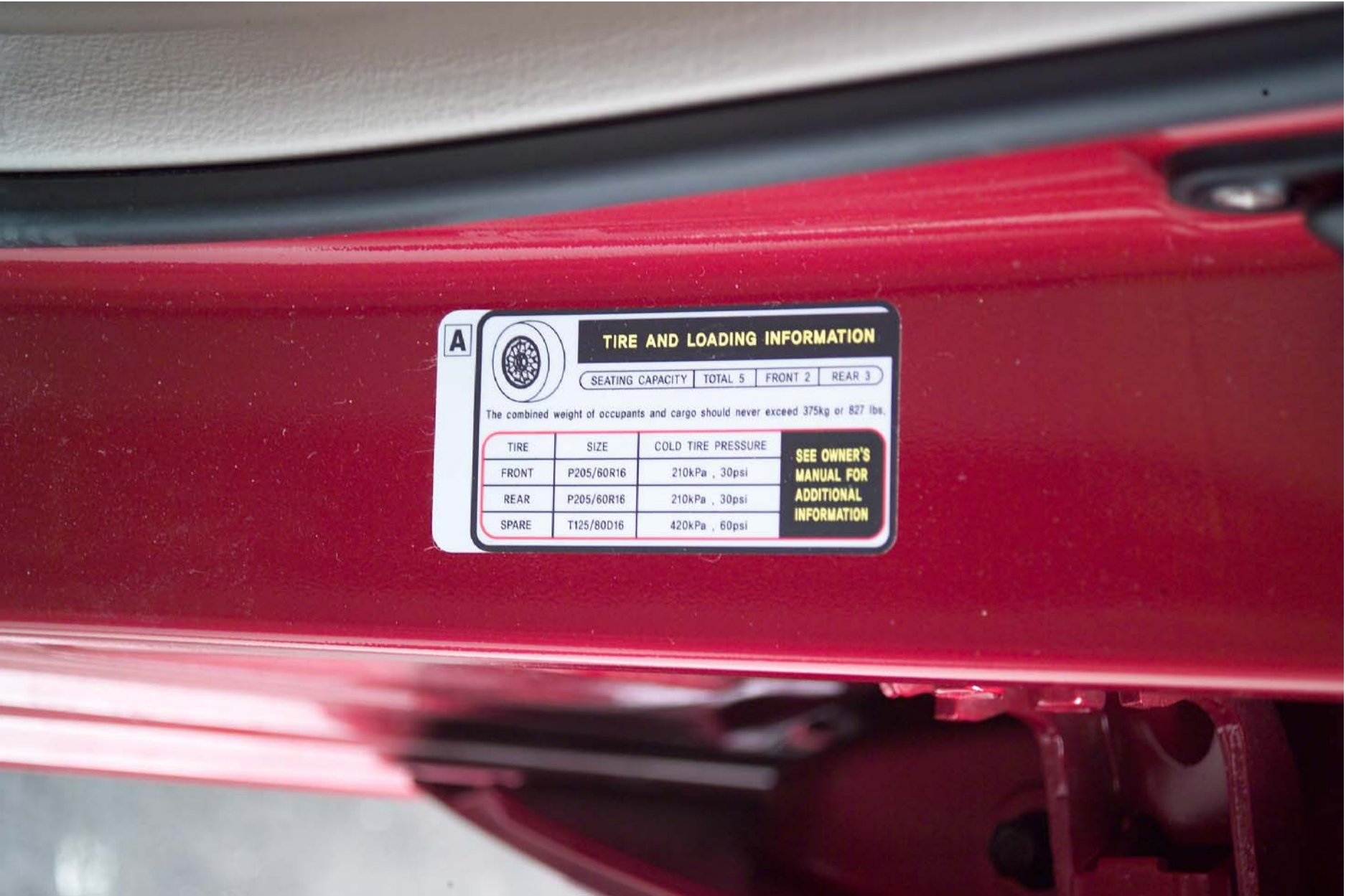
Figure A-82 Vehicle Tire Load Label View
