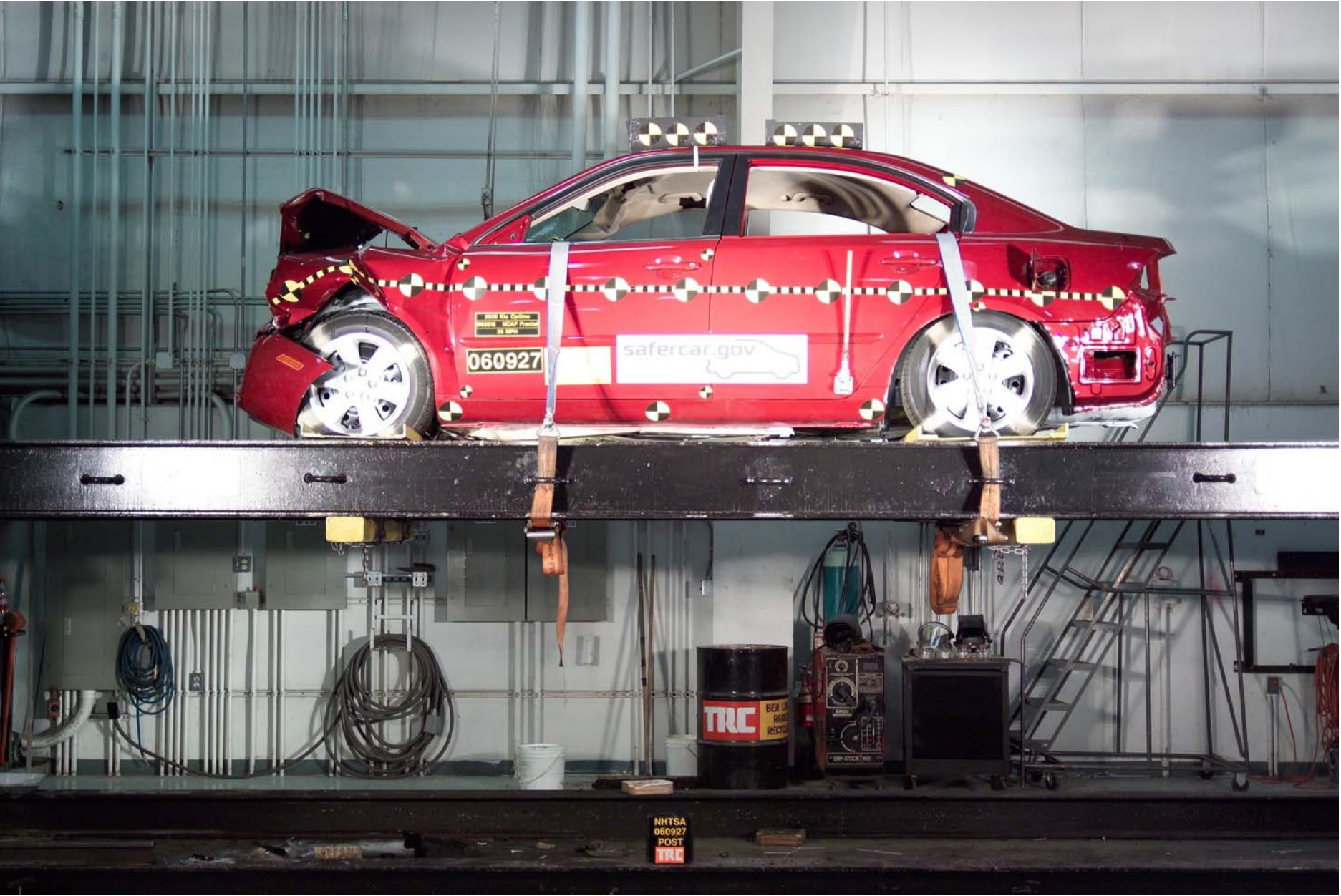
Figure A-86 FMVSS 301 Rollover View at 360°
