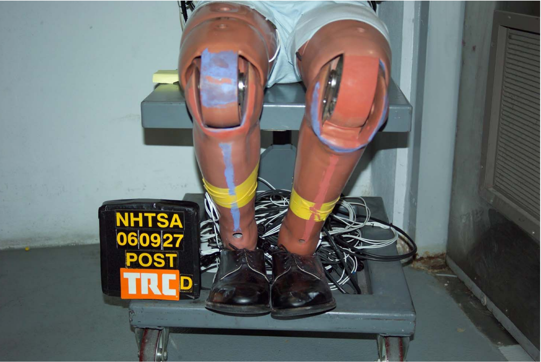
Figure A-57 Post-Test Driver Dummy Knee Contact - View 1
