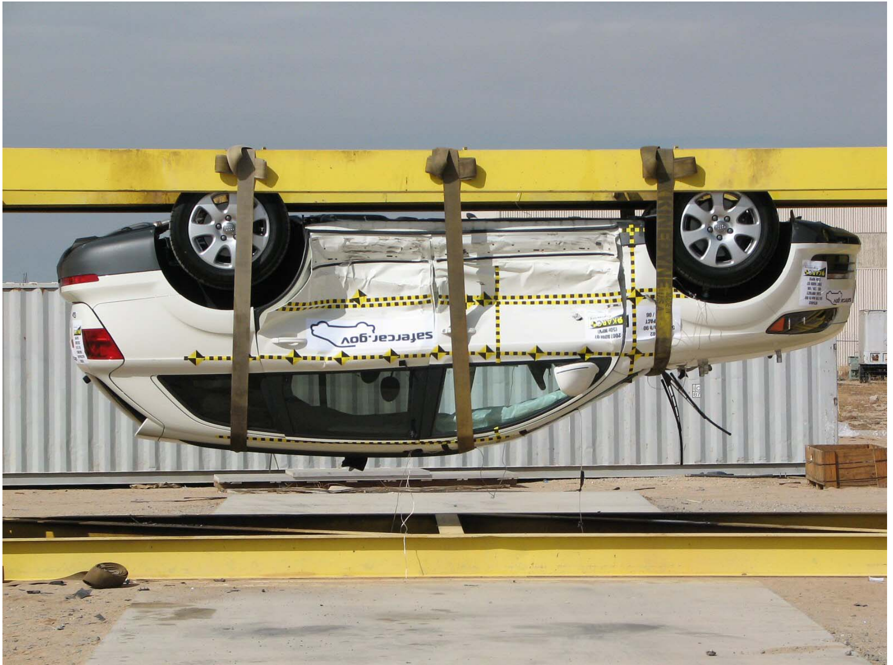
Figure A-63: Vehicle on Rollover Device (180°)
