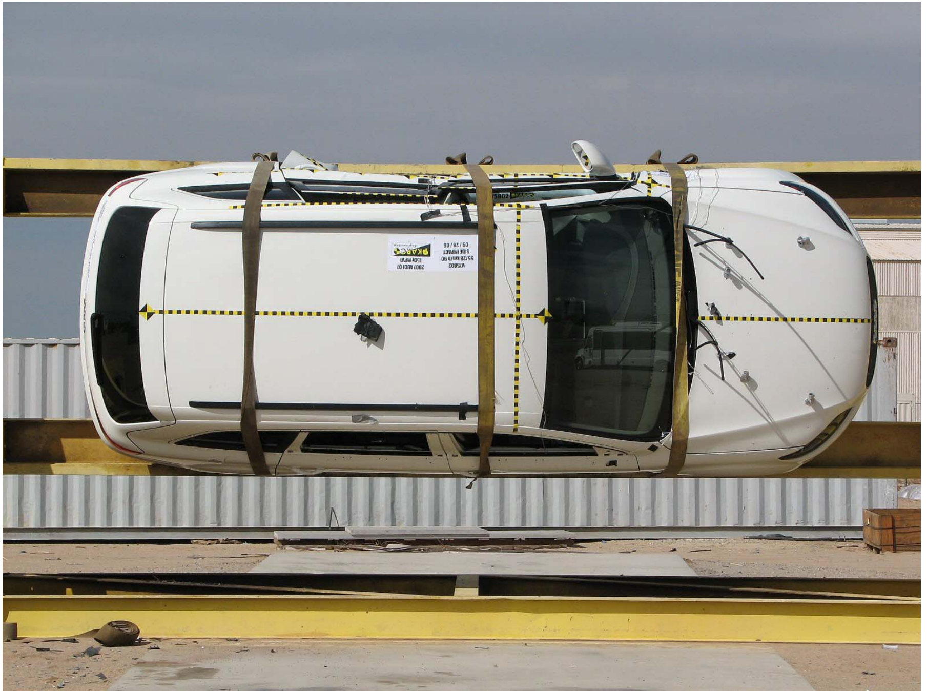
Figure A-62: Vehicle on Rollover Device (90°)
