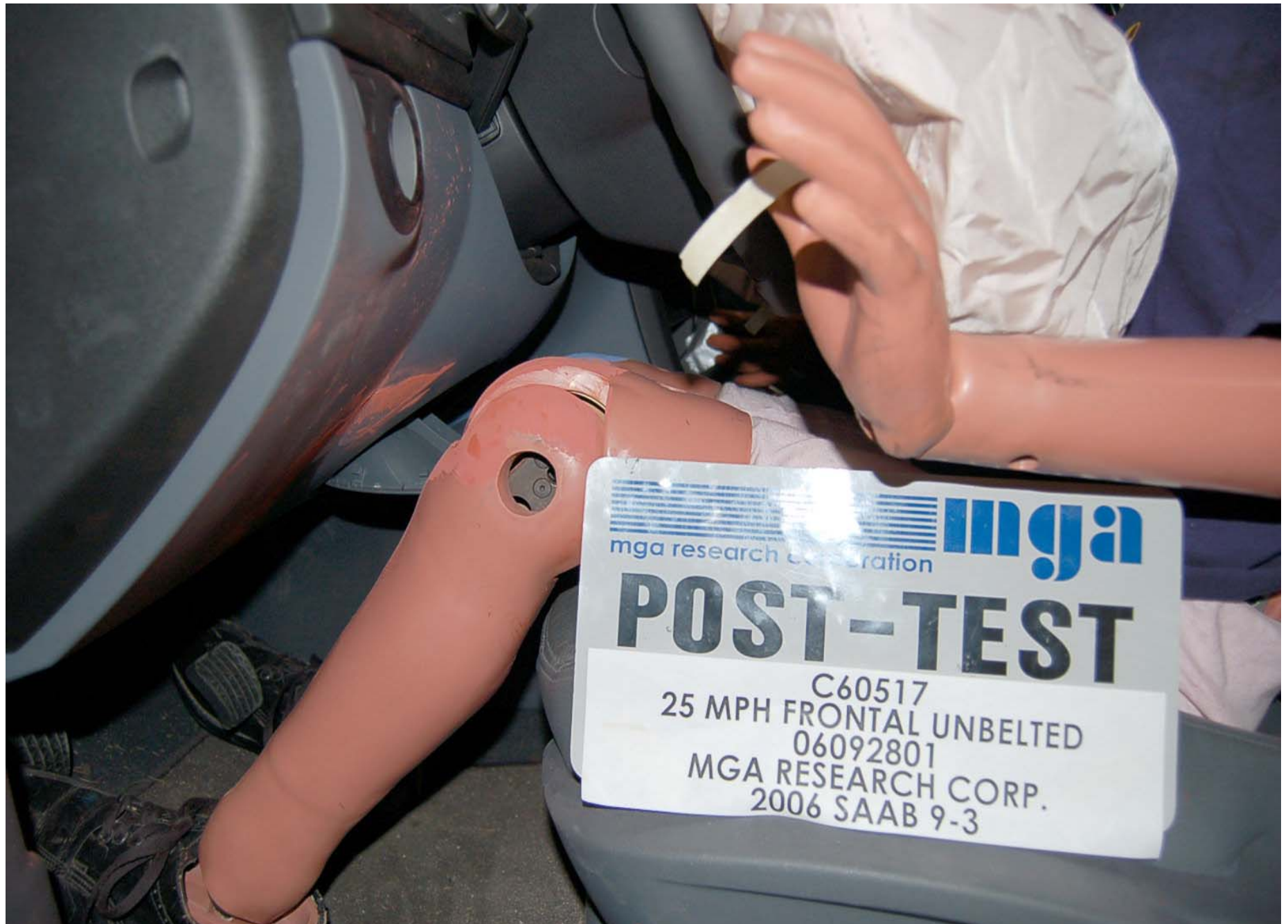
Post-Test Driver Side Knee Bolster View
