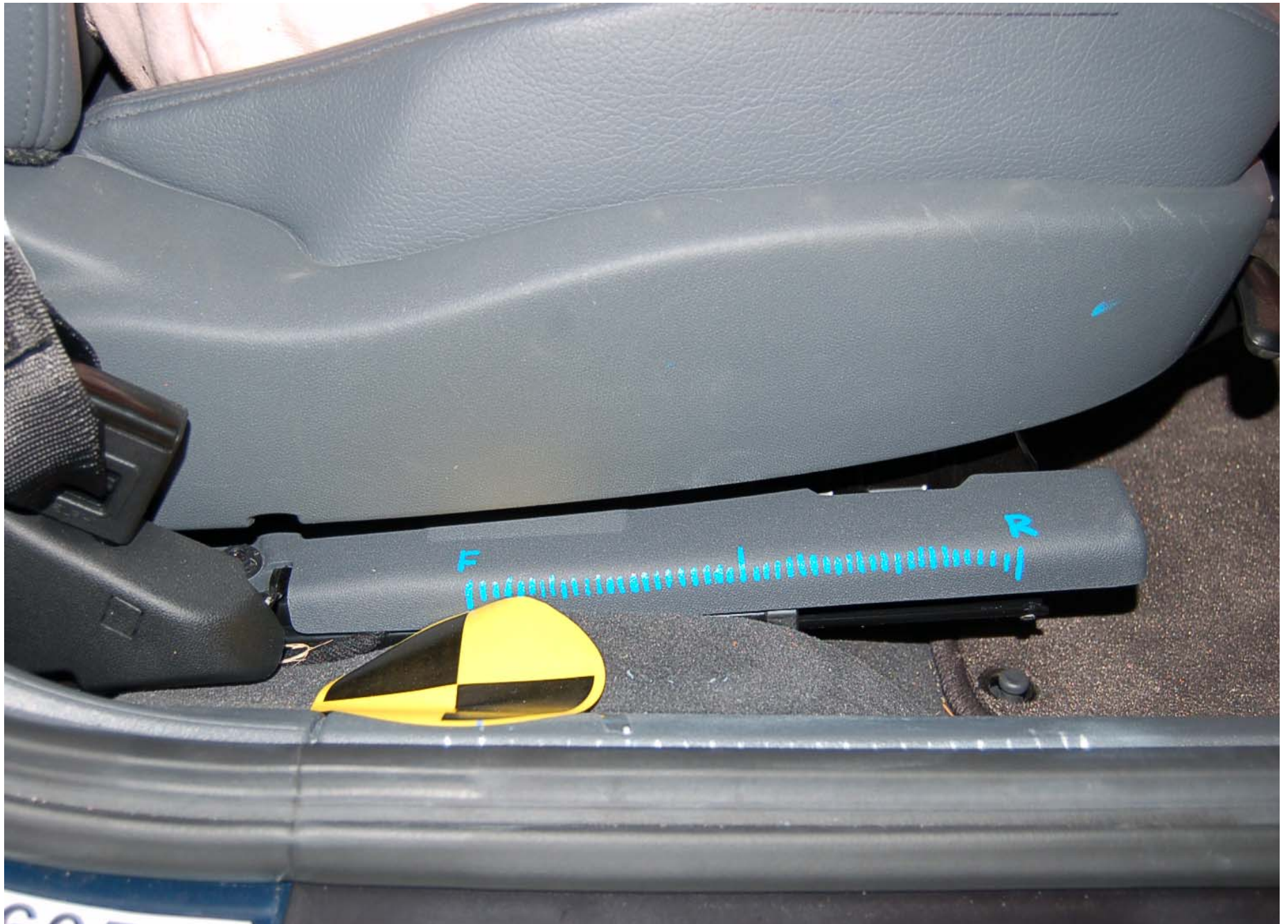
Pre-Test Passenger Dummy Seat Position
