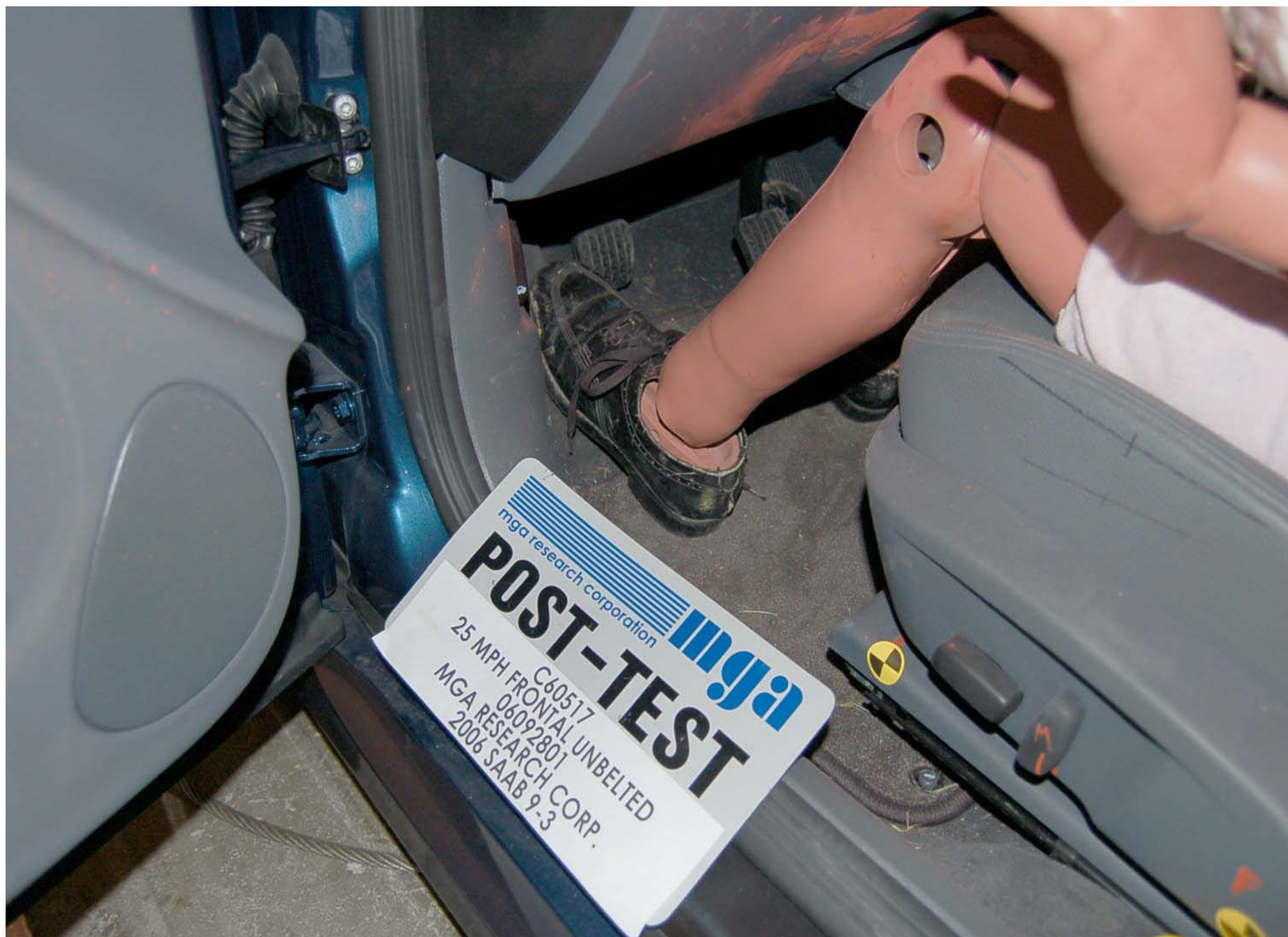
Post-Test Driver Dummy Feet Position
