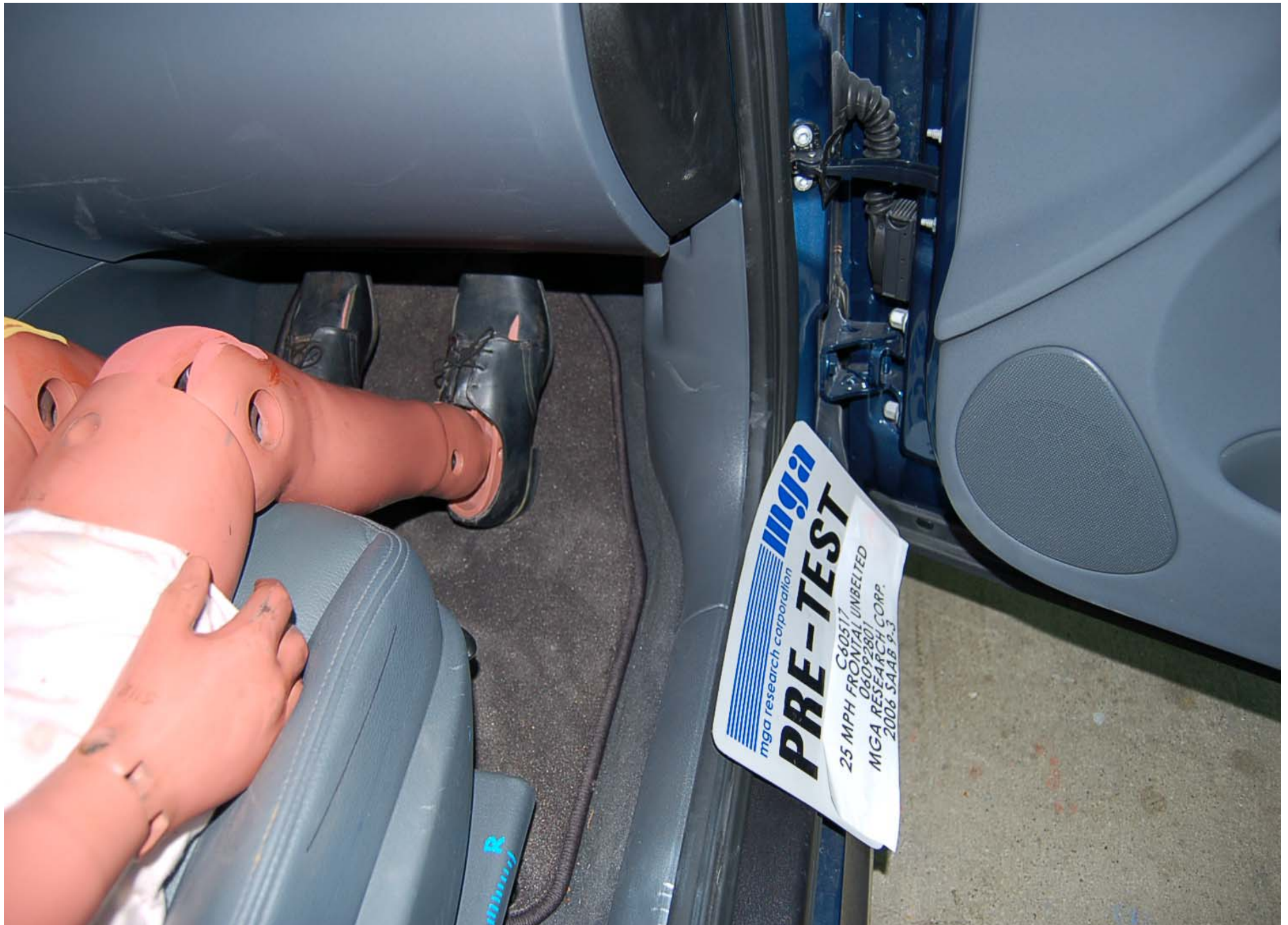
Pre-Test Passenger Dummy Feet Position
