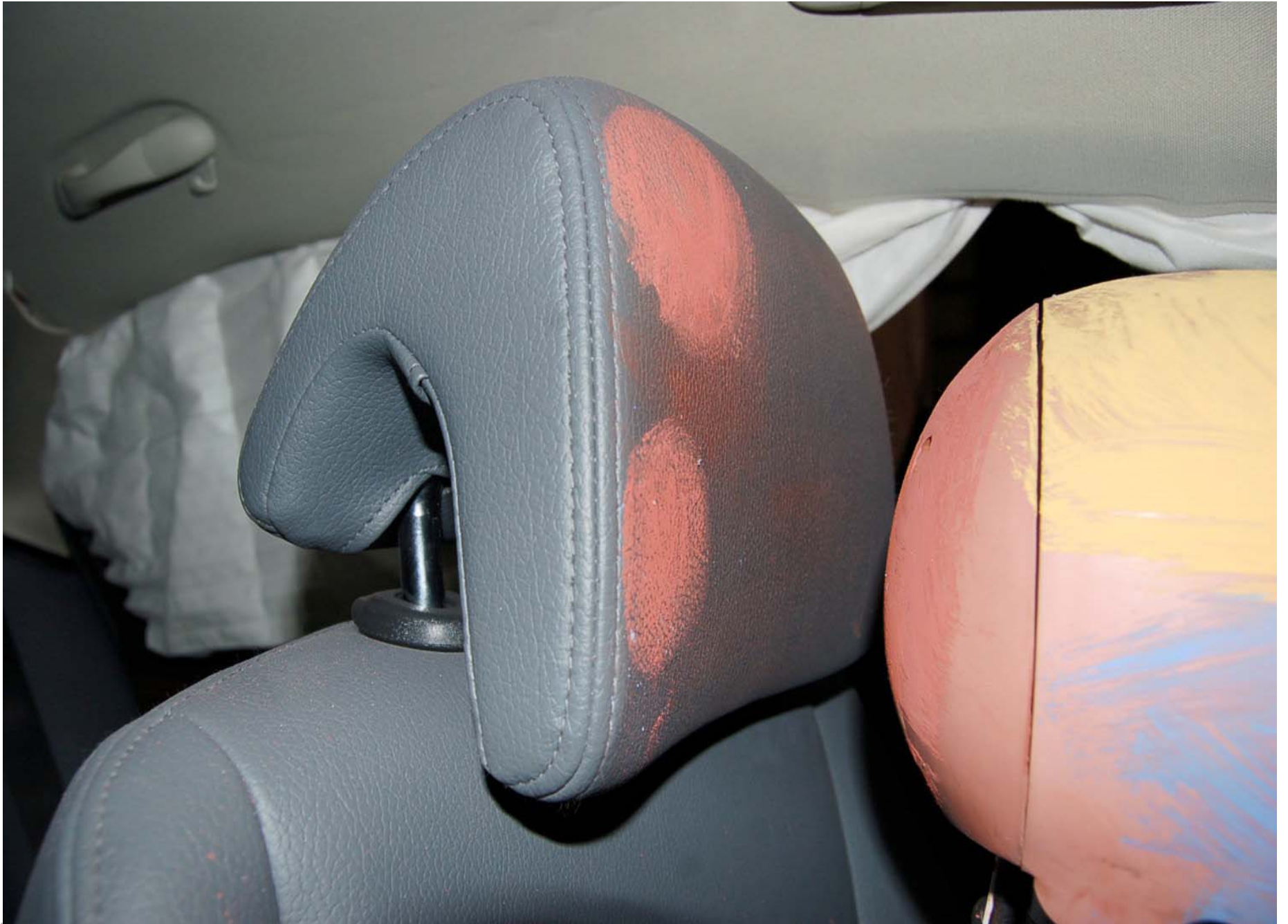
Post-Test Driver Dummy Head Contact (head rest)
