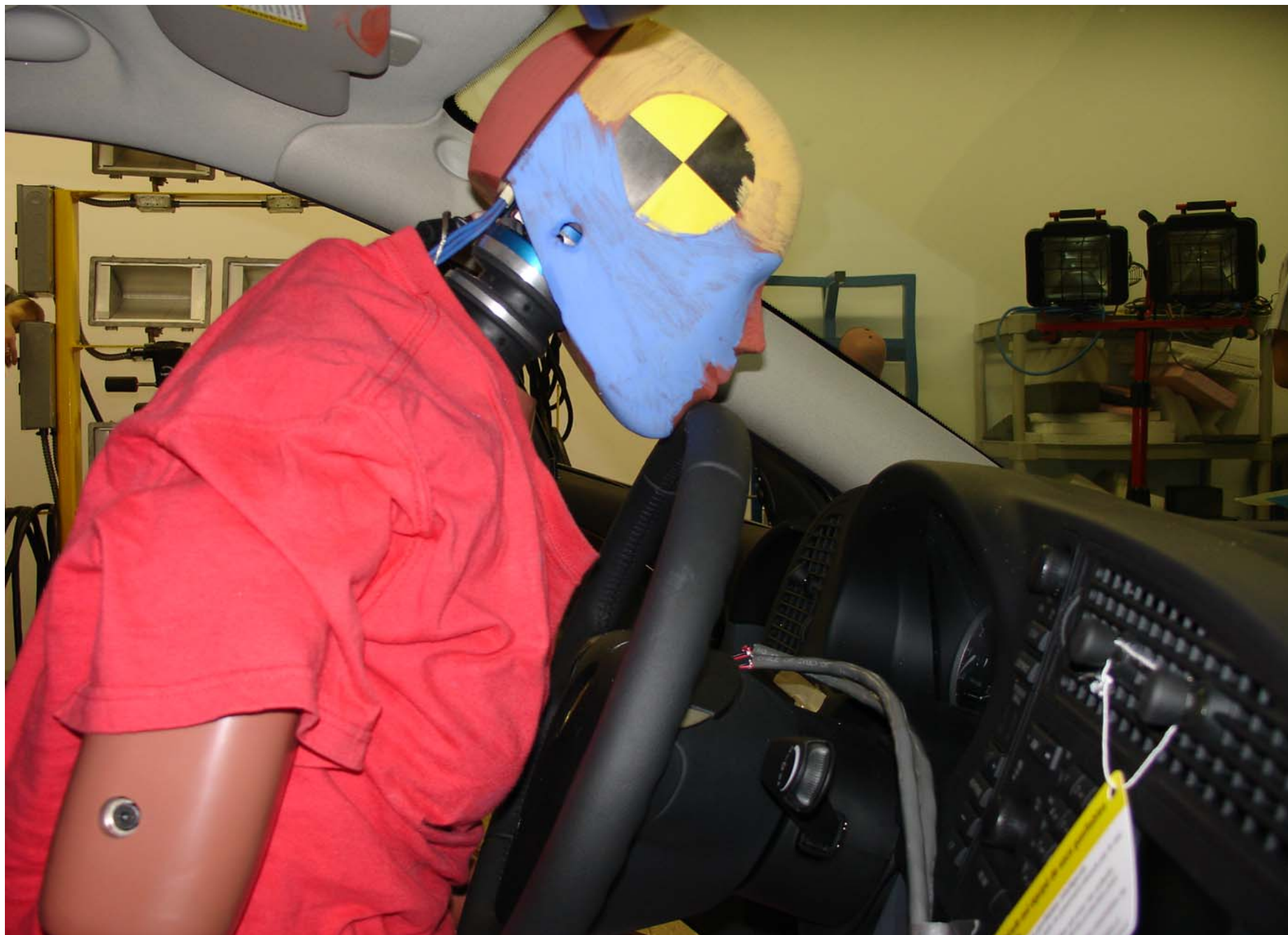
Pre-Test 5th Fem. P2 Trial 2 Driver Dummy Right Side Head Position View
