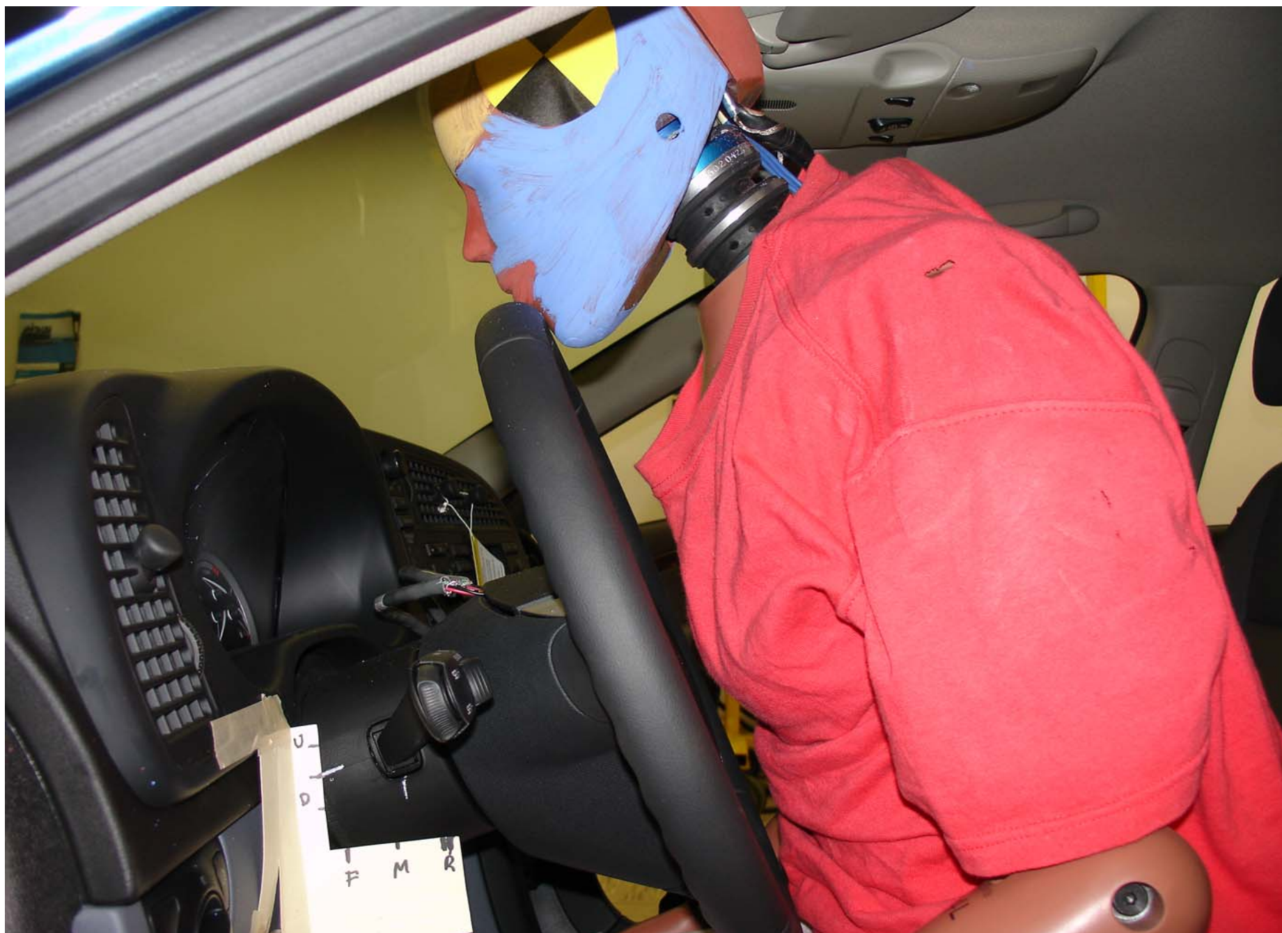
Pre-Test 5th Fem. P2 Trial 2 Driver Dummy Left Side Head Position View
