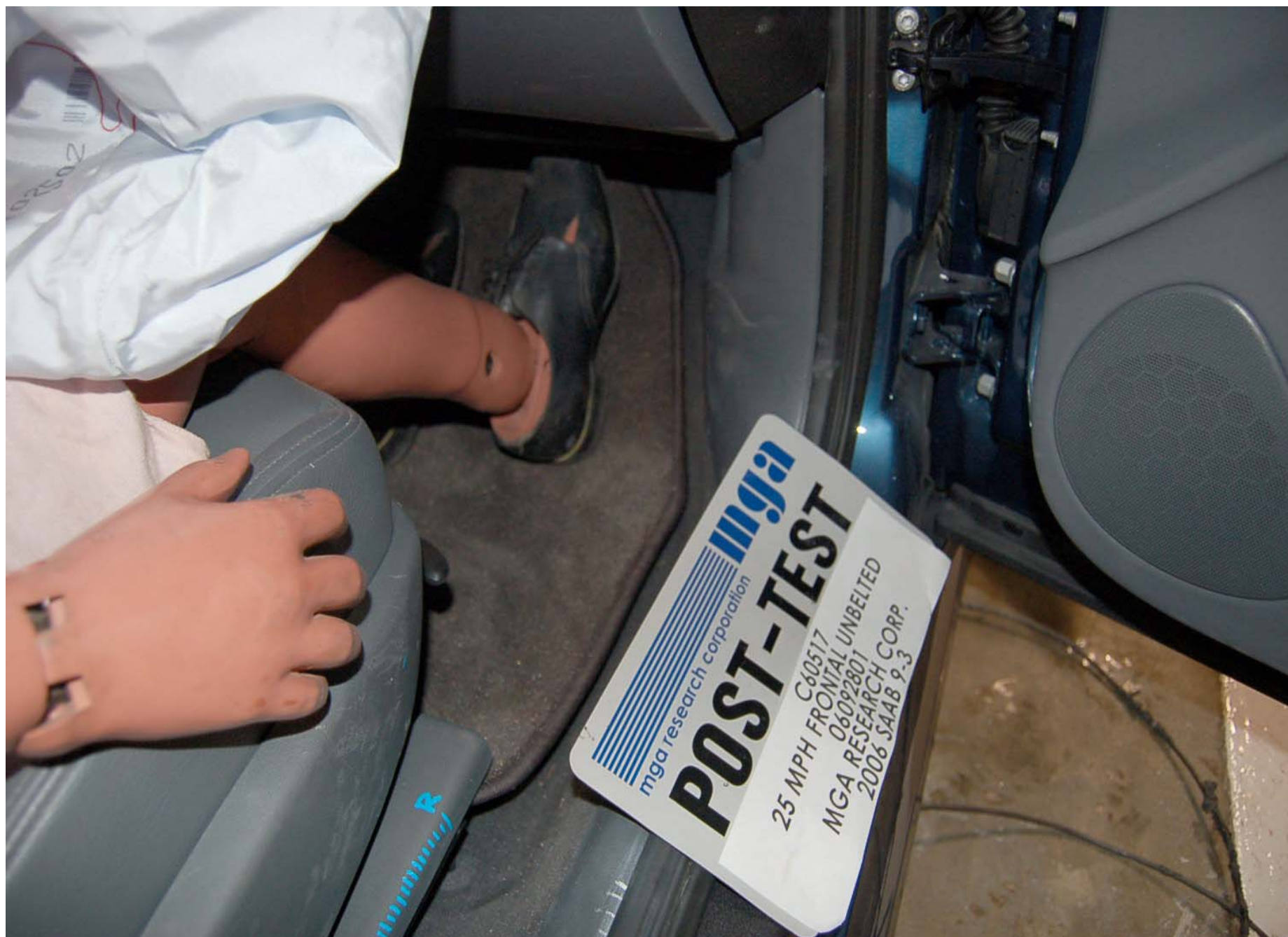
Post-Test Passenger Dummy Feet Position
