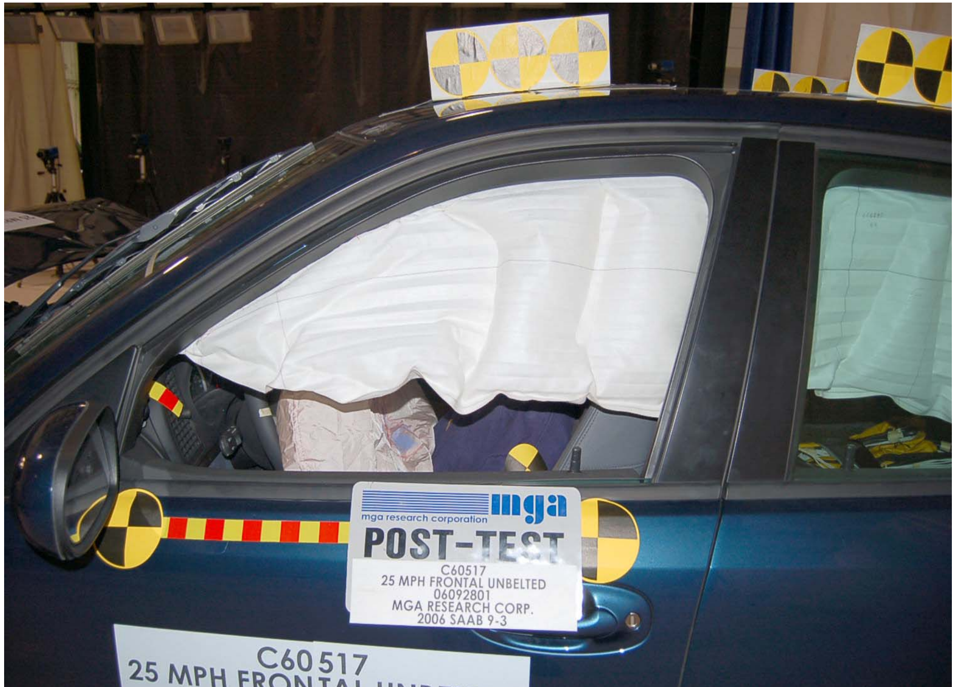
Post-Test Driver Dummy Position Left Side View
