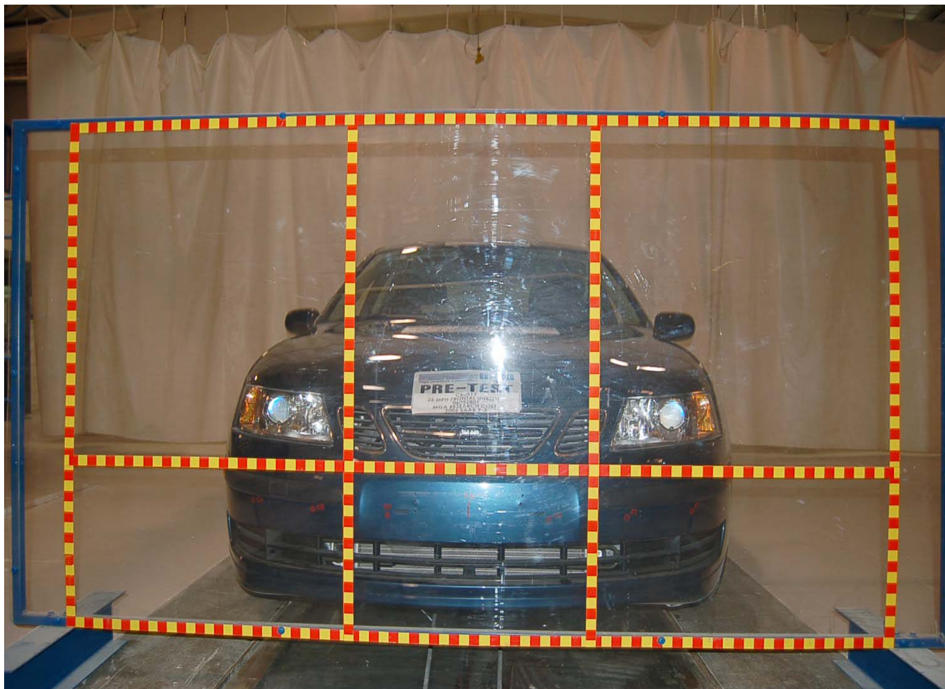
Vehicle in Relation to The Load Cell Grid
