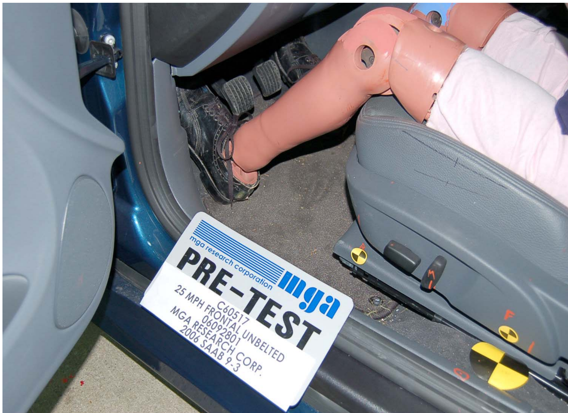
Pre-Test Driver Dummy Feet Position
