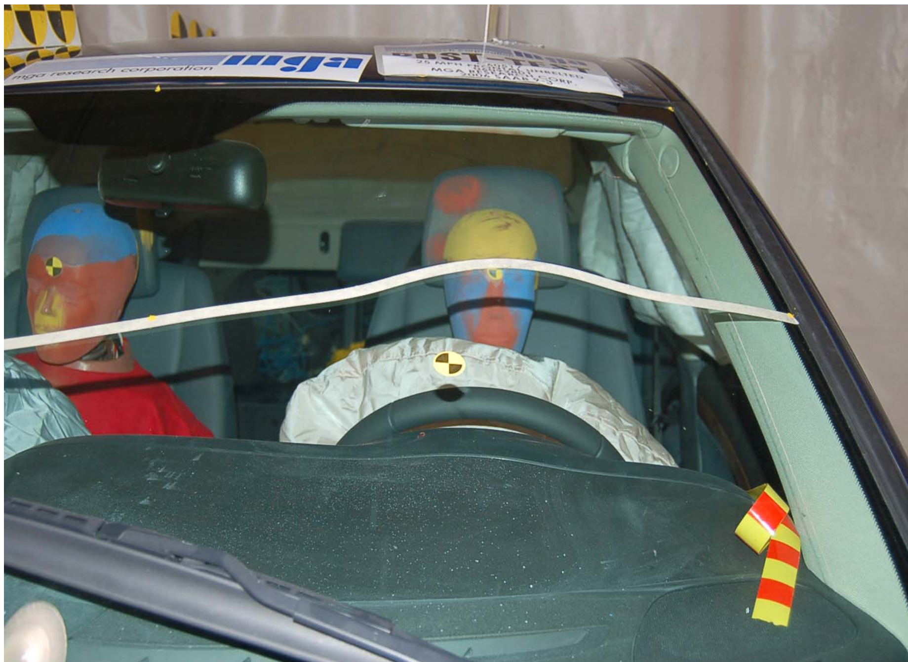
Post-Test Driver Dummy Front View (head position)
