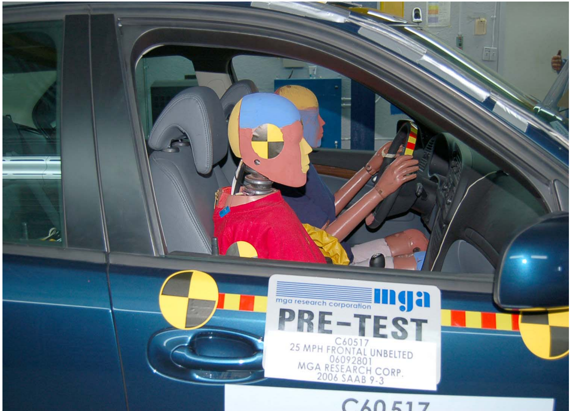
Pre-Test Passenger Dummy Position Right Side View
