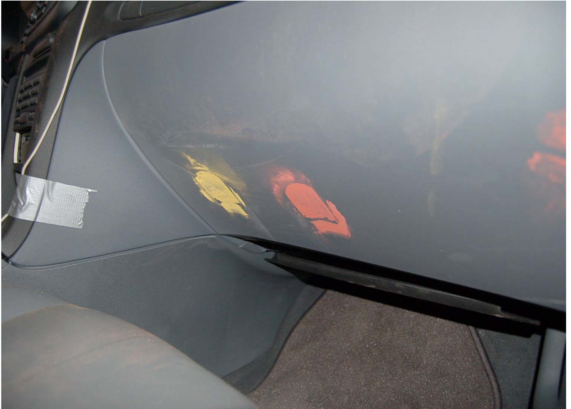
Post-Test Passenger Dummy Knee Contact
