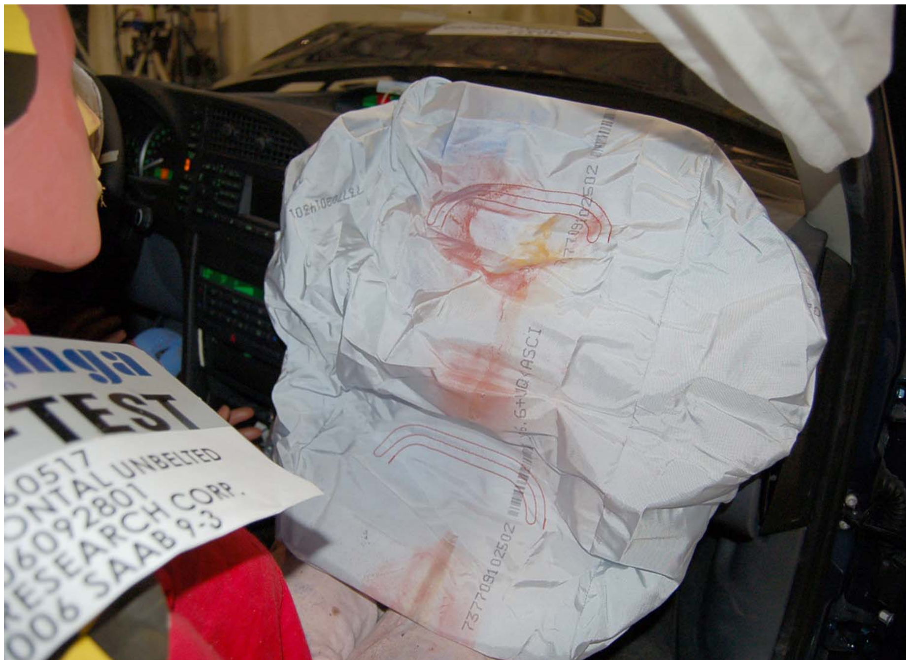
Post-Test Passenger Dummy Airbag Contact
