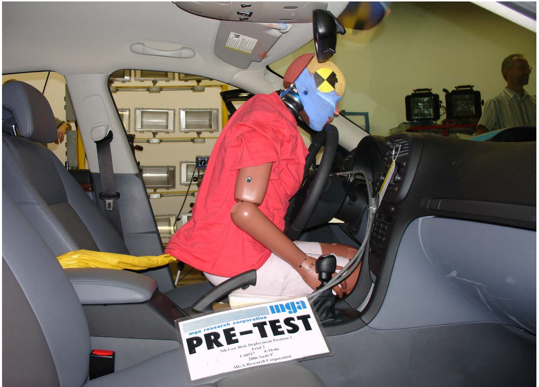
Pre-Test 5th Fem. P2 Trial 2 Driver Dummy Right Side View (Door Open)
