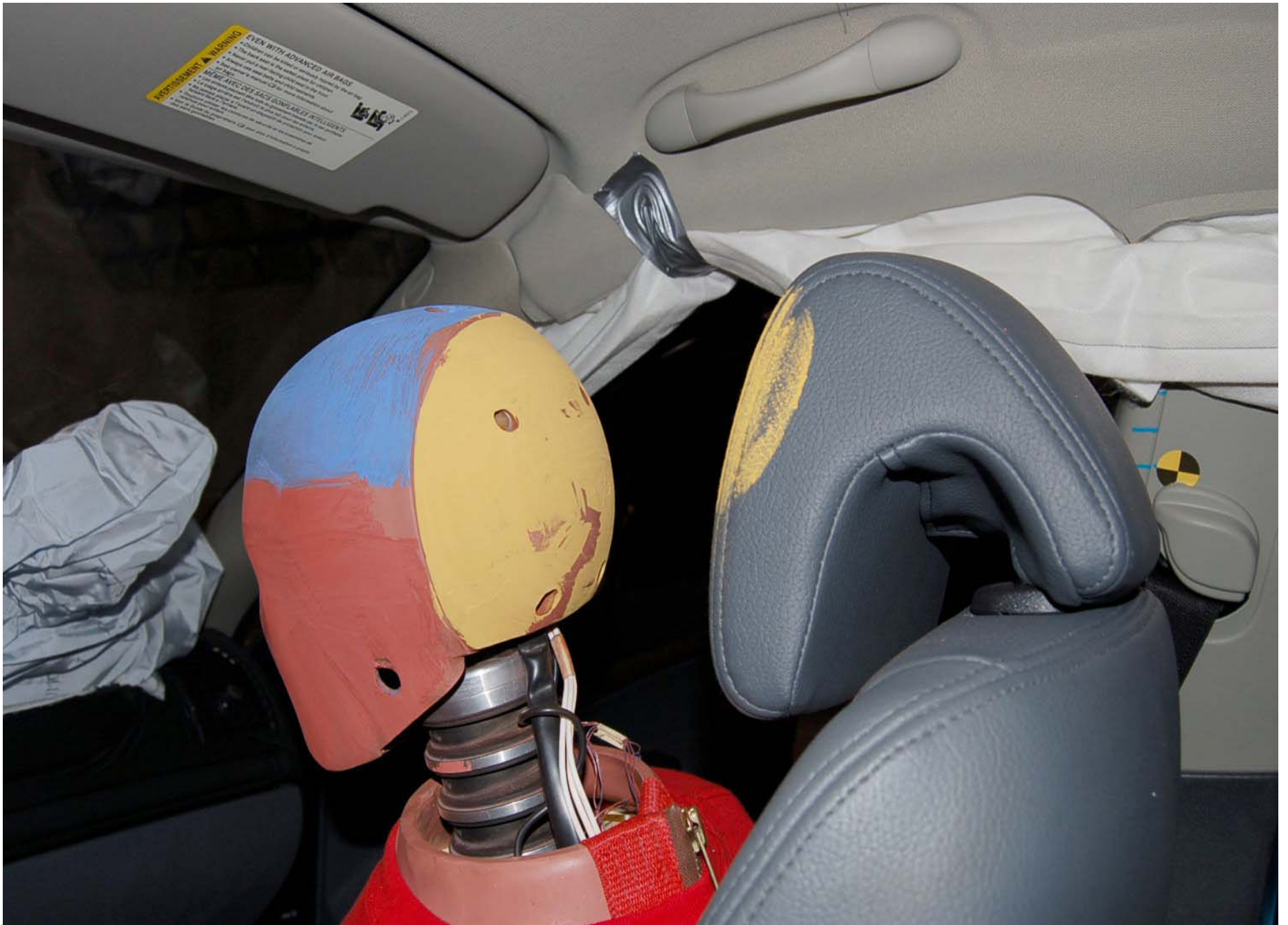
Post-Test Passenger Dummy Head Contact (head rest)
