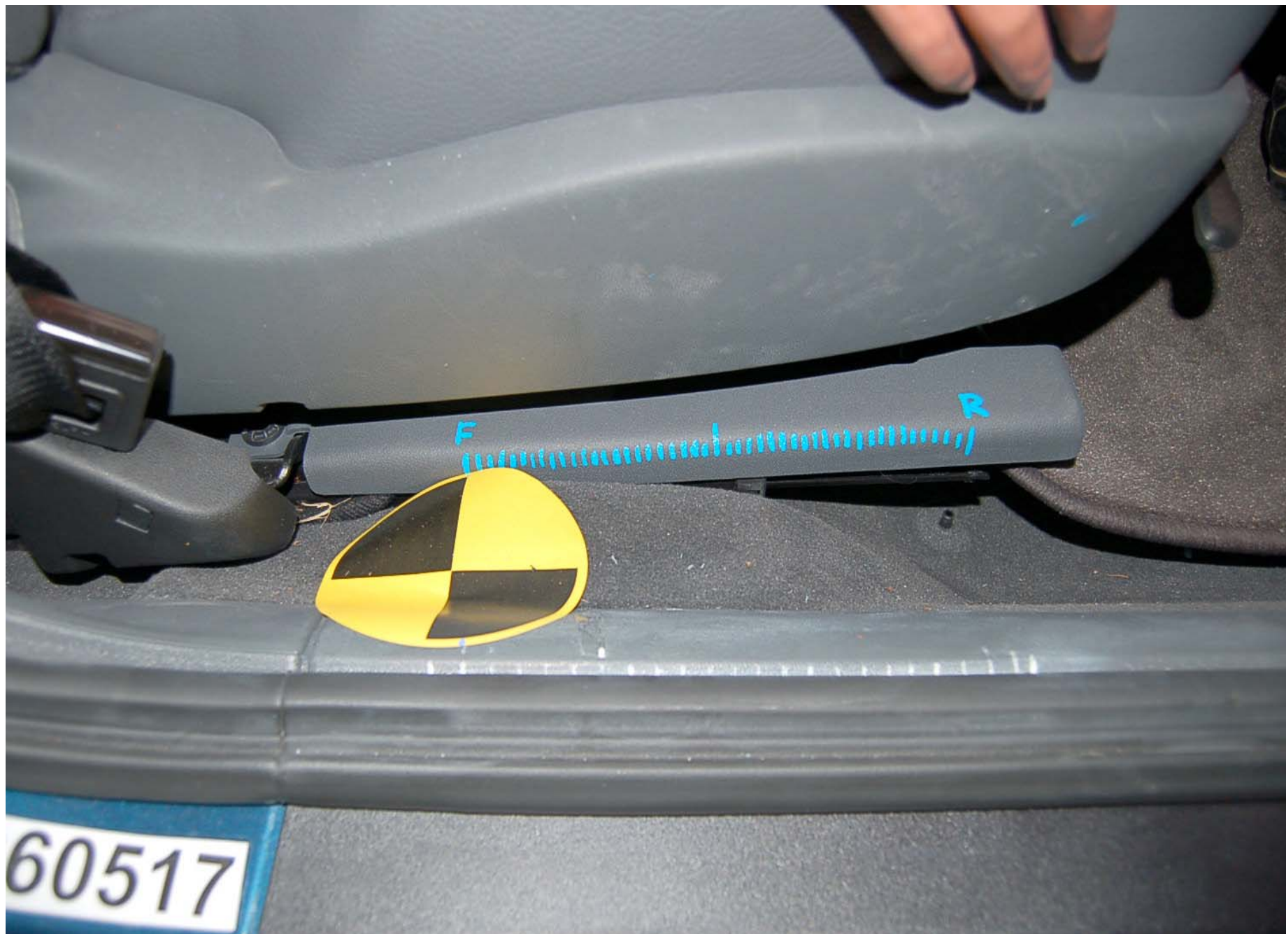
Post-Test Passenger Dummy Seat Position
