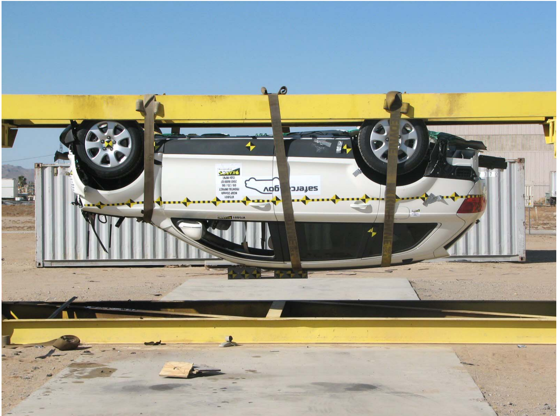
Figure A-60: Vehicle on Rollover Device (180°)
