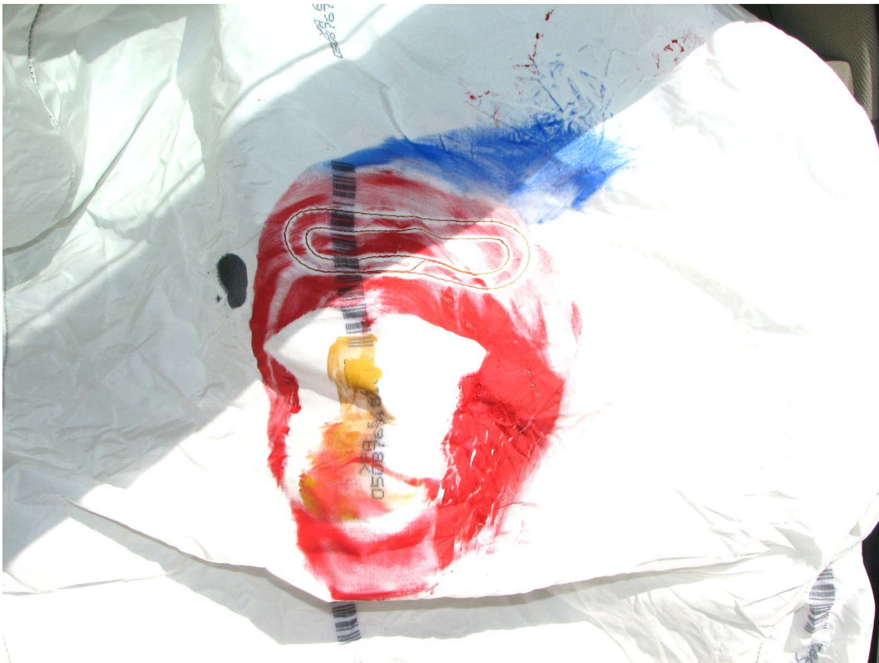
Figure A-57: Post-Test Passenger Dummy Airbag Contact
