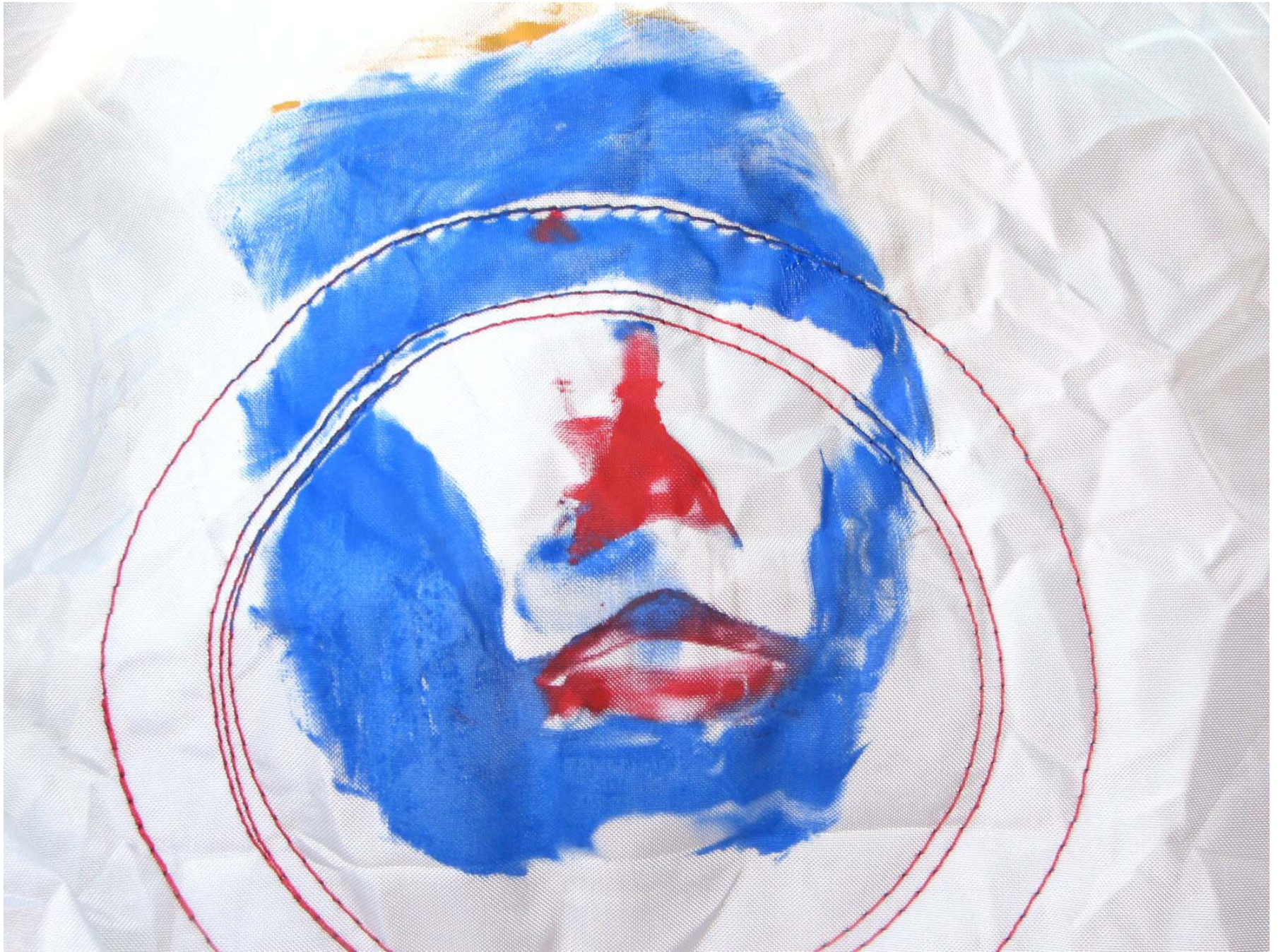
Figure A-43: Post-Test Driver Dummy Airbag Contact
