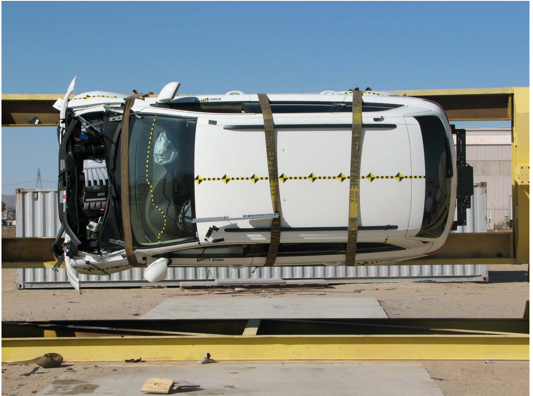
Figure A-59: Vehicle on Rollover Device (90°)
