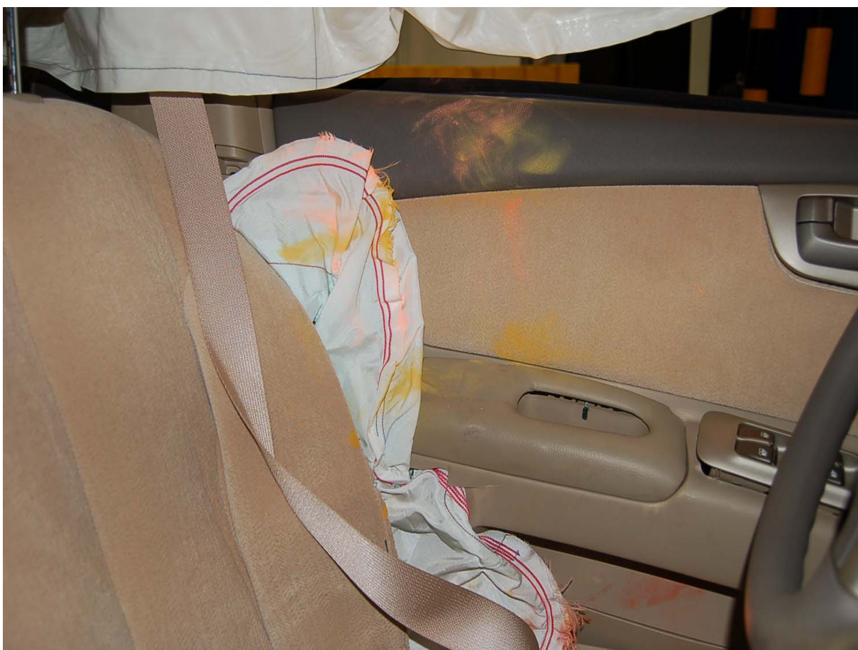
Post-Test Driver Dummy Torso Contact
