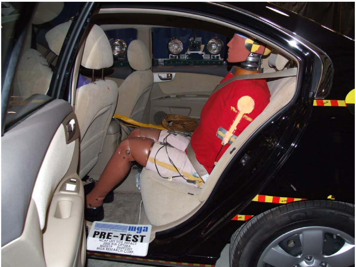
Pre-Test Passenger Dummy (Door Open)
