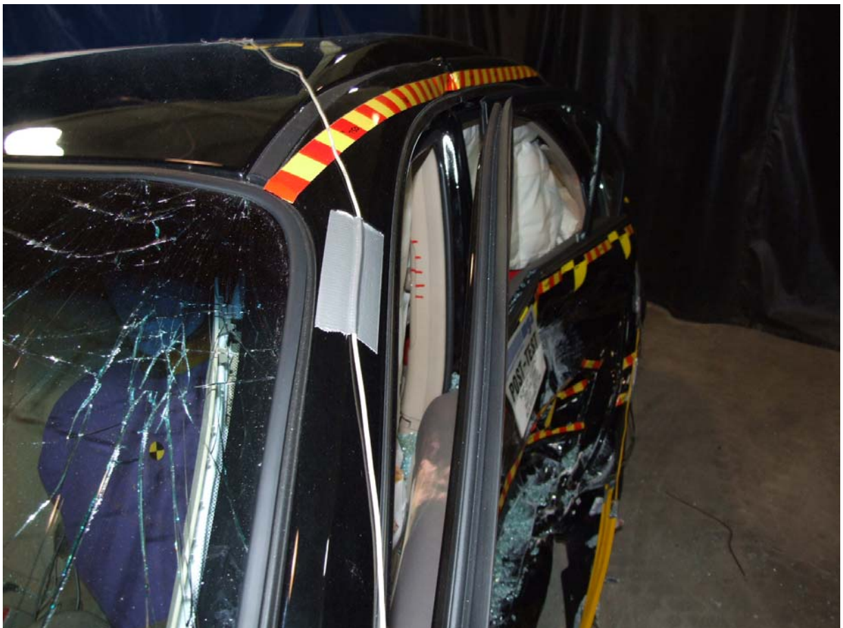
Post-Test Driver Dummy Clearance From Door
