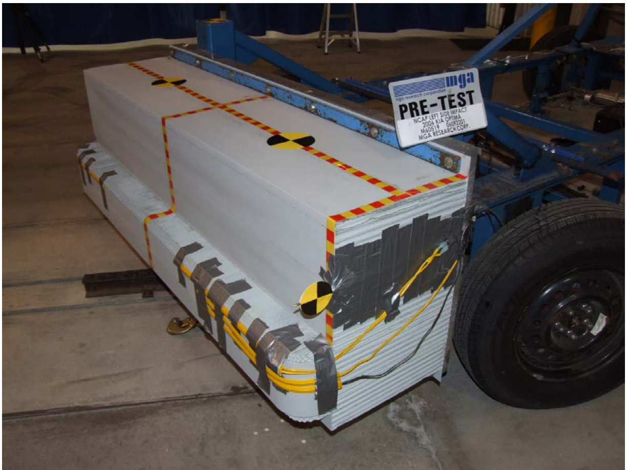
Pre-Test Left Side View of Deformable Barrier
