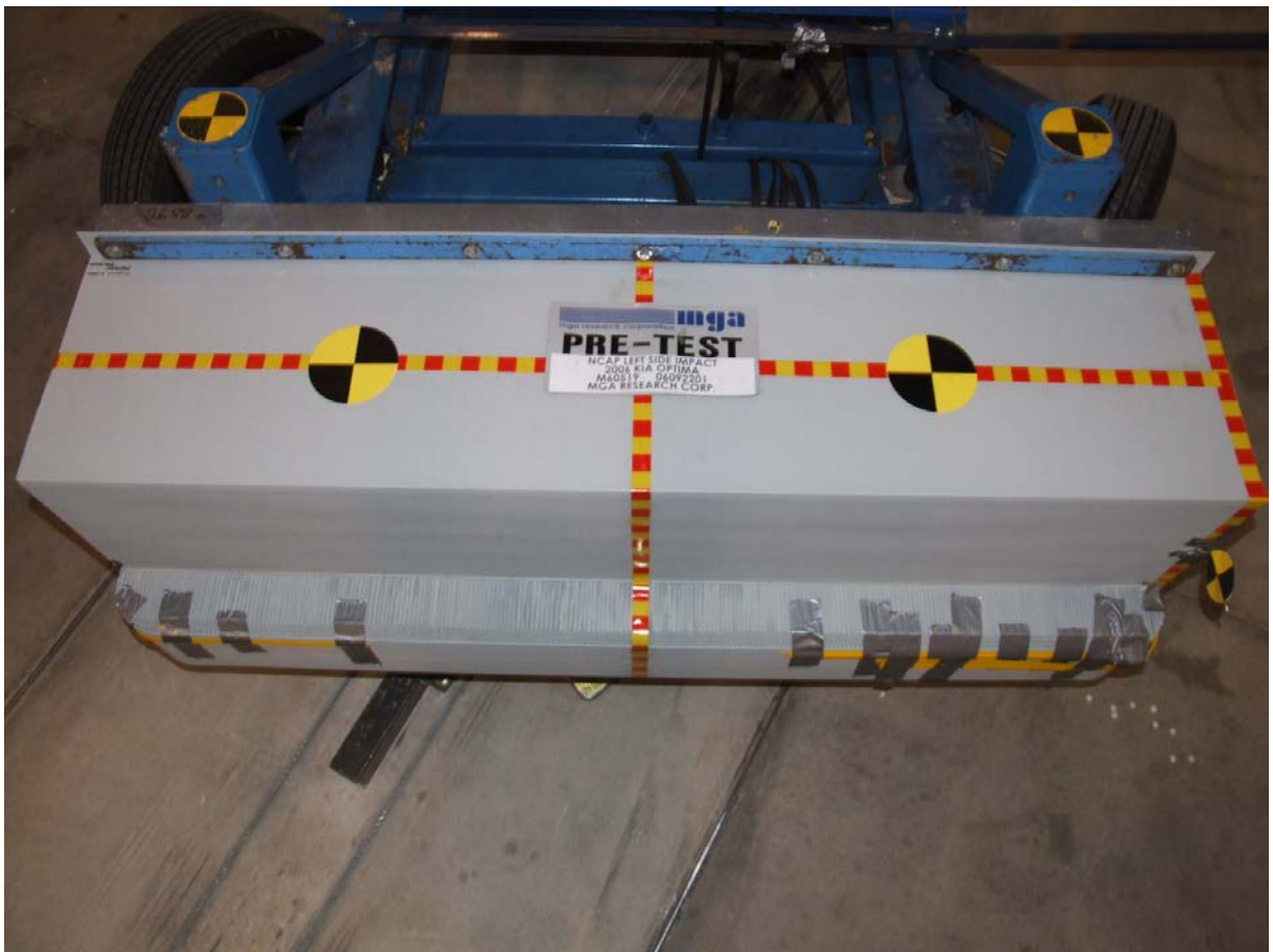
Pre-Test Top View of Deformable Barrier
