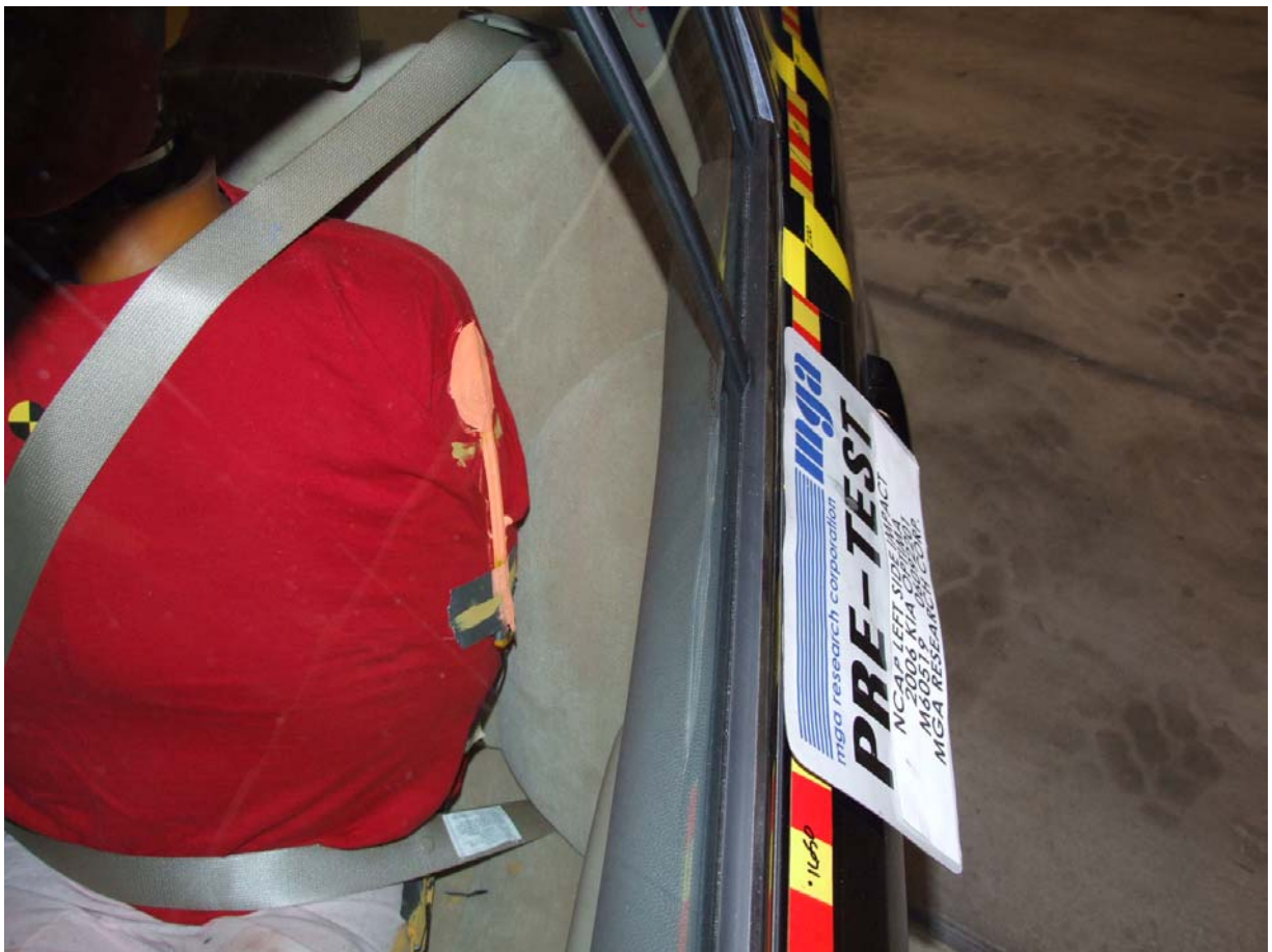
Pre-Test Passenger Dummy Clearance From Door
