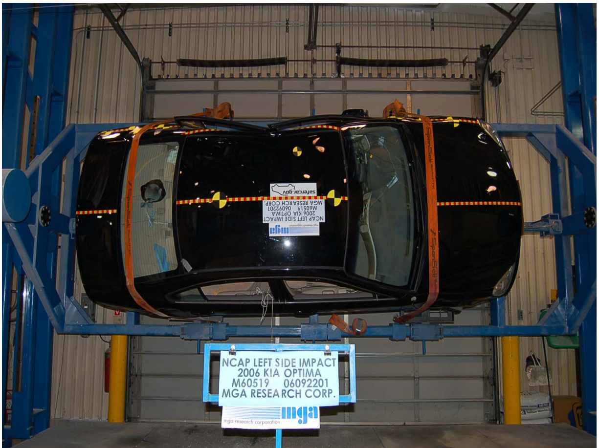
Vehicle on Rollover Device (270 Degrees)
