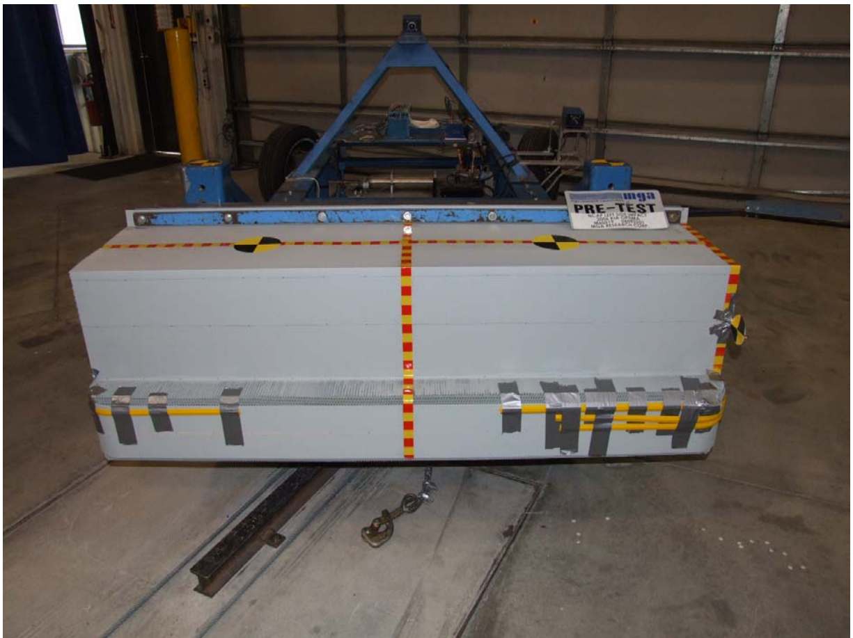
Pre-Test Front View of Deformable Barrier
