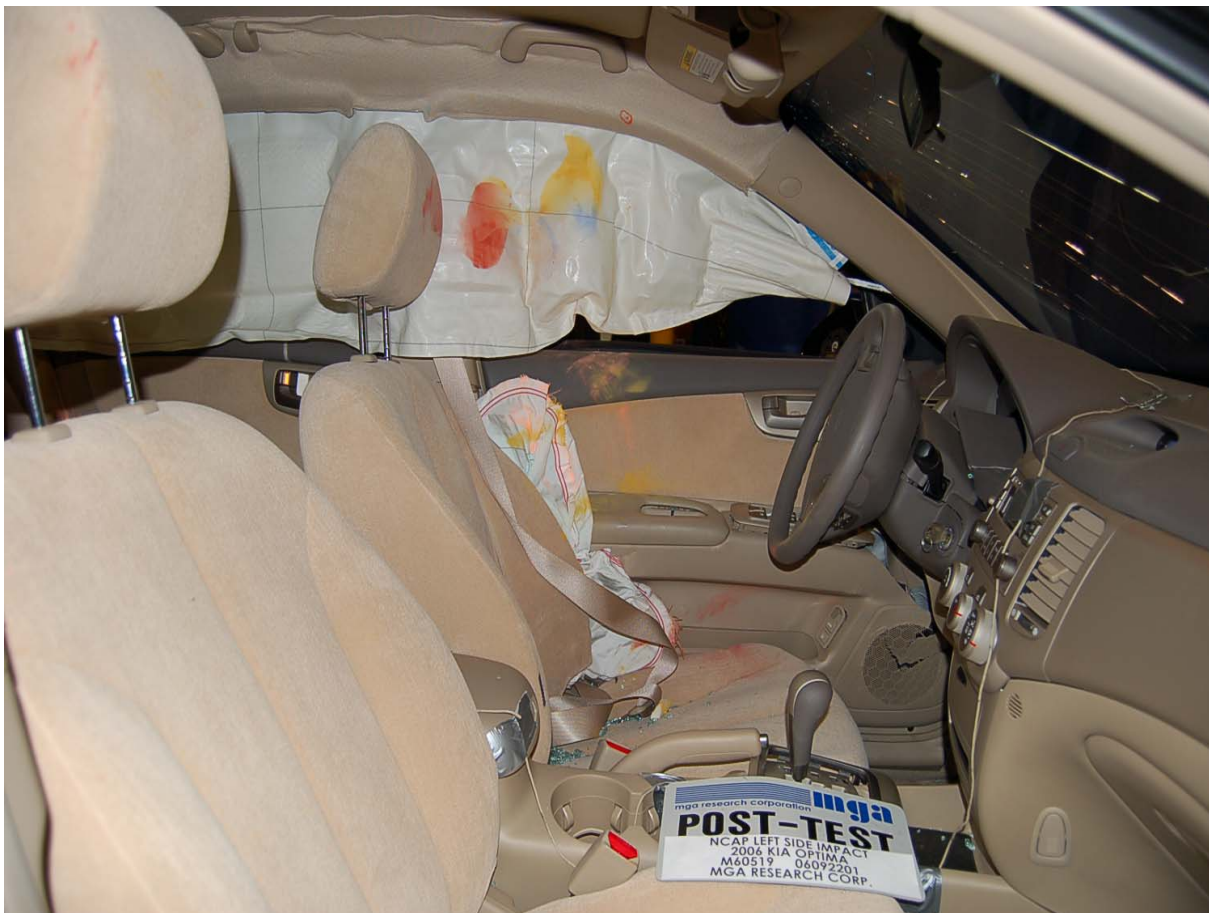
Post-Test Driver Dummy Contact
