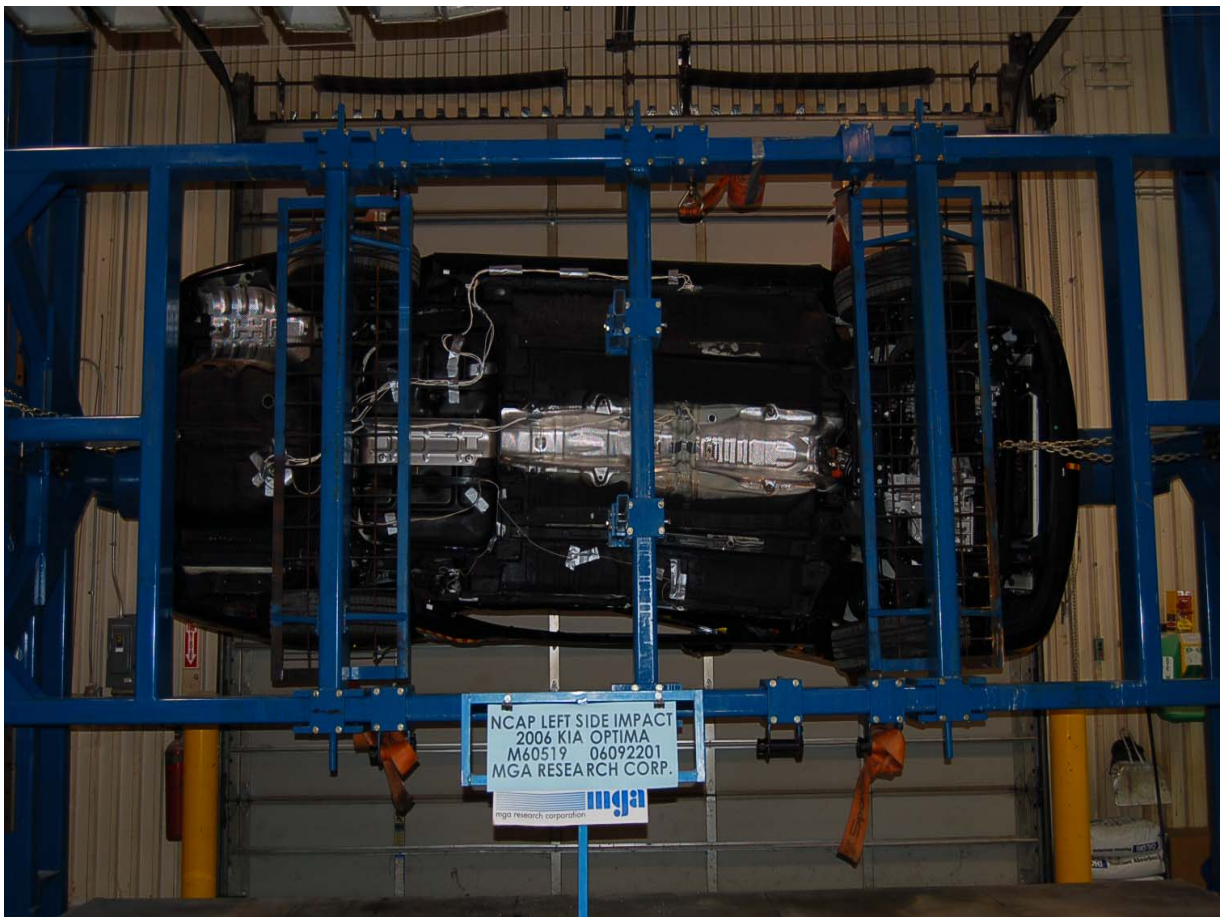
Vehicle on Rollover Device (90 Degrees)
