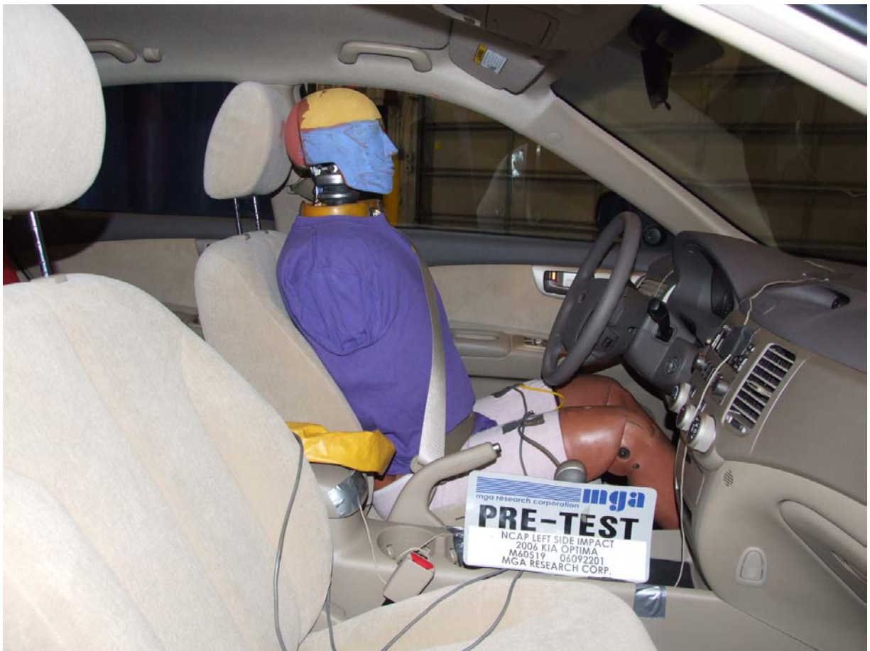
Pre-Test Driver Dummy Right Side View
