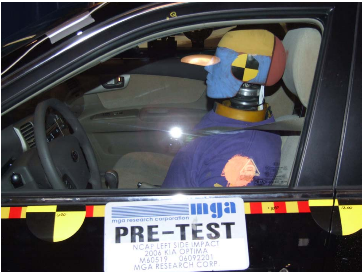
Pre-Test Driver Dummy (Through Window)
