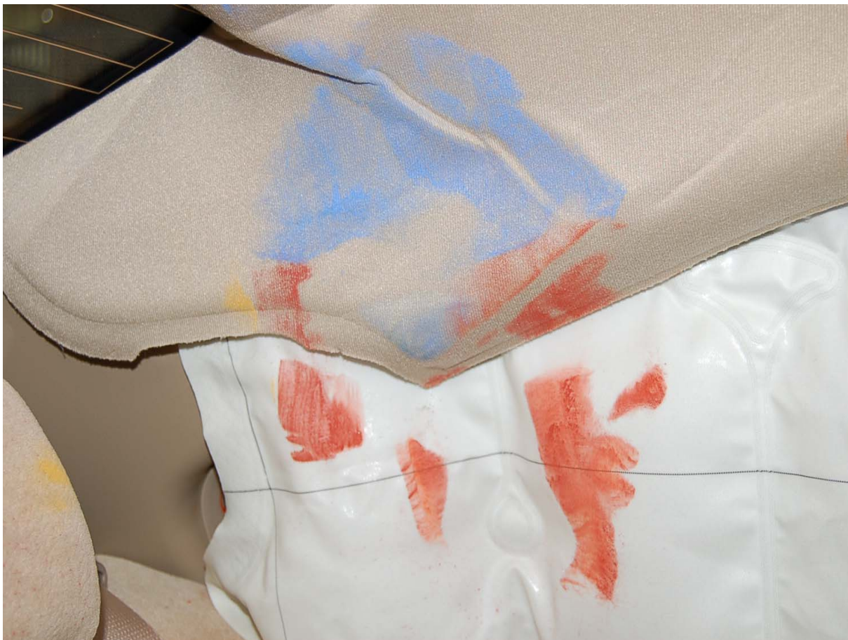
Post-Test Passenger Dummy Head Contact
