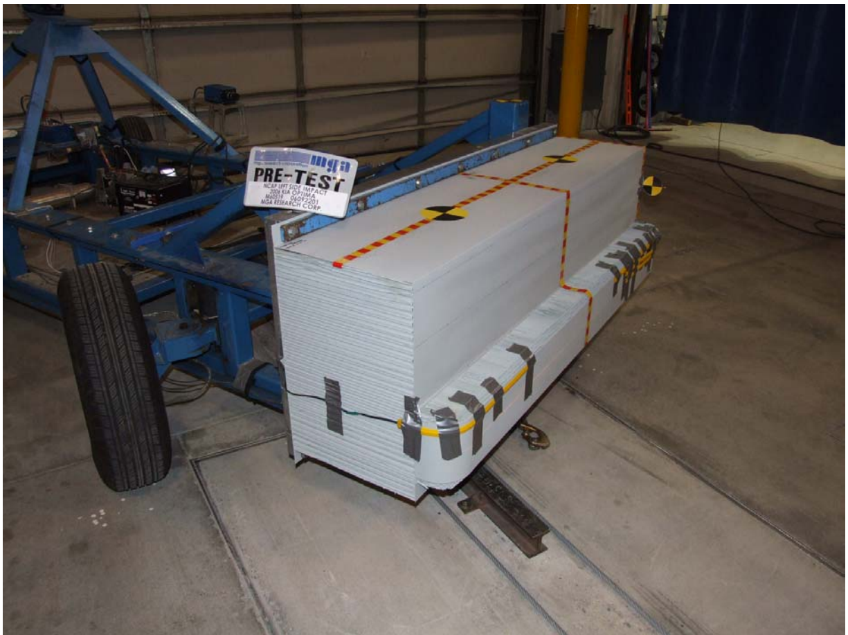
Pre-Test Right Side View of Deformable Barrier
