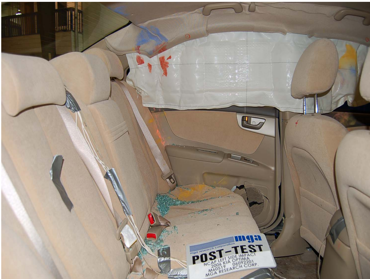
Post-Test Passenger Dummy Contact
