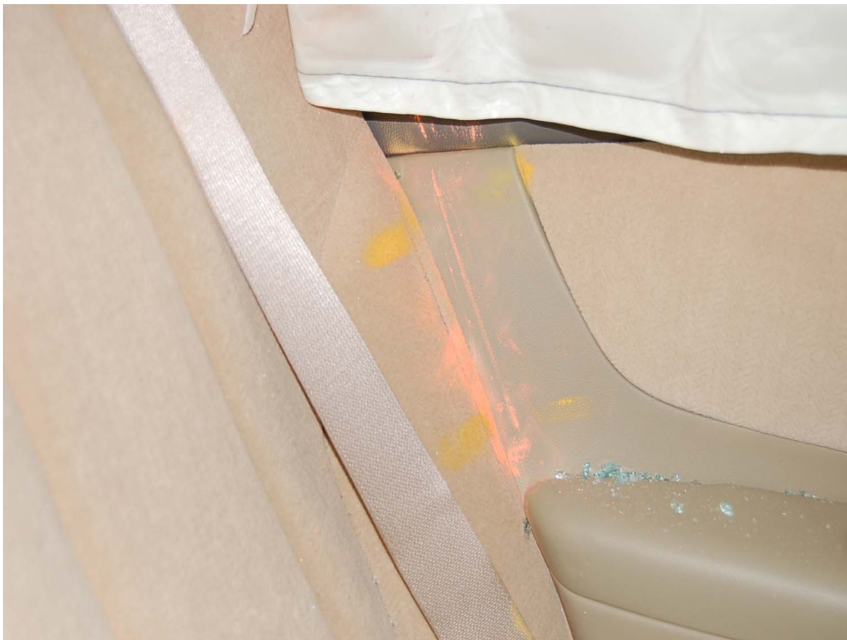
Post-Test Passenger Dummy Upper Torso Contact
