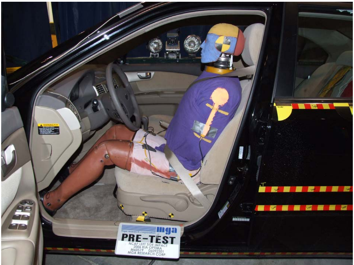
Pre-Test Driver Dummy (Door Open)
