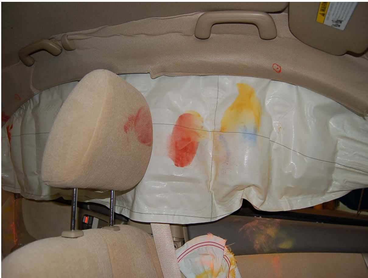
Post-Test Driver Dummy Head Contact
