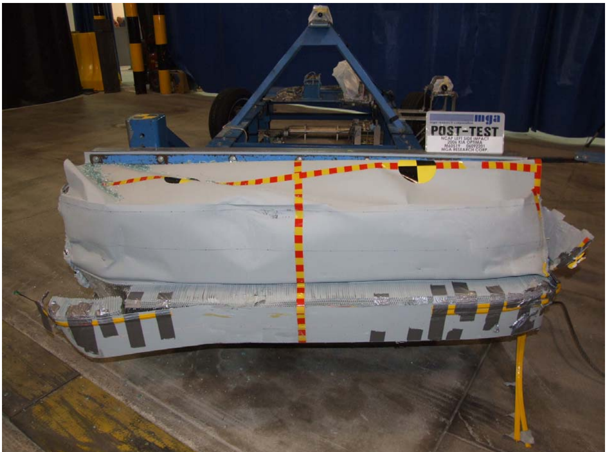
Post-Test Front View of Deformable Barrier
