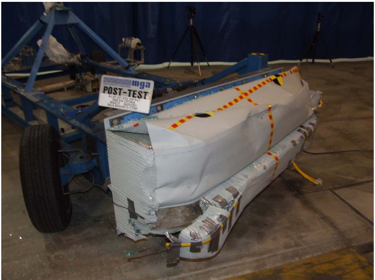
Post-Test Right Side View of Deformable Barrier
