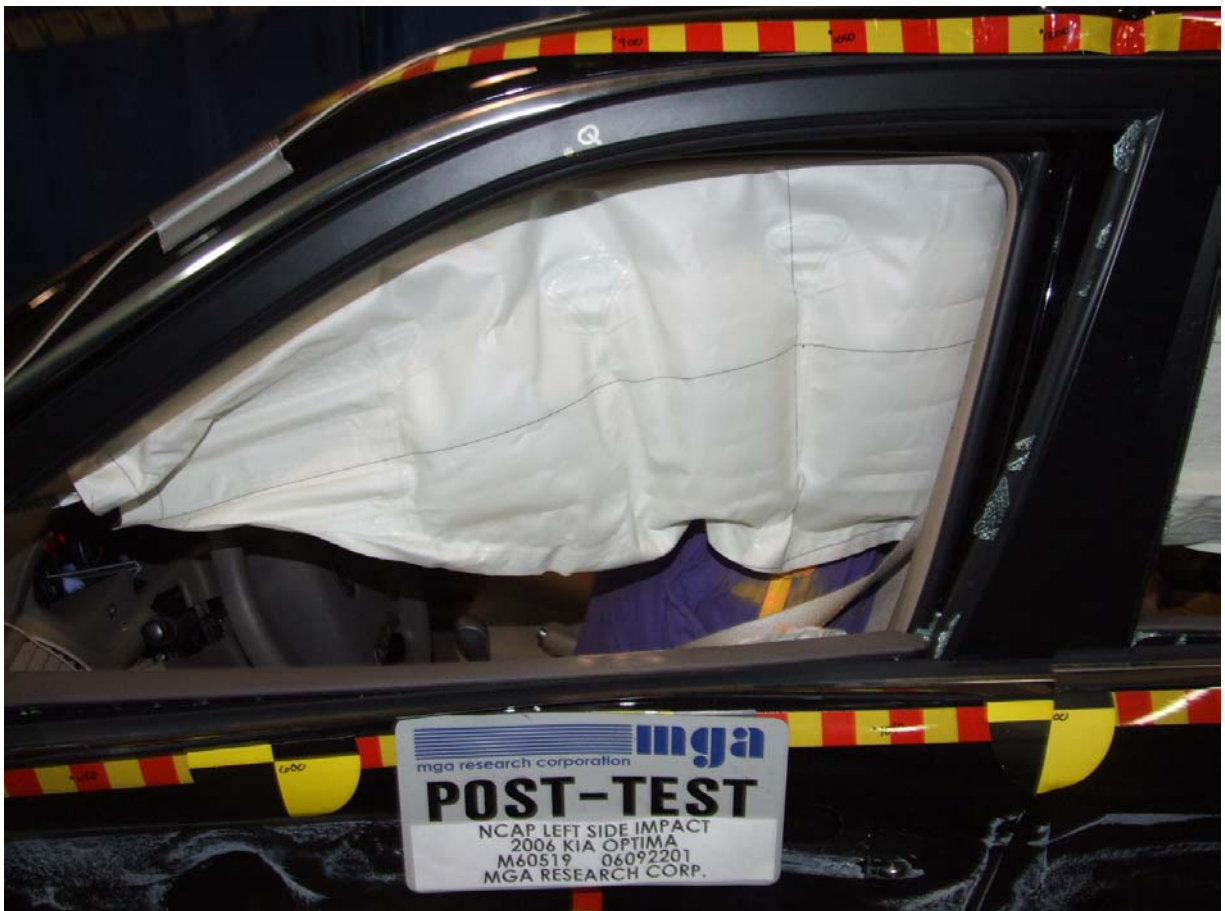
Post-Test Driver Dummy (Through Window)
