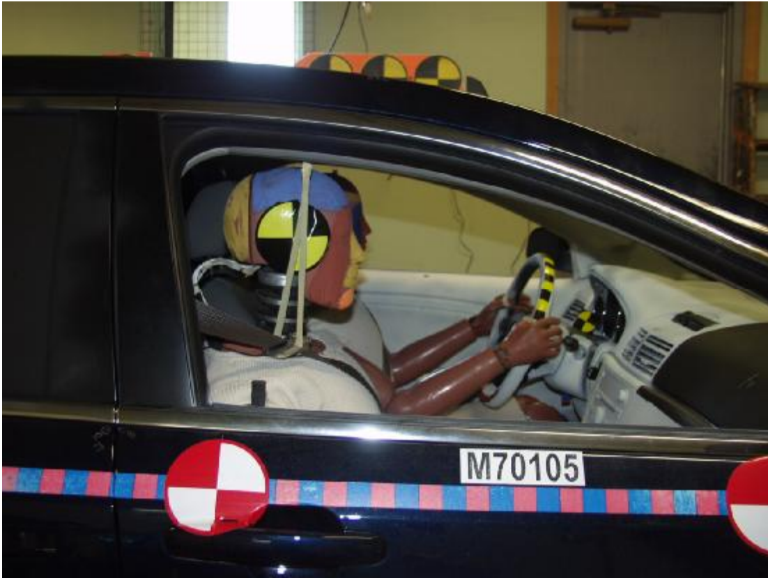
Figure A-46: Pre-Test Passenger Position View
