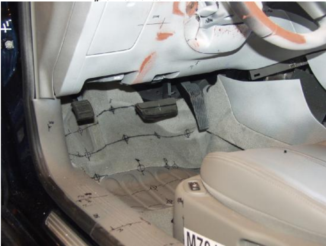
Figure A-41: Post-Test Driver Floor Pan View
