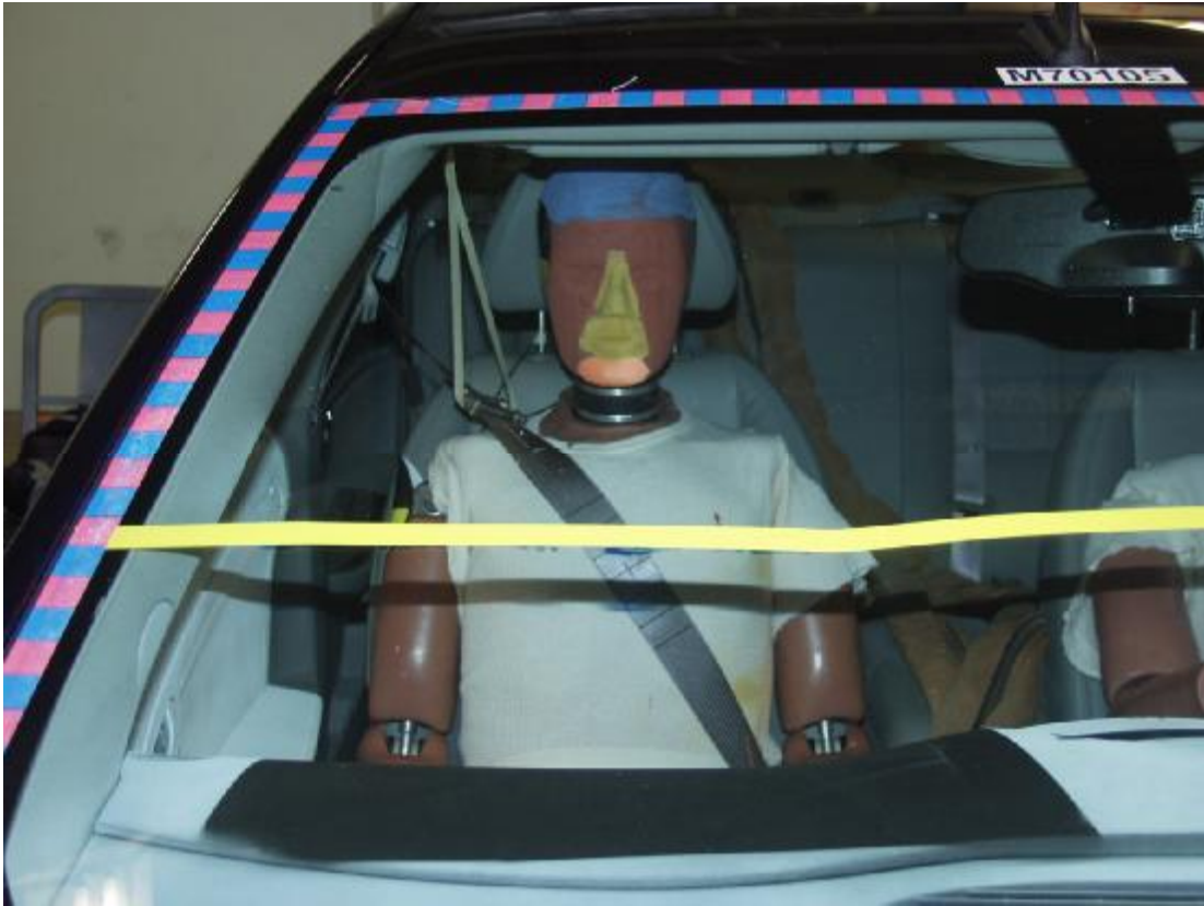
Figure A-44: Pre-Test Passenger Head Location
