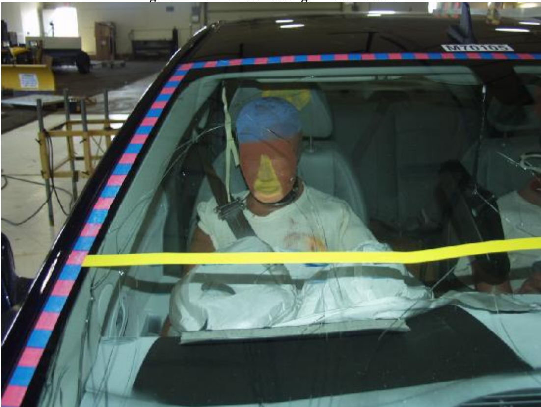
Figure A-45: Post-Test Passenger Head Location
