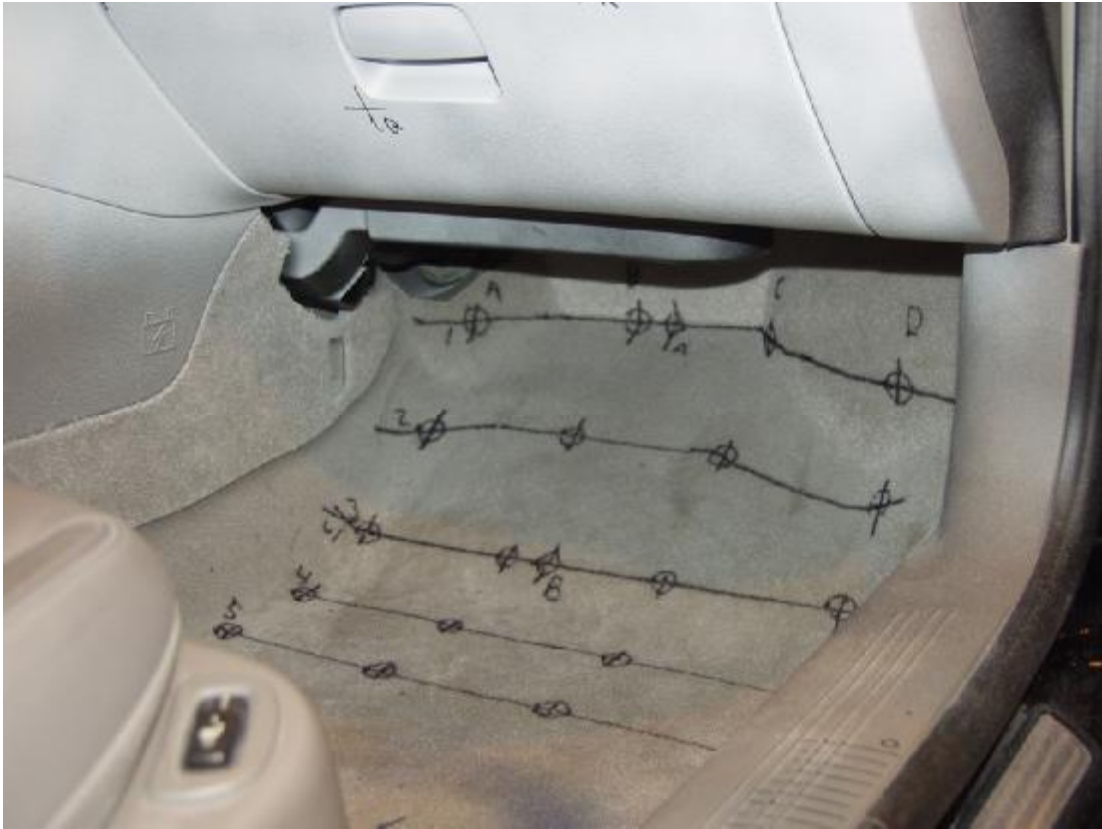
Figure A-54: Pre-Test Passenger Floor Pan View
