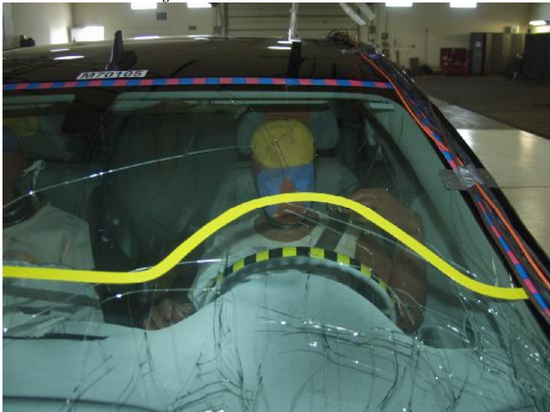
Figure A-31: Post-Test Driver Head Location
