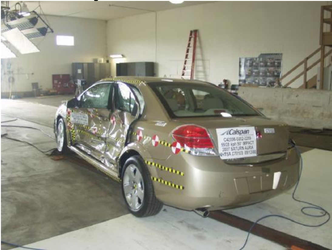
Figure A-12: Post-Test Left Rear \frac{3}{4} View
