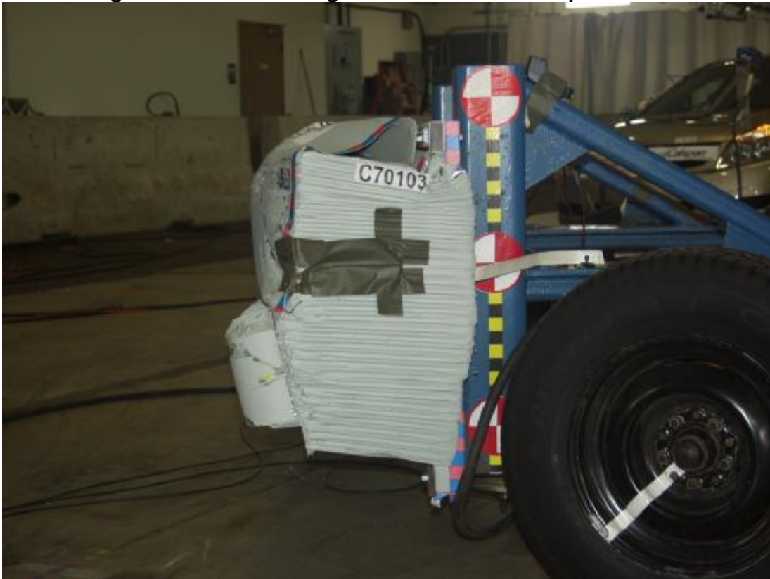
Figure A-26: Post-Test Right Side View of MDB Impactor Face
