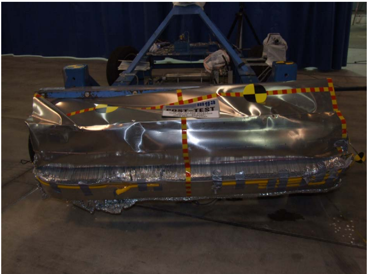
Post-Test Front View of Deformable Barrier
