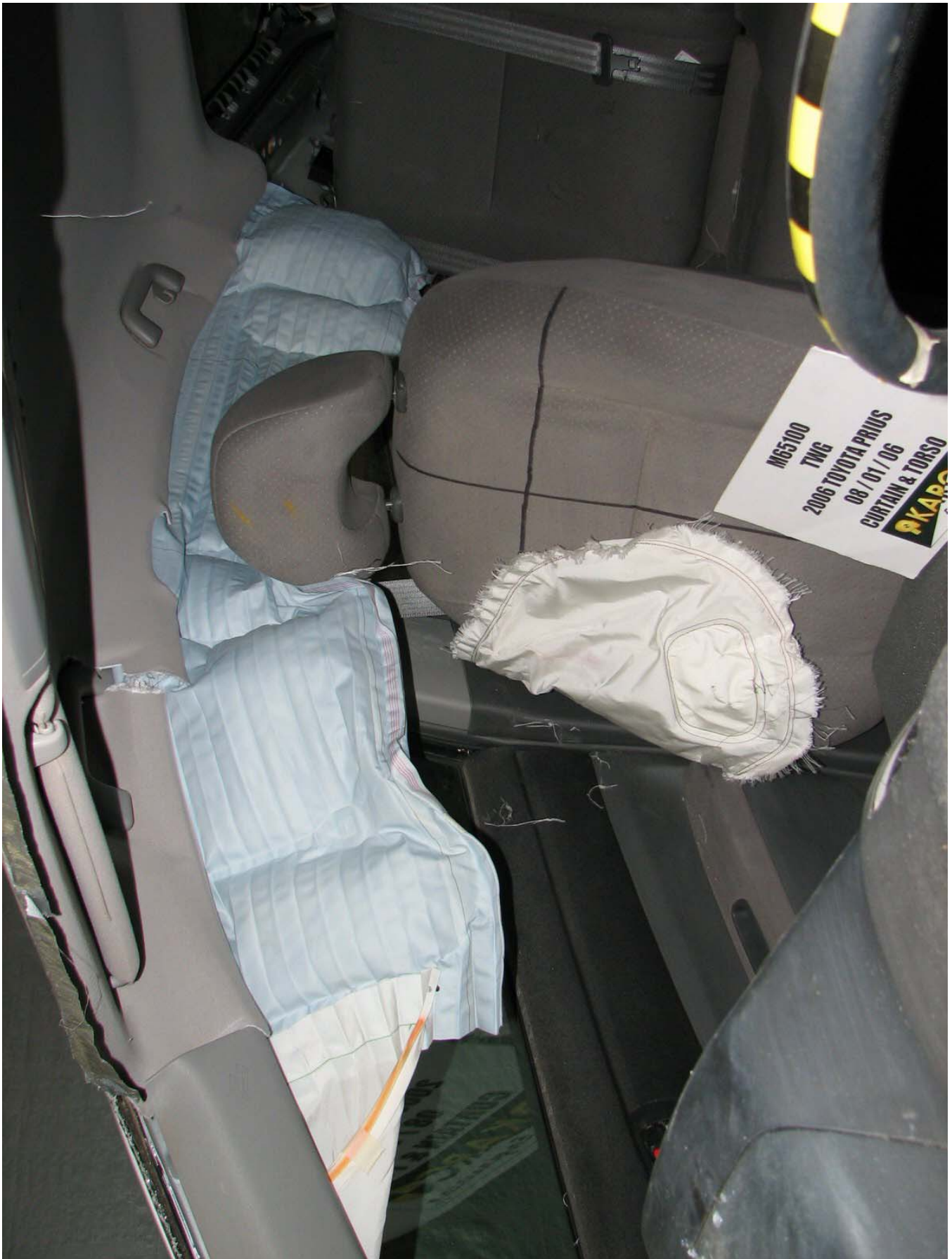
Figure A-10: Post-Test Airbags, Close-up View
