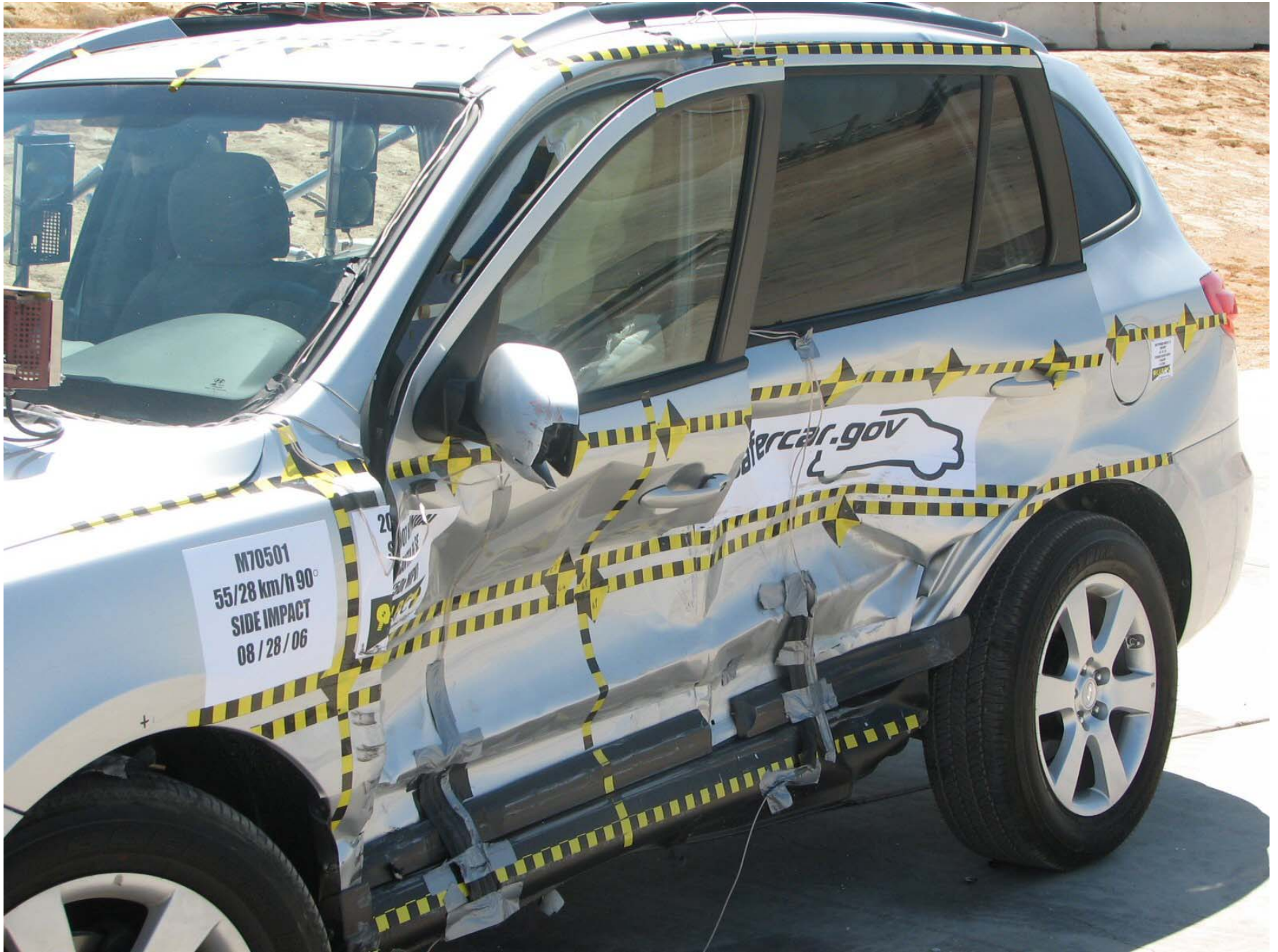
Figure A-28: Post-Test Front ¾ View of Left Side Door
