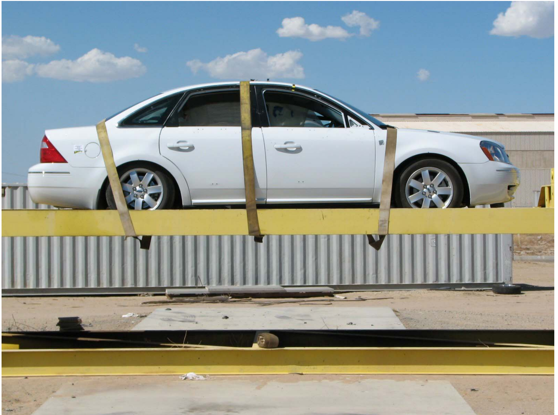
Figure A-61: Vehicle on Rollover Device (0°)
