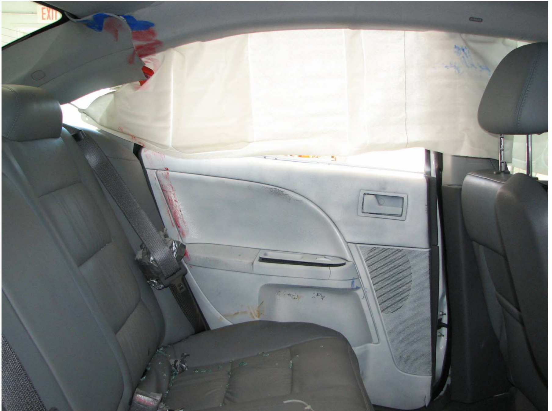
Figure A-52: Post-Test Rear Door Panel (Interior)
