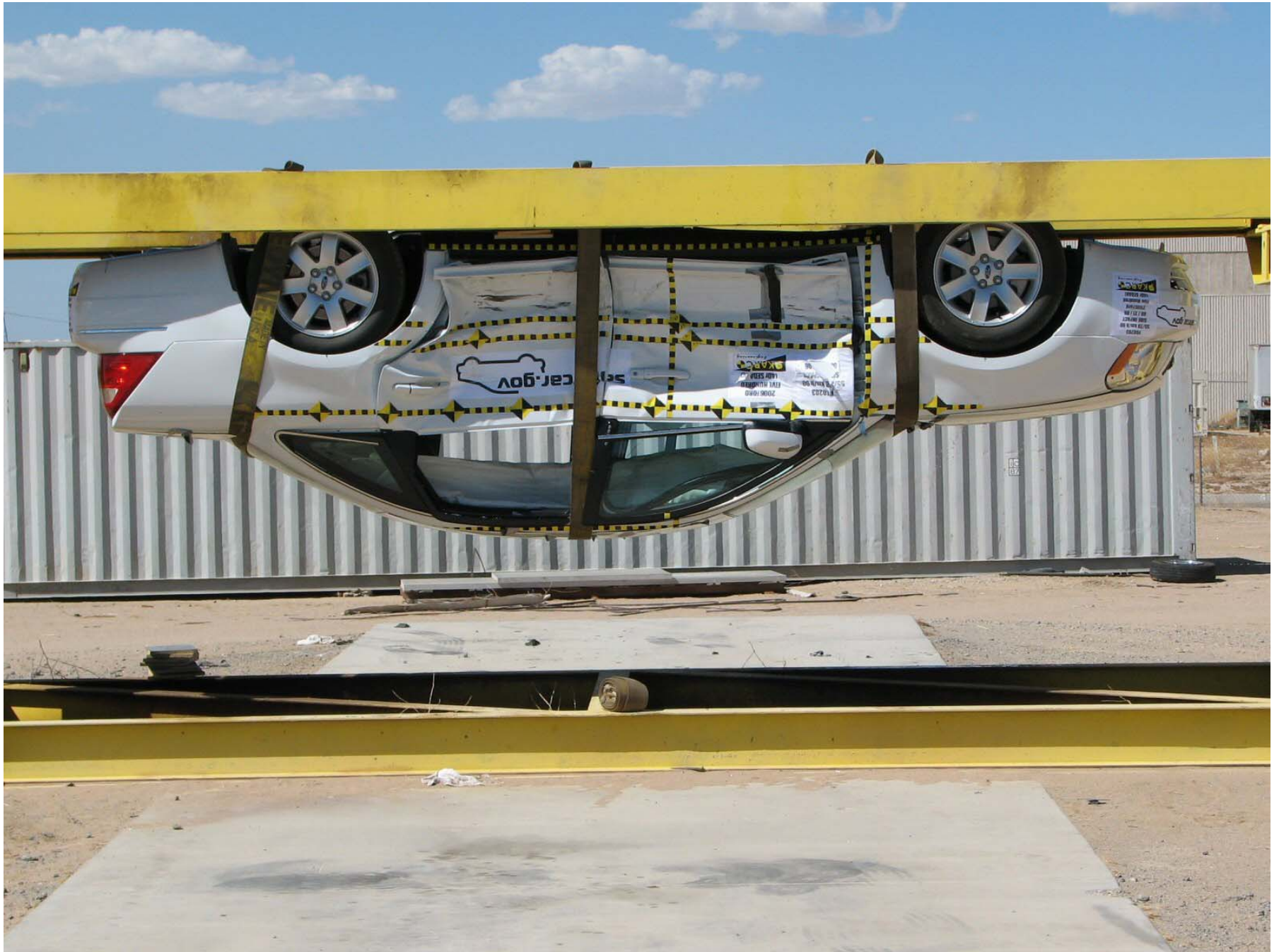
Figure A-63: Vehicle on Rollover Device (180°)
