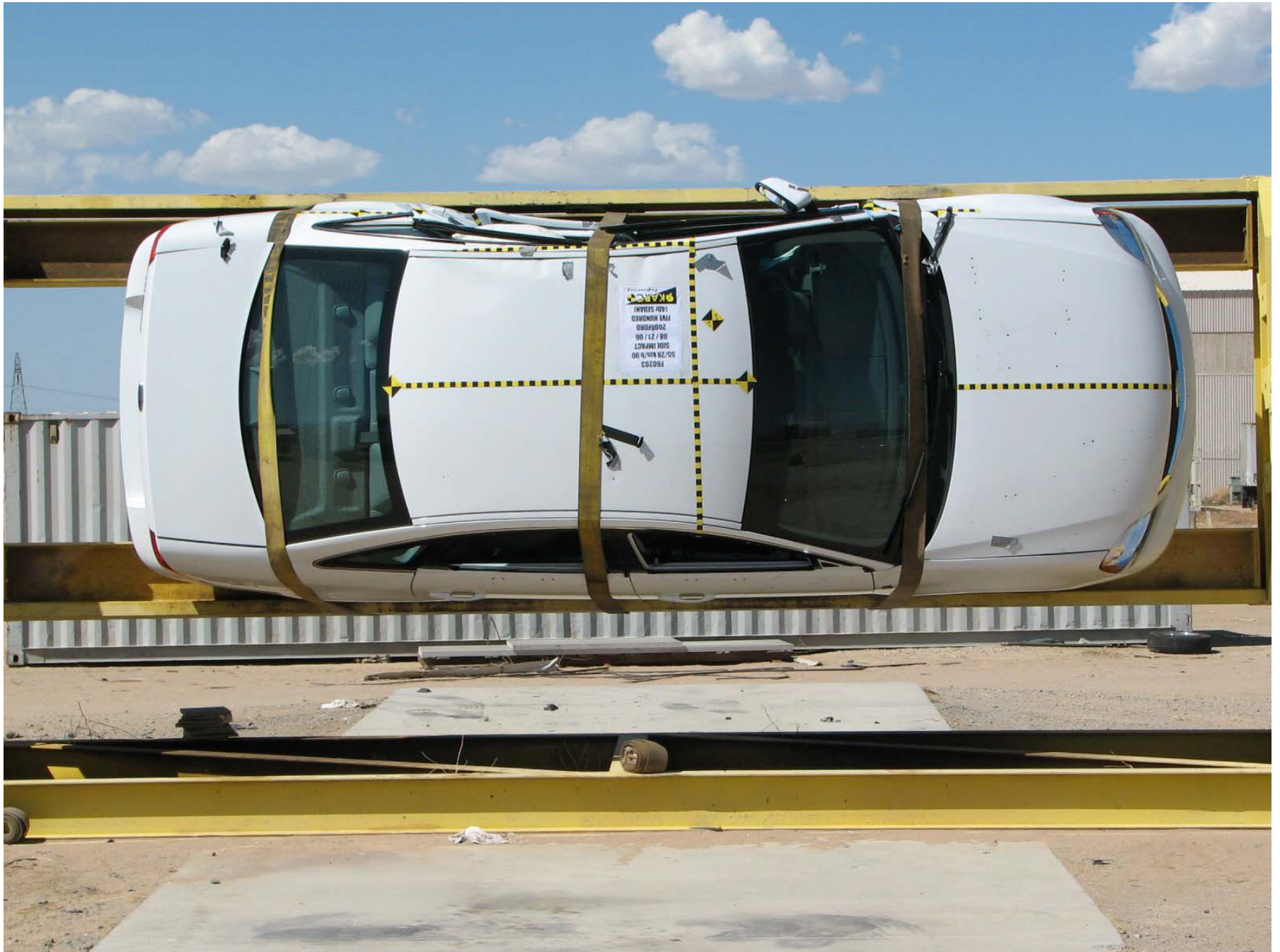
Figure A-62: Vehicle on Rollover Device (90°)
