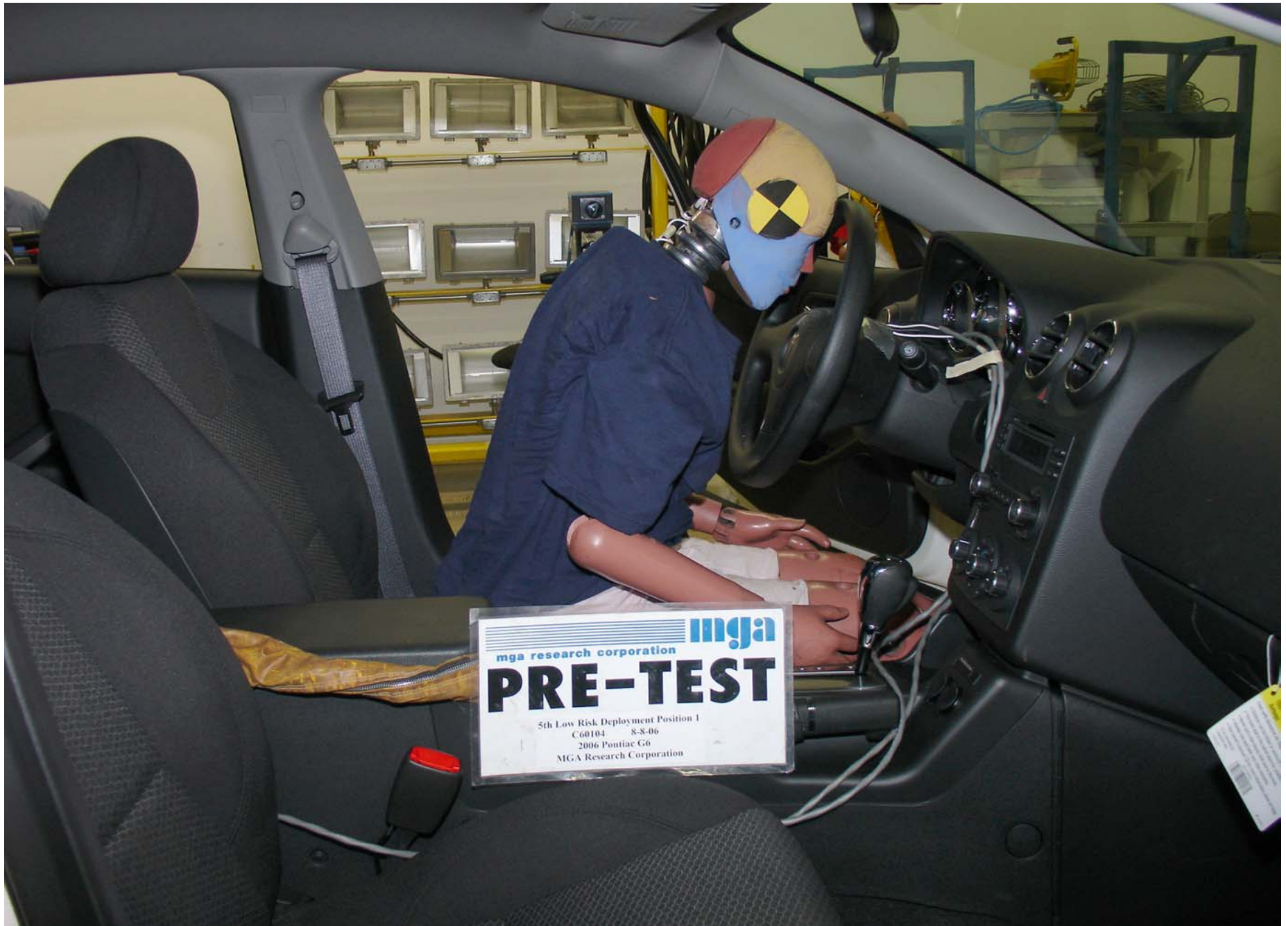
Pre-Test 5th Fem. P1 Driver Dummy Right Side View (Door Open)
