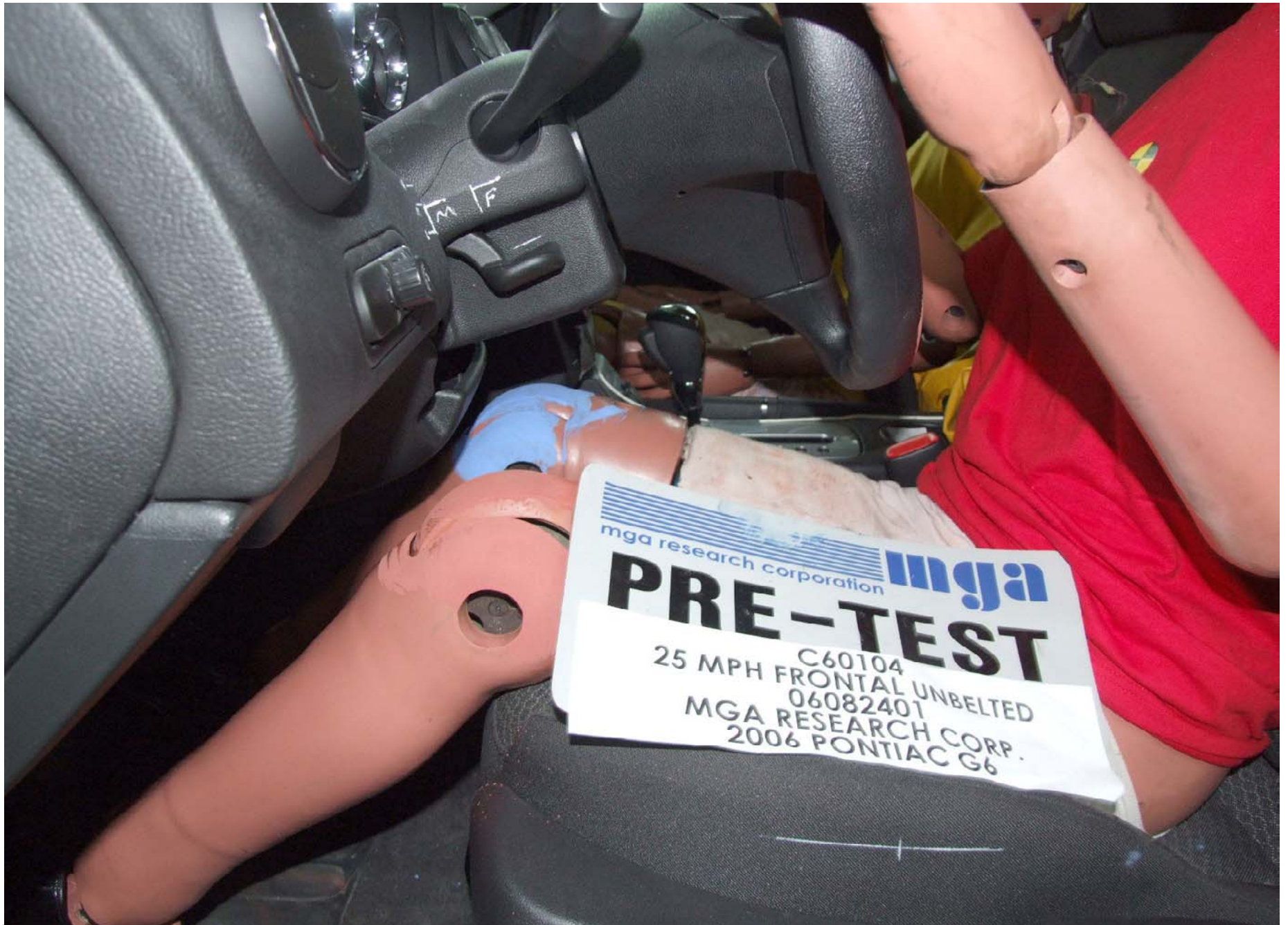
Pre-Test Driver Side Knee Bolster View
