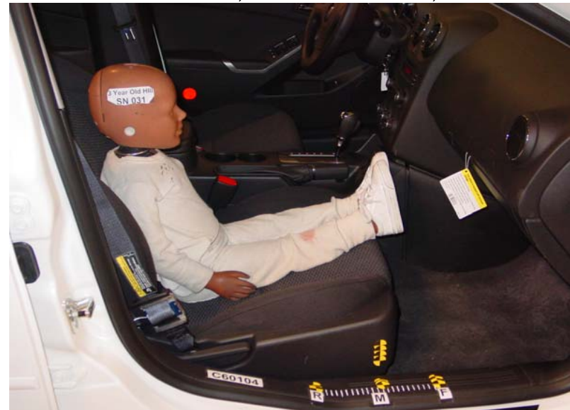
3-Year-Old Unbelted, Middle Seat Track, Position 1
