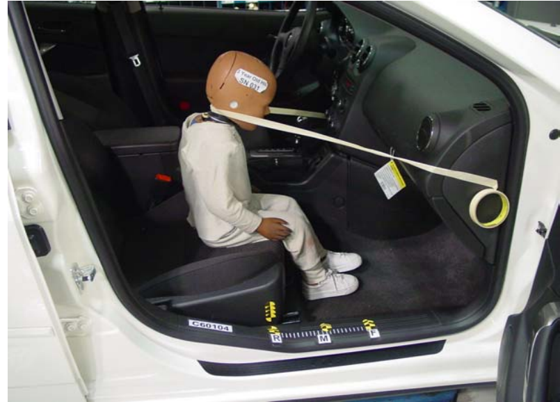
3-Year-Old Unbelted, Rearward Seat Track, Position 4
