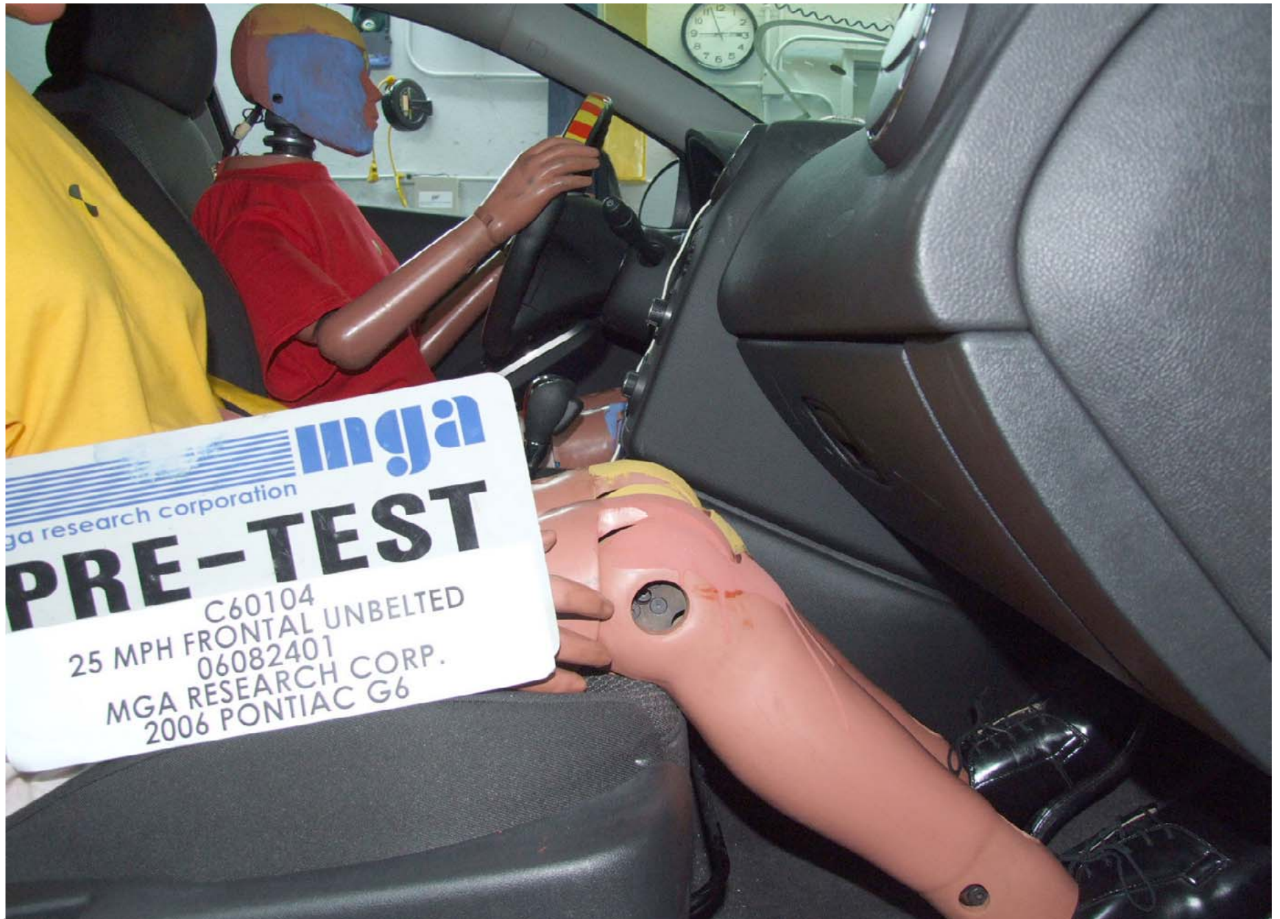
Pre-Test Passenger Side Knee Bolster View
