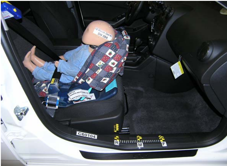
Britax Handle With Care 191 With Belt, Rearward Seat Track, Handle Down
