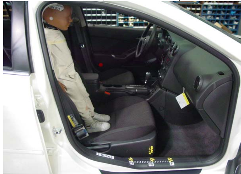
3-Year-Old Unbelted, Middle Seat Track, Position 5
