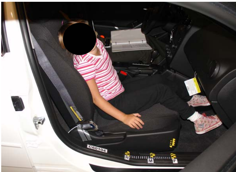
6-Year-Old Unbelted, Forward Seat Track, Position 1
