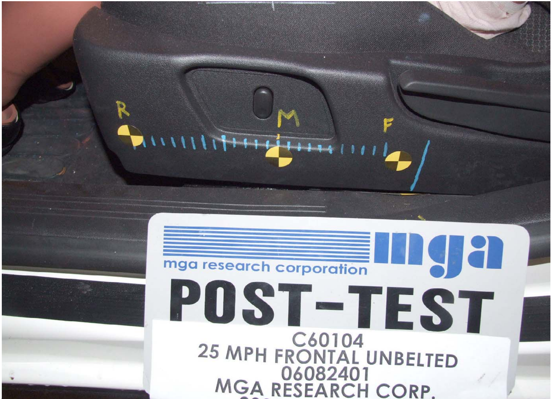
Post-Test Driver Dummy Seat Position
