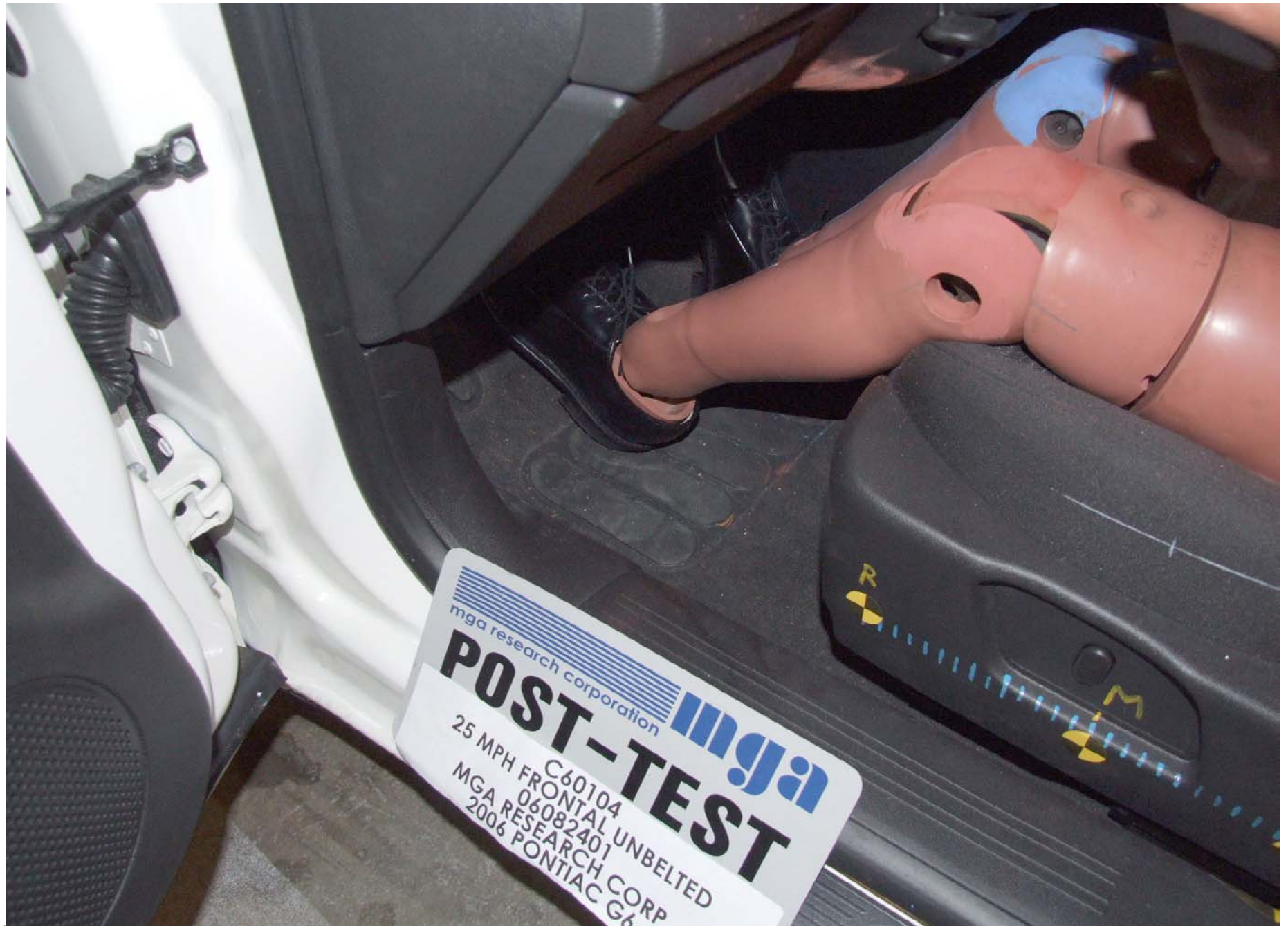
Post-Test Driver Dummy Feet Position
