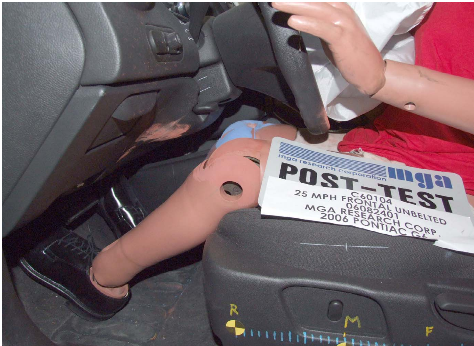
Post-Test Driver Side Knee Bolster View
