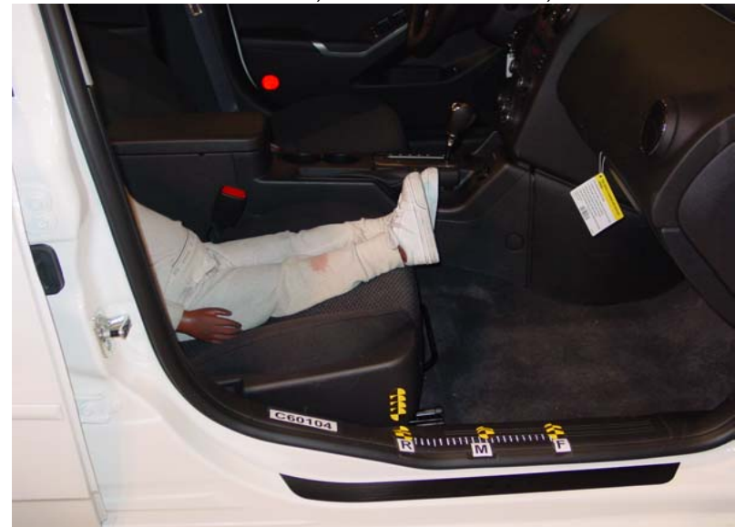
3-Year-Old Unbelted, Rearward Seat Track, Position 2
