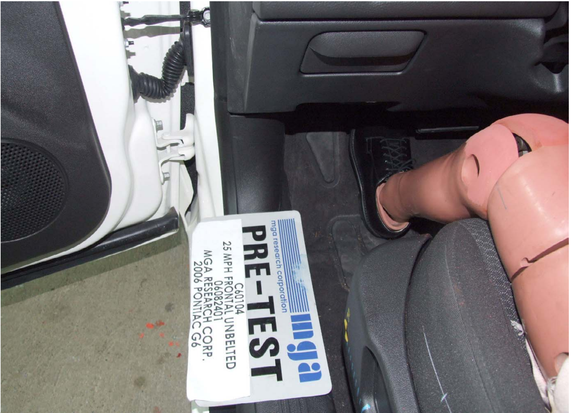
Pre-Test Driver Dummy Feet Position
