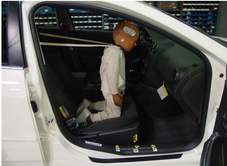
3-Year-Old Unbelted, Middle Seat Track, Position 6
