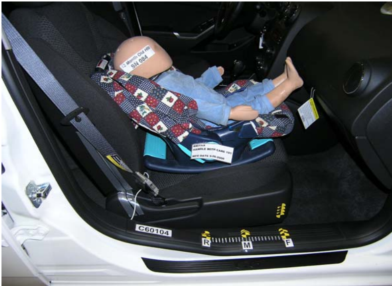
Britax Handle With Care 191 Fwd Facing Unbelted, Forward Seat Track, Handle Down
