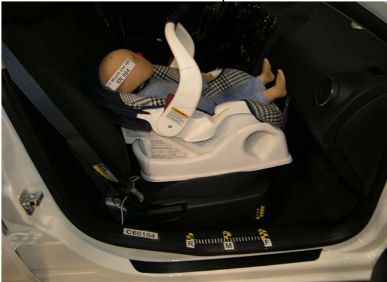
Graco Infant W/ Base Fwd Facing Unbelted, Forward Seat Track, Handle Up
