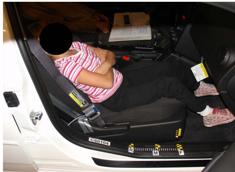
6-Year-Old Unbelted, Forward Seat Track, Position 2
