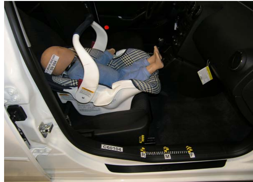
Graco Infant W/O Base Fwd Facing Unbelted, Rearward Seat Track, Handle Up
