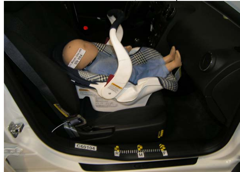
Graco Infant W/O Base Fwd Facing Unbelted, Forward Seat Track, Handle Up
