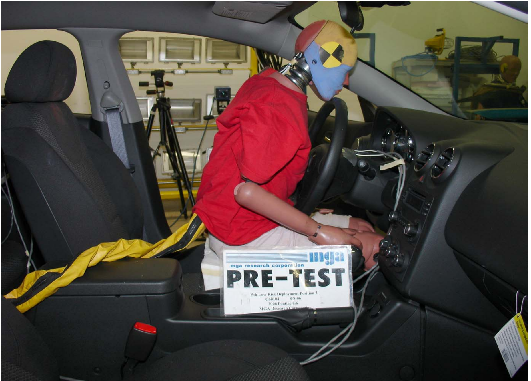
Pre-Test 5th Fem. P2 Driver Dummy Right Side View (Door Open)
