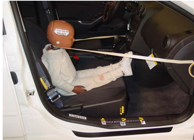
3-Year-Old Unbelted, Middle Seat Track, Position 3
