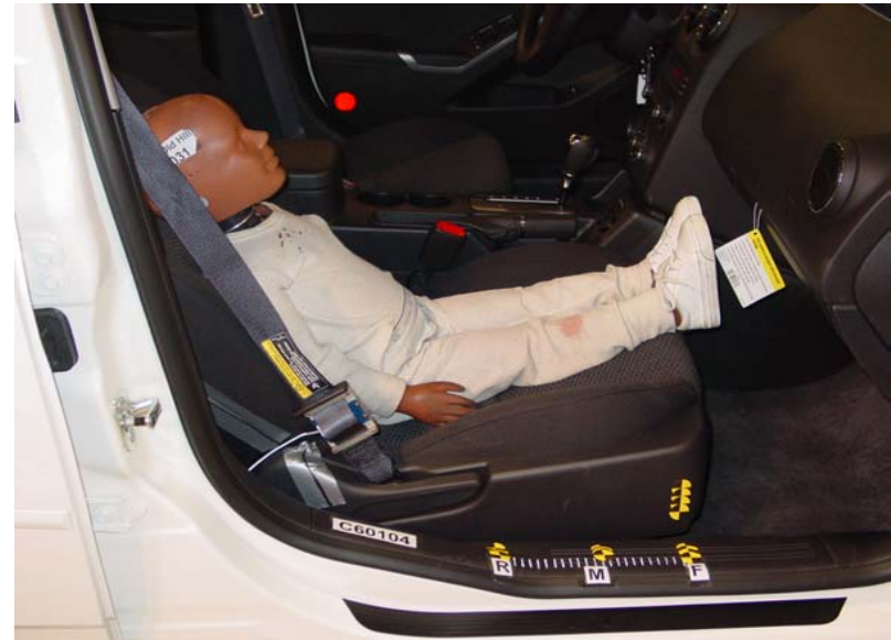
3-Year-Old Unbelted, Forward Seat Track, Position 2
