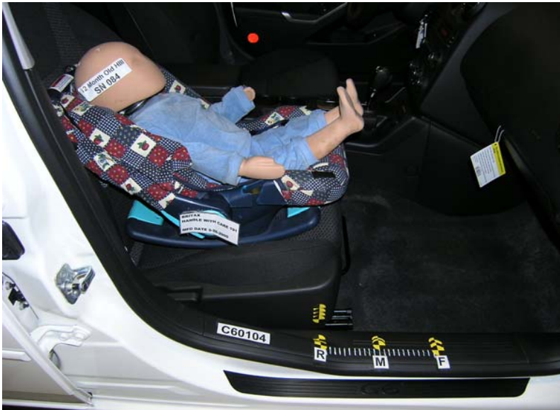
Britax Handle With Care 191 Fwd Facing Unbelted, Rearward Seat Track, Handle Down
