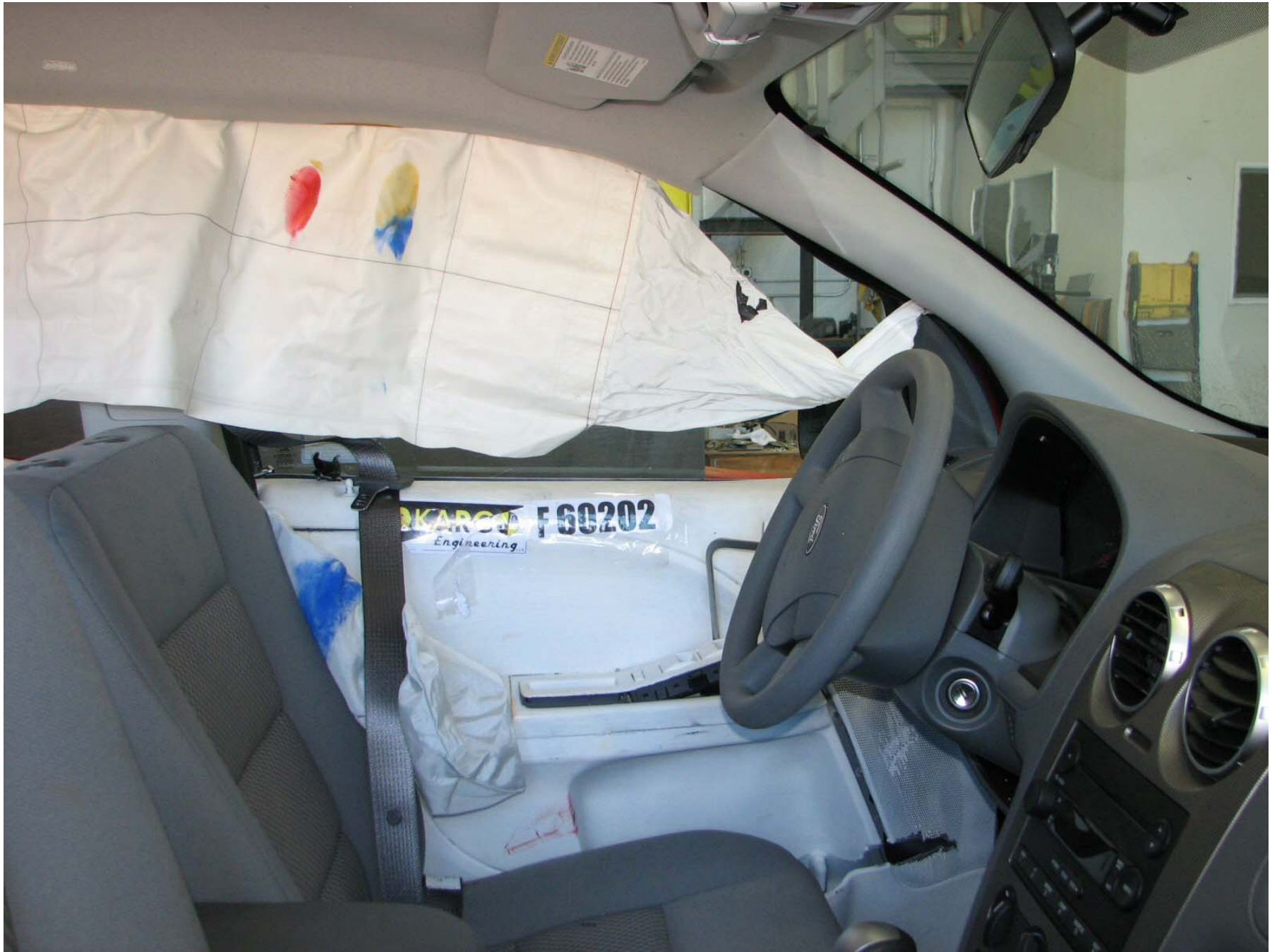
Figure A-43: Post-Test Front Door Panel (Interior)
