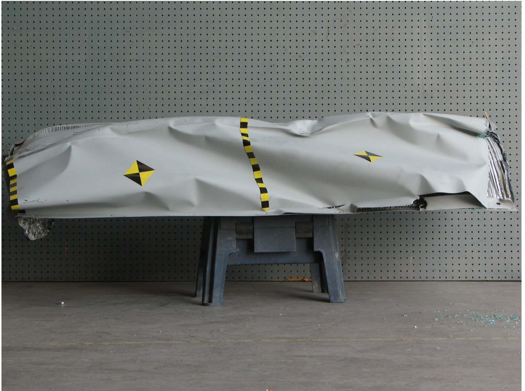
Figure A-56: Post-Test Top View of Deformable Barrier
