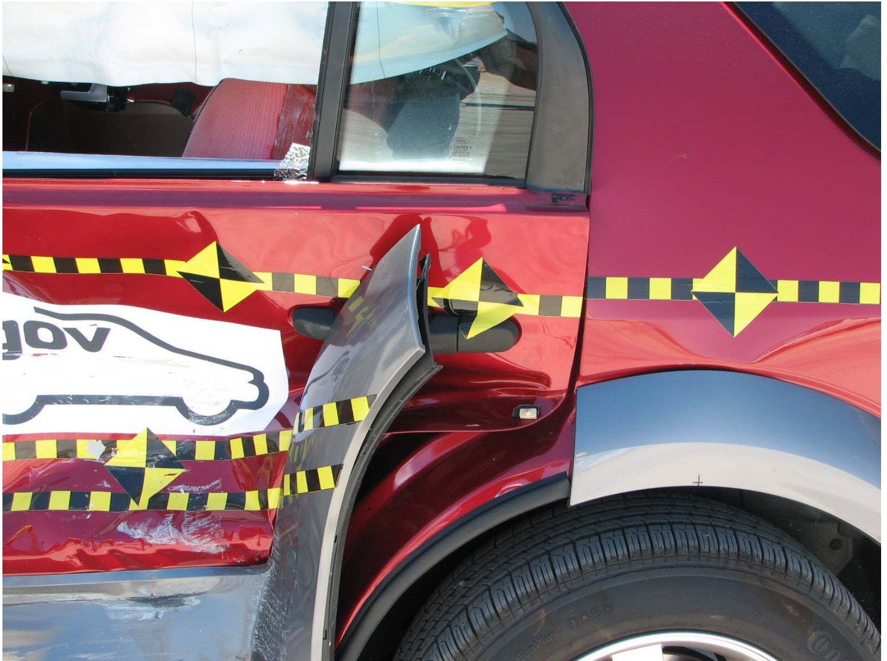
Figure A-34: Post-Test Left Rear Door
