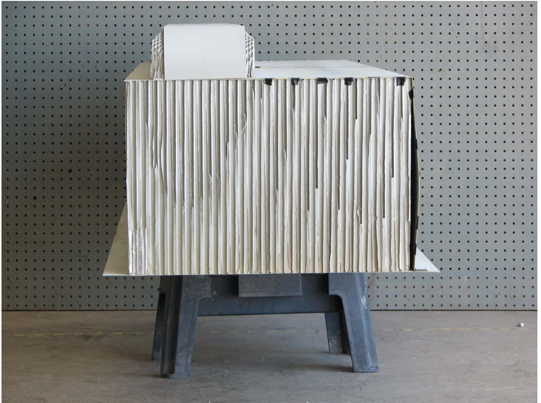
Figure A-59: Pre-Test Left Side View of Deformable Barrier
