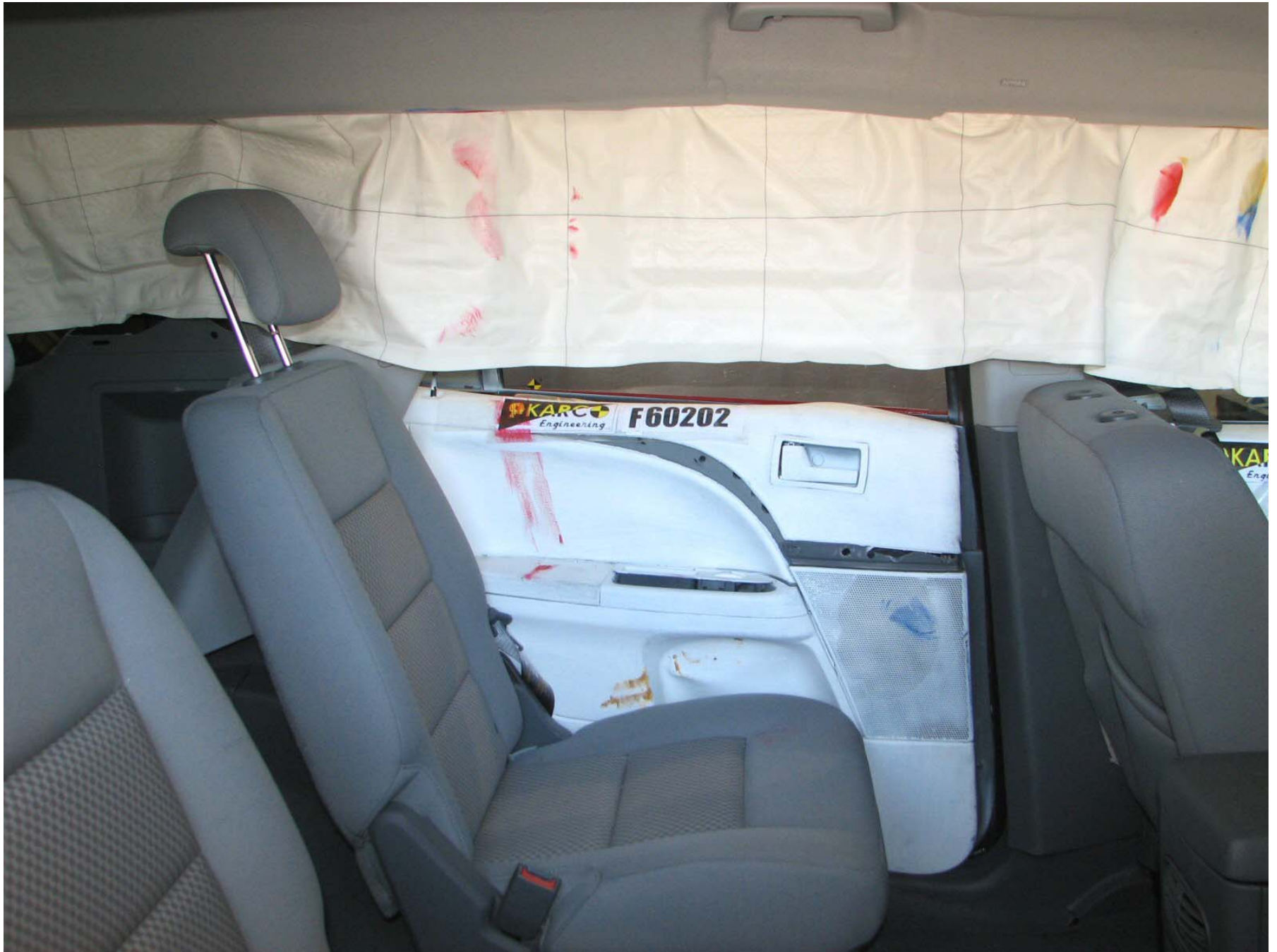
Figure A-52: Post-Test Rear Door Panel (Interior)
