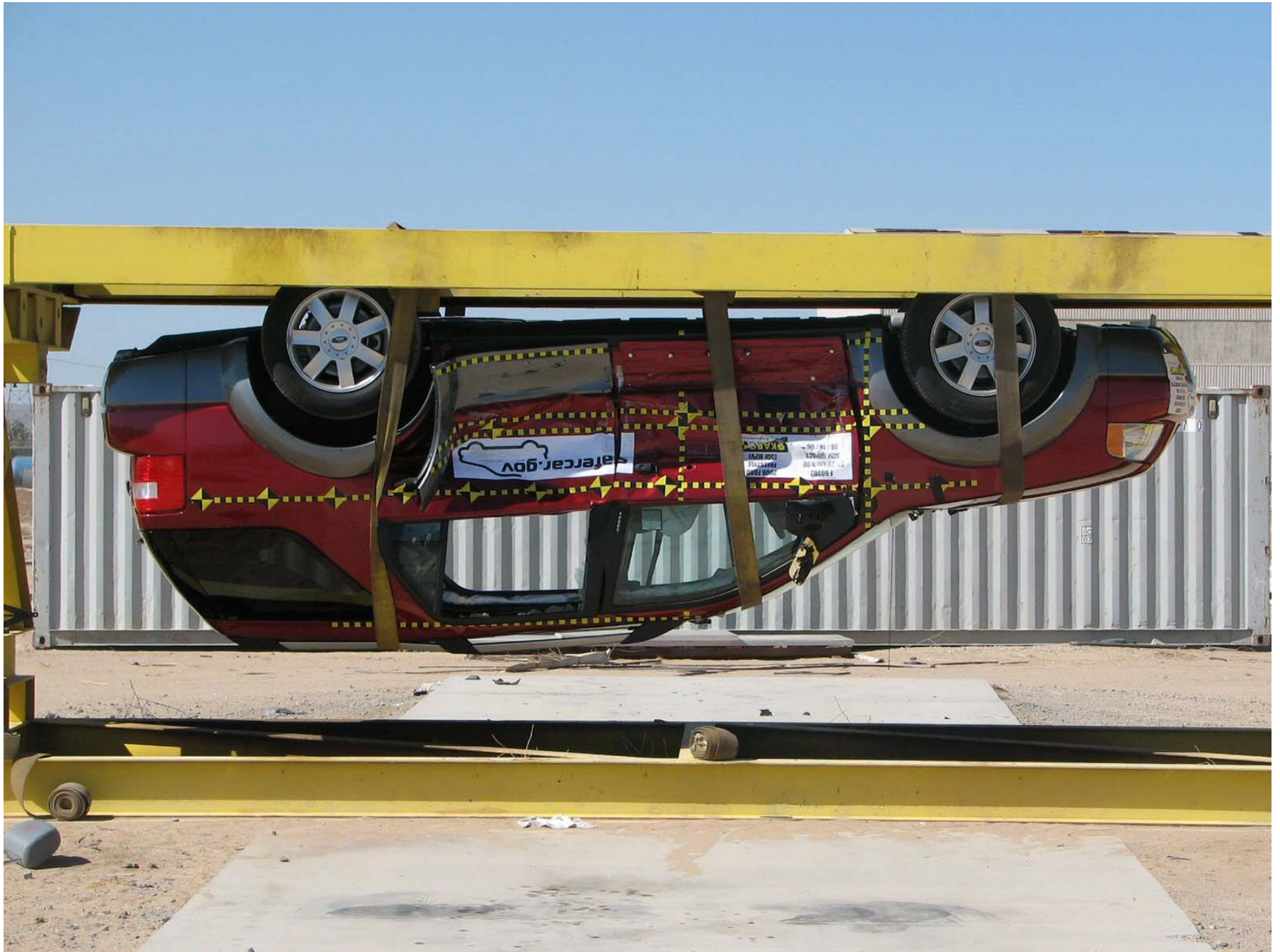
Figure A-63: Vehicle on Rollover Device (180°)
