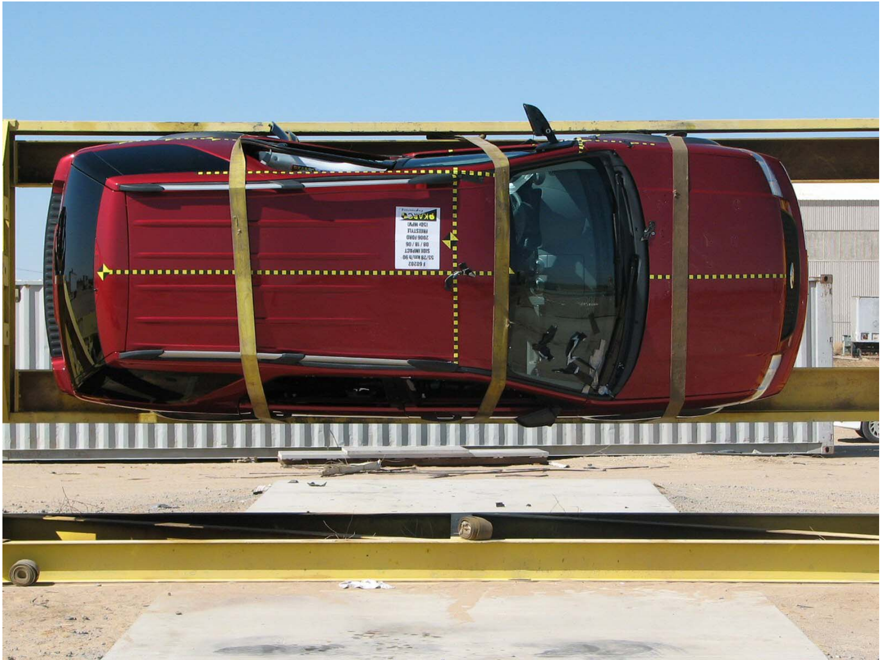
Figure A-62: Vehicle on Rollover Device (90°)
