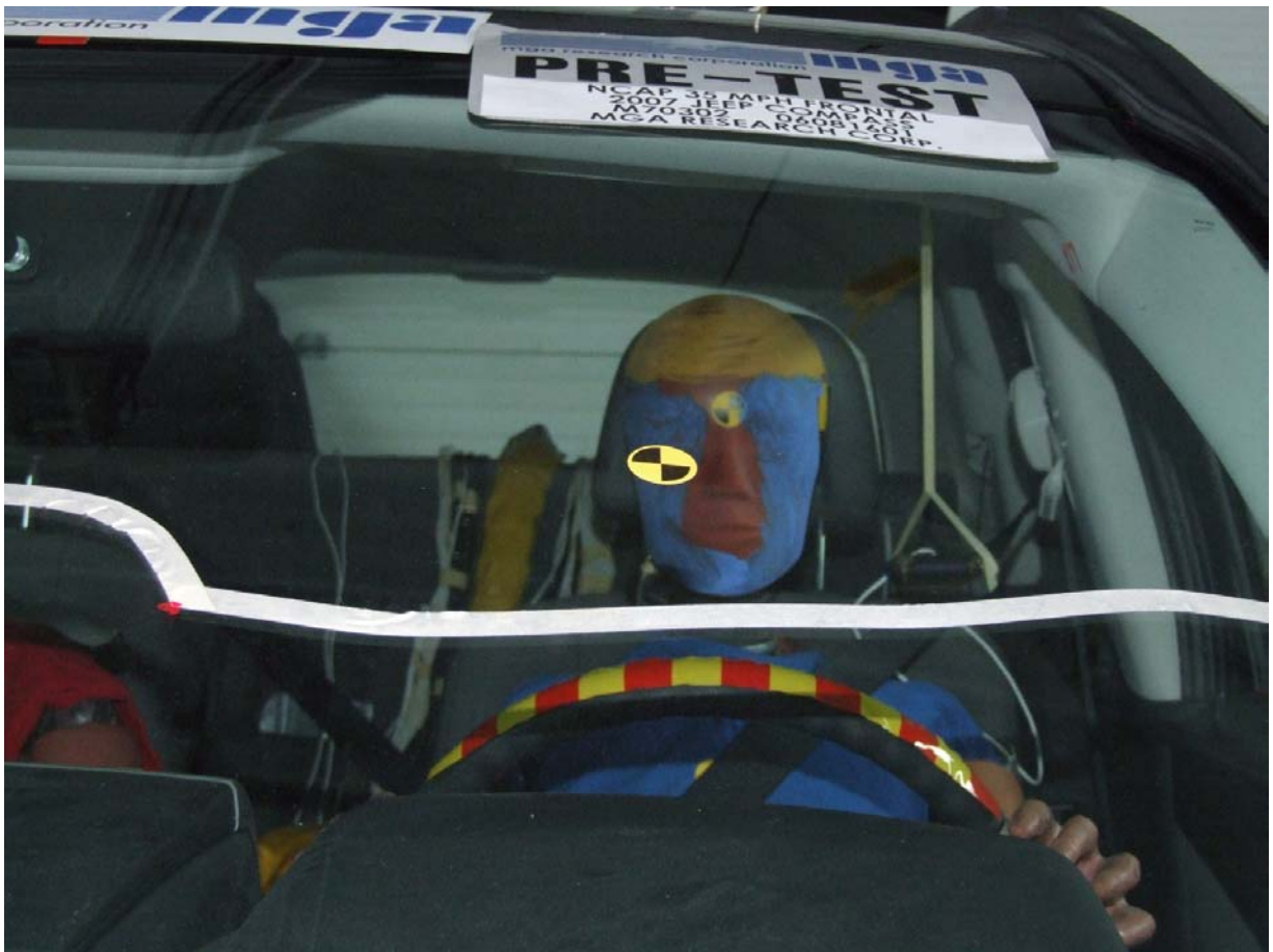
Pre-Test Driver Dummy Front View (Head Position)
