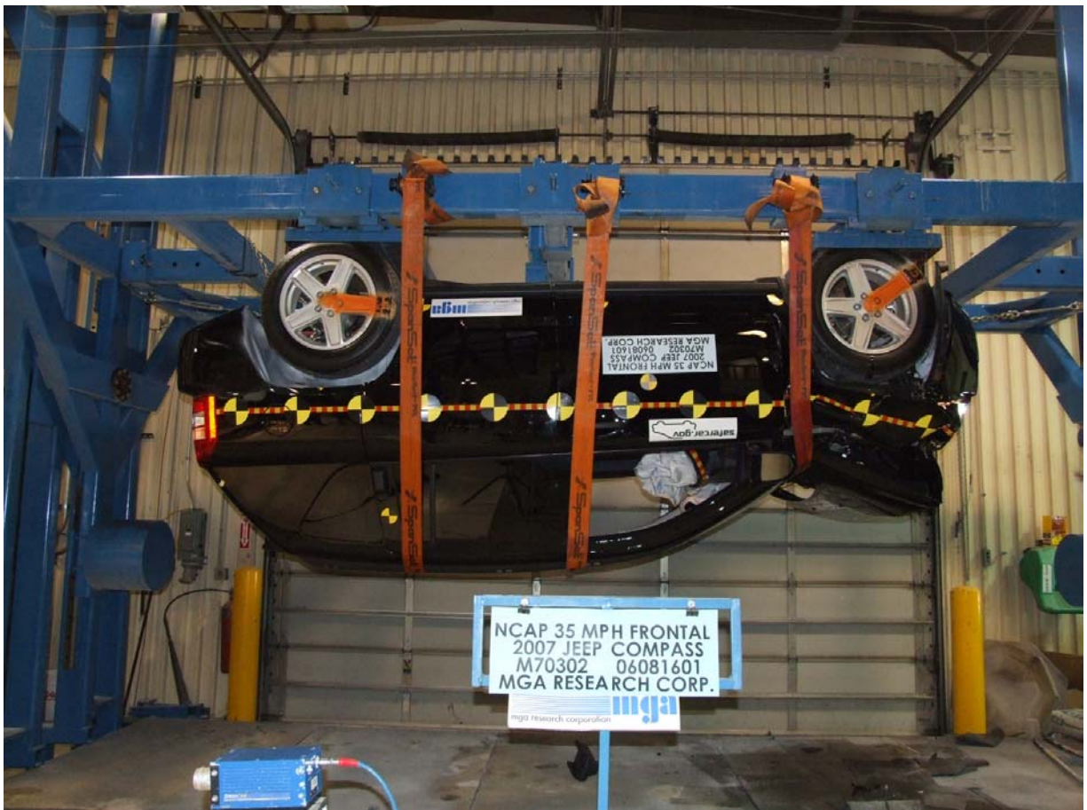
Vehicle on Rollover Device at 180 Degrees
