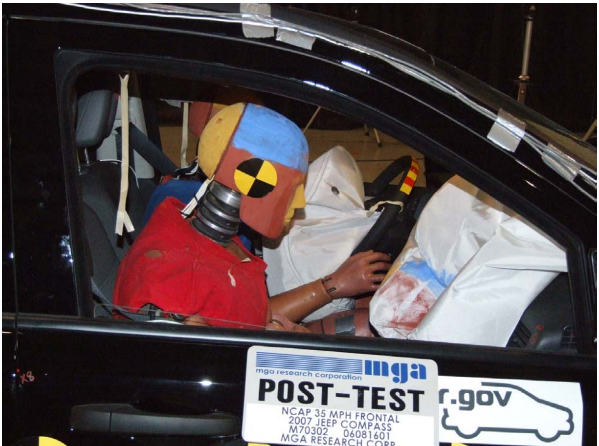
Post-Test Passenger Dummy (Through Window)
