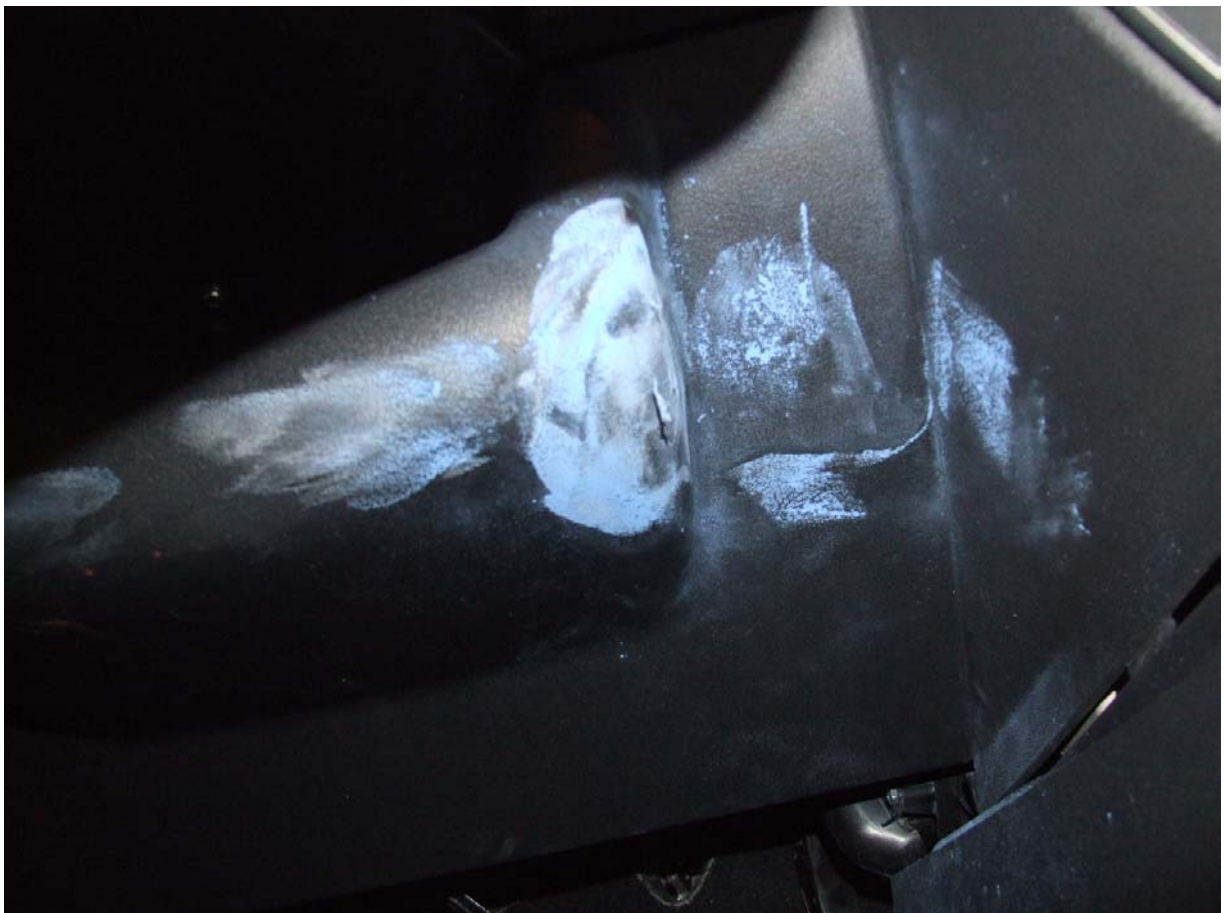
Post-Test Driver Dummy Right Knee Contact
