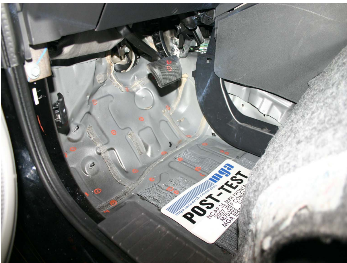
Post-Test Driver Side Floor Pan
