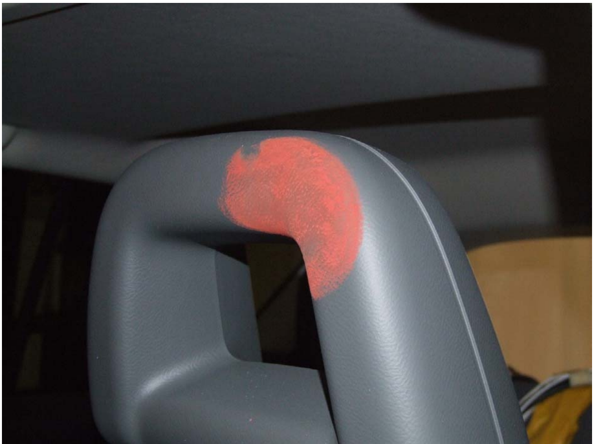
Post-Test Driver Dummy Head Contact
