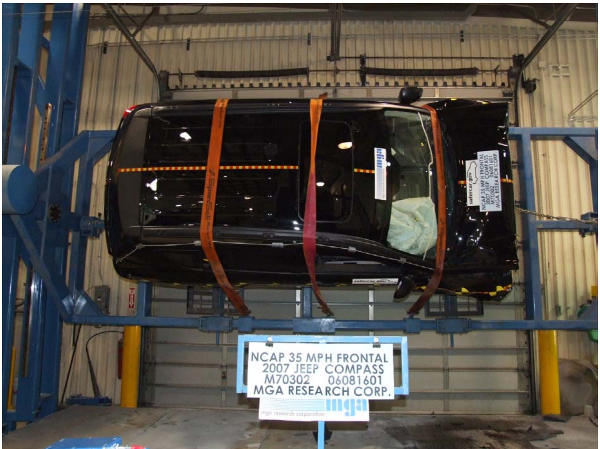
Vehicle on Rollover Device at 270 Degrees
