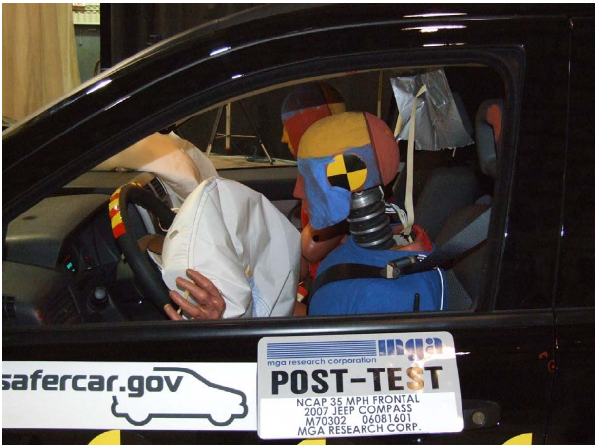
Post-Test Driver Dummy (Through Window)
