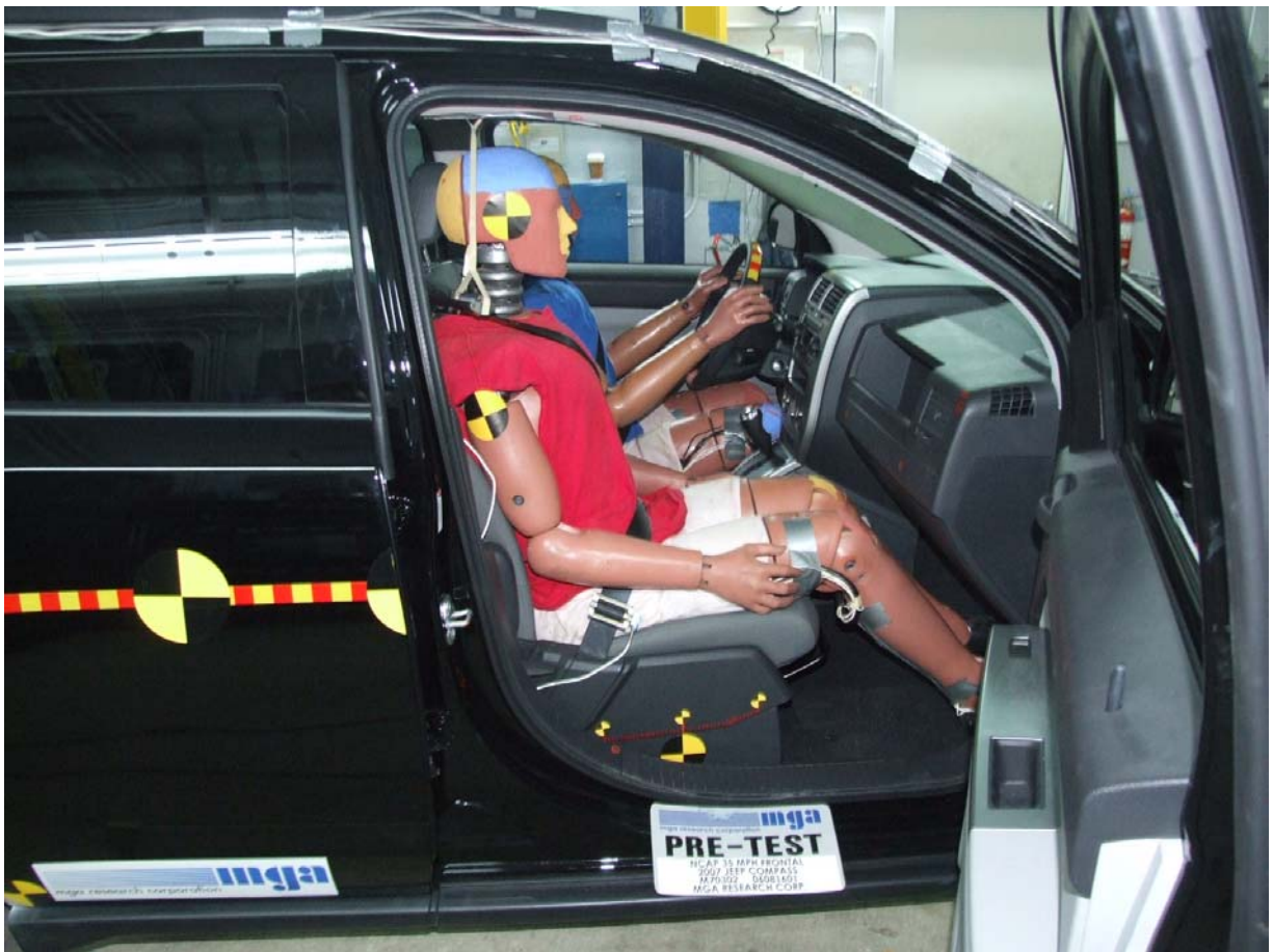
Pre-Test Passenger Dummy (Door Open)
