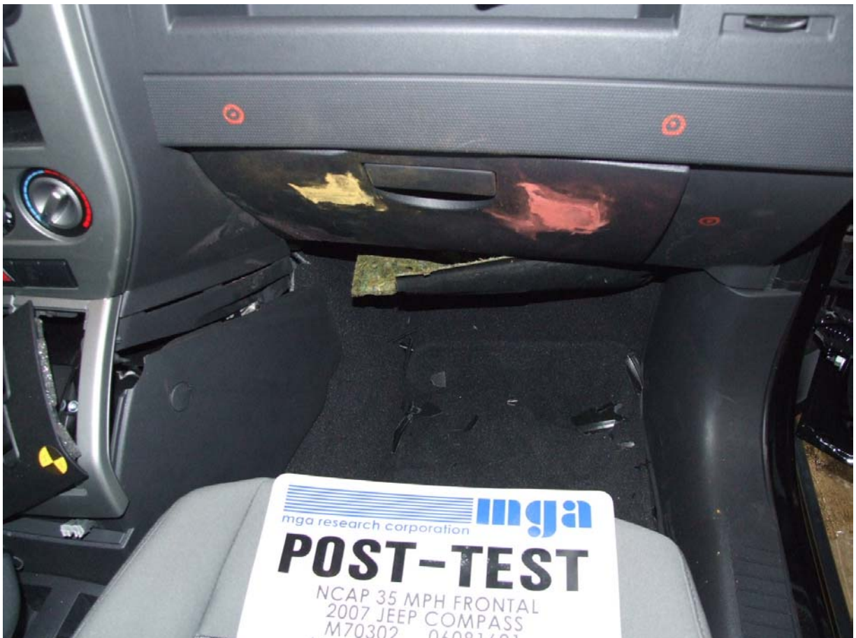
Post-Test Passenger Dummy Knee Contact
