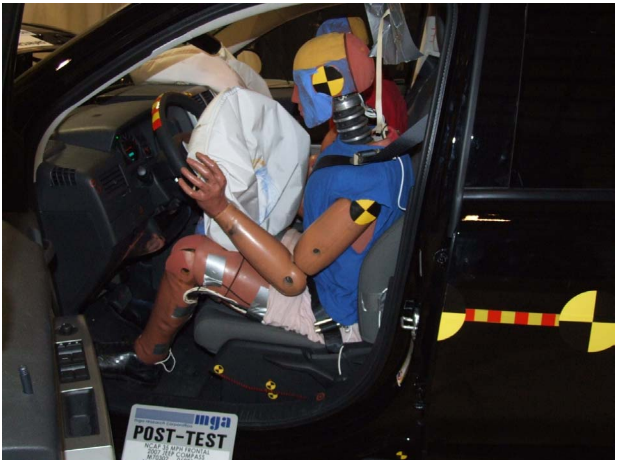
Post-Test Driver Dummy (Door Open)
