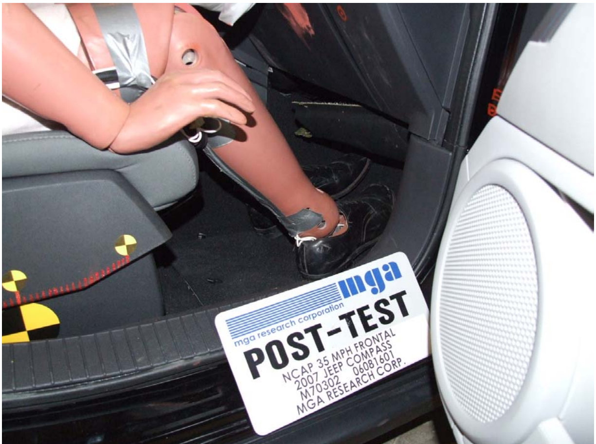
Post-Test Passenger Dummy Feet
