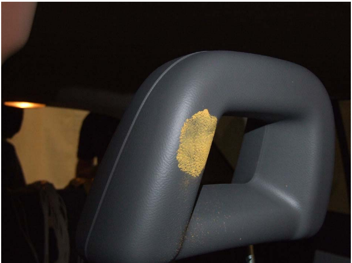
Post-Test Passenger Dummy Head Contact
