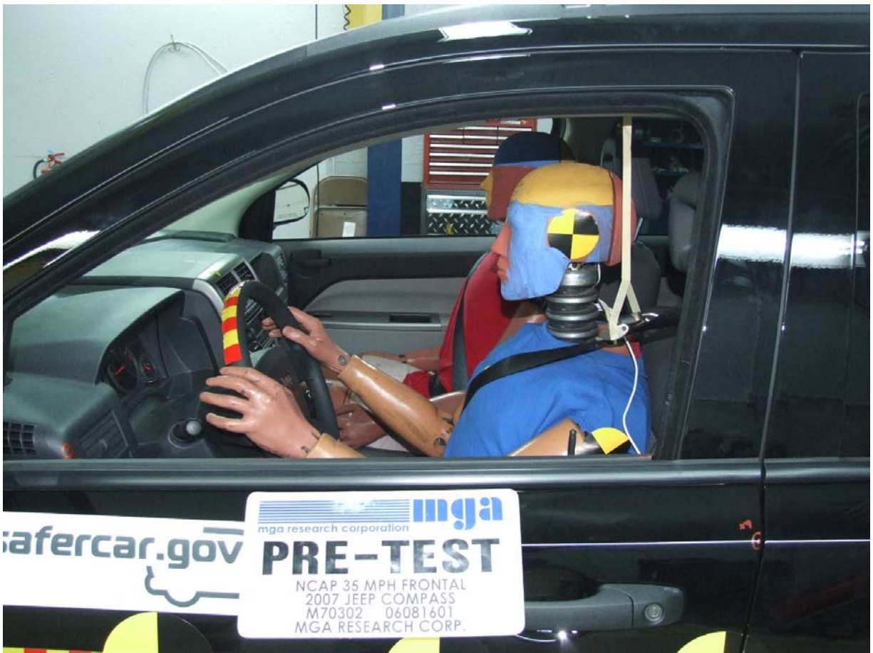
Pre-Test Driver Dummy (Through Window)
