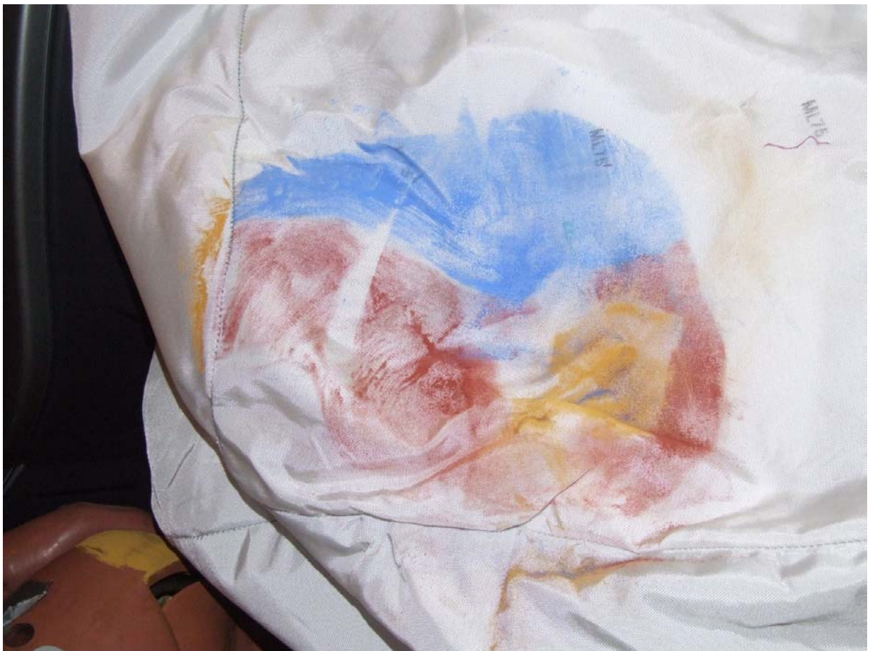
Post-Test Passenger Dummy Airbag Contact
