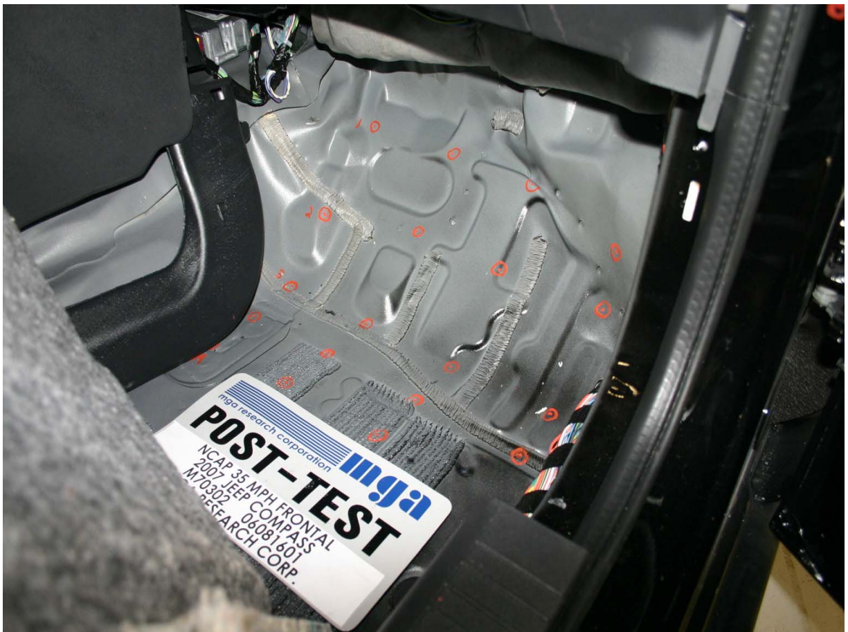
Post-Test Passenger Side Floor Pan
