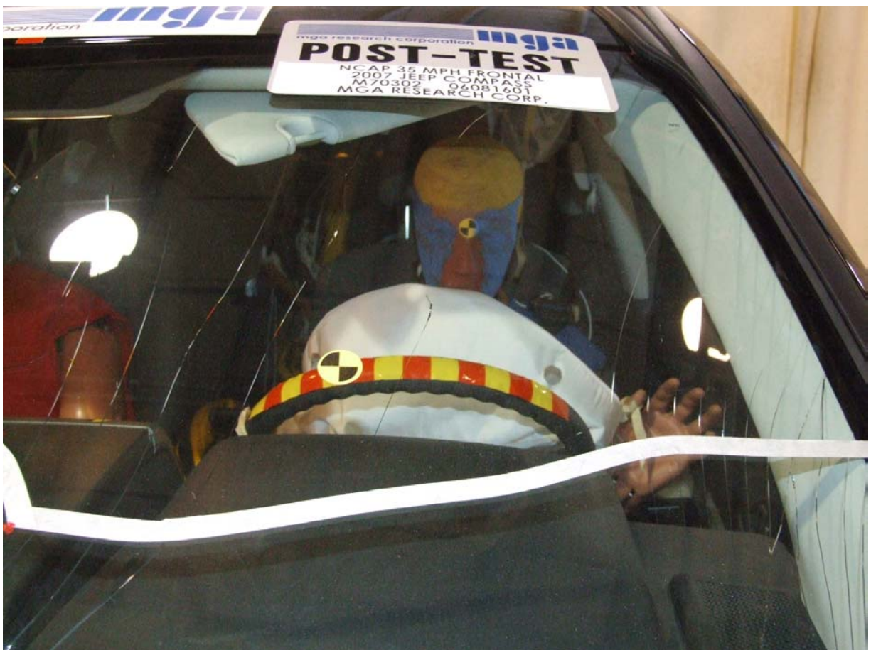
Post-Test Driver Dummy Front View (Head Position)
