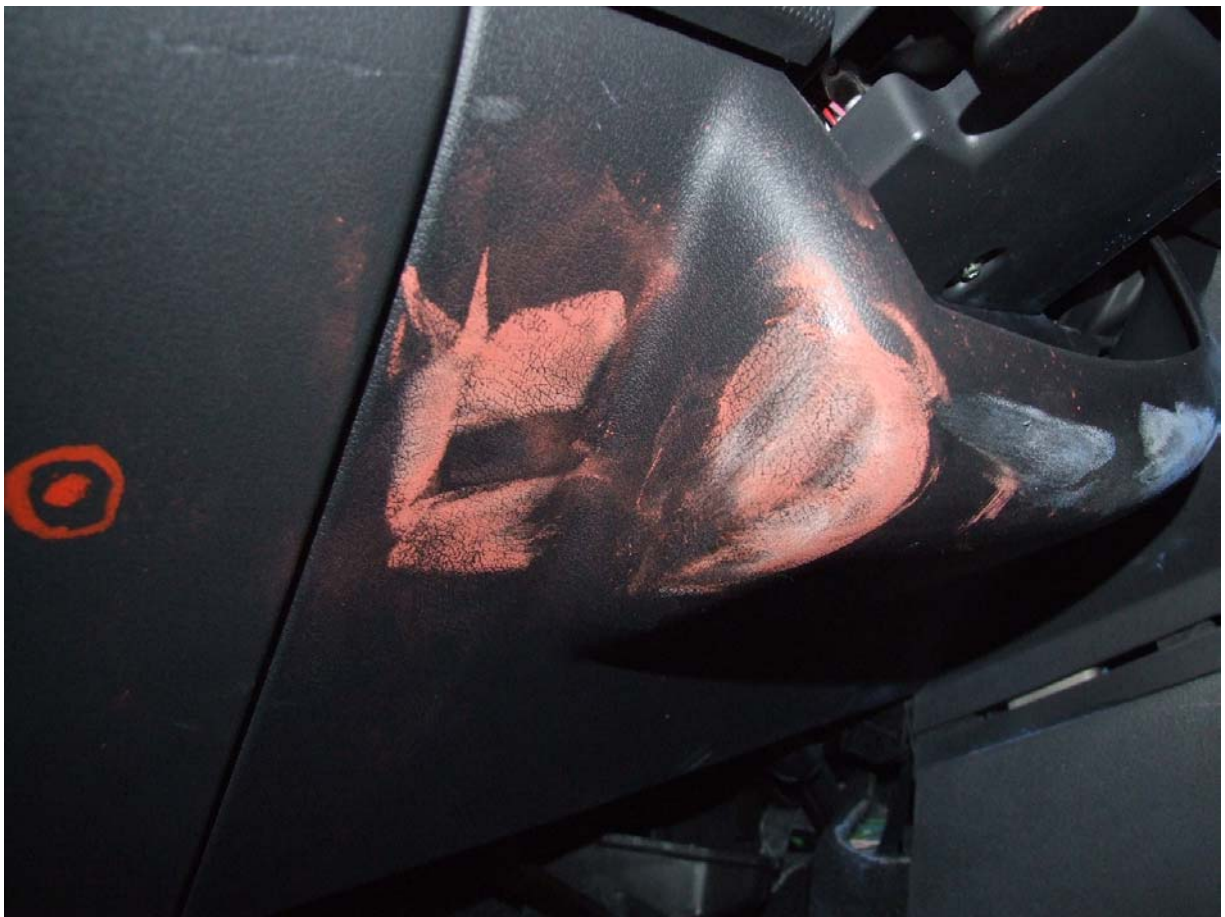
Post-Test Driver Dummy Left Knee Contact
