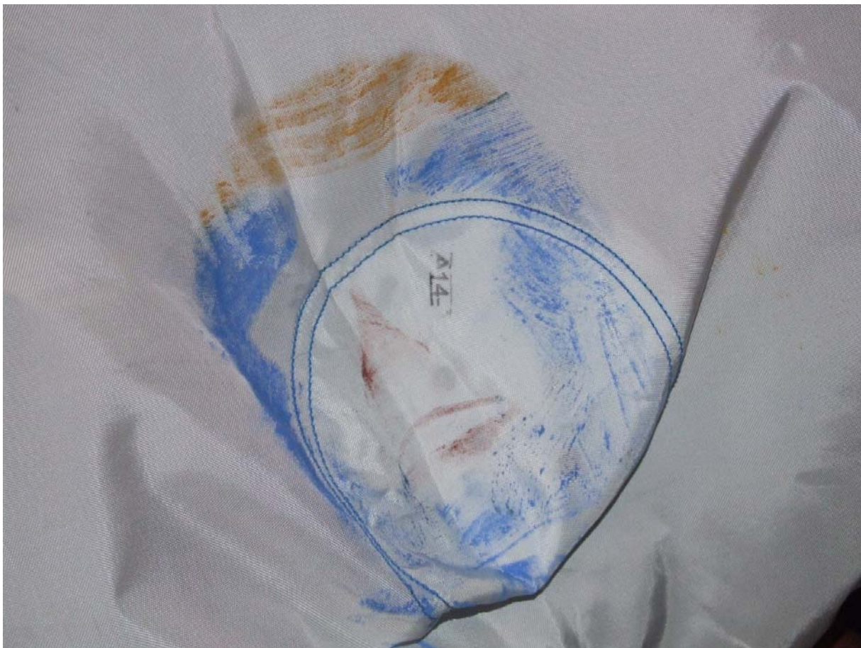
Post-Test Driver Dummy Airbag Contact
