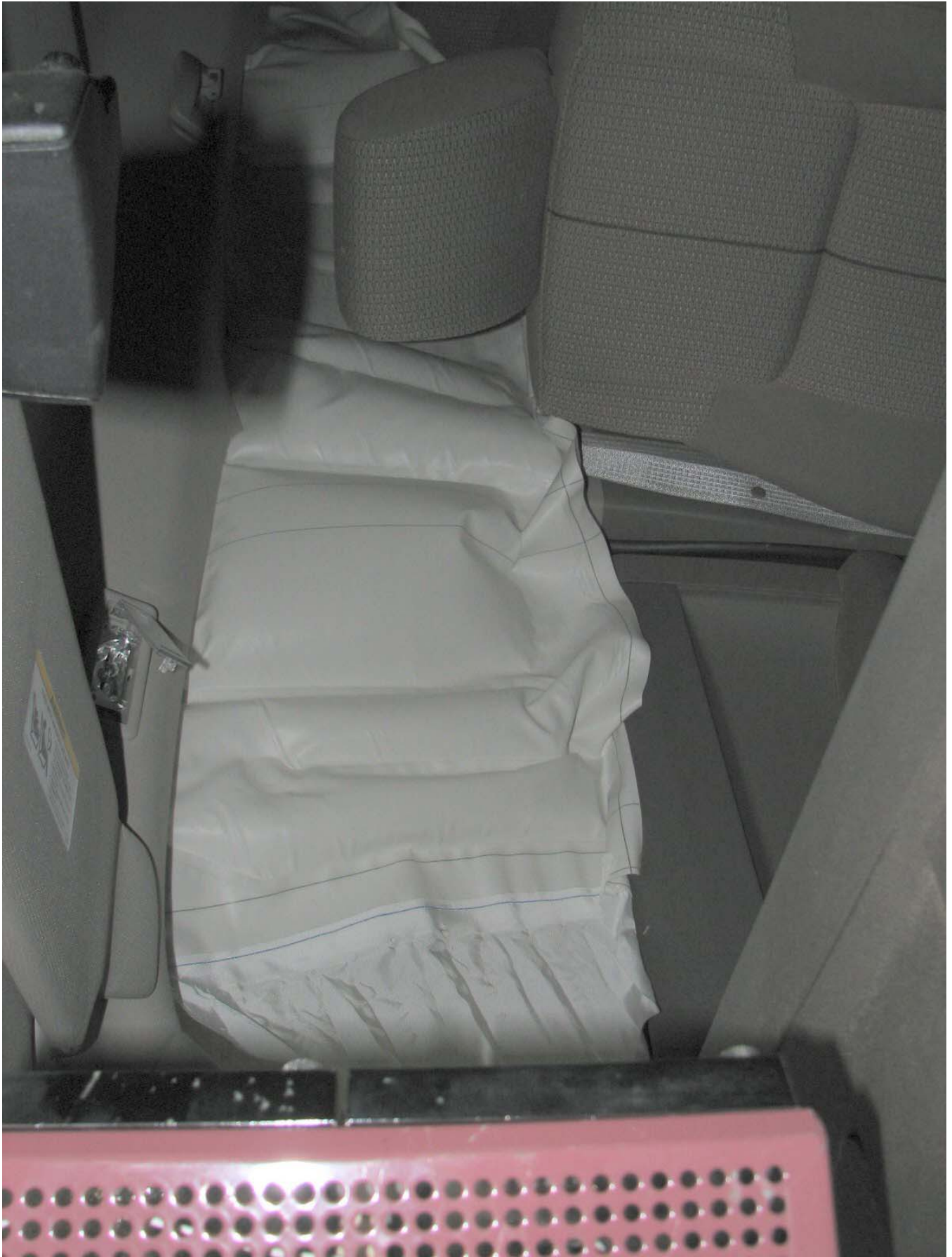
Figure A-10: Post-Test Airbags, Close-up View
