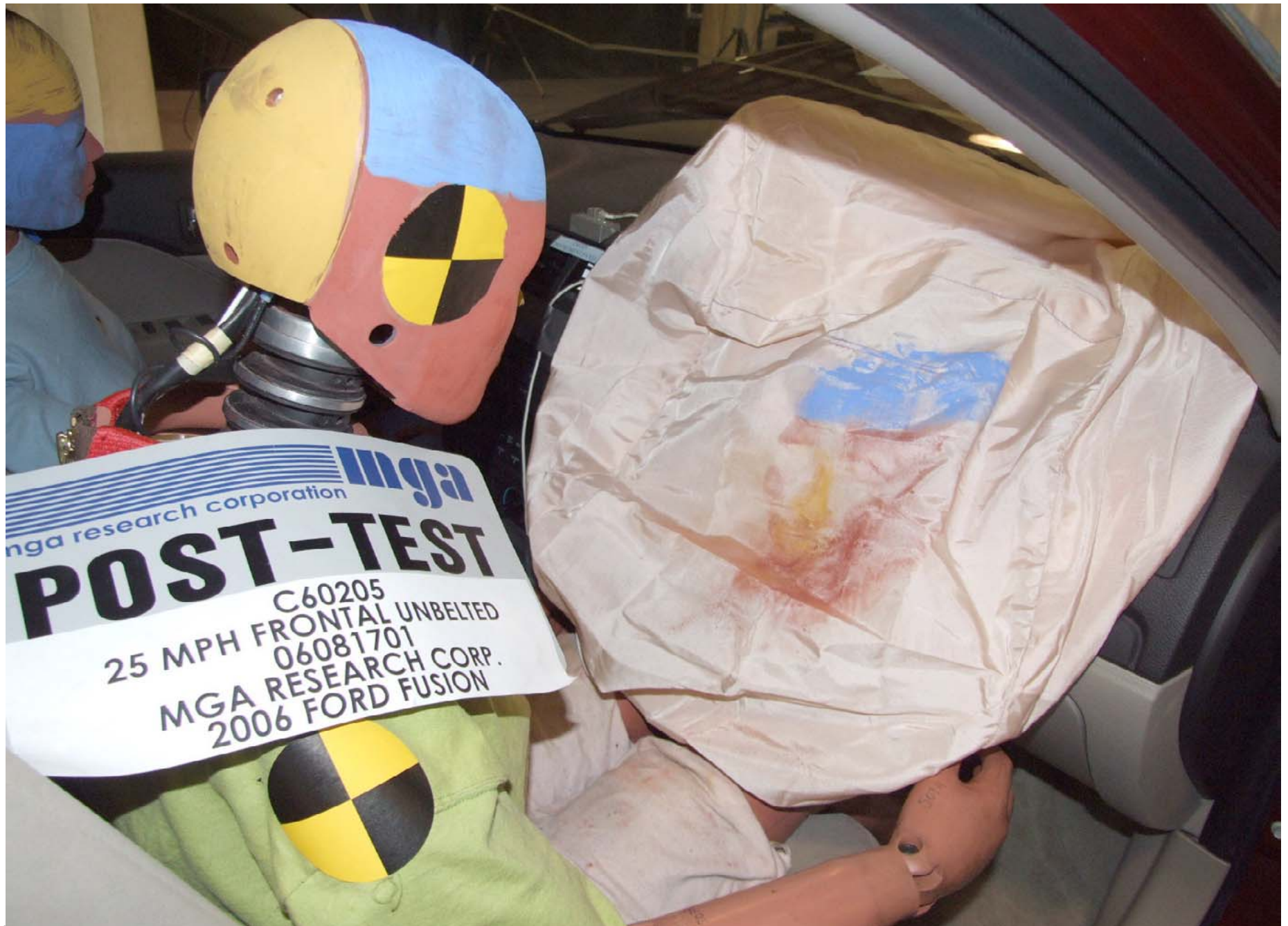
Post-Test Passenger Dummy Airbag Contact
