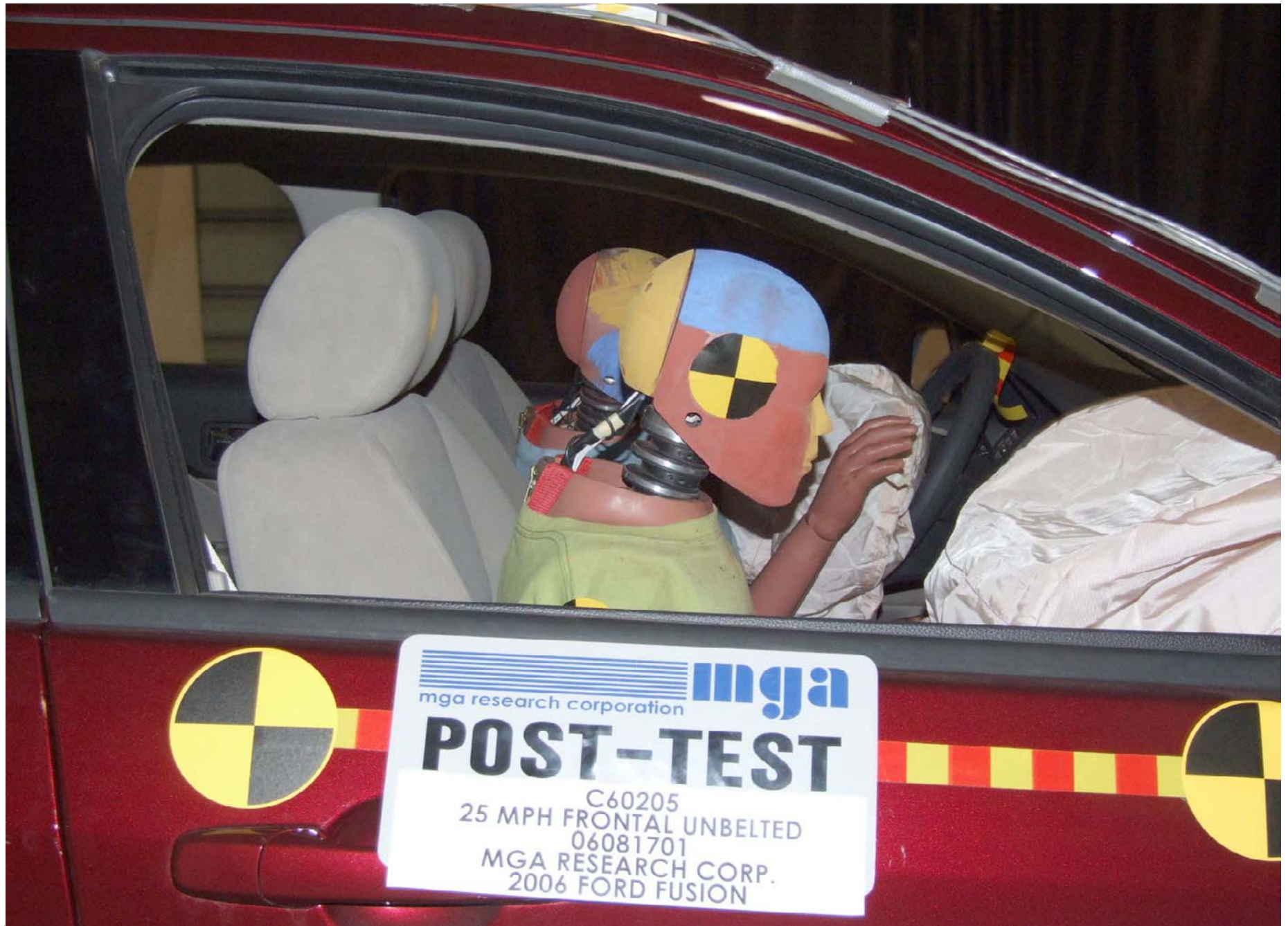
Post-Test Passenger Dummy Position Right Side View
