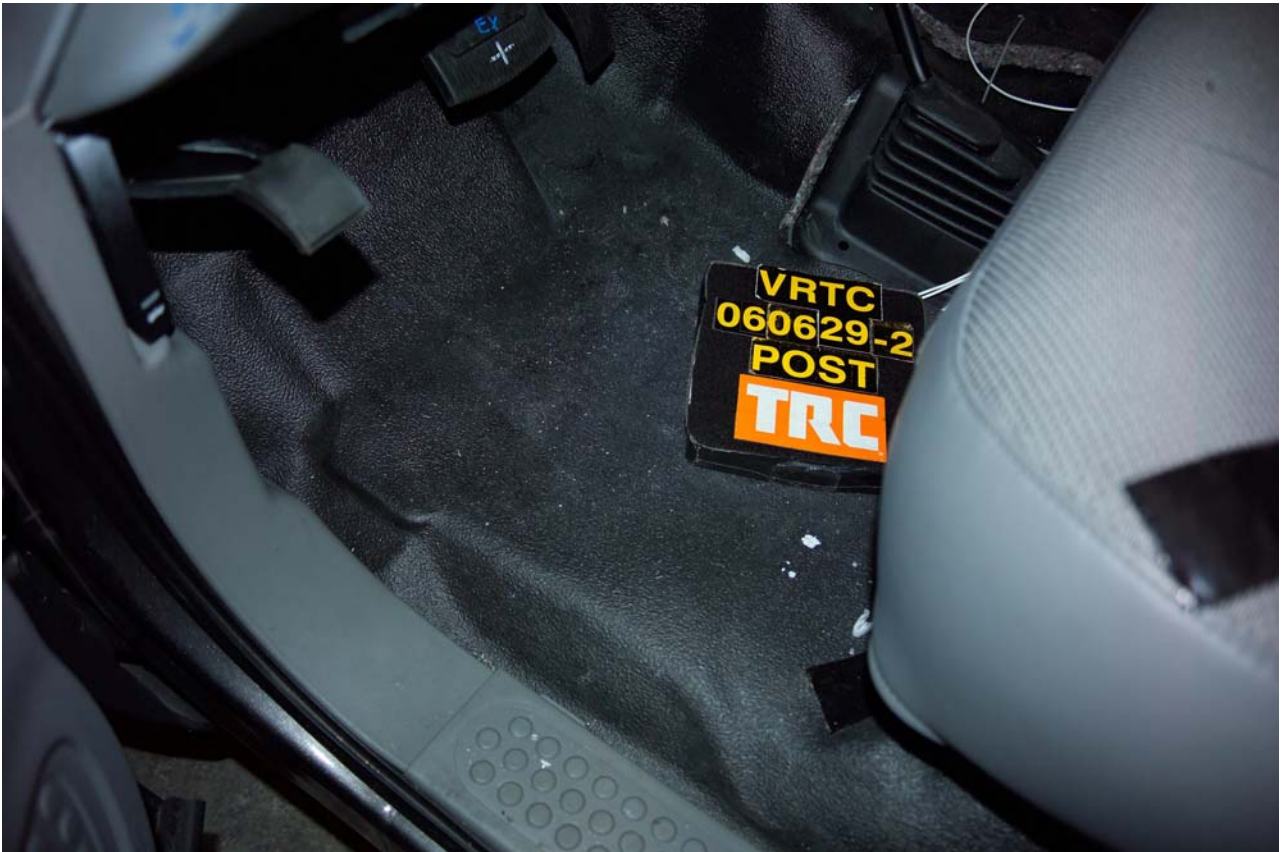
Figure A-66 Post-Test Driver Floorboard Deformation View
