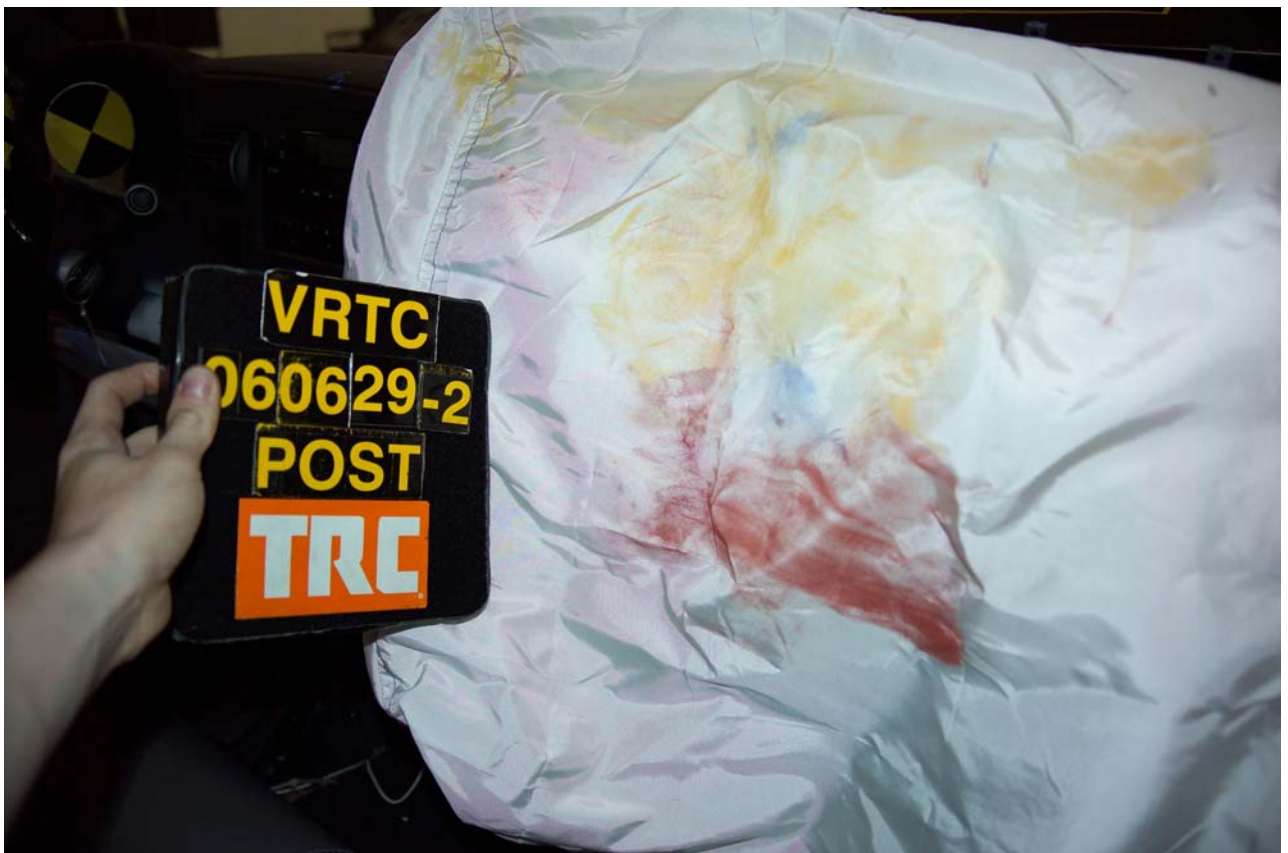
Figure A-69 Post-Test Right Front Passenger Dummy Head Contact - View 1
