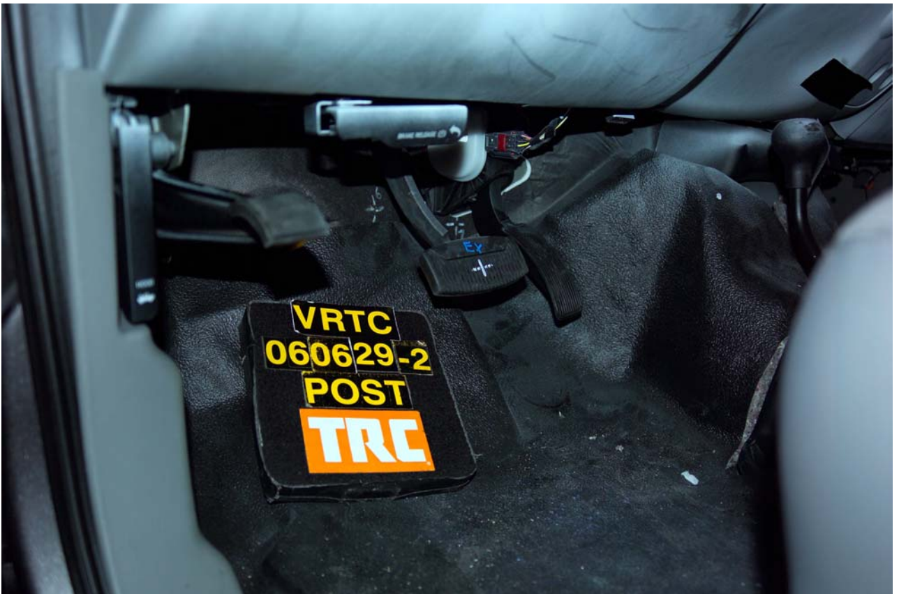
Figure A-67 Post-Test Driver Toeboard Deformation View
