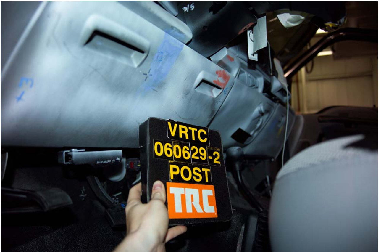
Figure A-65 Post-Test Driver Dummy Knee Contact View
