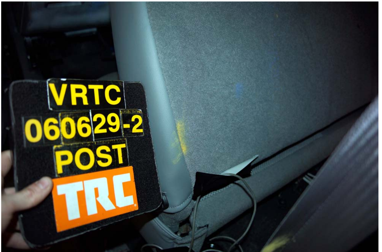
Figure A-76 Post-Test Left Rear Passenger Dummy Knee Contact View
