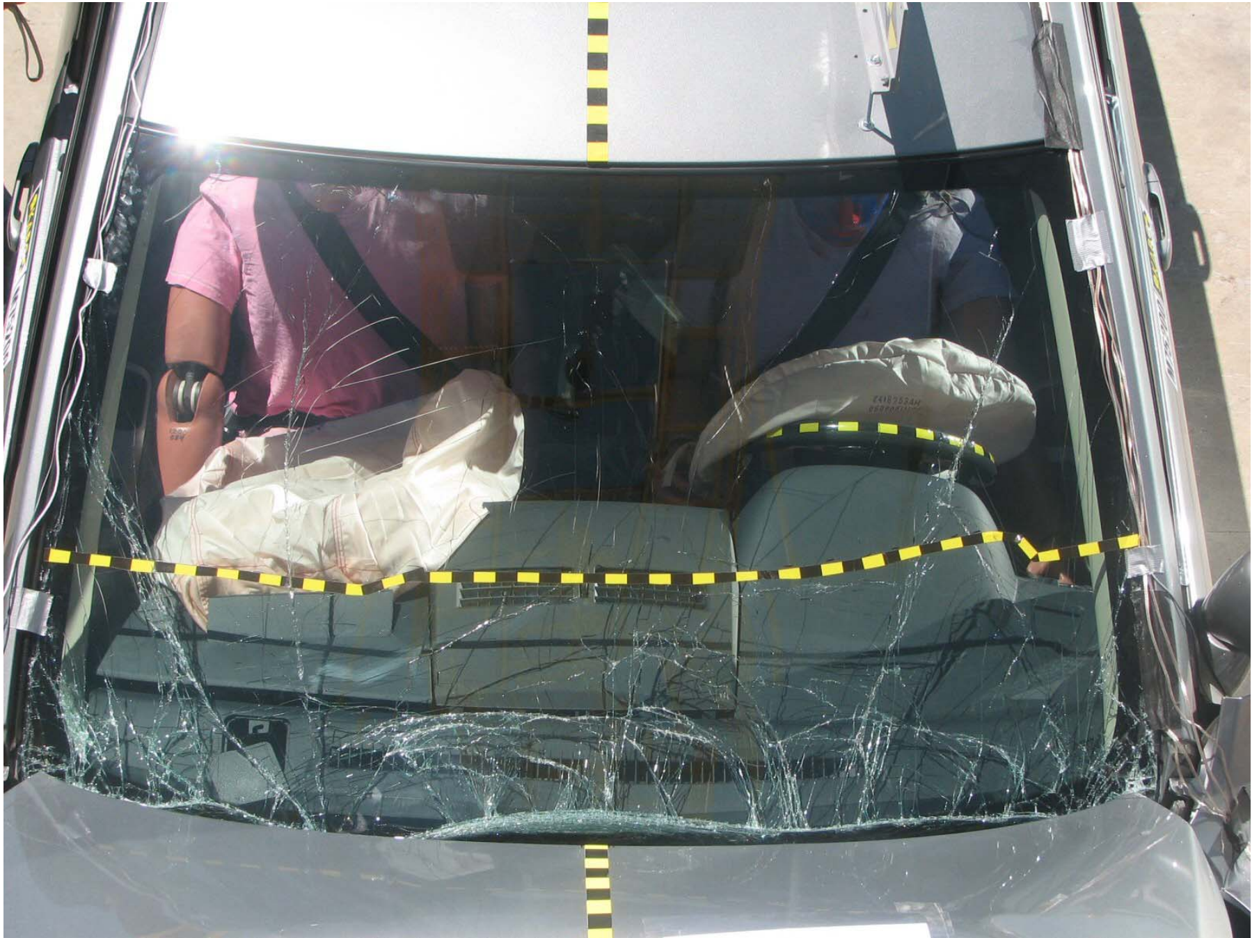
Figure A-19: Post-Test Windshield
