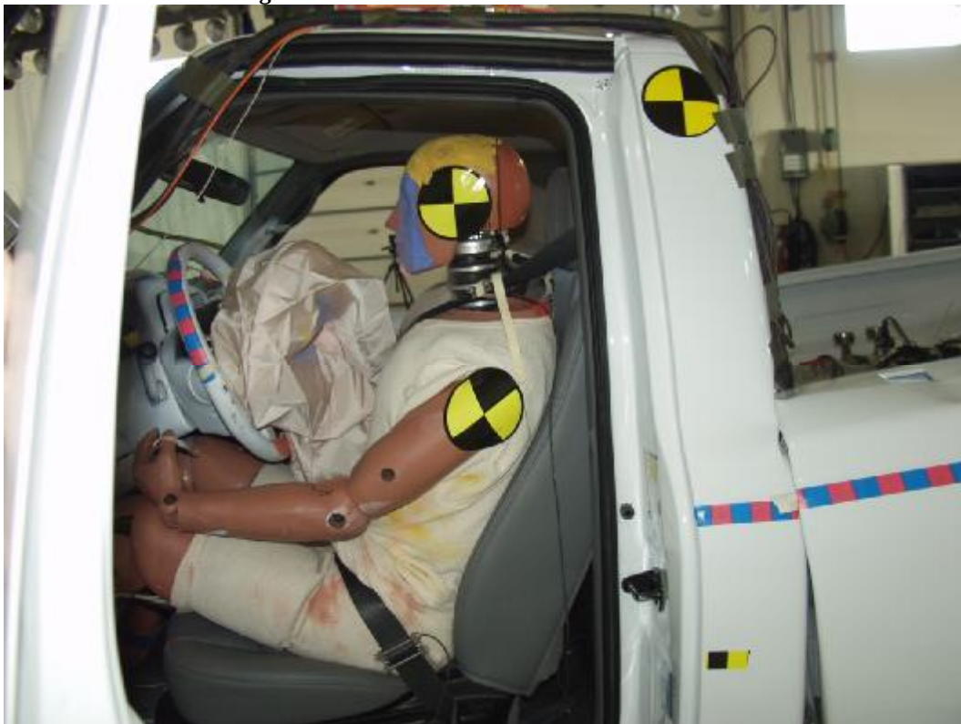
Figure A-35: Post-Test Driver and Interior View
