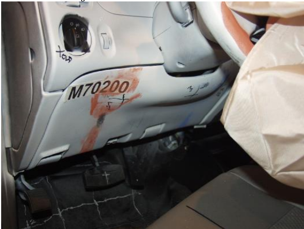
Figure A-39: Post-Test Driver Knee Bolster View
