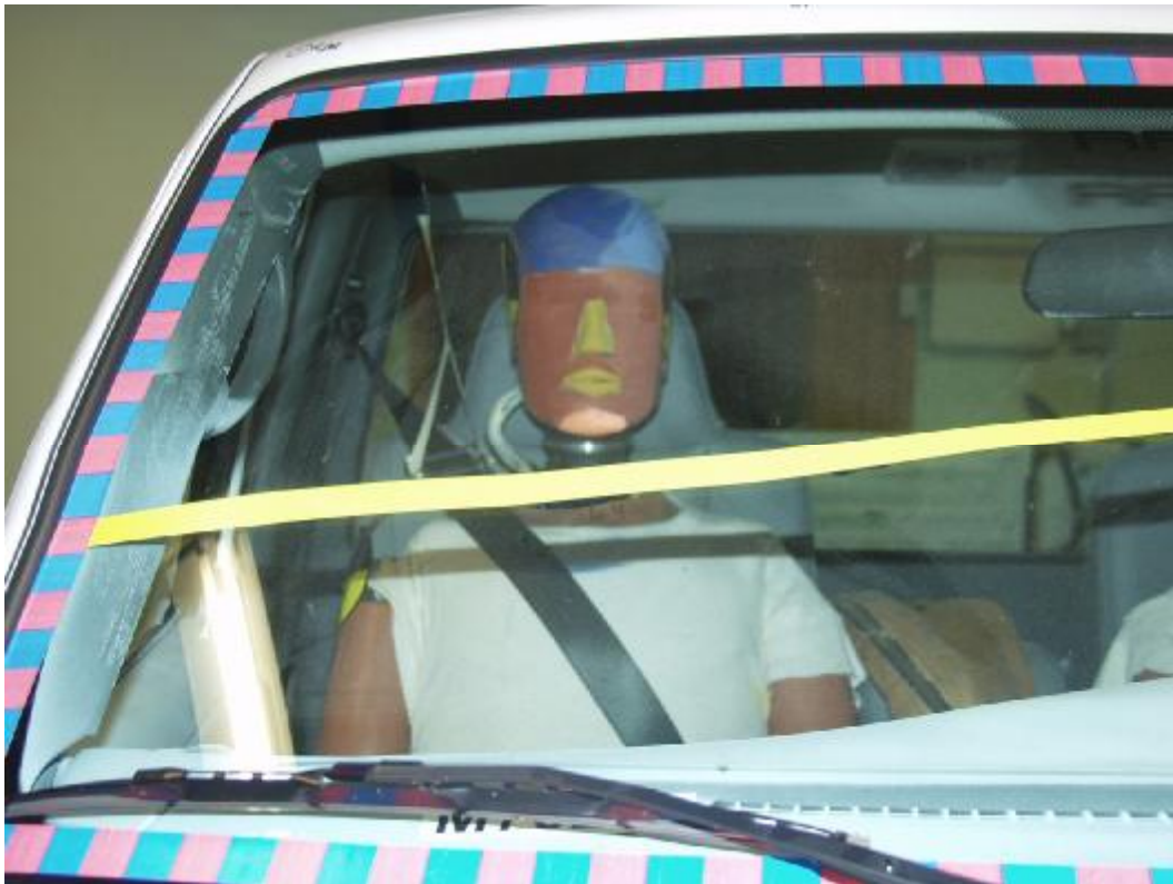
Figure A-44: Pre-Test Passenger Head Location
