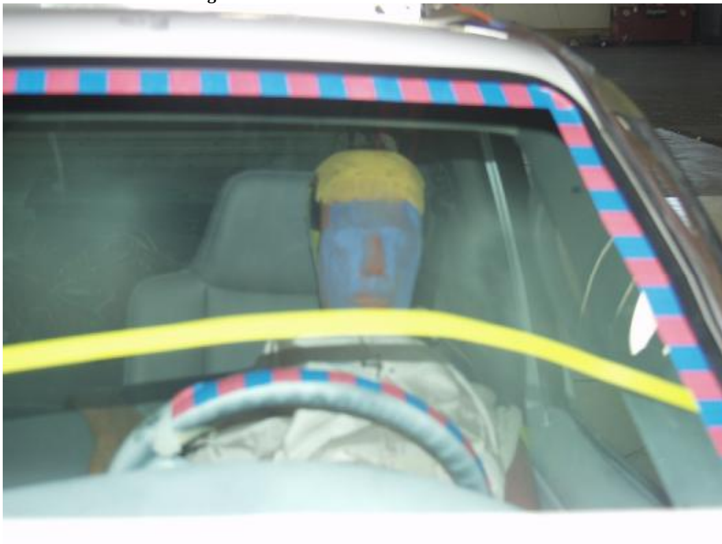
Figure A-31: Post-Test Driver Head Location
