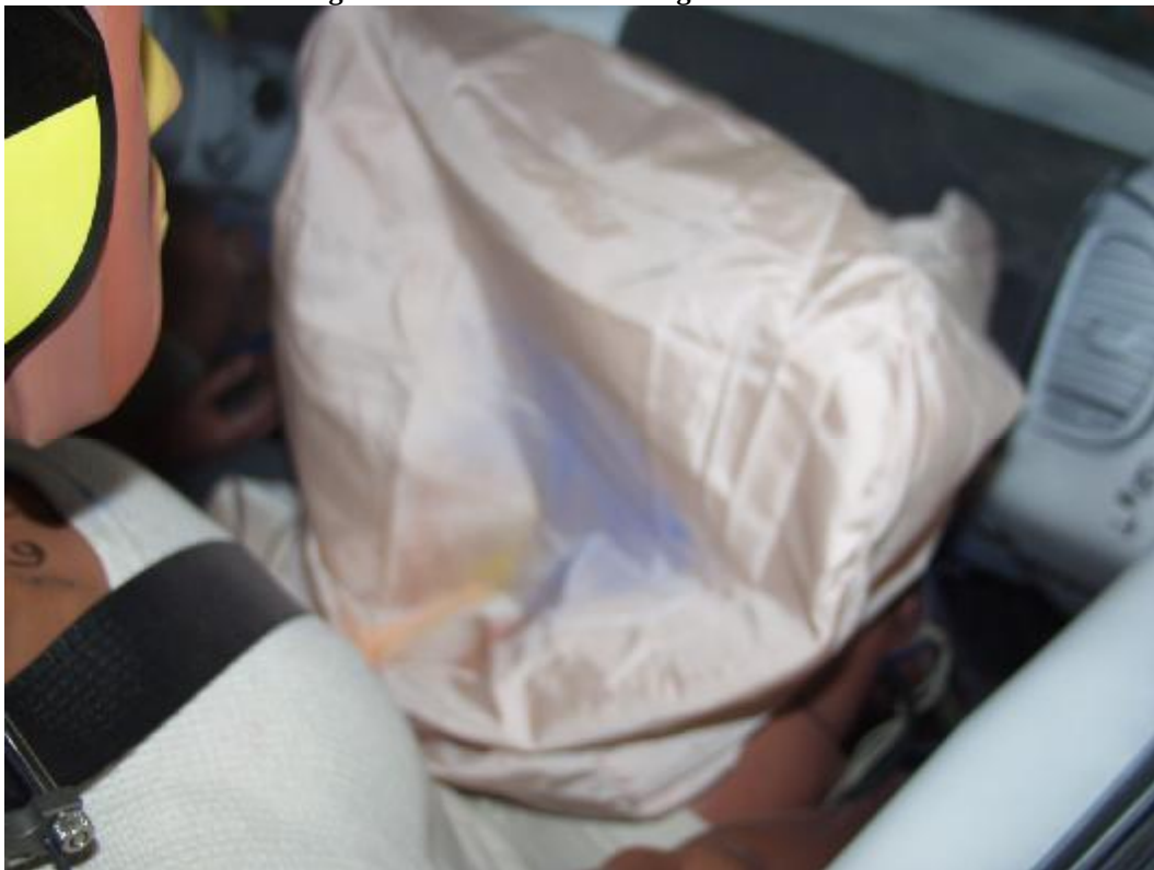
Figure A-57: Post-Test Passenger Contact to Airbag
