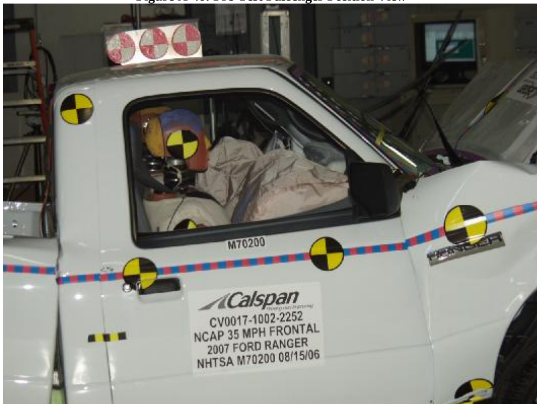
Figure A-47: Post-Test Passenger Position View
