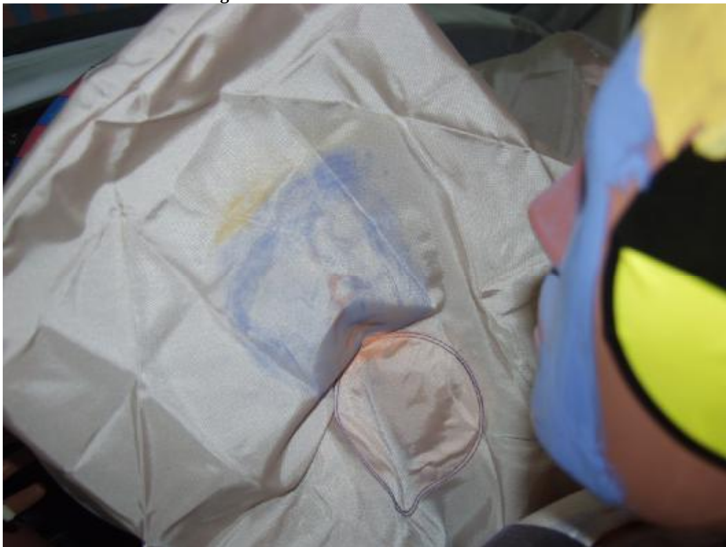
Figure A-43: Post-Test Driver Contact to Airbag
