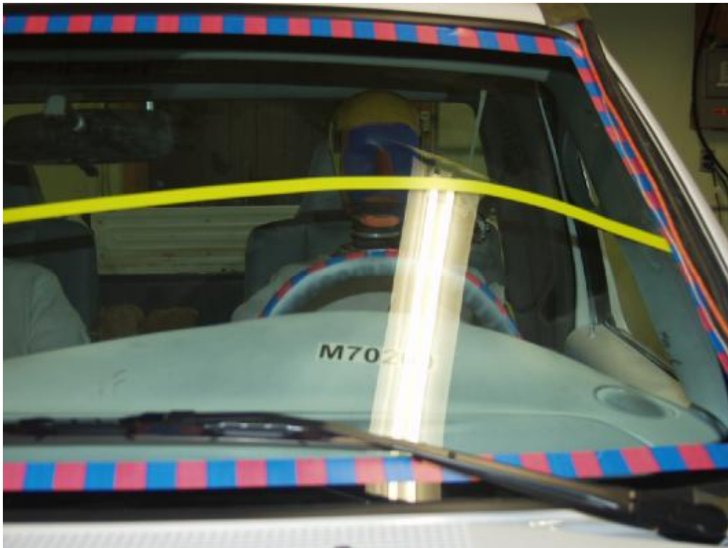
Figure A-30: Pre-Test Driver Head Location
