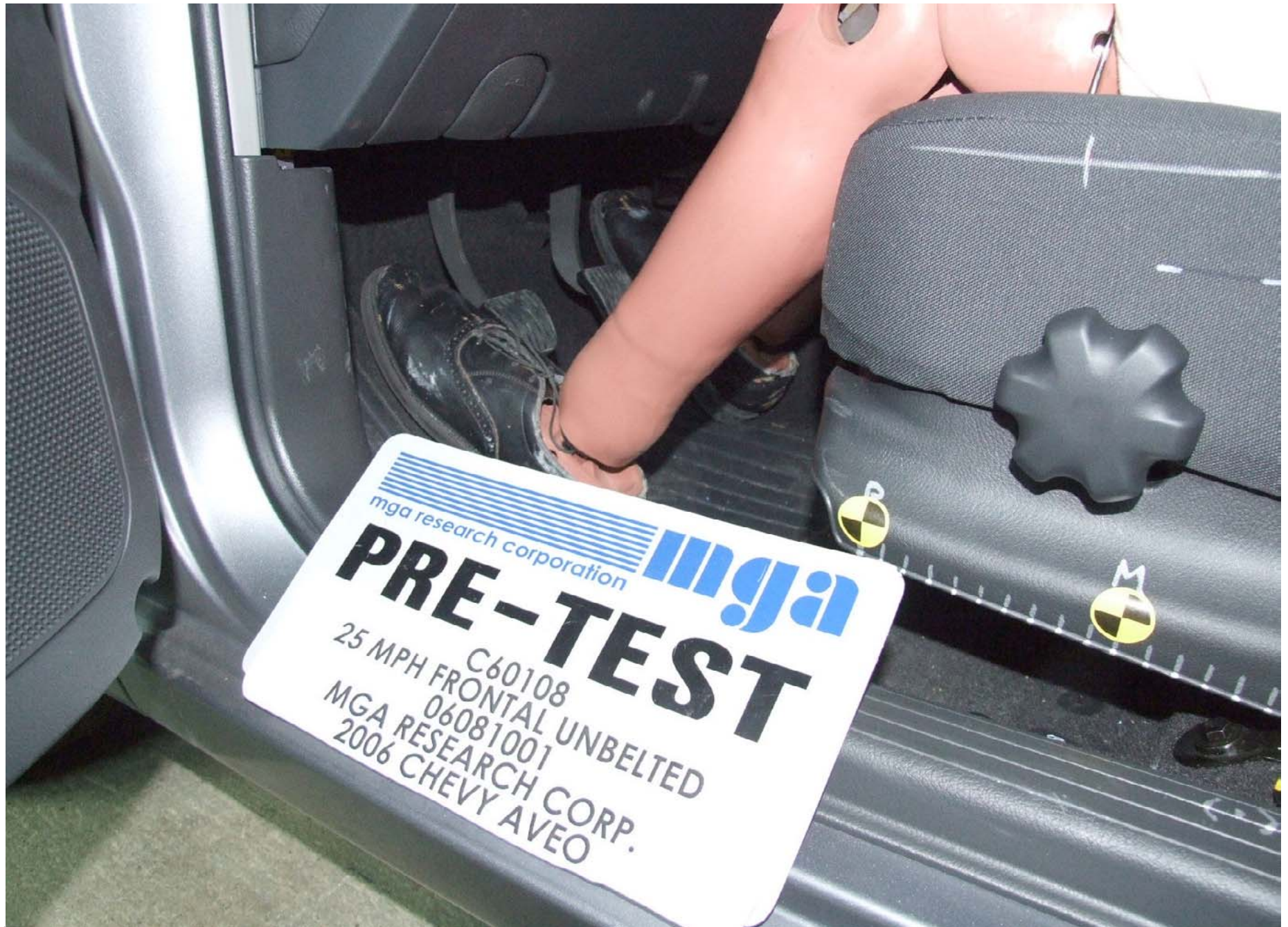
Pre-Test Driver Dummy Feet Position
