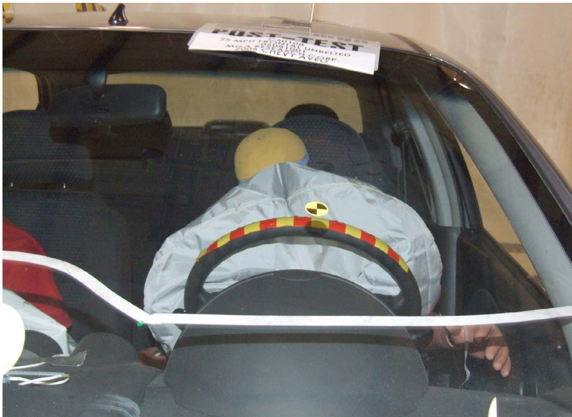
Post-Test Driver Dummy Front View (head position)
