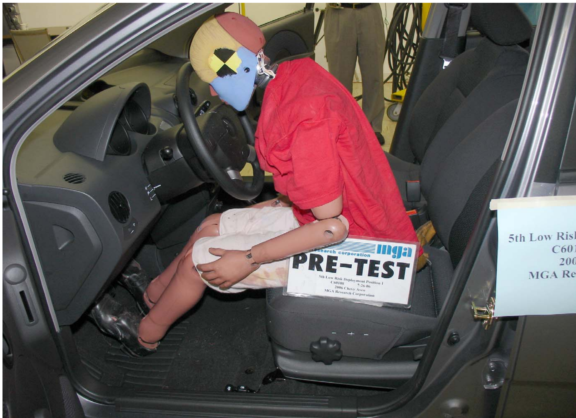
Pre-Test 5th Fem. P1 Driver Dummy Left Side View (Door Open)
