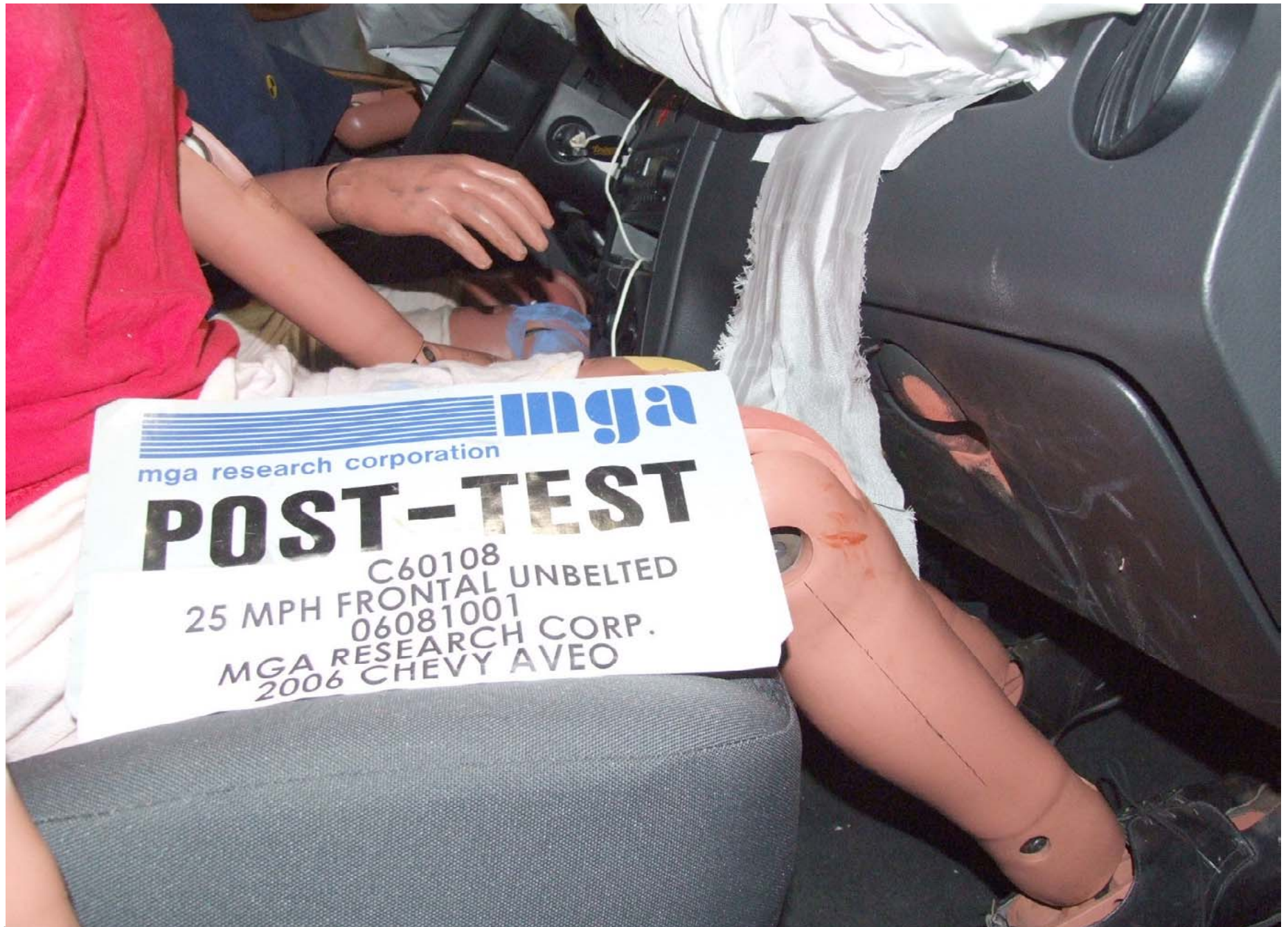
Post-Test Passenger Side Knee Bolster View
