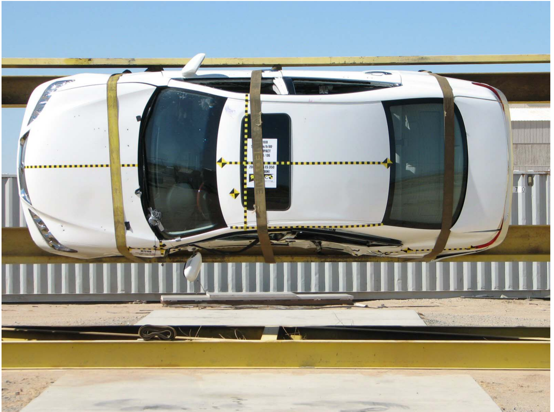
Figure A-62: Vehicle on Rollover Device (90°)
