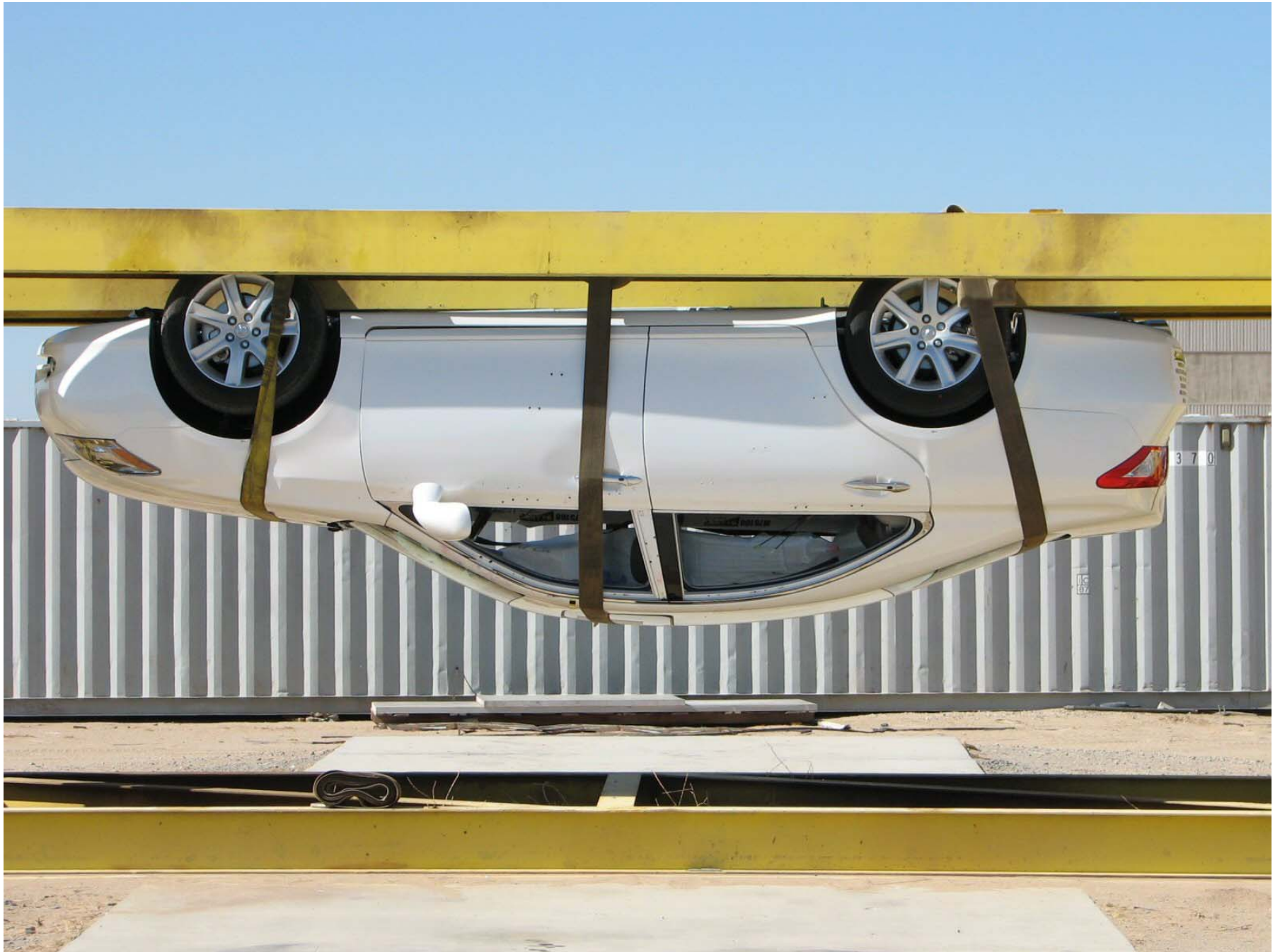
Figure A-63: Vehicle on Rollover Device (180°)
