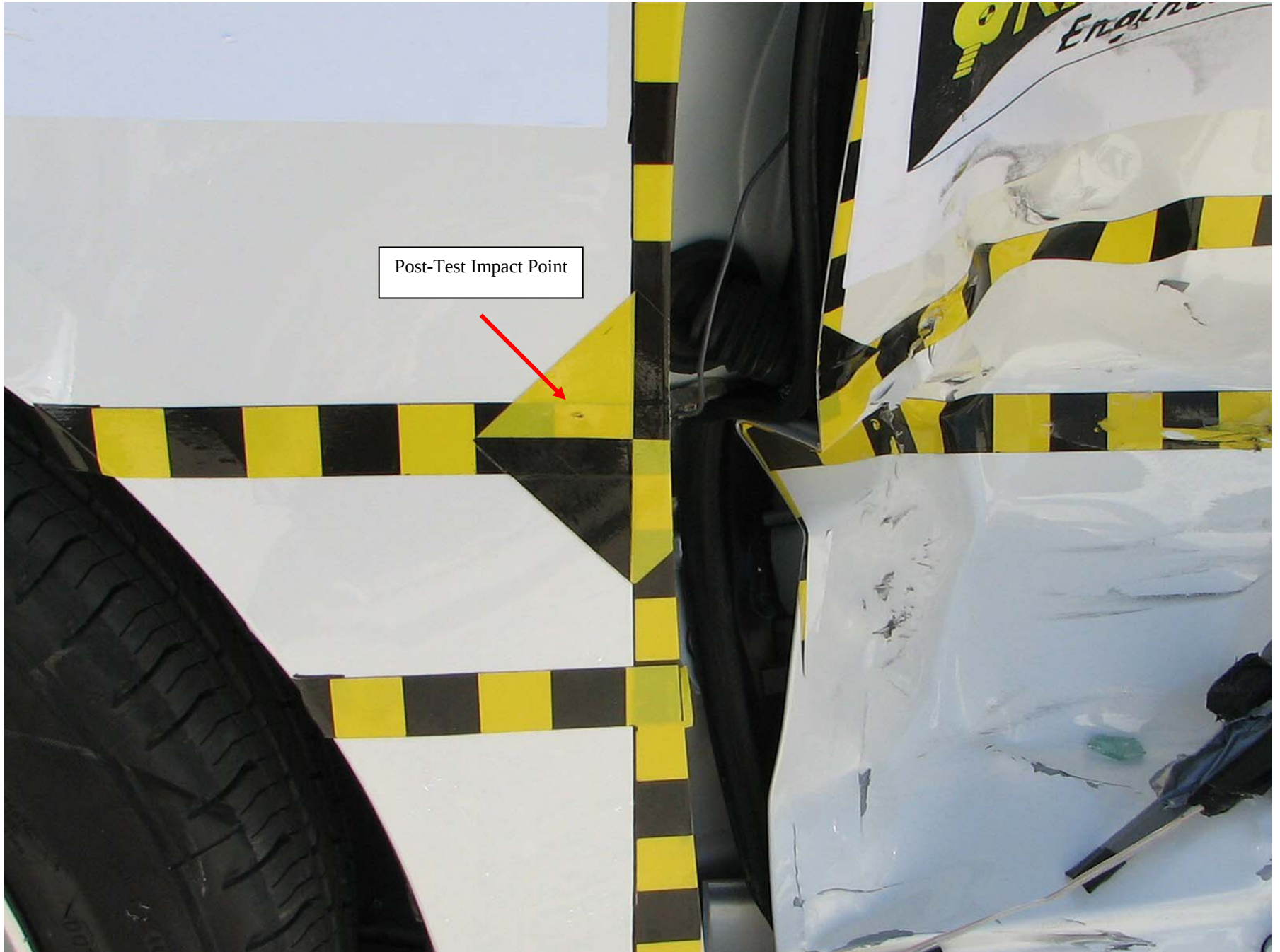
Figure A-26: Post-Test Left Impact Point
