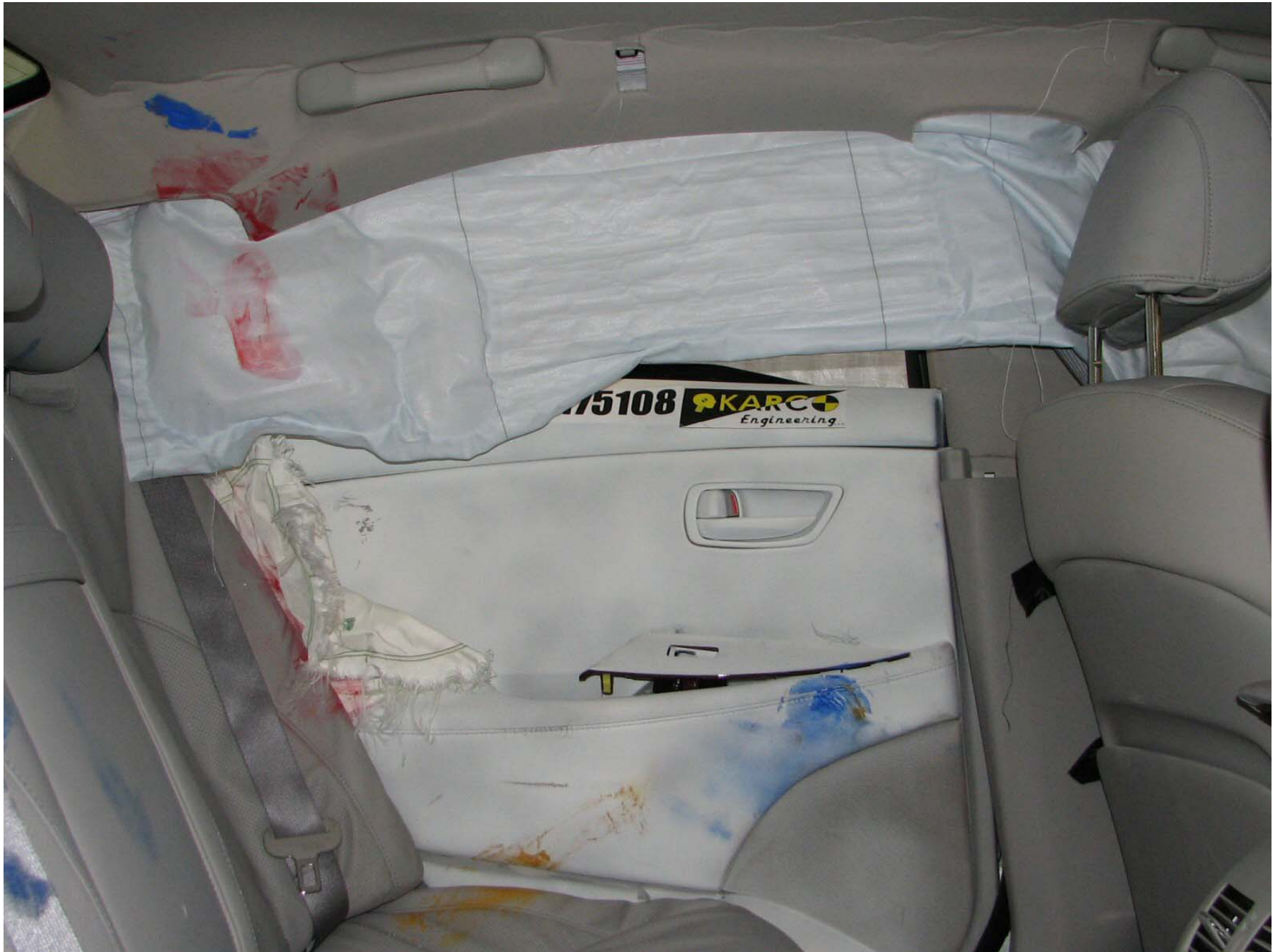
Figure A-52: Post-Test Rear Door Panel (Interior)
