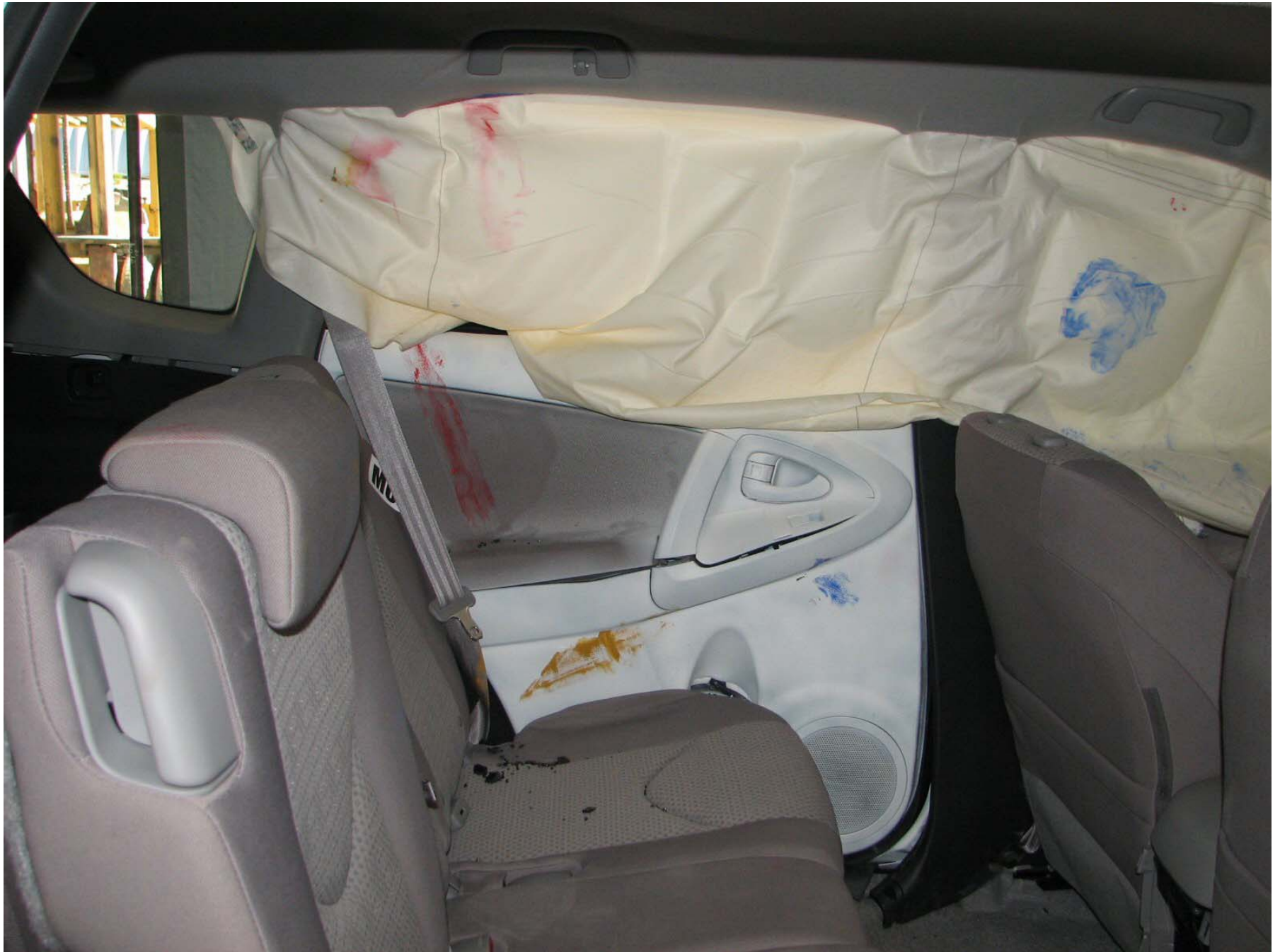
Figure A-52: Post-Test Rear Door Panel (Interior)
