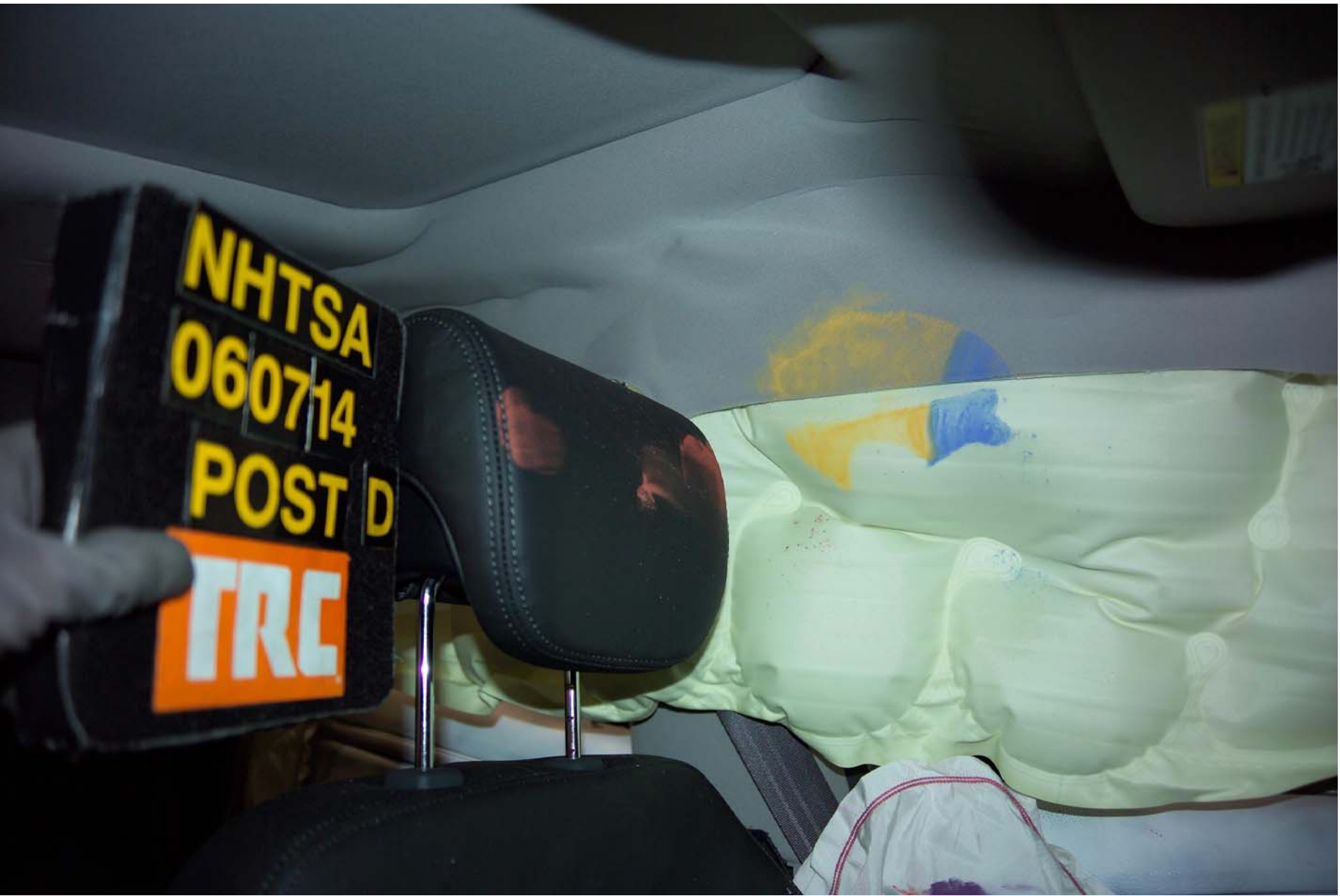
Figure A-59 Post-Test Front SID HIII Contact - View 1
