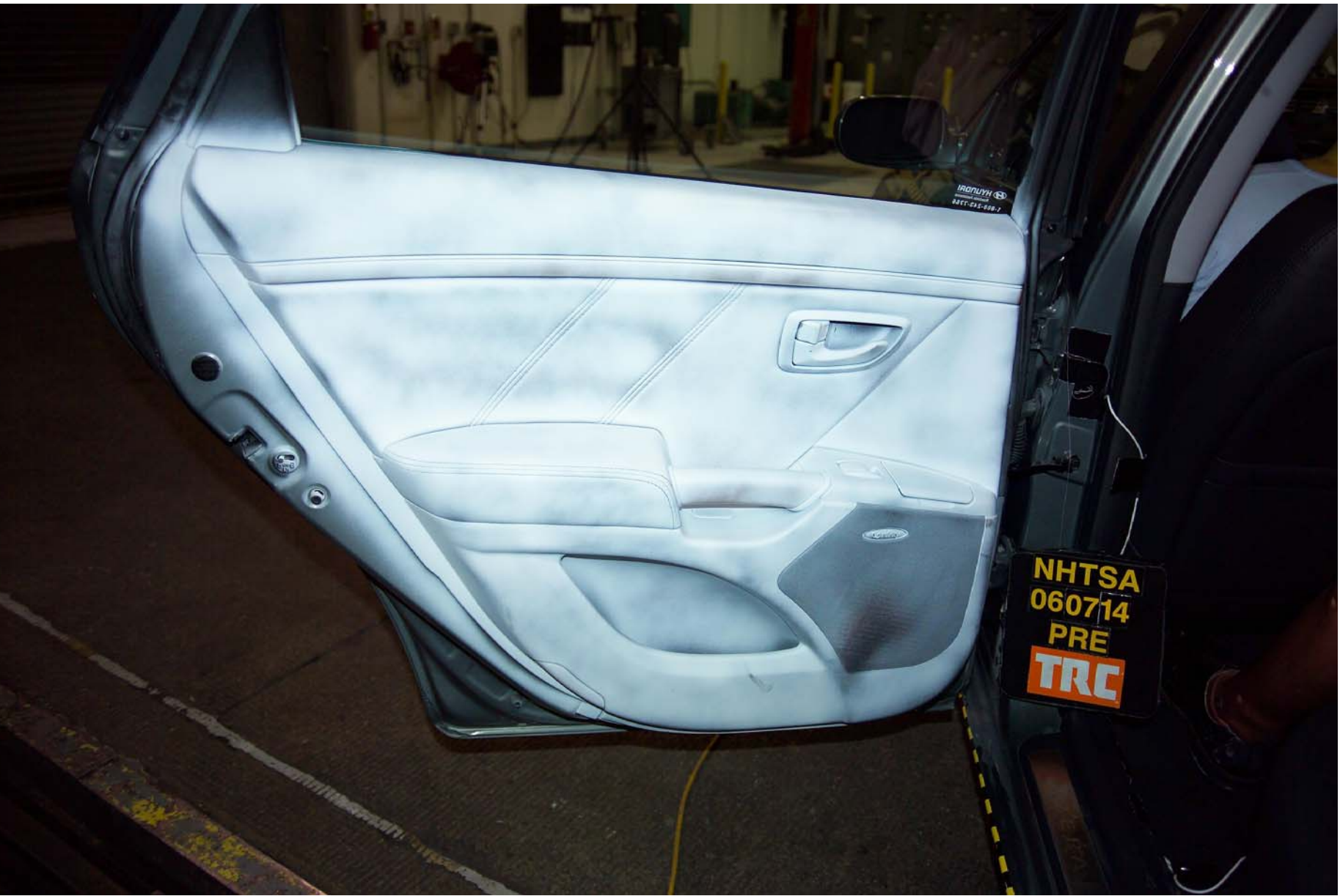
Figure A-62 Pre-Test Interior of Rear Panel
