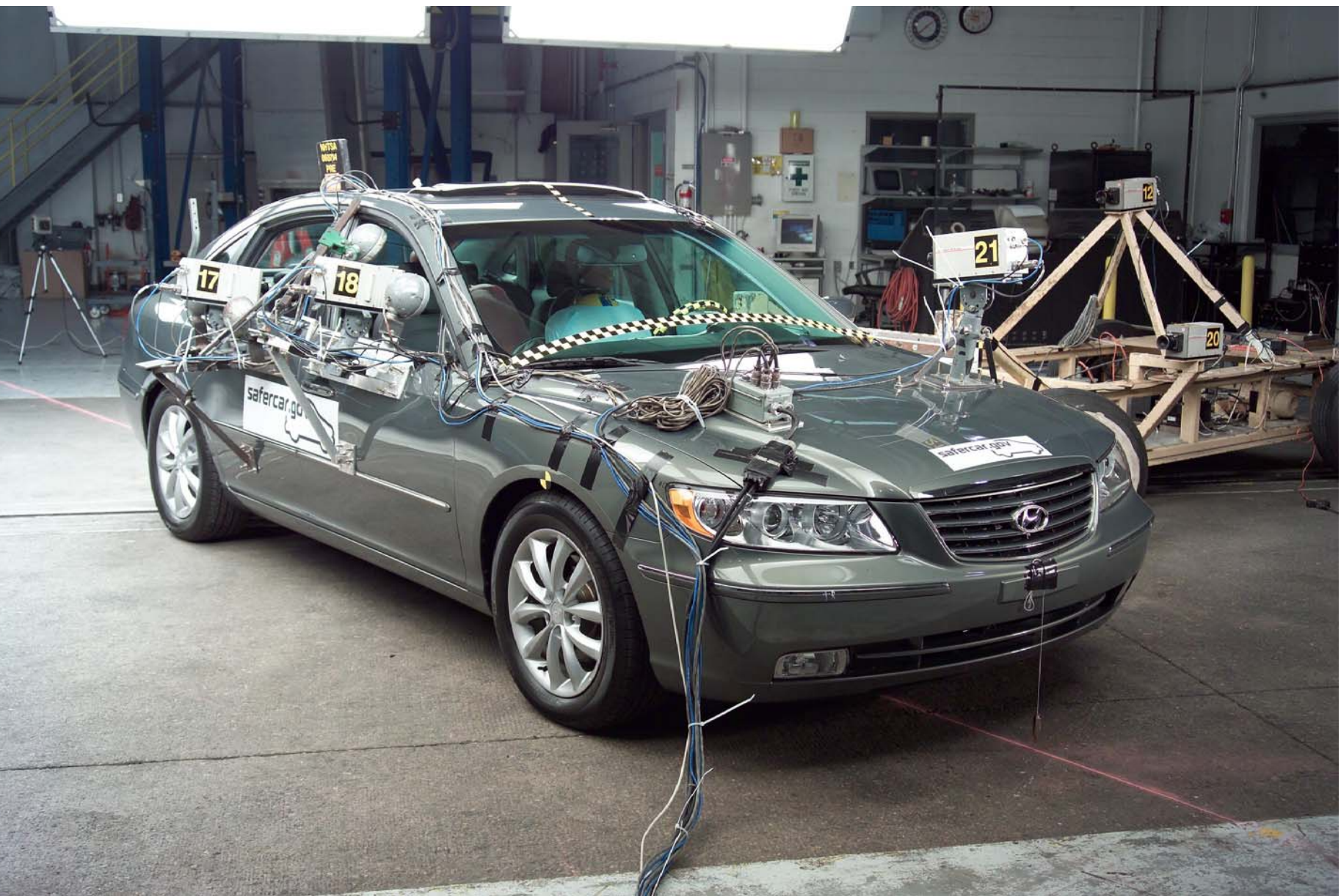
Figure A-15 Pre-Test Right Front View of Test Vehicle
