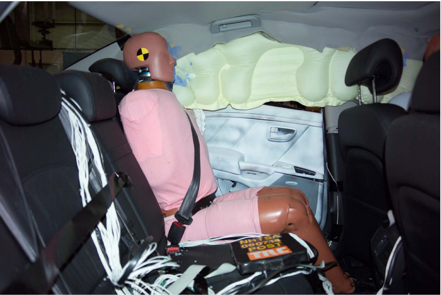
Figure A-46 Post-Test Right Occupant Compartment View of Rear SID HIII
