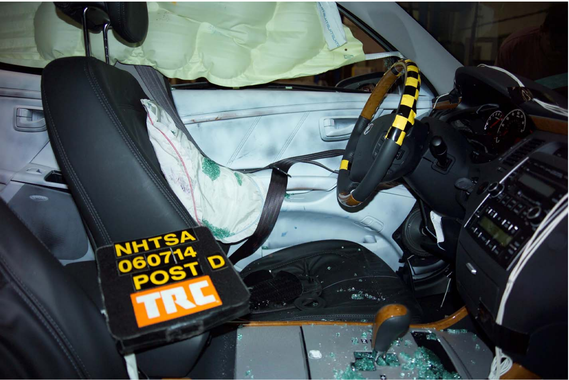
Figure A-58 Post-Test Interior of Front Door Showing SID HIII Impact Locations
