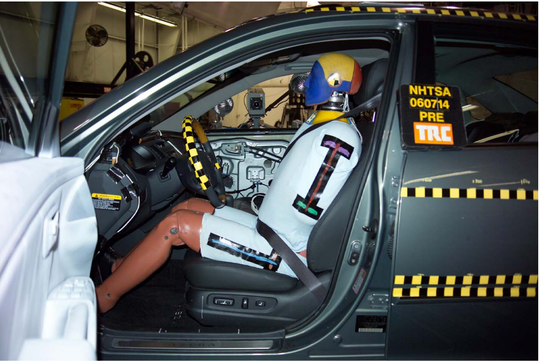
Figure A-49 Pre-Test Left View of Front SID Hill and Belt Position
