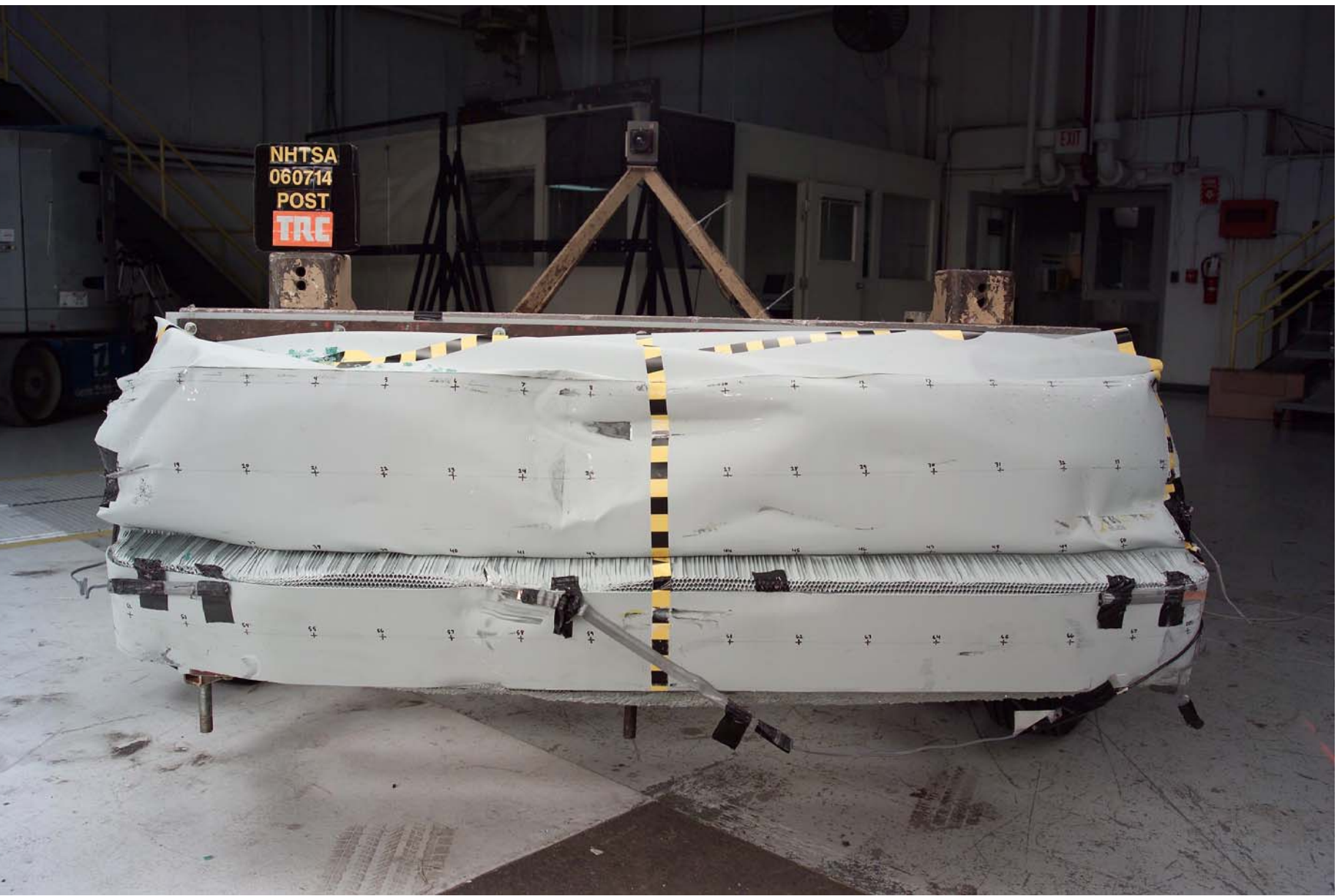
Figure A-26 Post-Test Front View of Impactor
