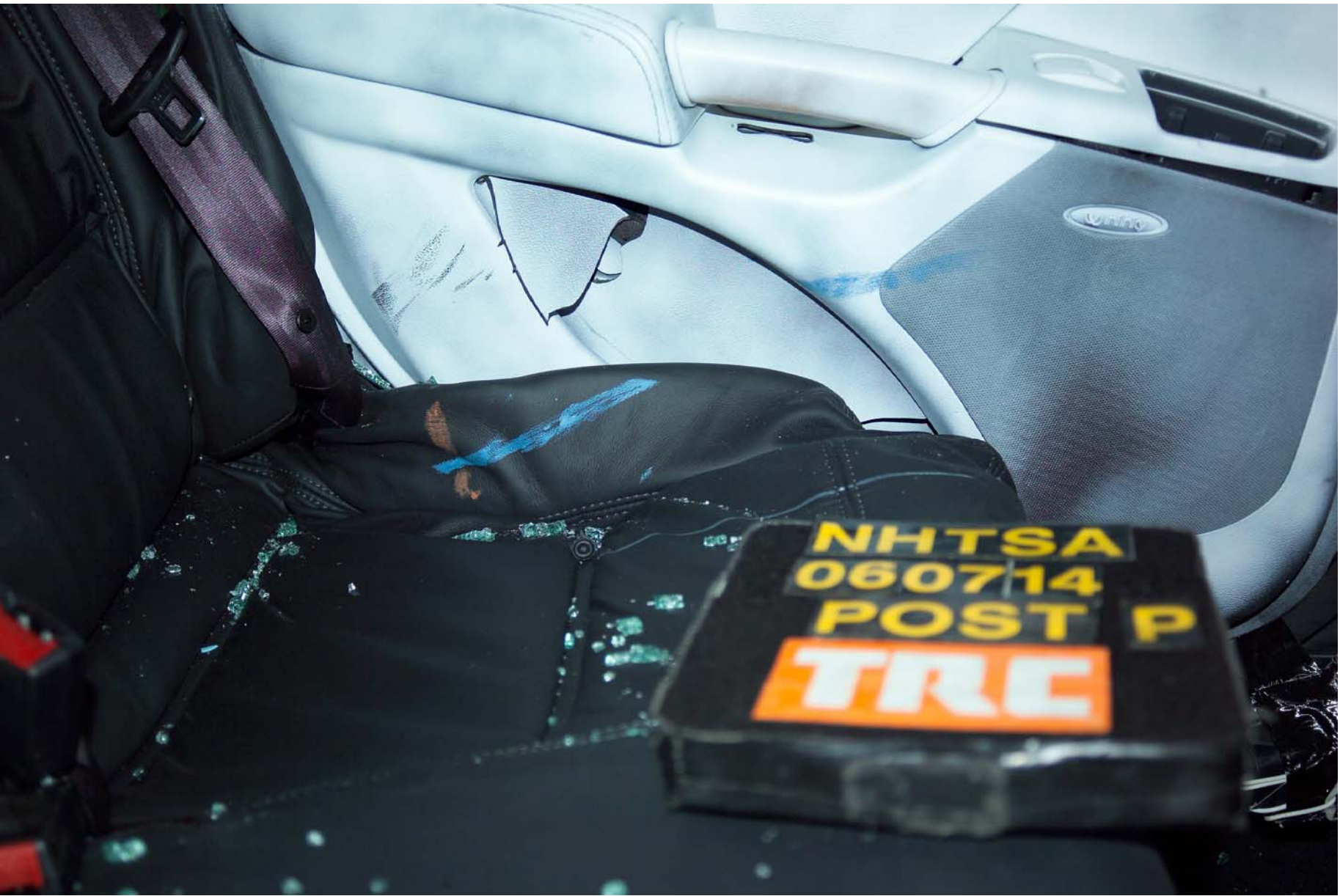
Figure A-66 Post-Test Rear SID HIII Contact - View 3
