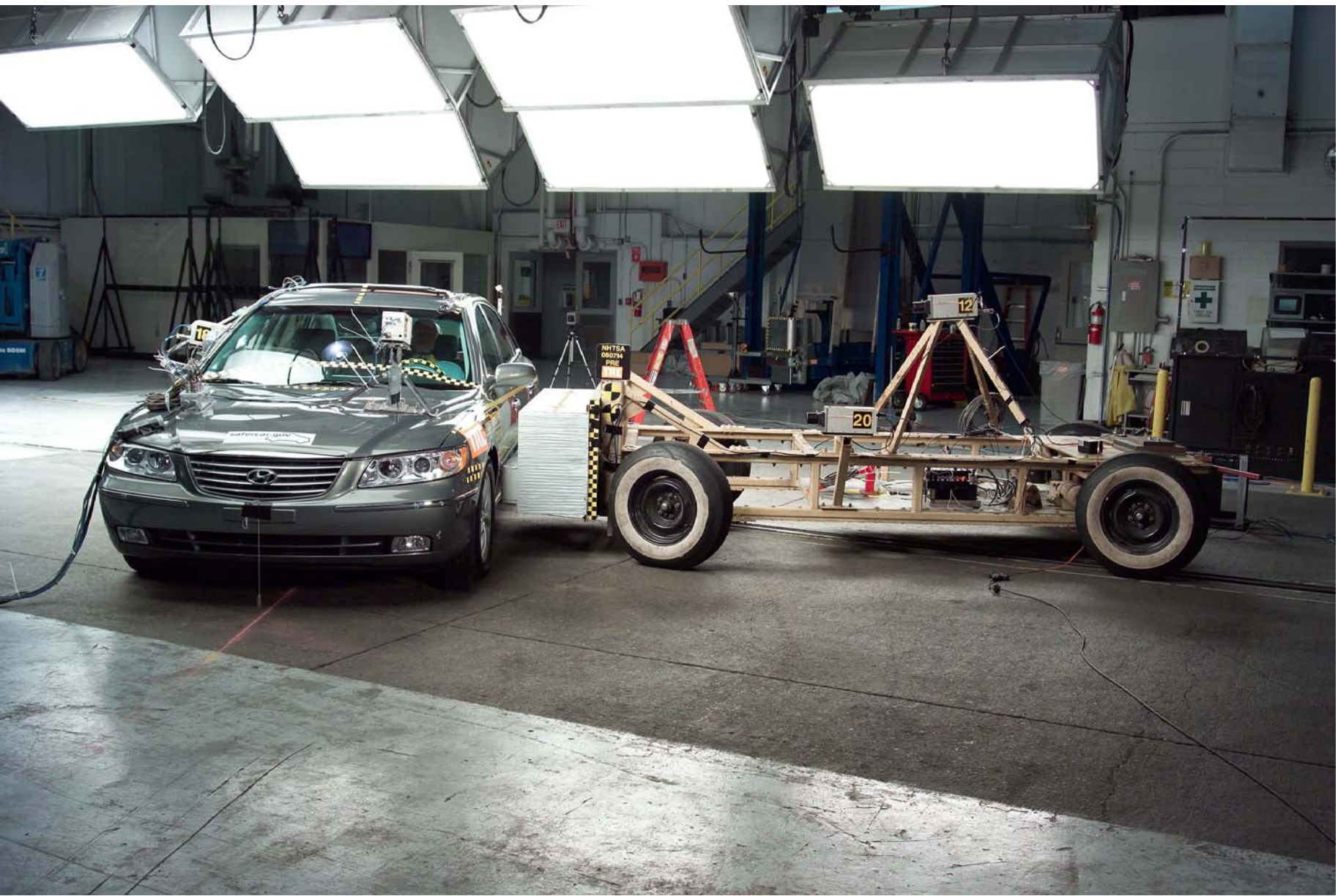
Figure A-67 Pre-Test Left Side View of MDB With Impactor Face in Position
