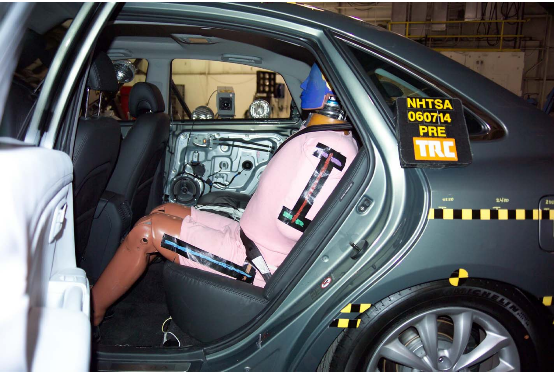
Figure A-54 Pre-Test Left of Rear SID HIII and Belt Position
