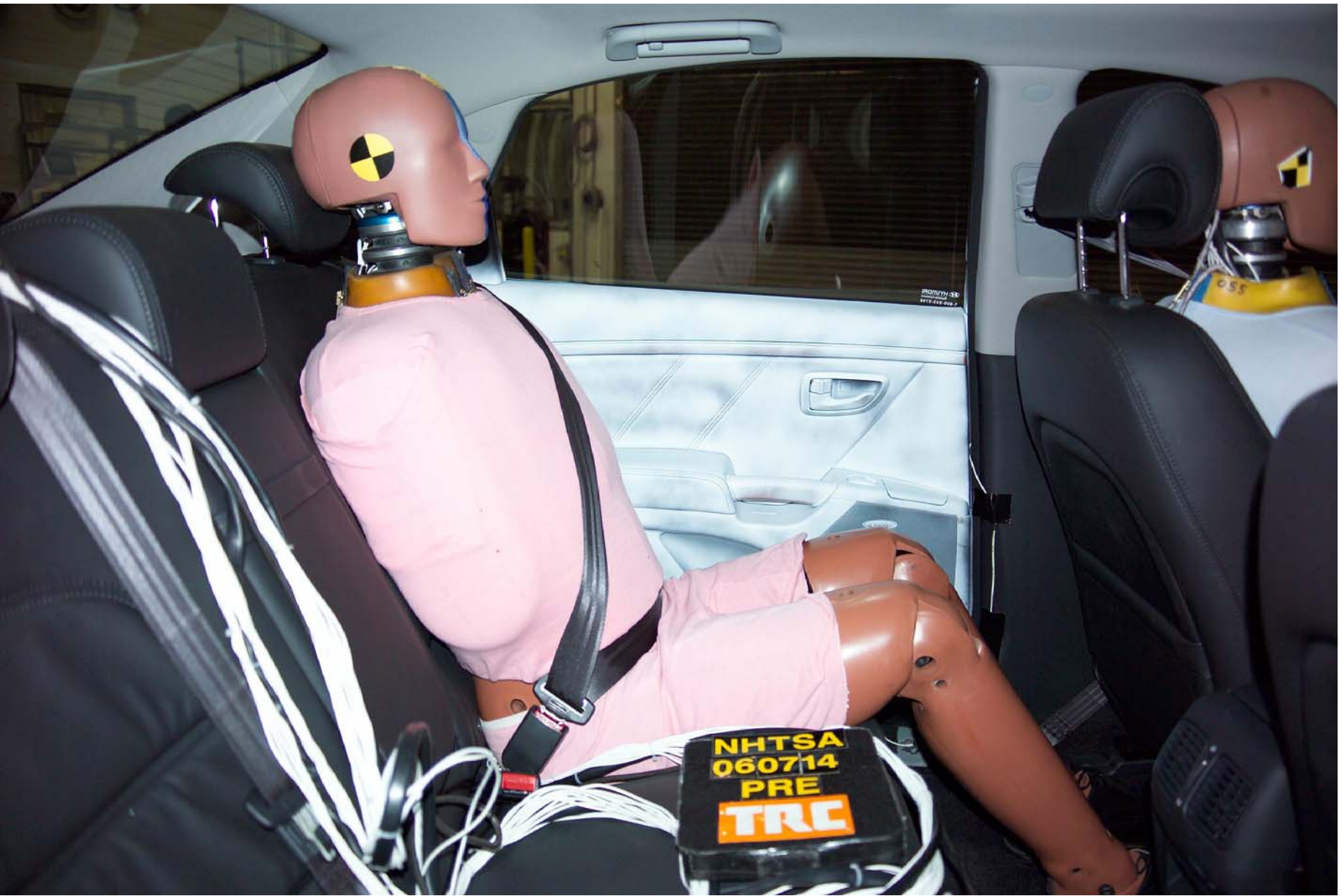
Figure A-45 Pre-Test Right Occupant Compartment View of Rear SID HIII
