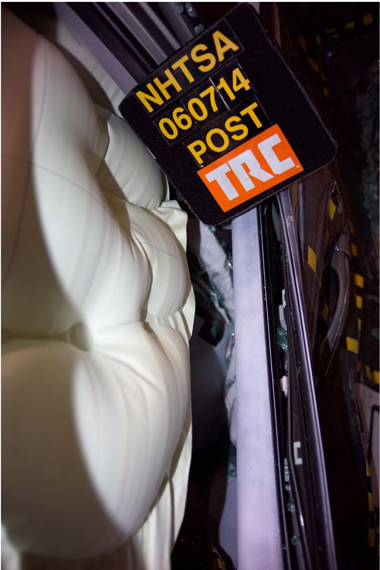
Figure A-51 Post-Test Left View of Front SID HIII and Door Clearance
