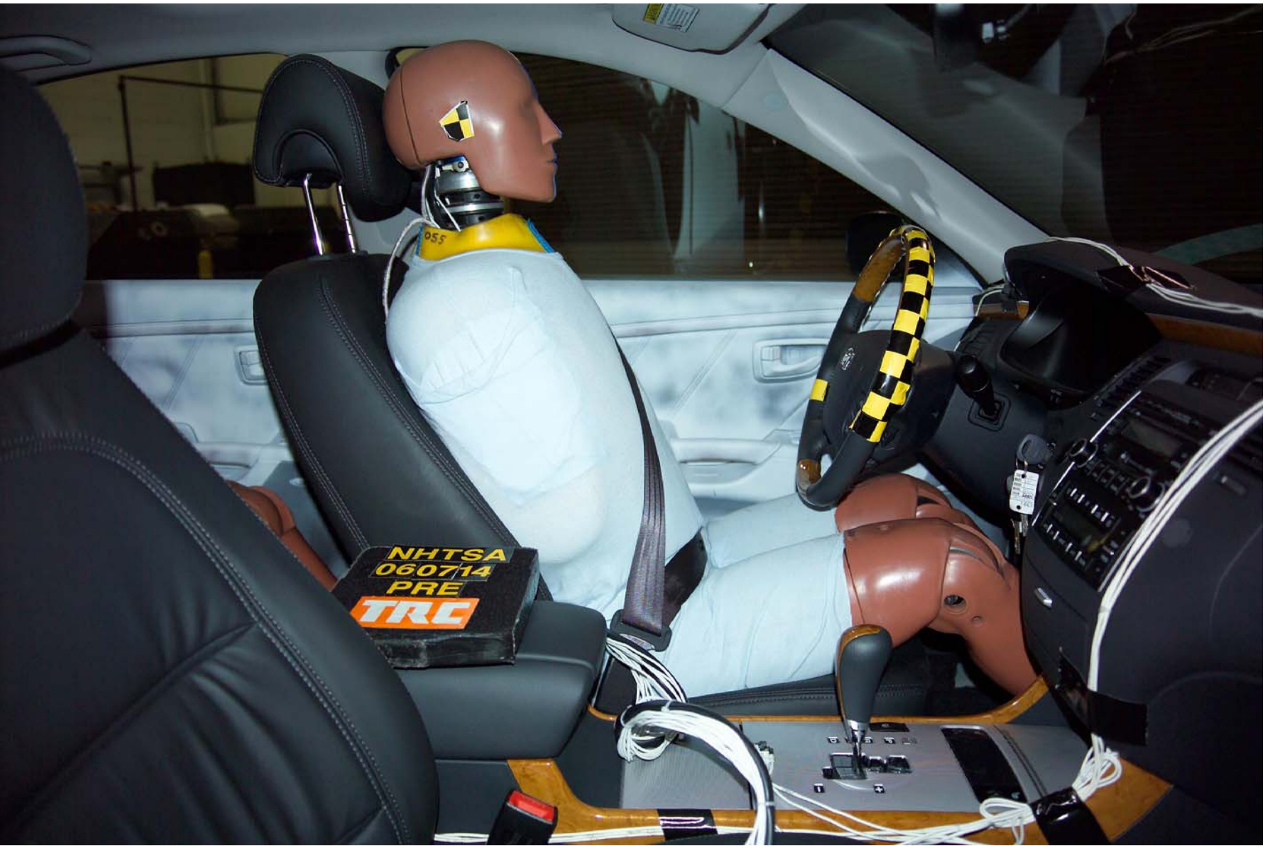
Figure A-43 Pre-Test Right Occupant Compartment View of Front SID HIII
