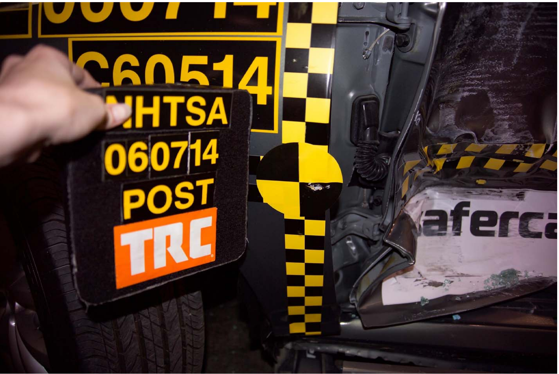
Figure A-70 Post-Test Primary Impact Point View
