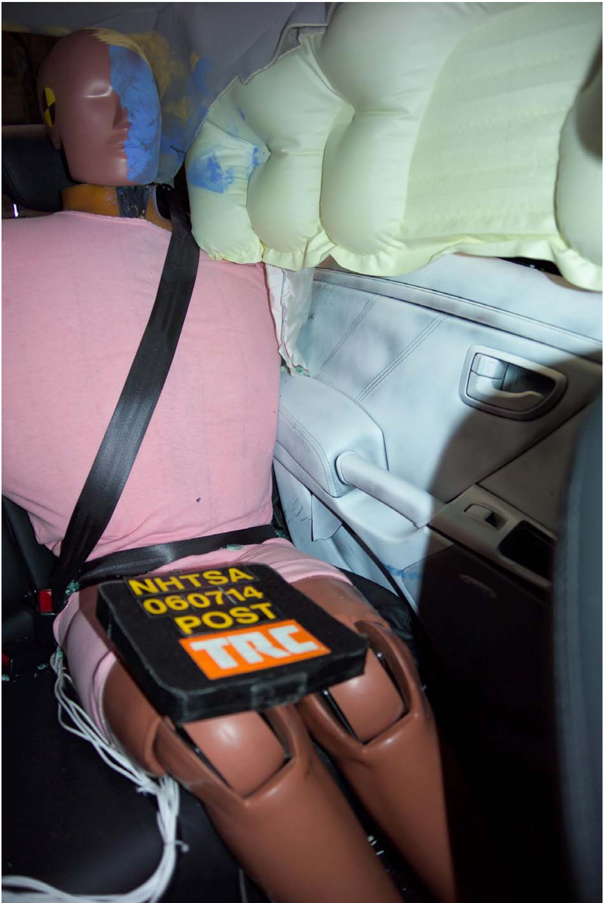
Figure A-56 Post-Test Left View of Rear SID HIII and Door Clearance
