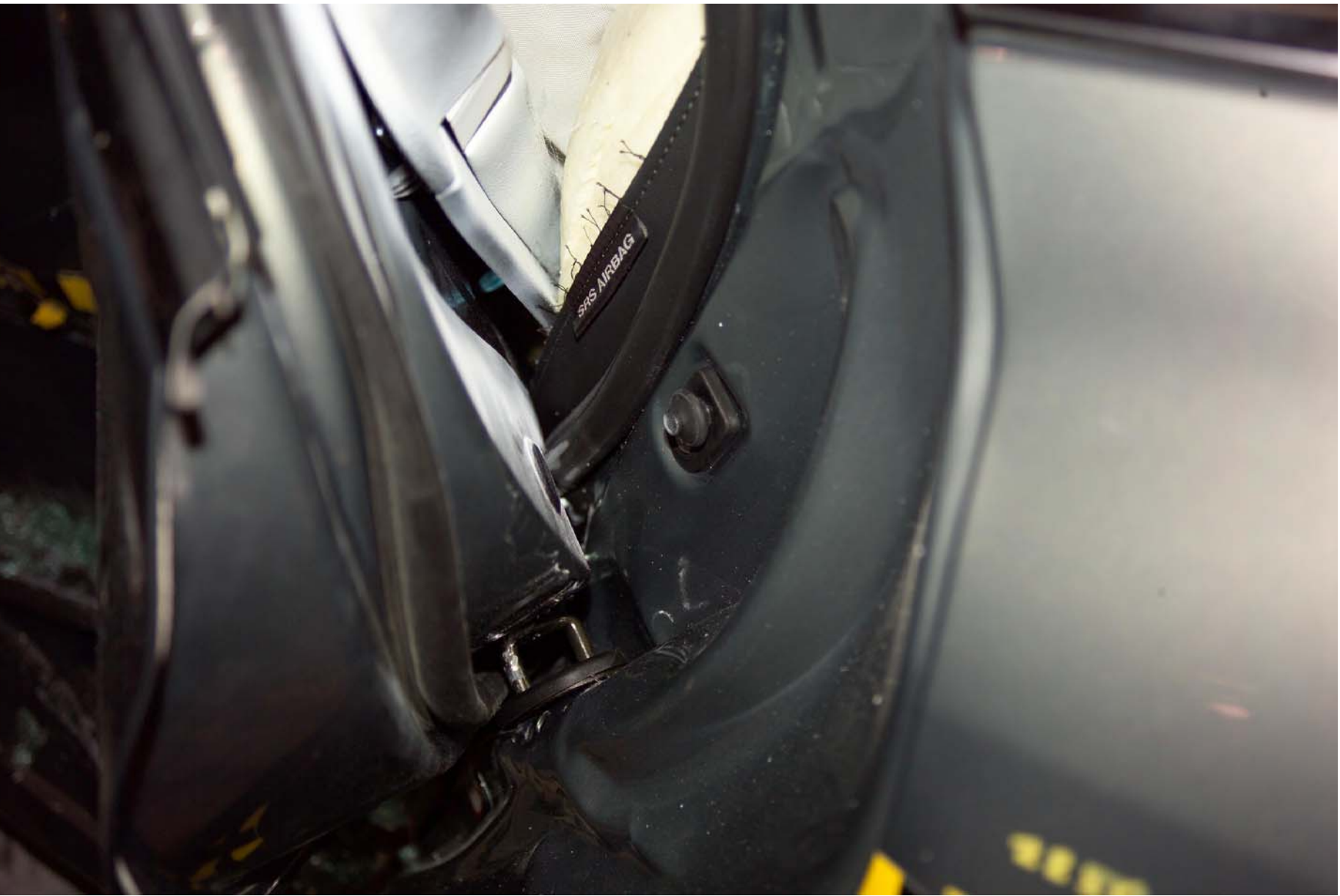
Figure A-88 Post-Test Left Rear Door Latch - View 2
