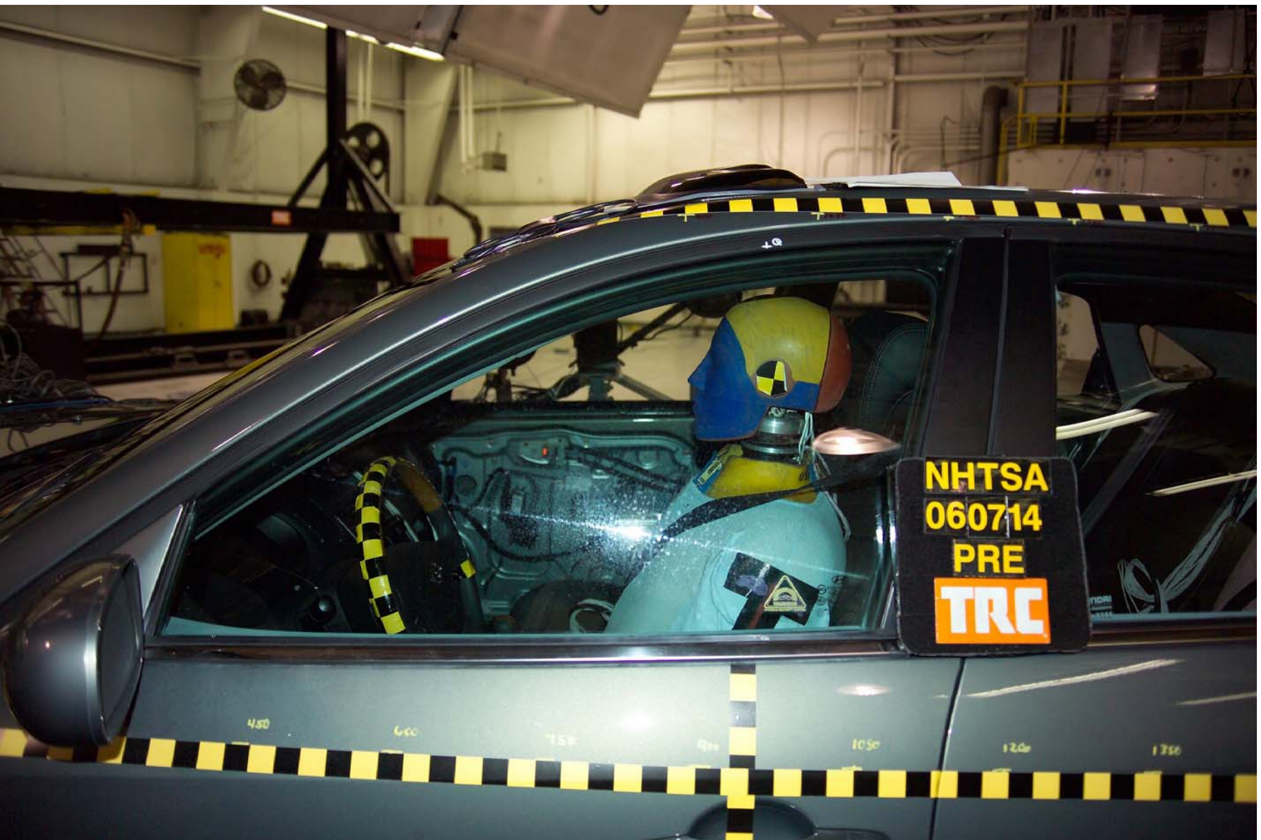
Figure A-47 Pre-Test Left View of Front SID HIII
