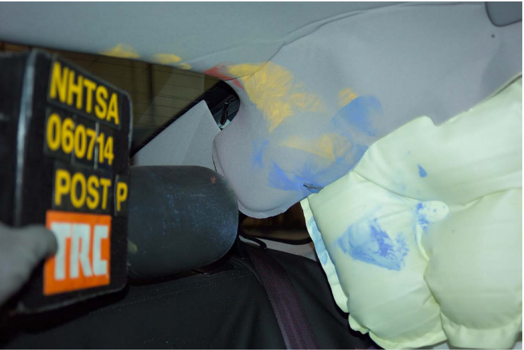
Figure A-64 Post-Test Rear SID HIII Contact - View 1
