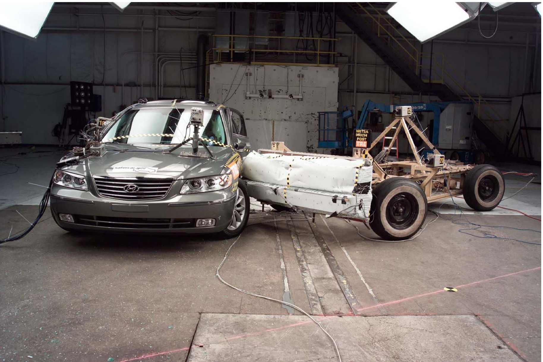
Figure A-68 Post-Test Left Side View of MDB With Impactor Face in Position
