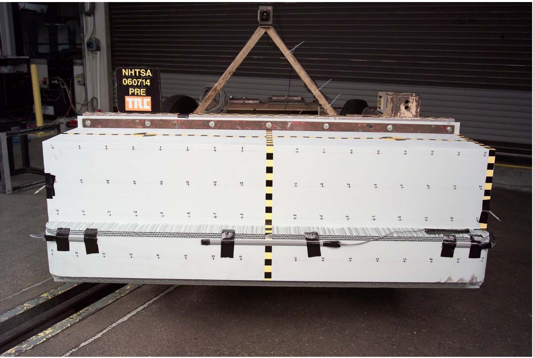
Figure A-39 Pre-Test View of MDB Showing Contact Switches in Place
