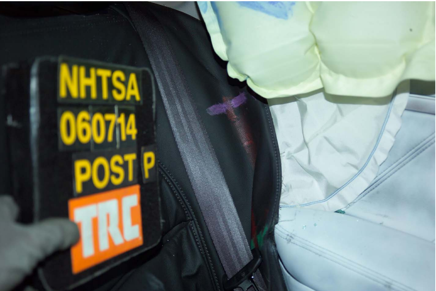
Figure A-65 Post-Test Rear SID HIII Contact - View 2
