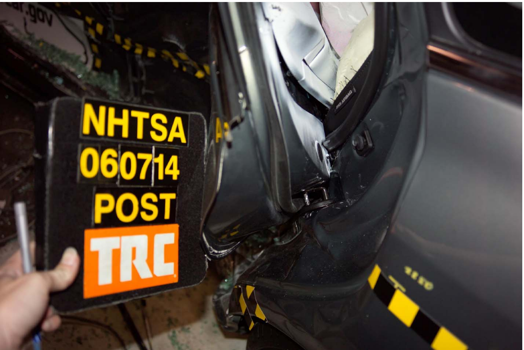
Figure A-87 Post-Test Left Rear Door Latch - View 1
