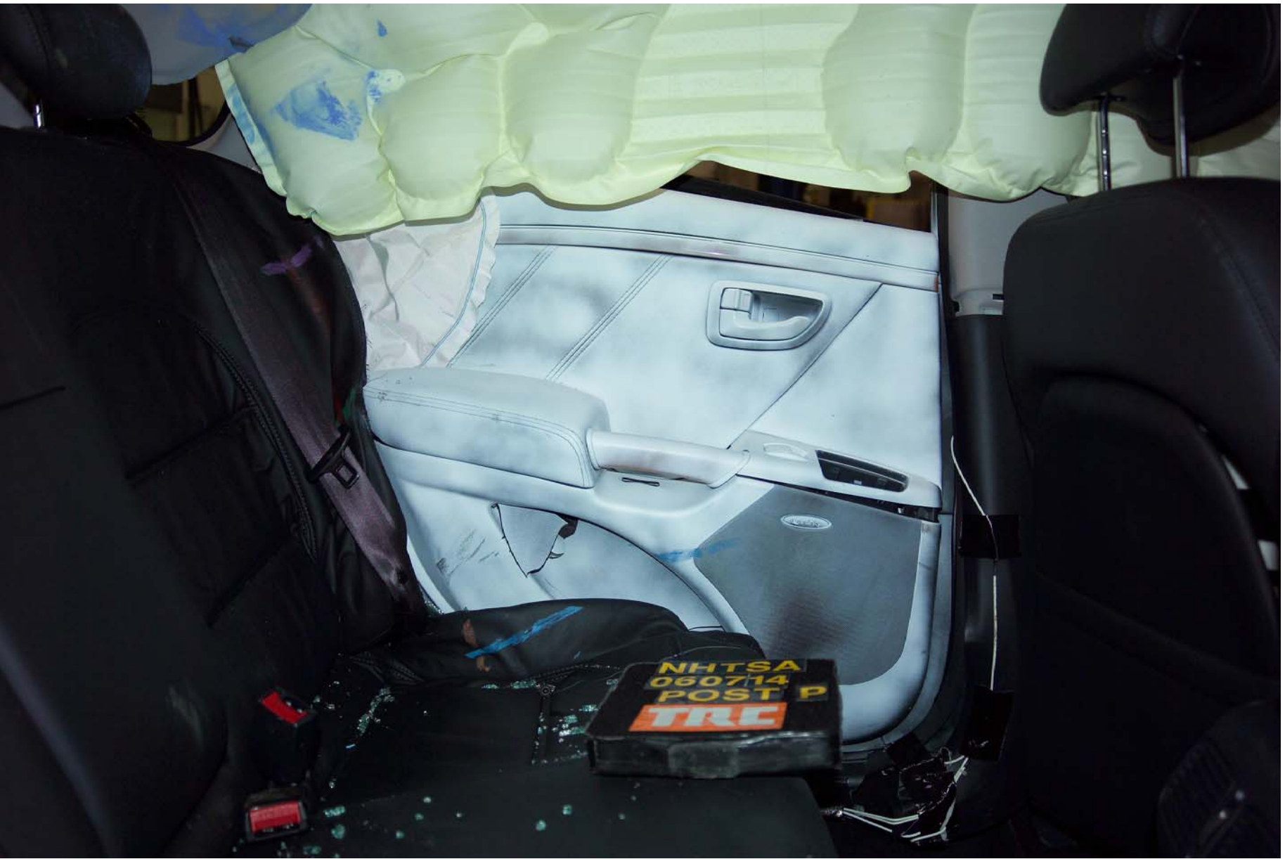
Figure A-63 Post-Test Interior of Rear Panel Showing SID HIII Impact Locations
