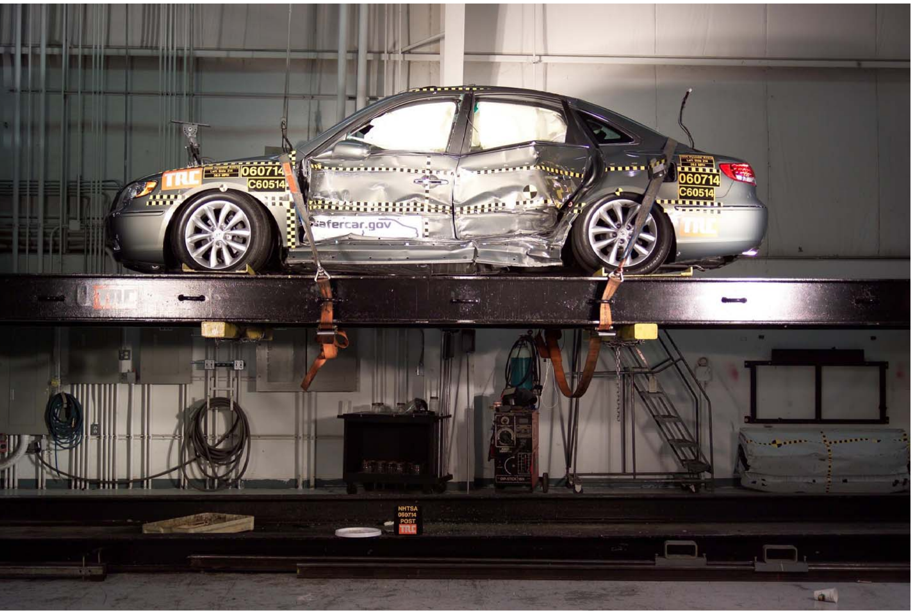
Figure A-86 FMVSS 301 Rollover View at 360°
