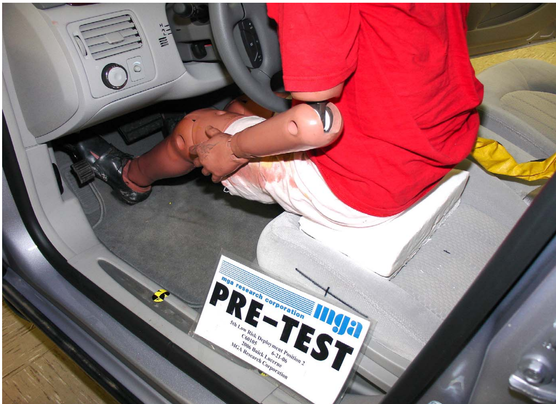
Pre-Test 5th Fem. P2 Driver Dummy Left Side Mid Position View
