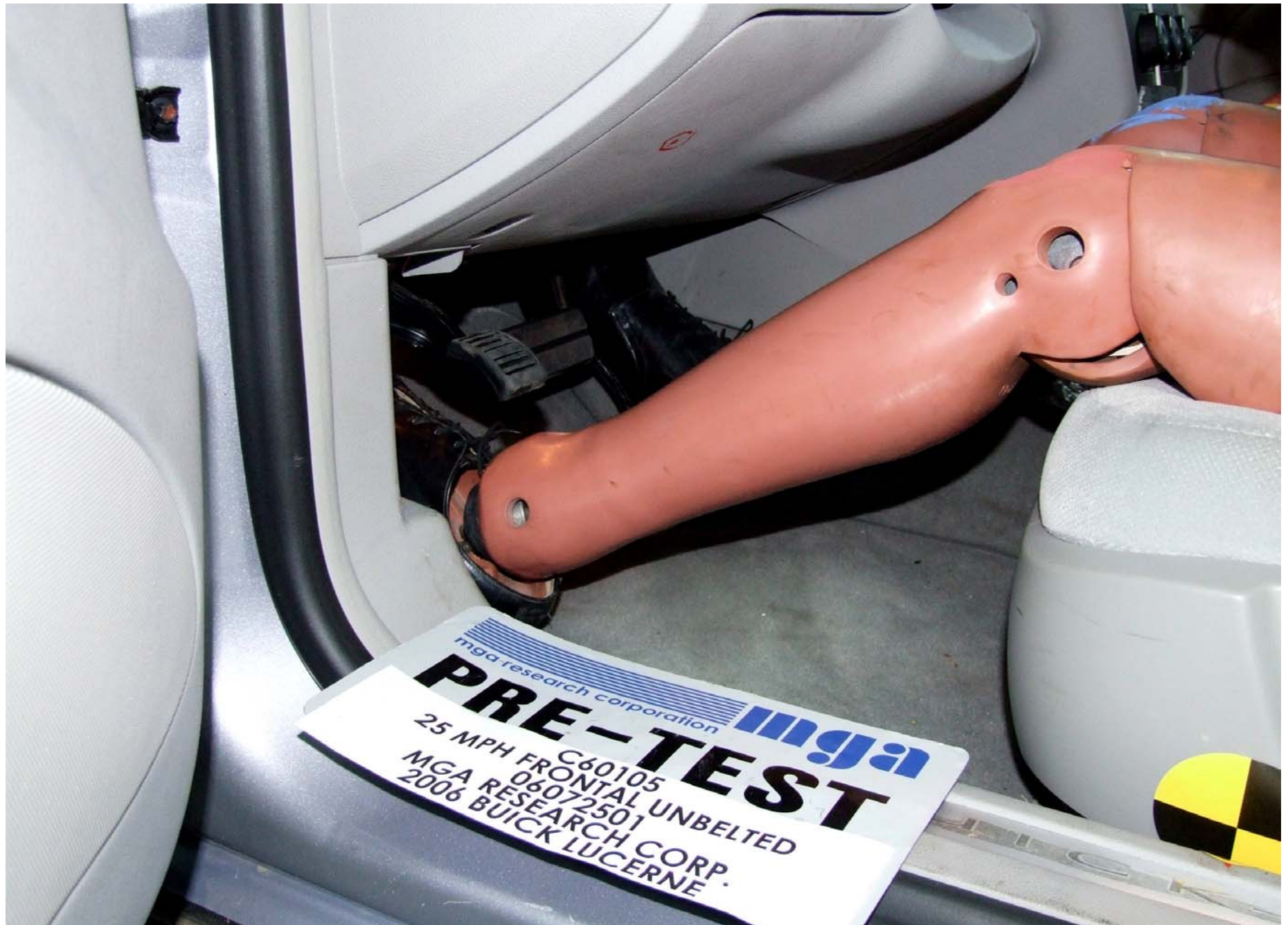
Pre-Test Driver Dummy Feet Position
