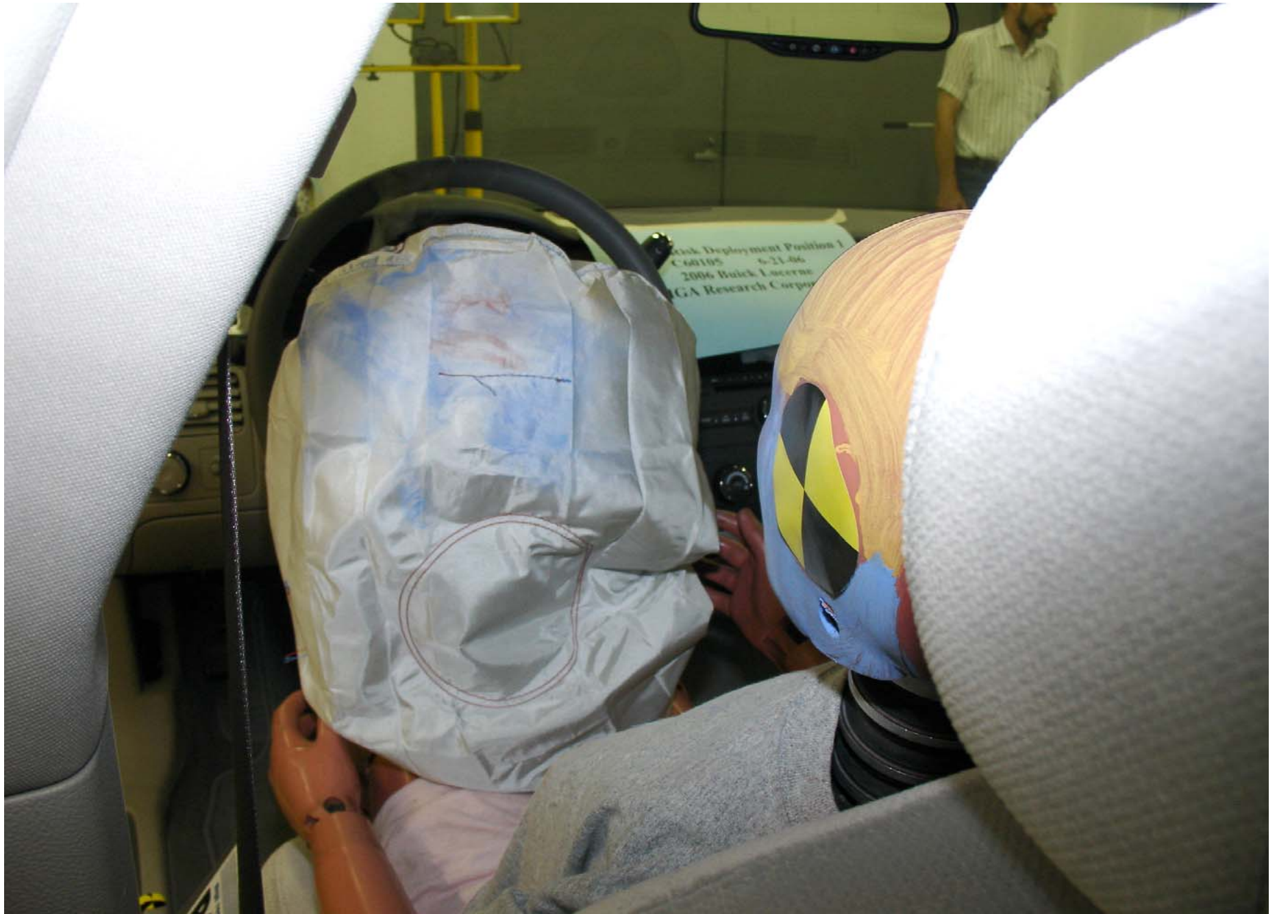
Post-Test 5th Fem. P1 Driver Dummy Airbag Left View
