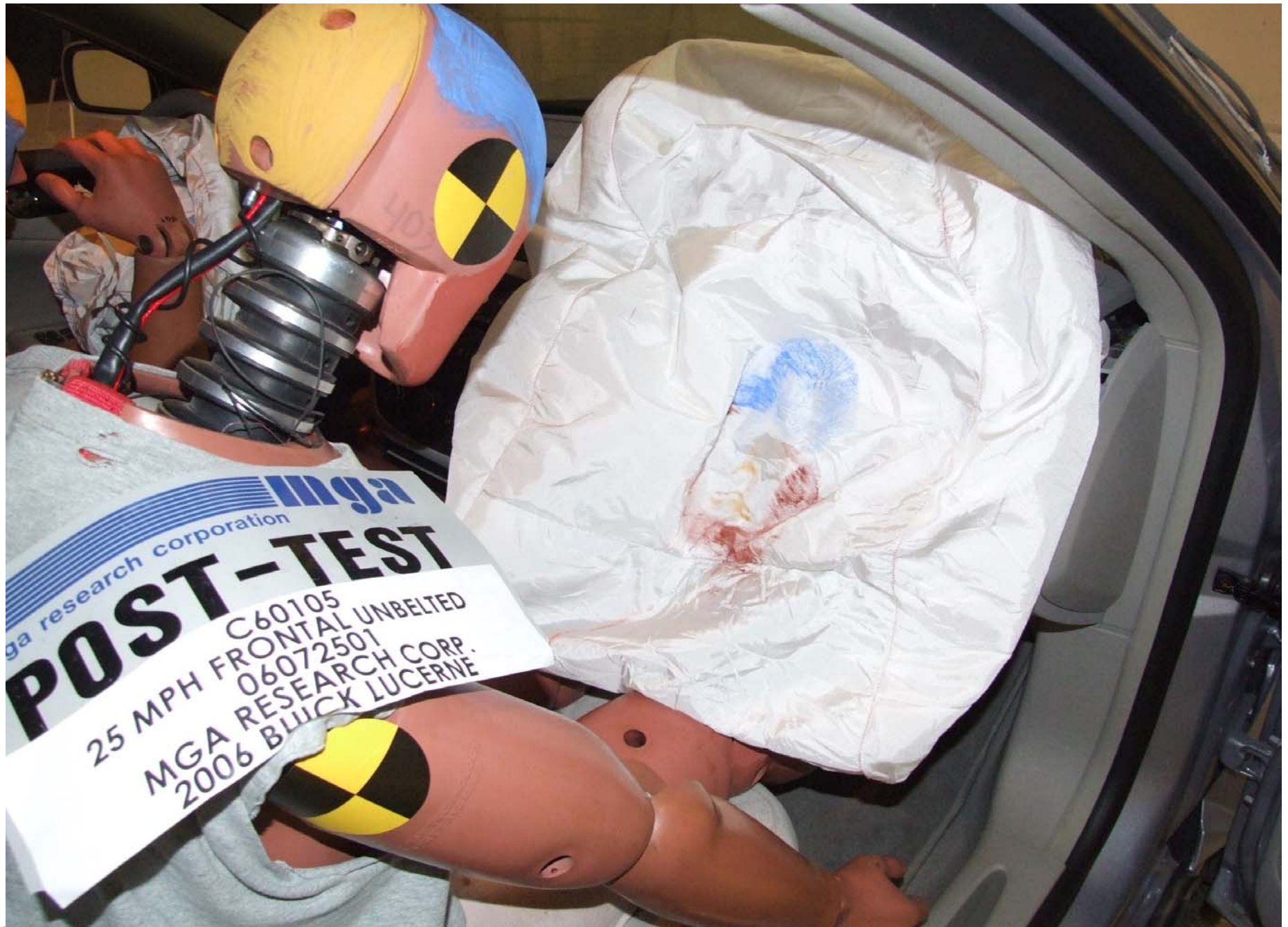
Post-Test Passenger Dummy Airbag Contact
