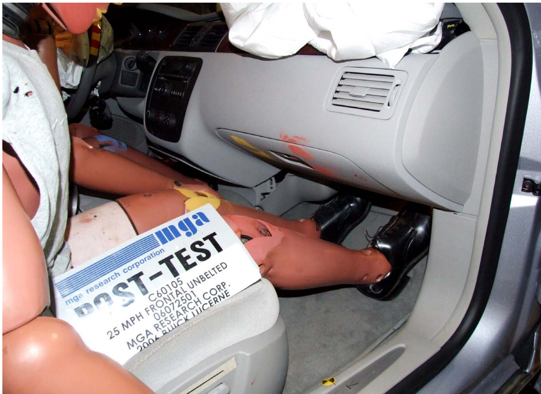
Post-Test Passenger Dummy Feet Position
