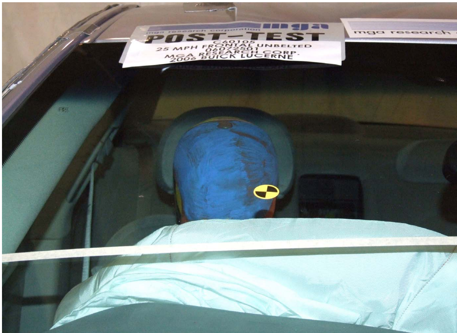
Post-Test Passenger Dummy Front View (head position)
