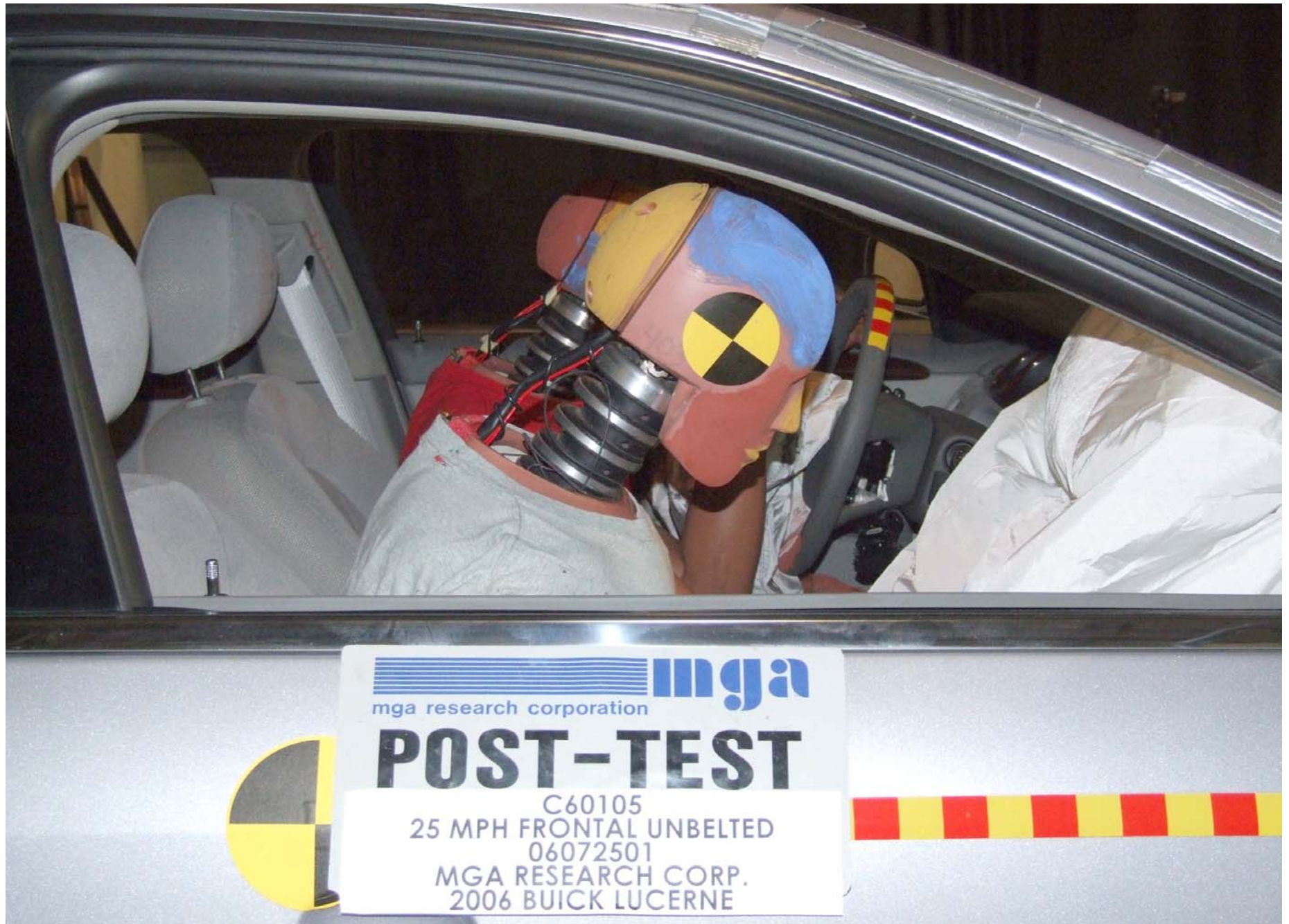
Post-Test Passenger Dummy Position Right Side View
