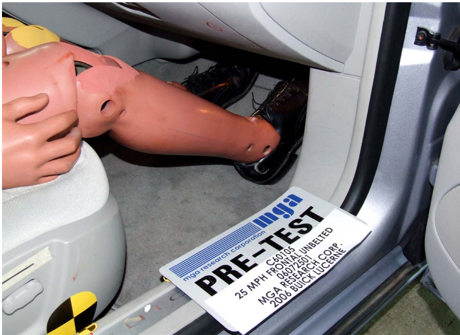
Pre-Test Passenger Dummy Feet Position
