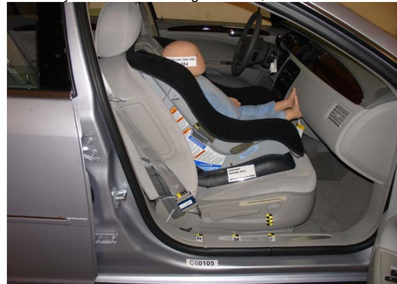
Century Encore Fwd Facing Unbelted, Forward Seat Track
