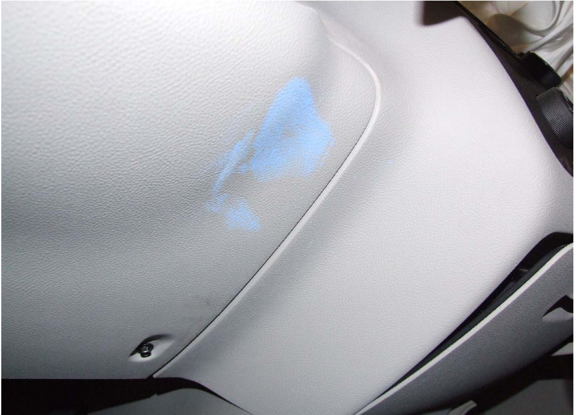
Post-Test Driver Dummy Knee Contact (right side view)
