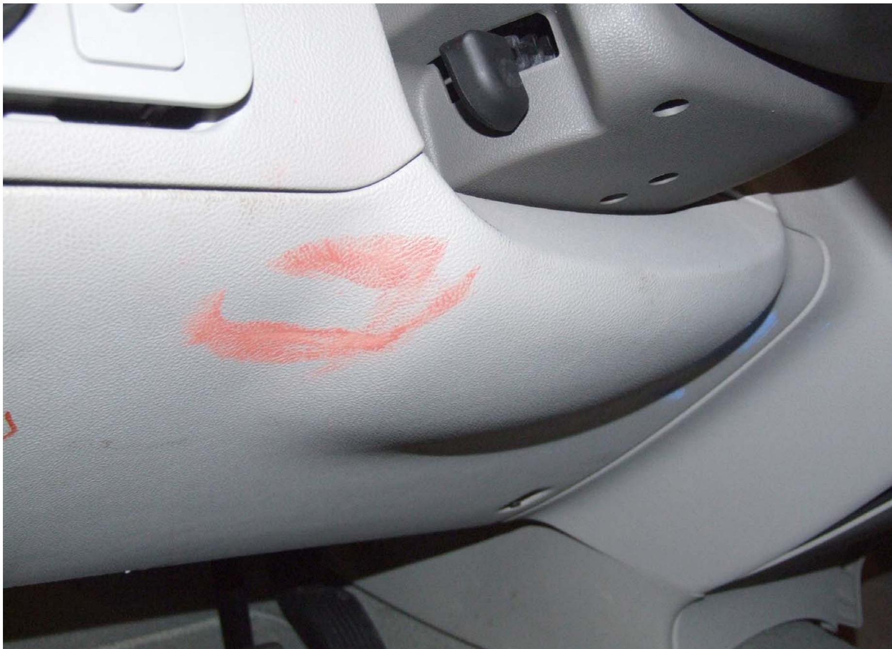
Post-Test Driver Dummy Knee Contact (left side view)
