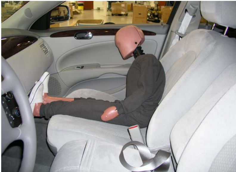
6-Year-Old Unbelted, Forward Seat Track, Position 4, View 2
