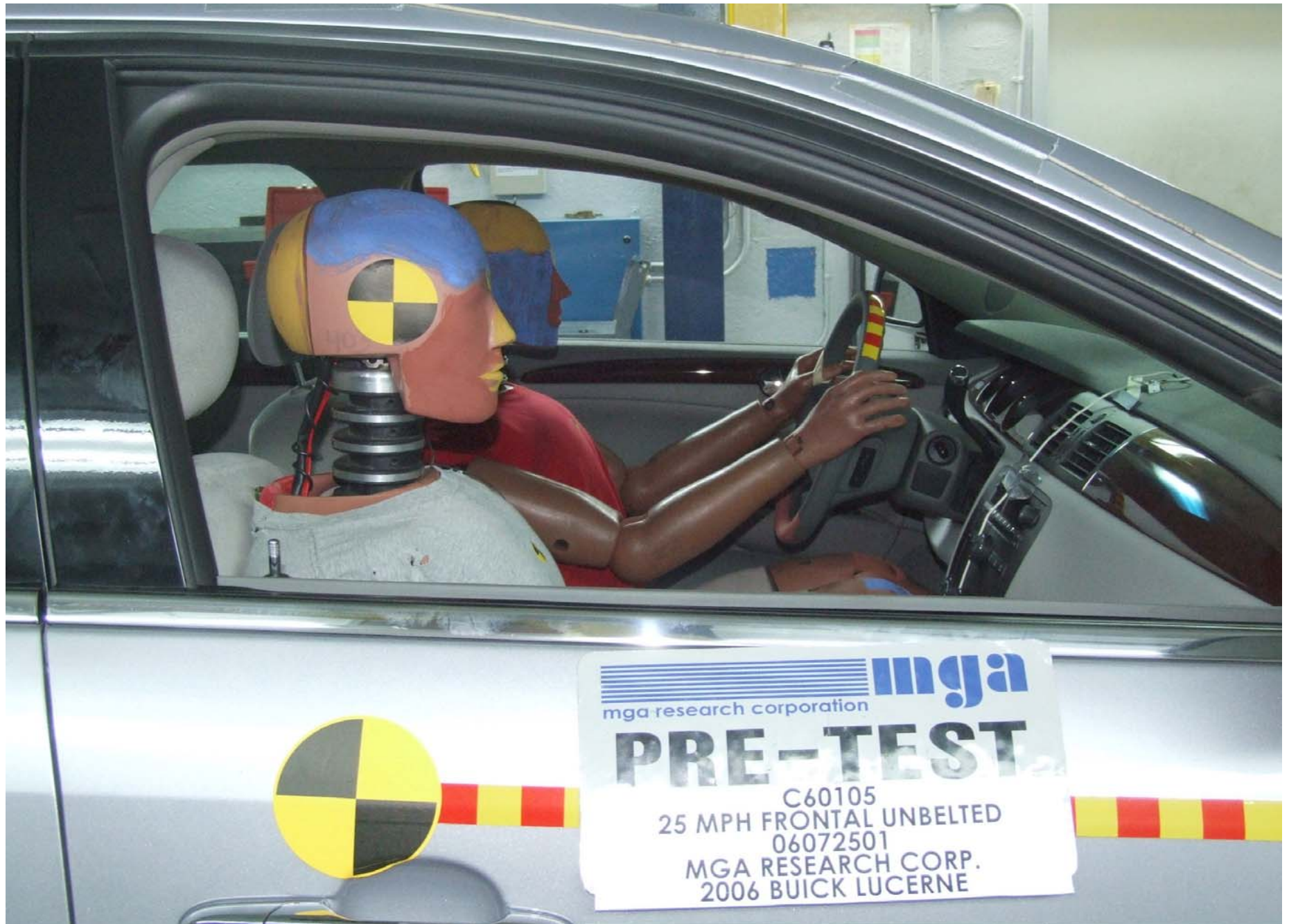
Pre-Test Passenger Dummy Position Right Side View
