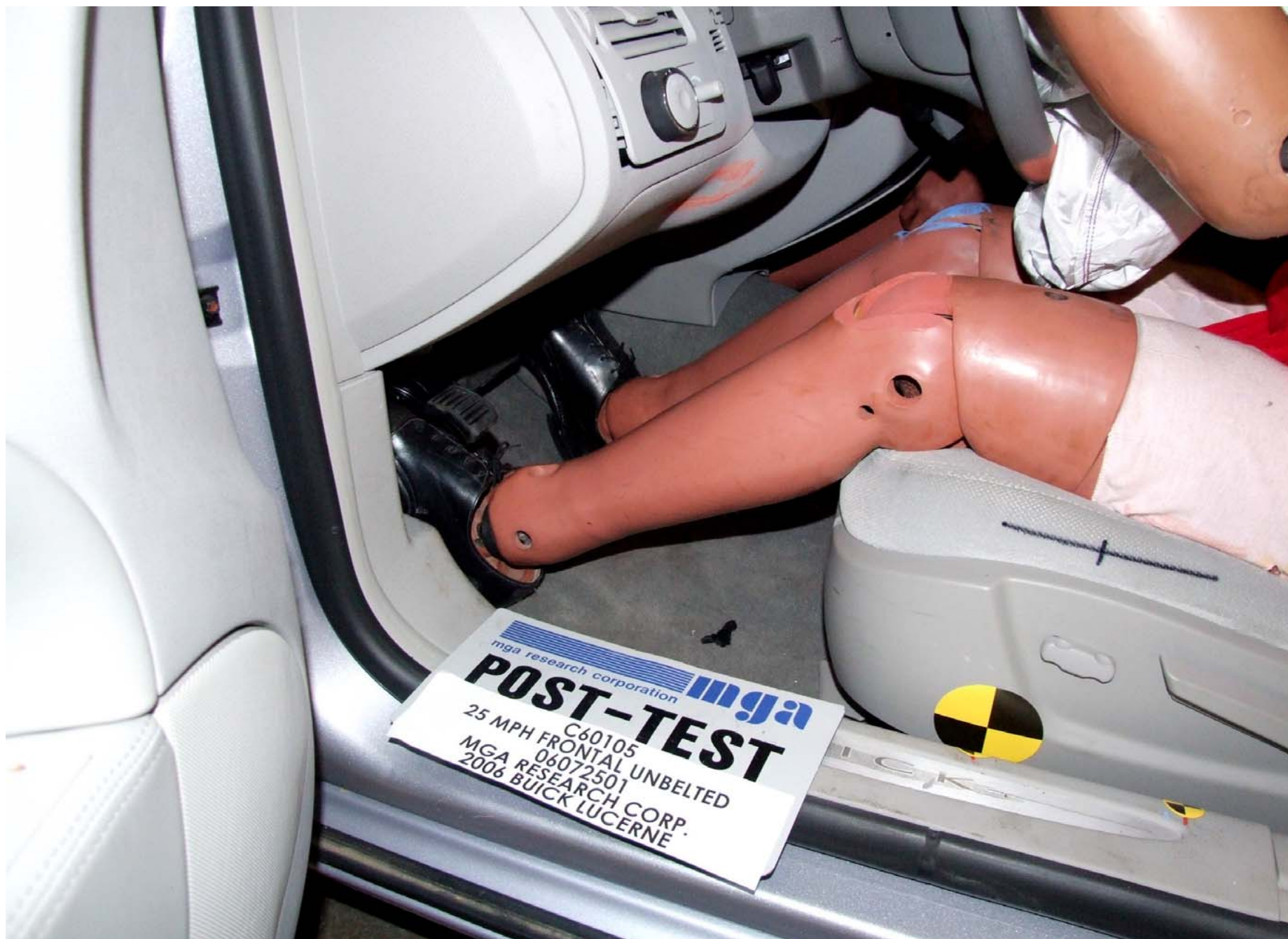
Post-Test Driver Dummy Feet Position
