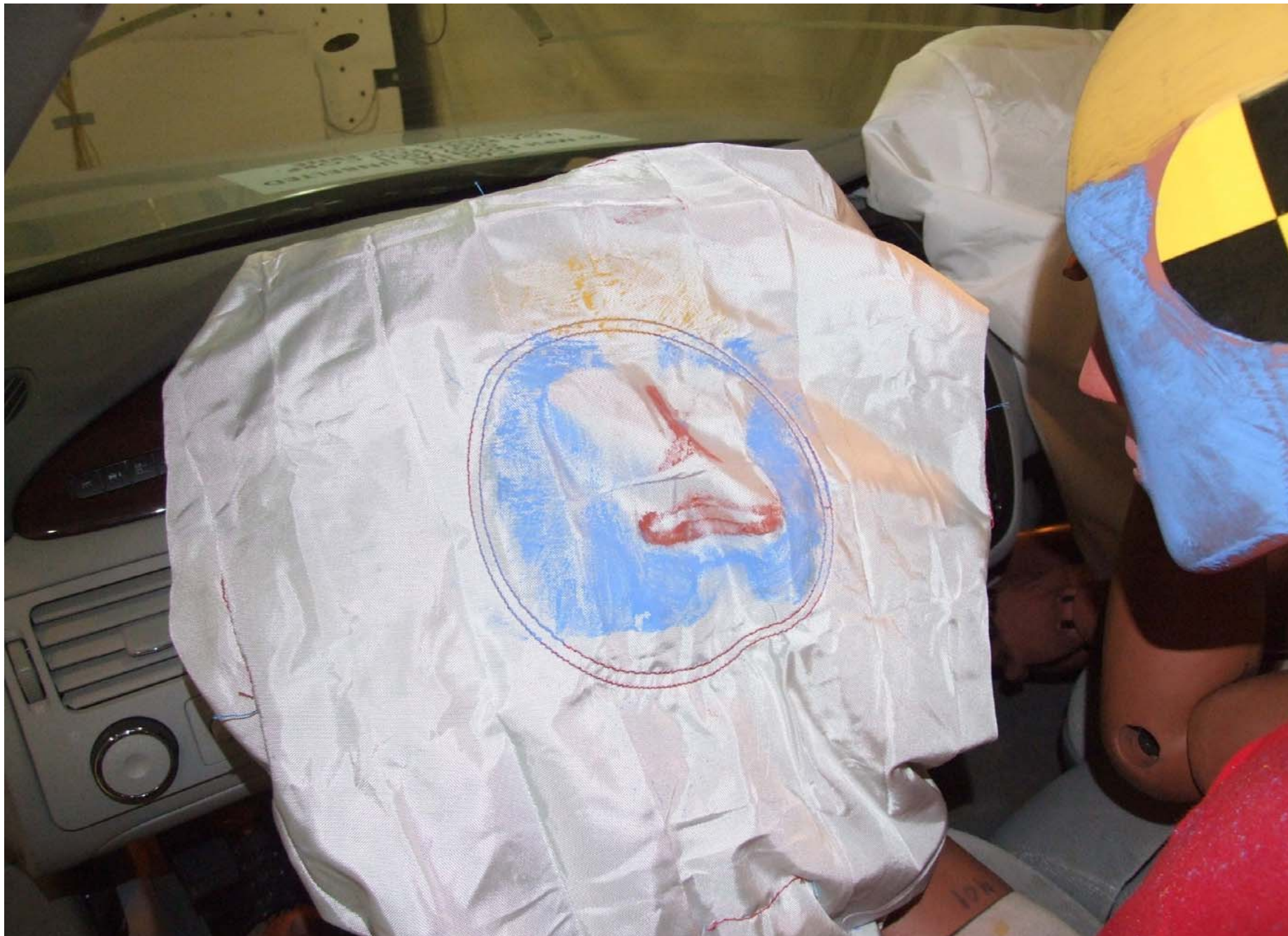
Post-Test Driver Dummy Airbag Contact
