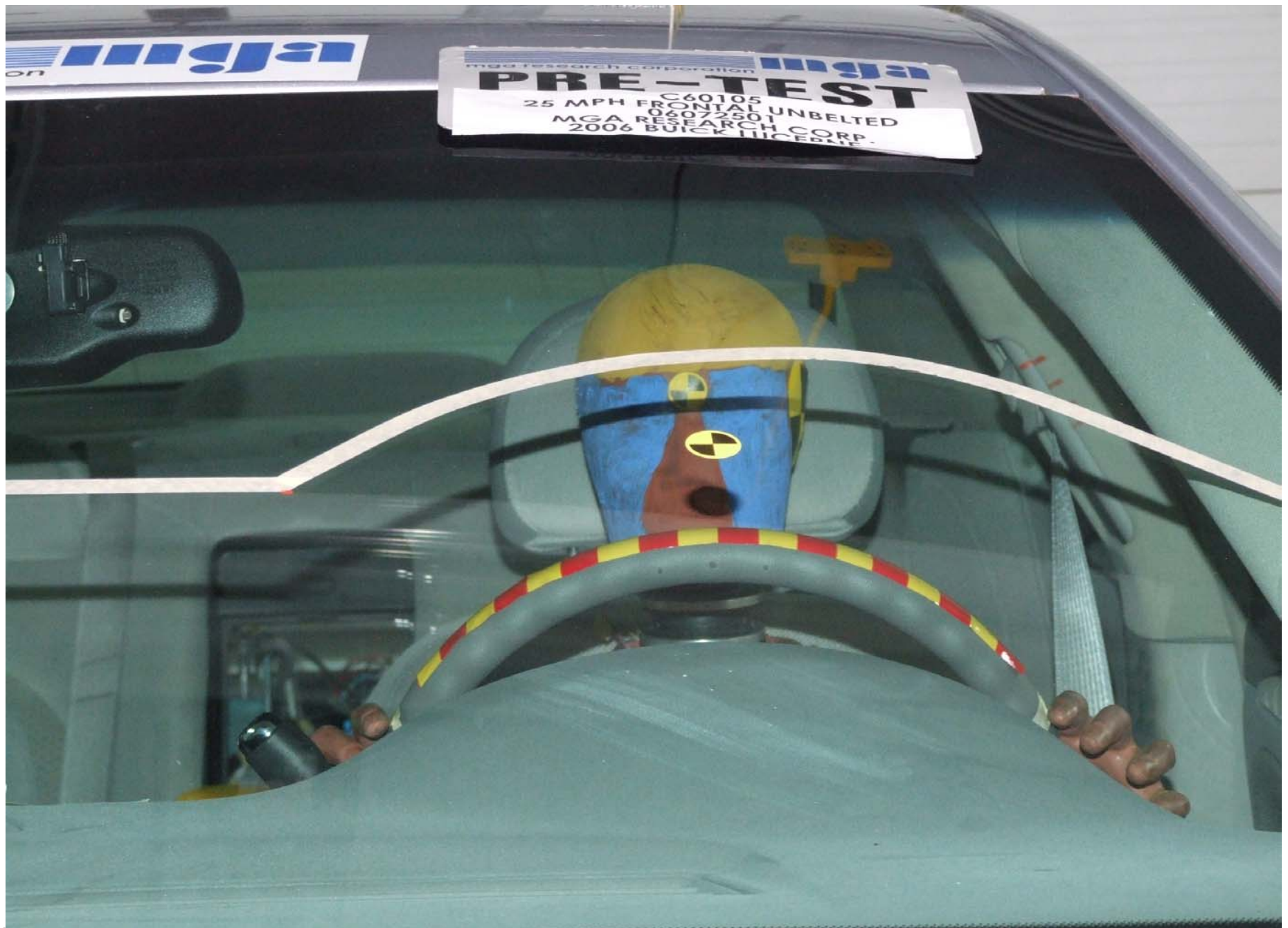
Pre-Test Driver Dummy Front View (head position)
