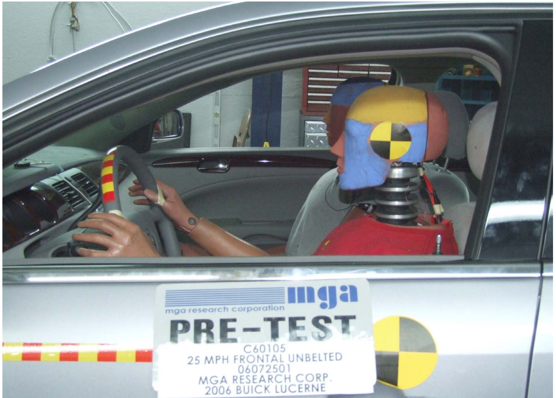
Pre-Test Driver Dummy Position Left Side View
