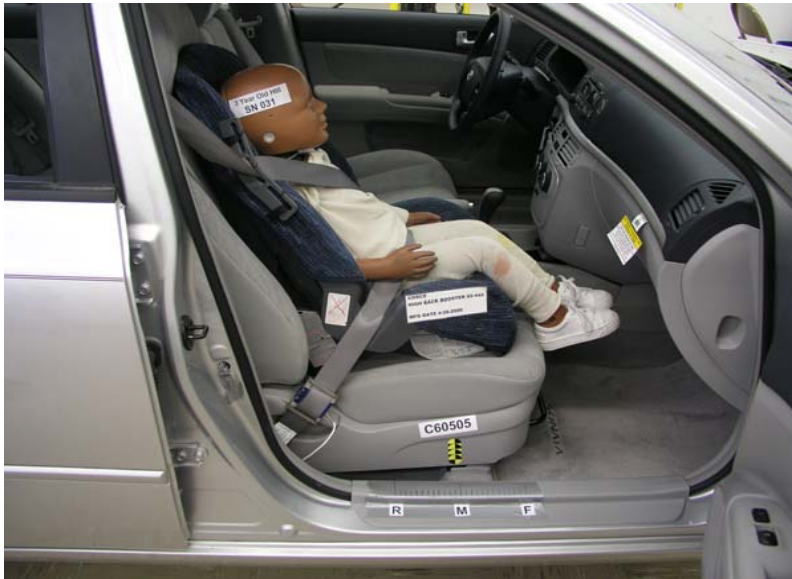
3-Year-Old Cosco High Back Booster With Belt, Middle Seat Track
