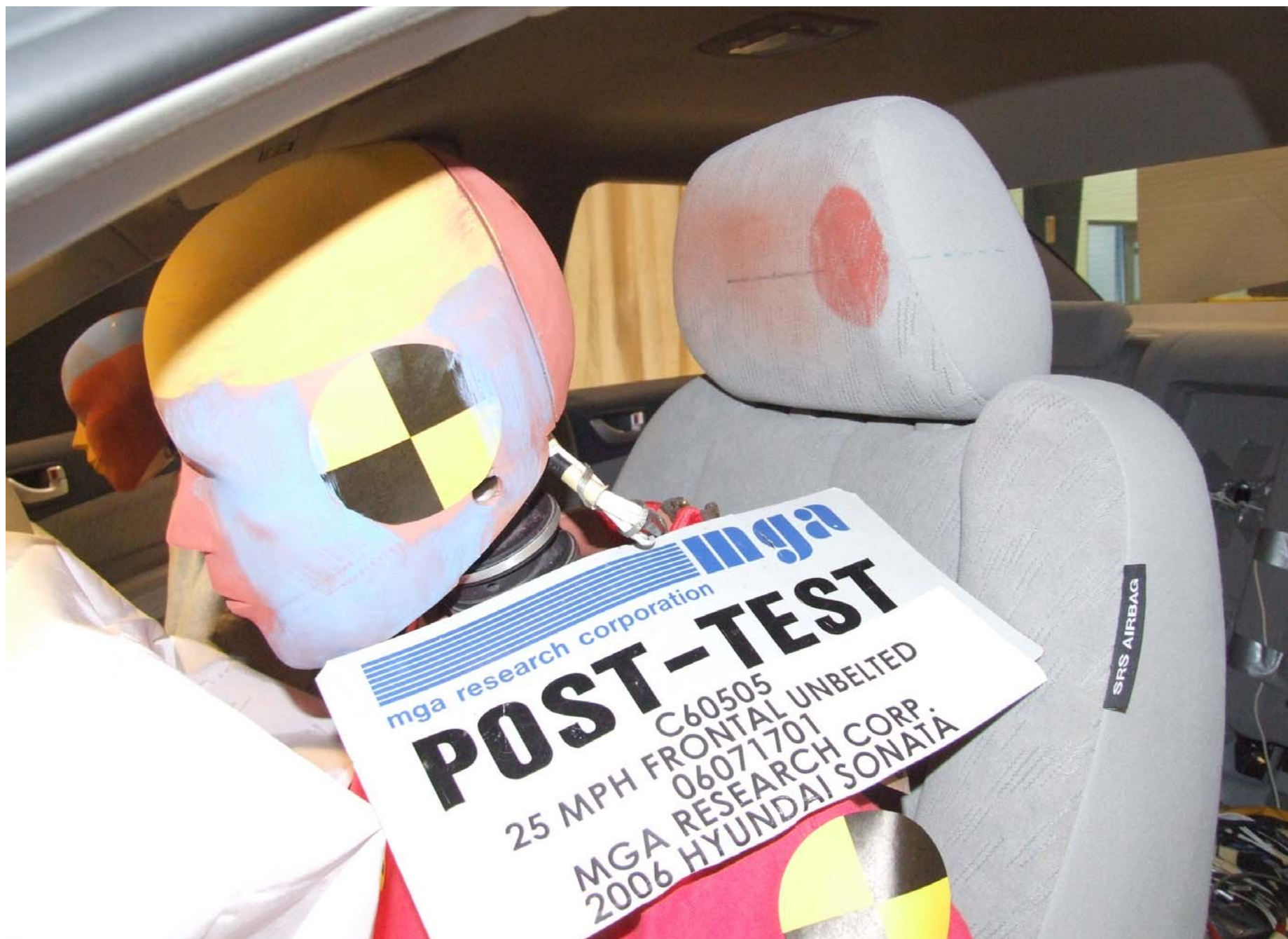
Post-Test Driver Dummy Head Contact (head rest)
