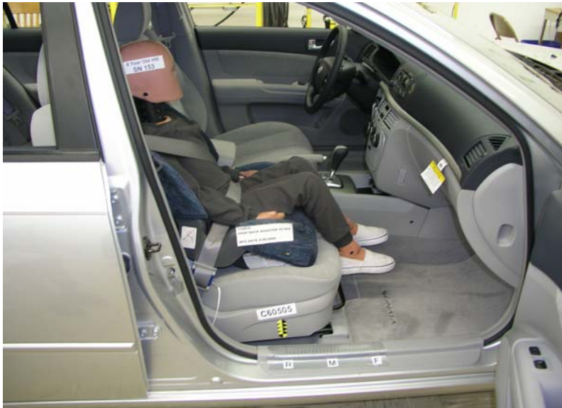
6-Year-Old Cosco High Back Booster With Belt, Rearward Seat Track
