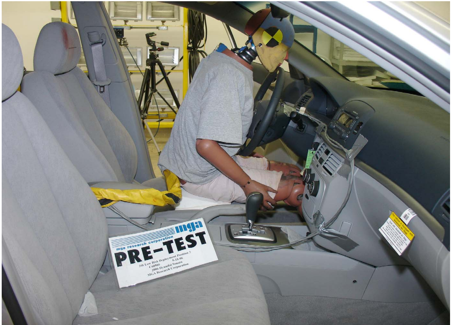
Pre-Test 5th Fem. P2 Driver Dummy Right Side View (Door Open) Trial 2
