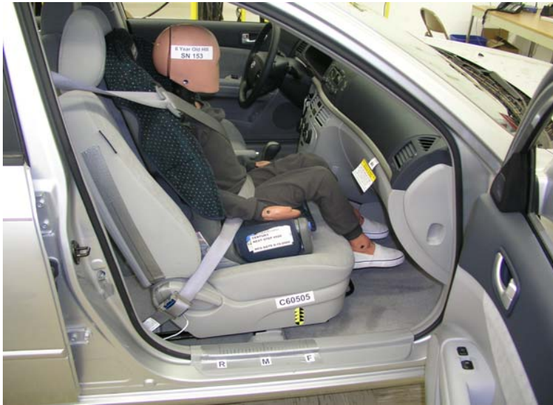
6-Year-Old Century Next Step With Belt, Forward Seat Track
