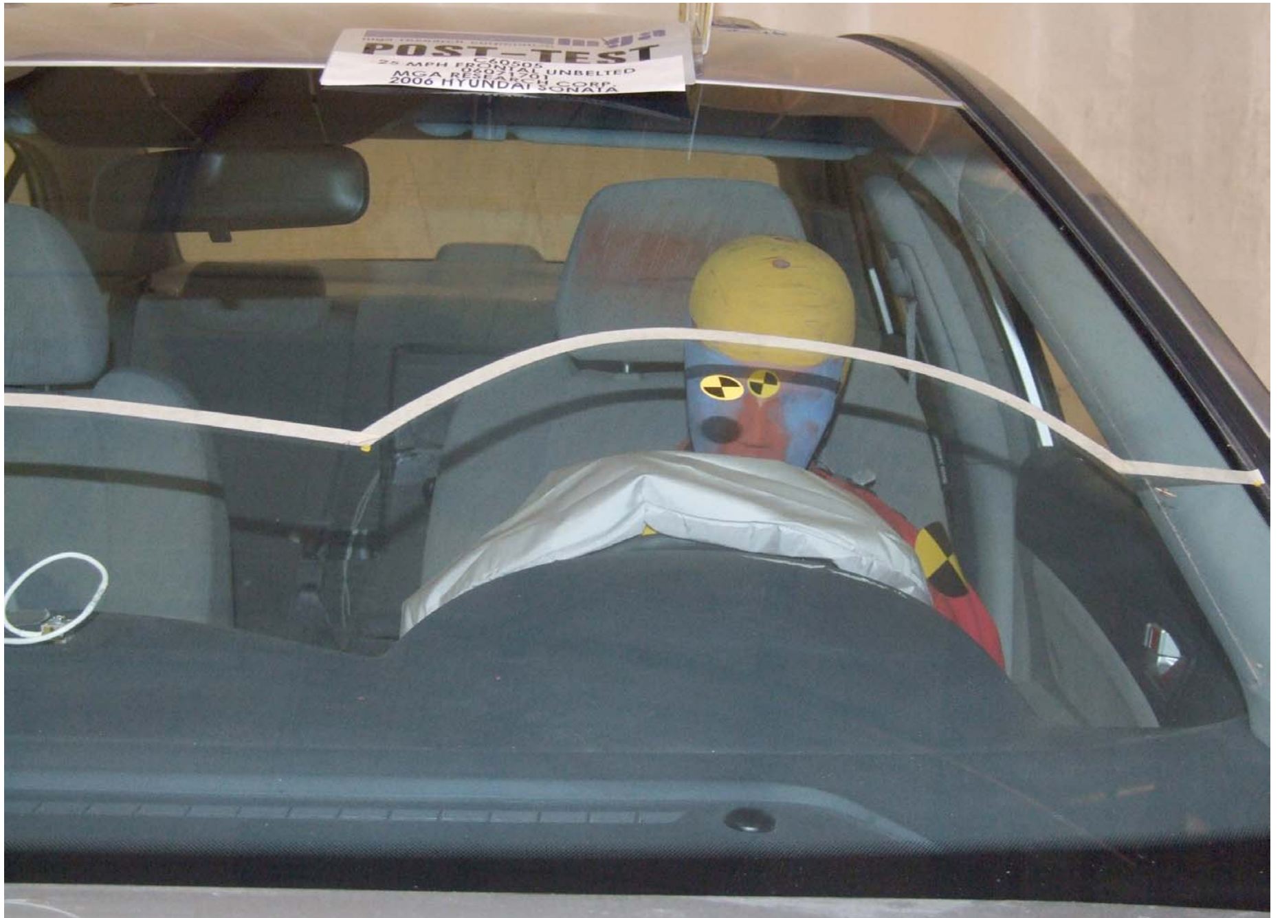
Post-Test Driver Dummy Front View (head position)
