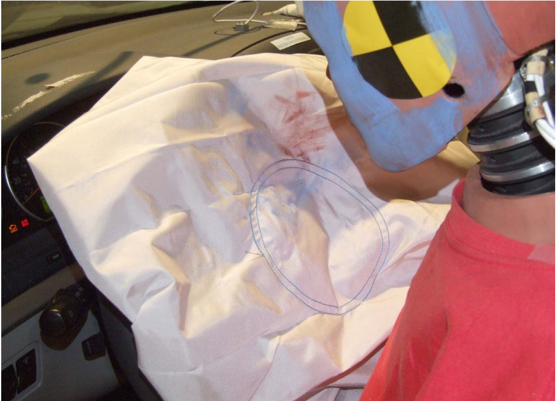
Post-Test Driver Dummy Airbag Contact
