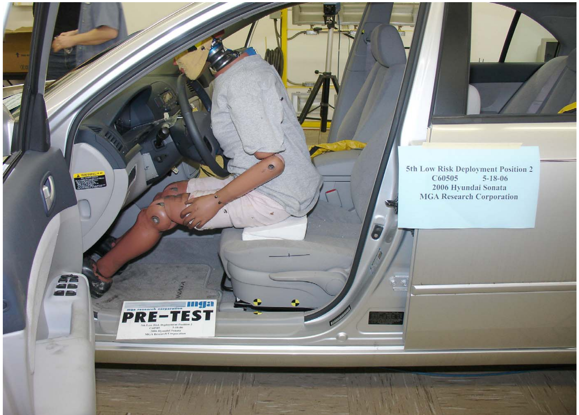
Pre-Test 5th Fem. P2 Driver Dummy Left Side View (Door Open) Trial 2
