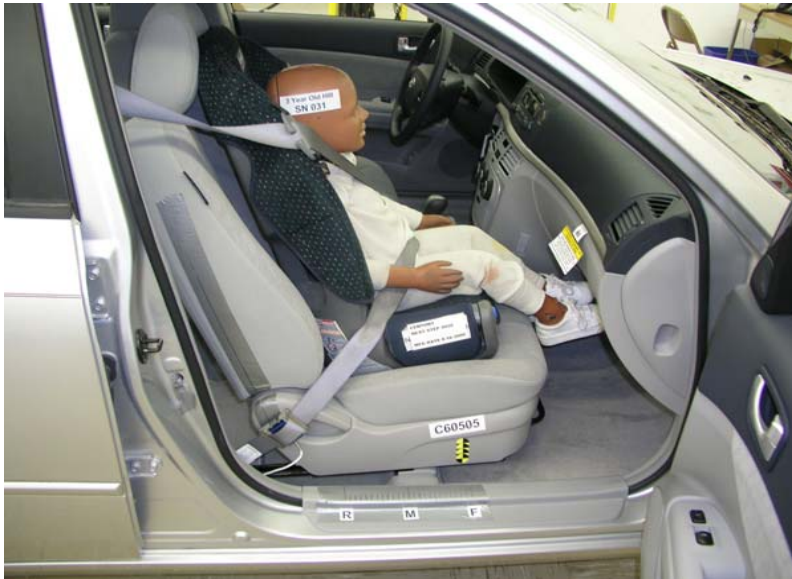
3-Year-Old Century Next Step With Belt, Forward Seat Track
