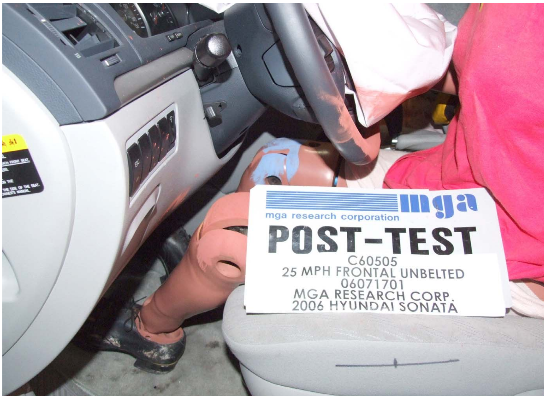
Post-Test Driver Side Knee Bolster View
