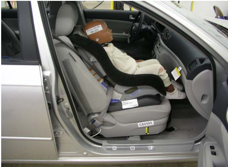
3-Year-Old Fwd Facing Century Encore With Belt, Forward Seat Track
