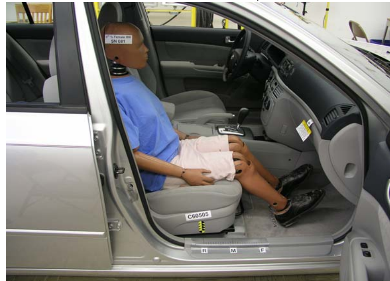
Unbelted 5th Percentile Female Reactivation, Rearward Seat Track
