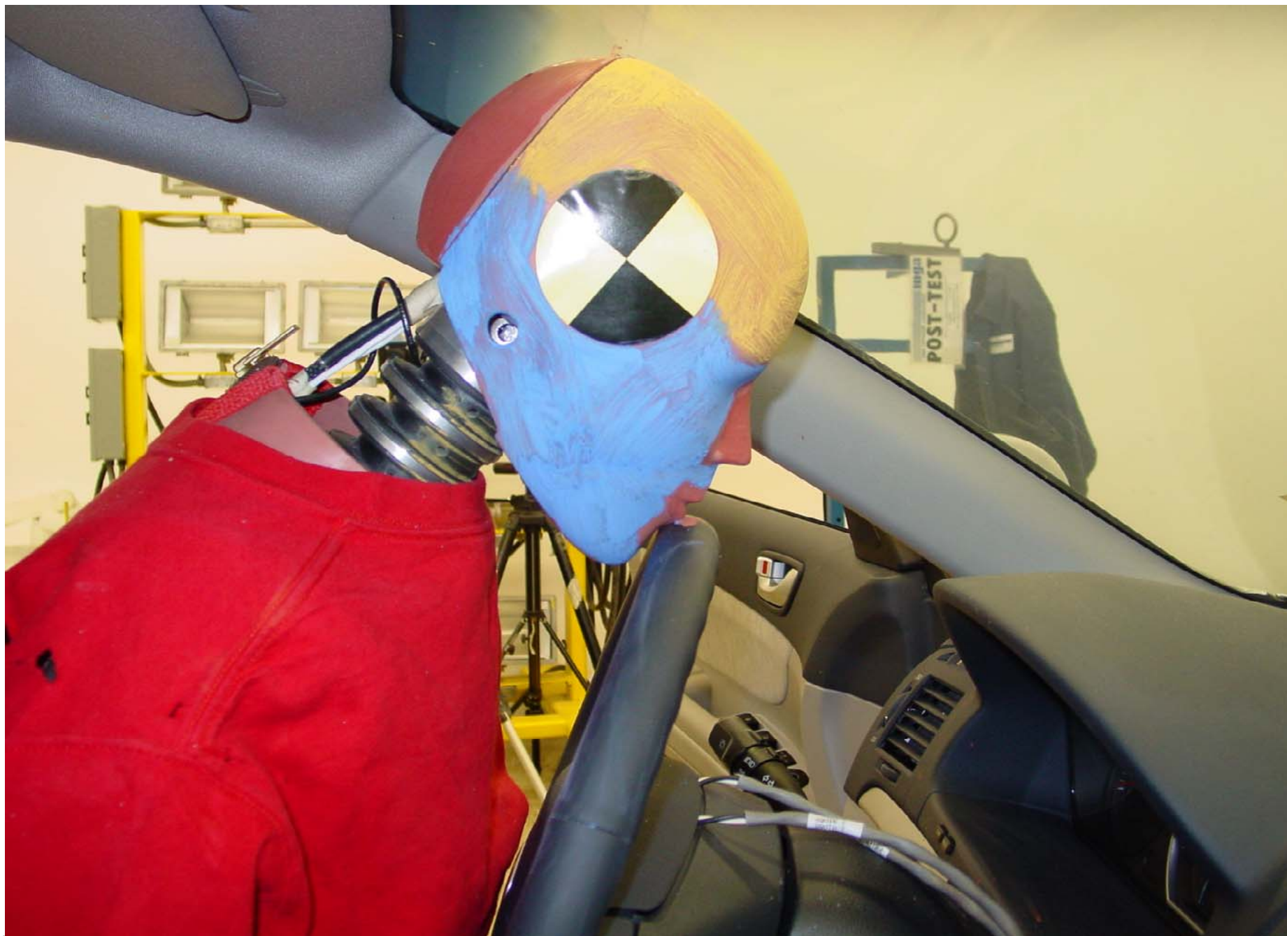
Pre-Test 5th Fem. P2 Driver Dummy Right Side Head Position View Trial 1
