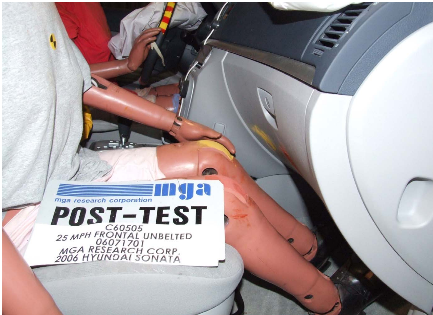
Post-Test Passenger Side Knee Bolster View
