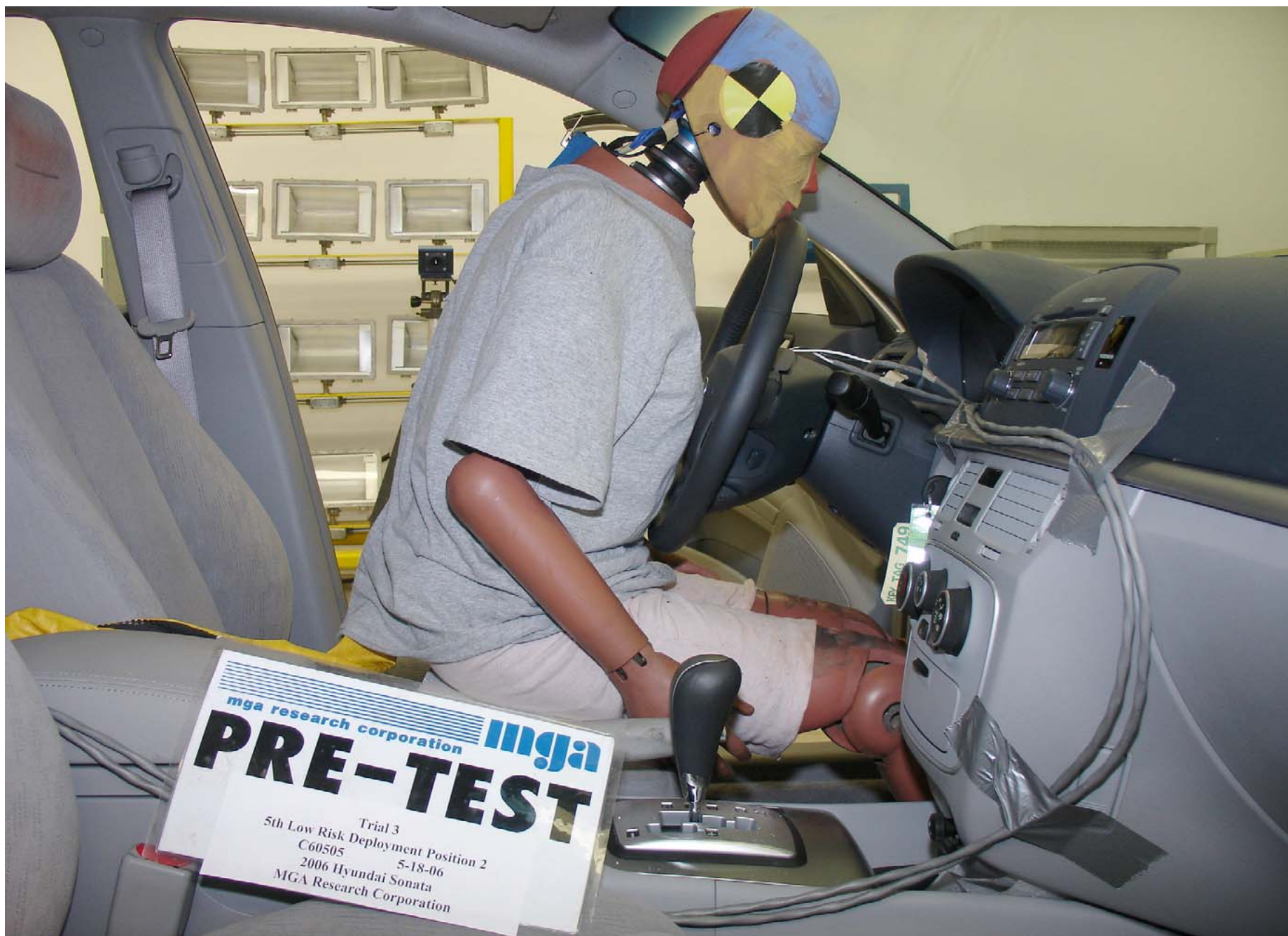
Pre-Test 5th Fem. P2 Driver Dummy Right Side View (Door Open) Trial 3
