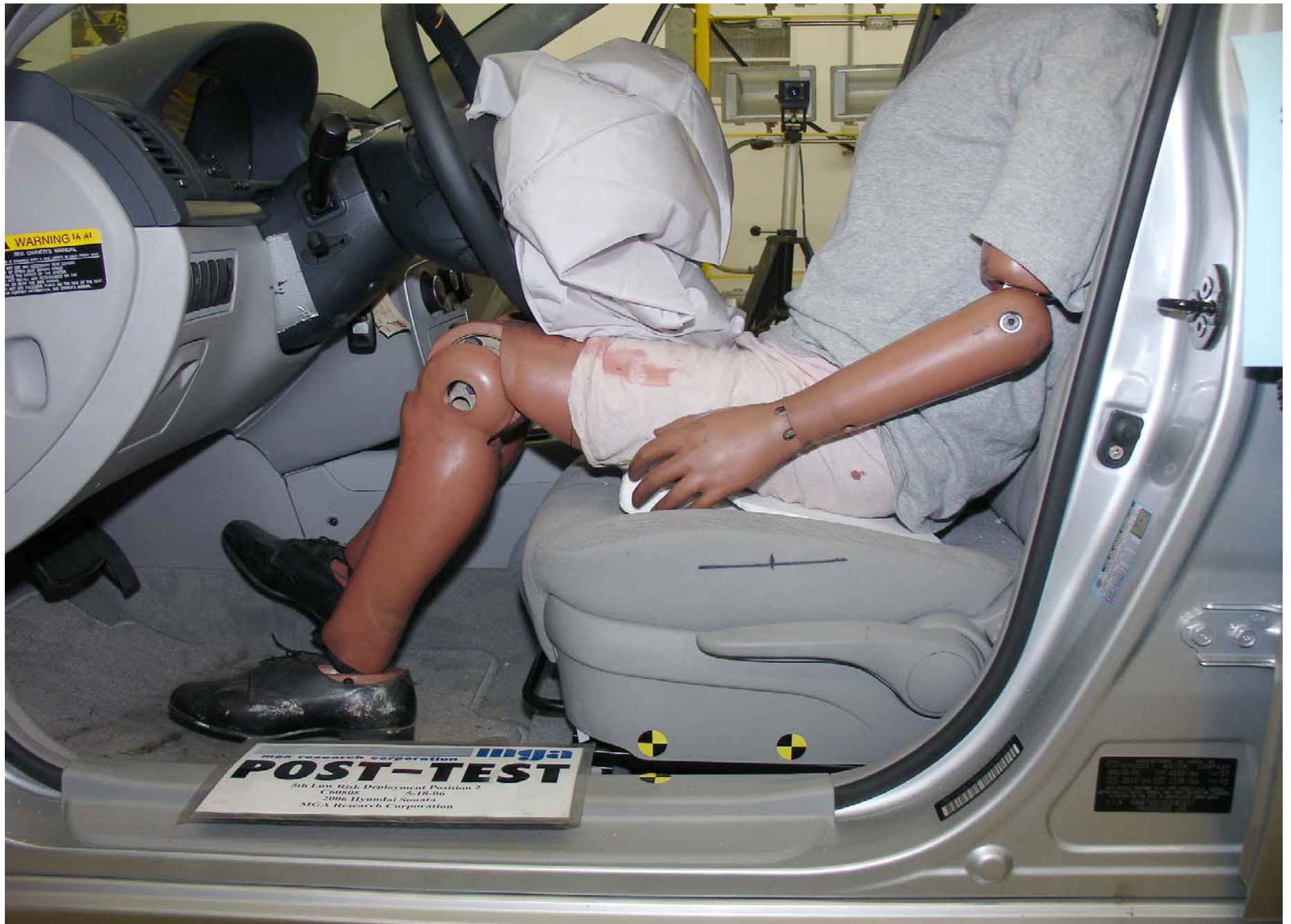
Post-Test 5th Fem. P2 Driver Dummy Left Side Mid Position View Trial 2
