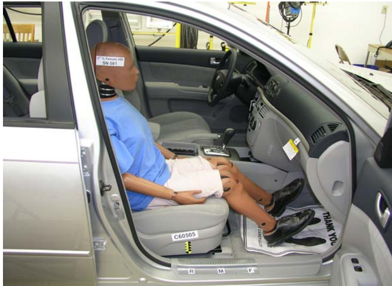
Unbelted 5th Percentile Female Reactivation, Rear Seat Track
