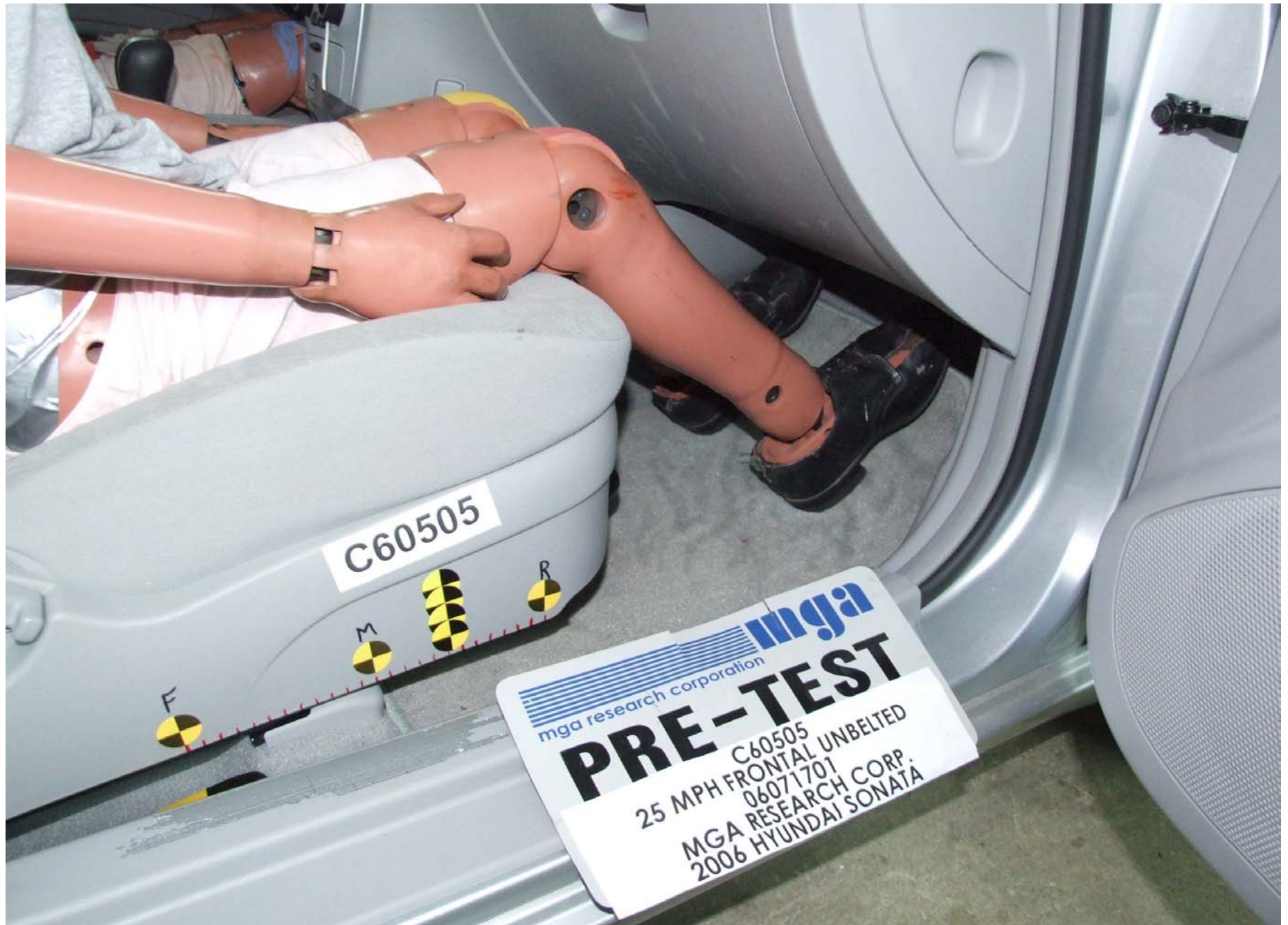
Pre-Test Passenger Dummy Feet Position
