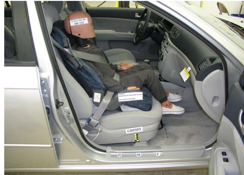
6-Year-Old Cosco High Back Booster With Belt, Middle Seat Track
