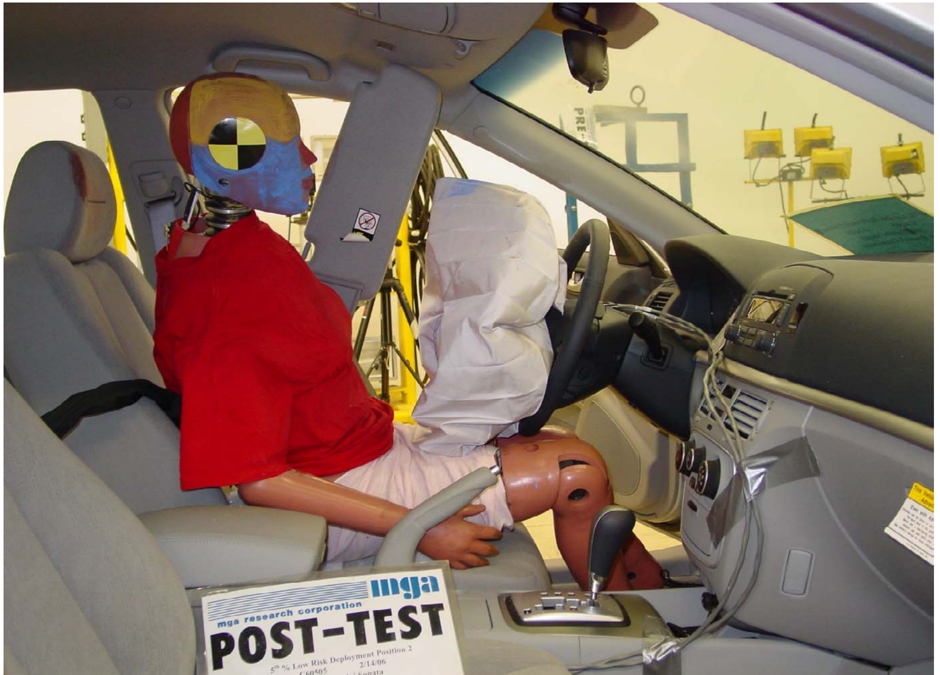
Post-Test 5th Fem. P2 Driver Dummy Right Side View (Door Open) Trial 1
