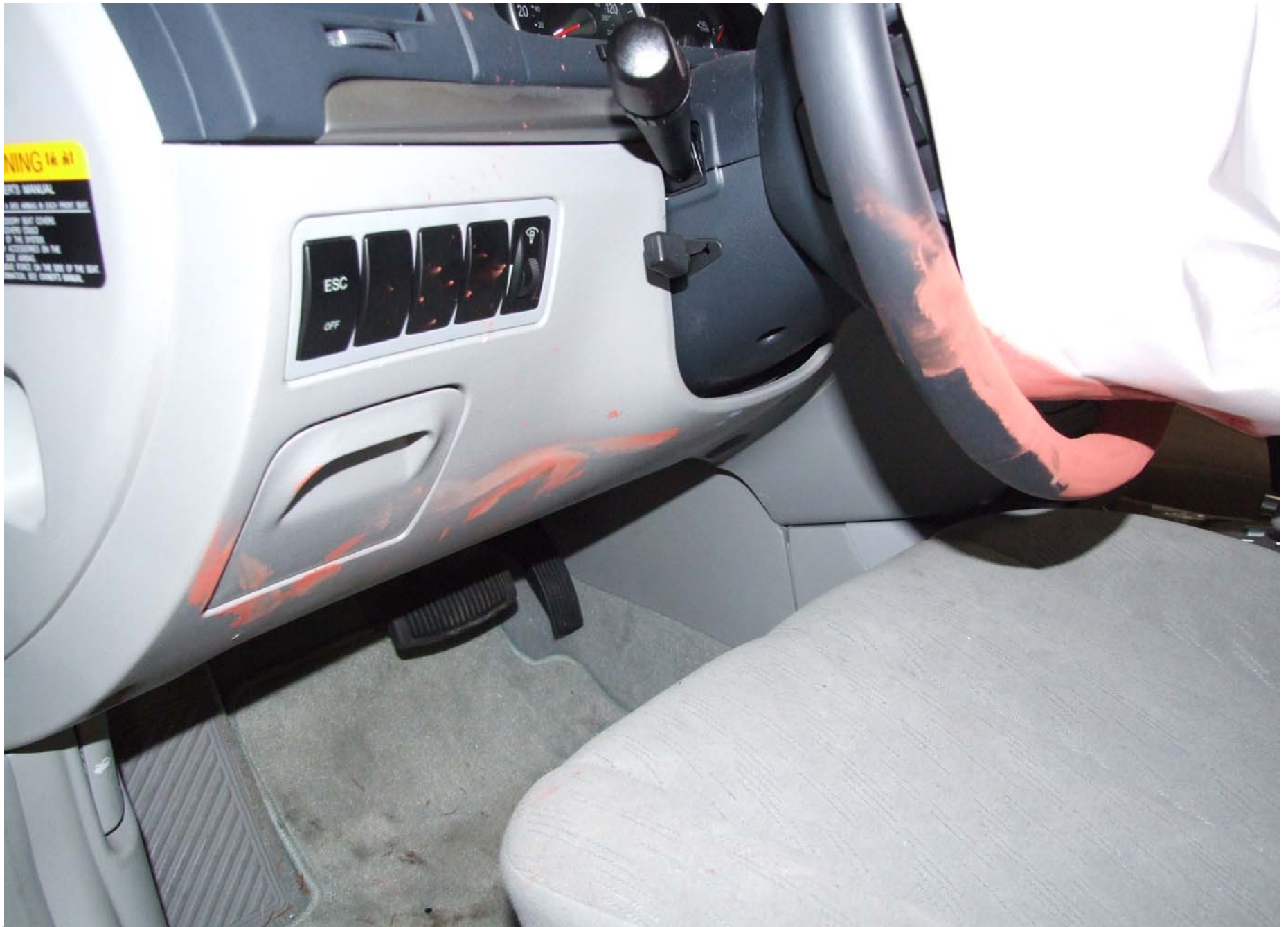
Post-Test Driver Dummy Knee Contact
