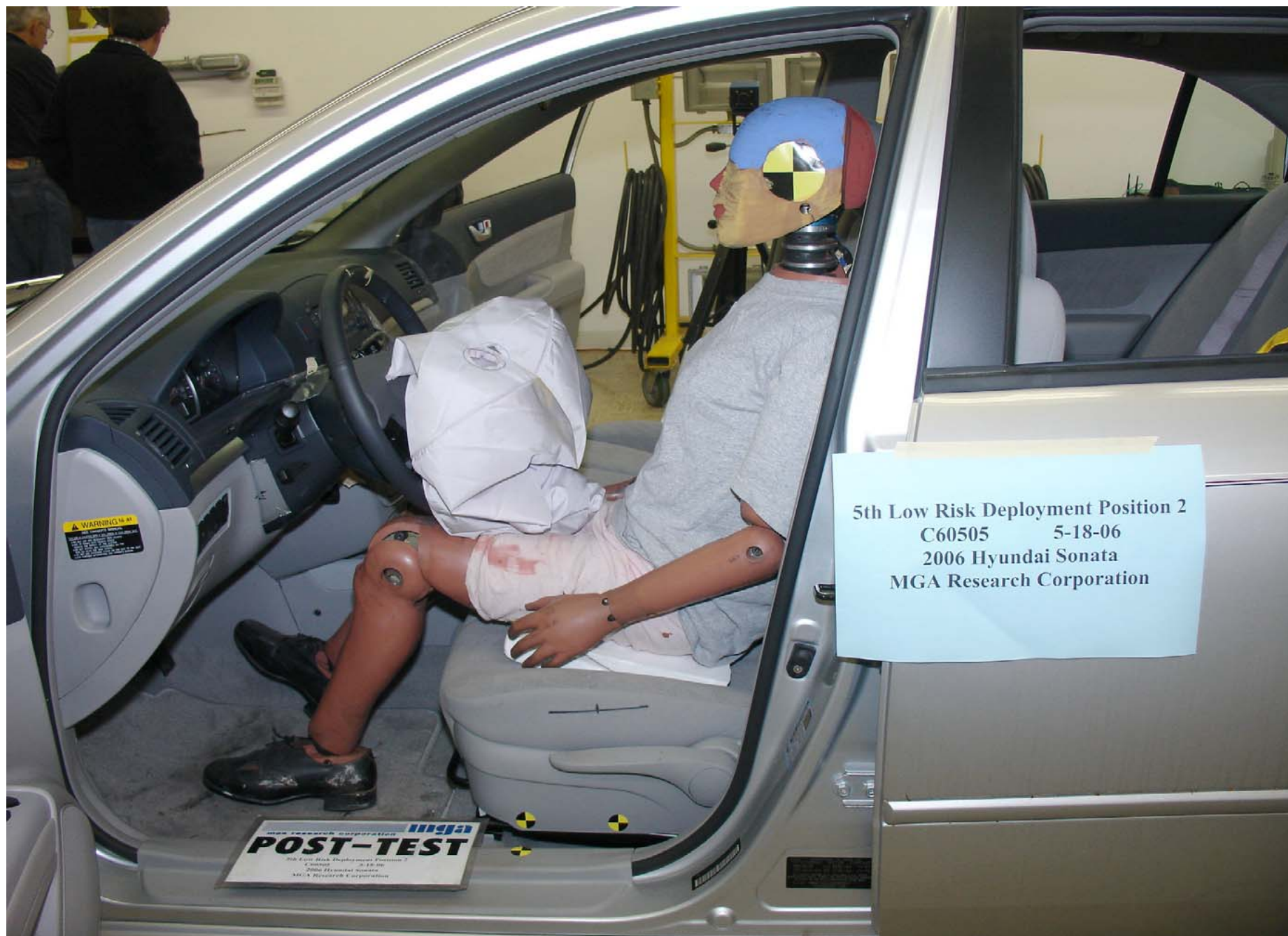
Post-Test 5th Fem. P2 Driver Dummy Left Side View (Door Open) Trial 2
