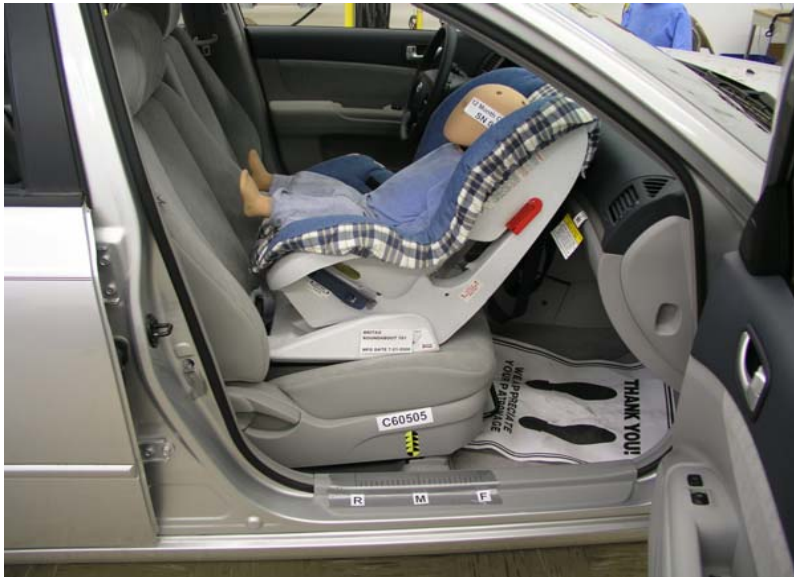
Britax Roundabout 161 Rear Facing Unbuckled, Middle Seat Track
