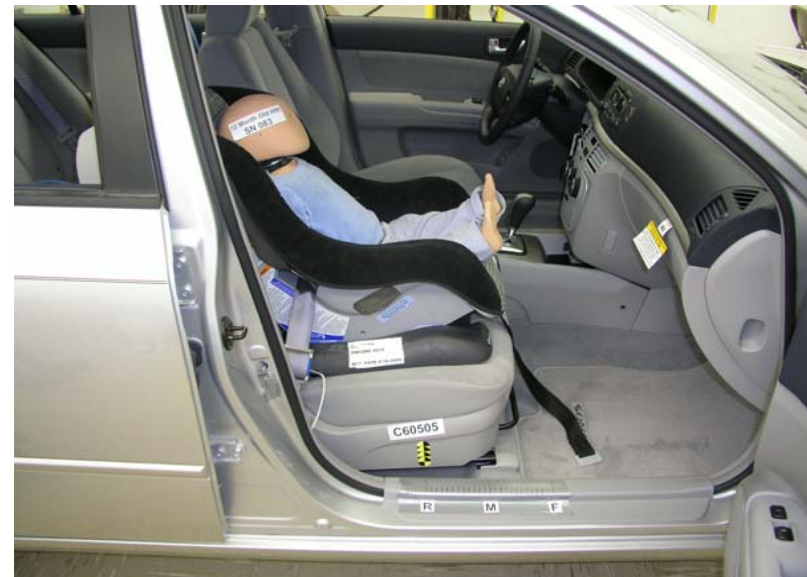
Century Encore Fwd Facing With Belt, Rearward Seat Track
