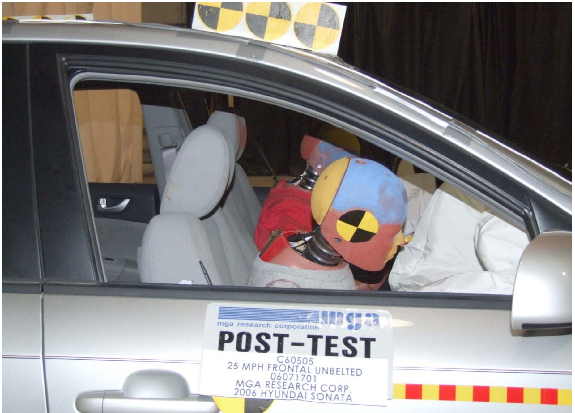
Post-Test Passenger Dummy Position Right Side View
