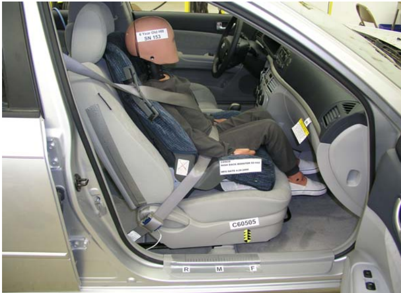
6-Year-Old Cosco High Back Booster With Belt, Forward Seat Track
