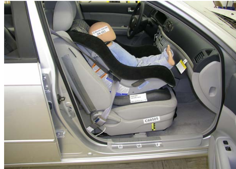
Century Encore Fwd Facing With Belt, Forward Seat Track
