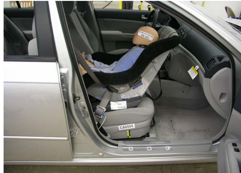
Century Encore Rear Facing With Belt, Rearward Seat Track
