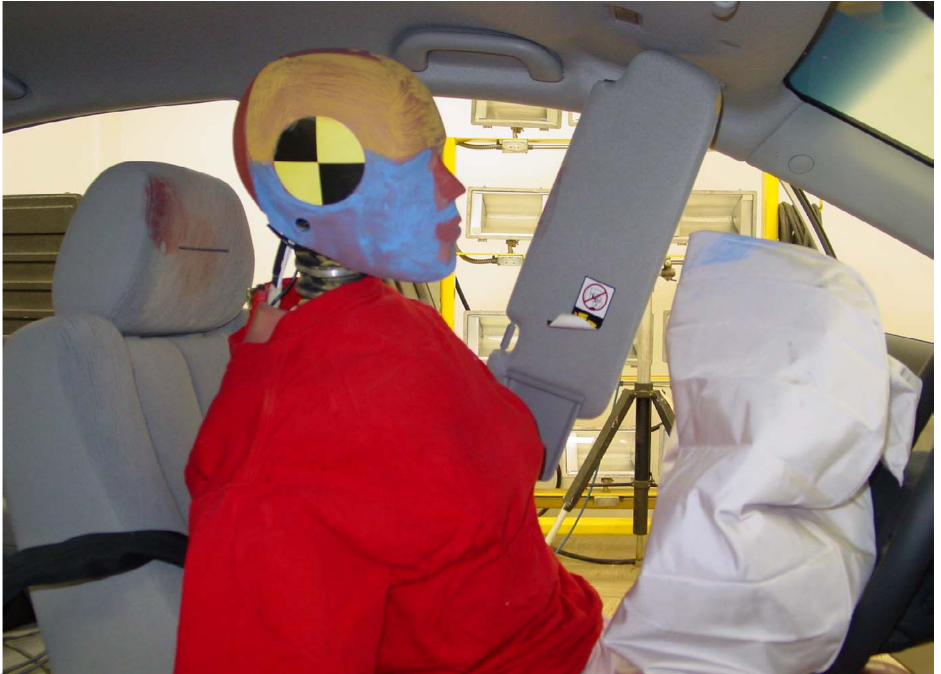
Post-Test 5th Fem. P2 Driver Dummy Right Side Head Position View Trial 1
