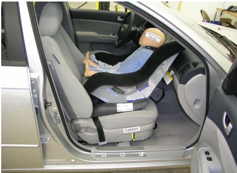
Century Encore Rear Facing Unbelted, Forward Seat Track
