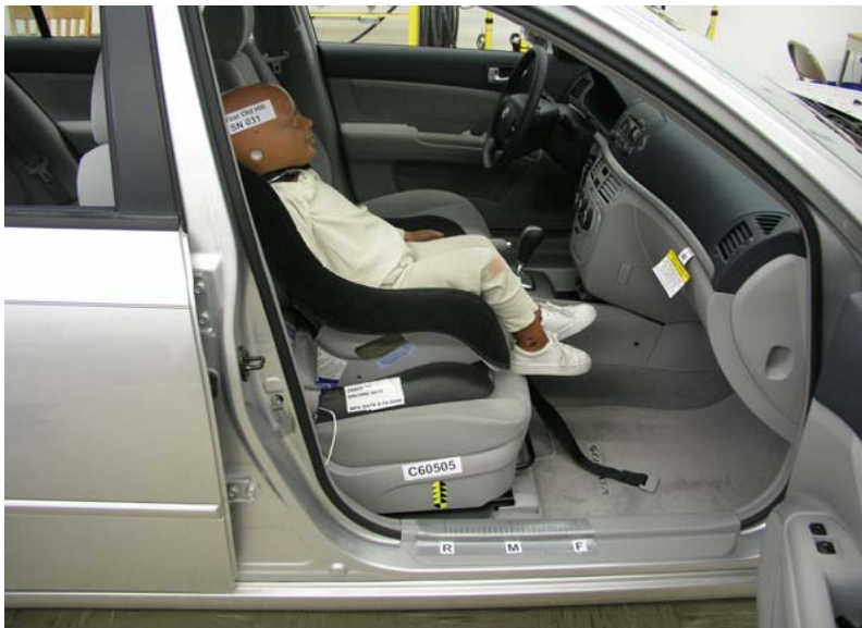
3-Year-Old Fwd Facing Century Encore With Belt, Rearward Seat Track
