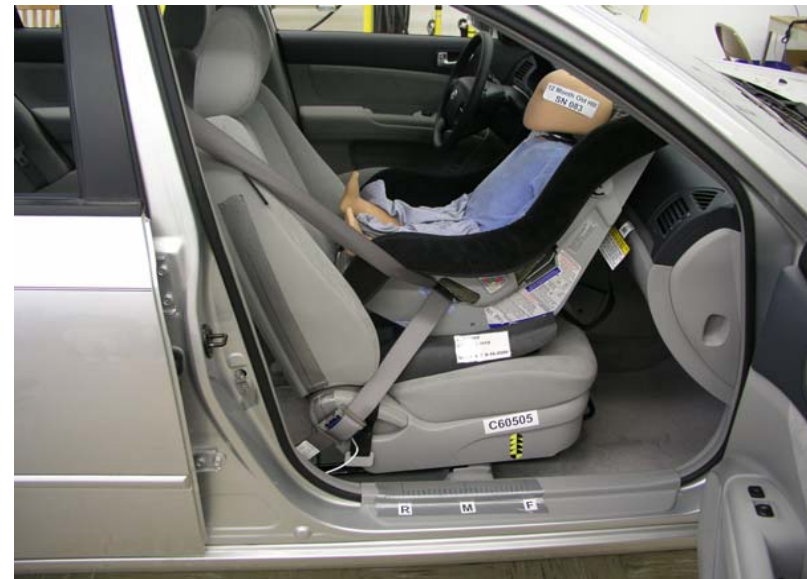
Century Encore Rear Facing With Belt, Forward Seat Track
