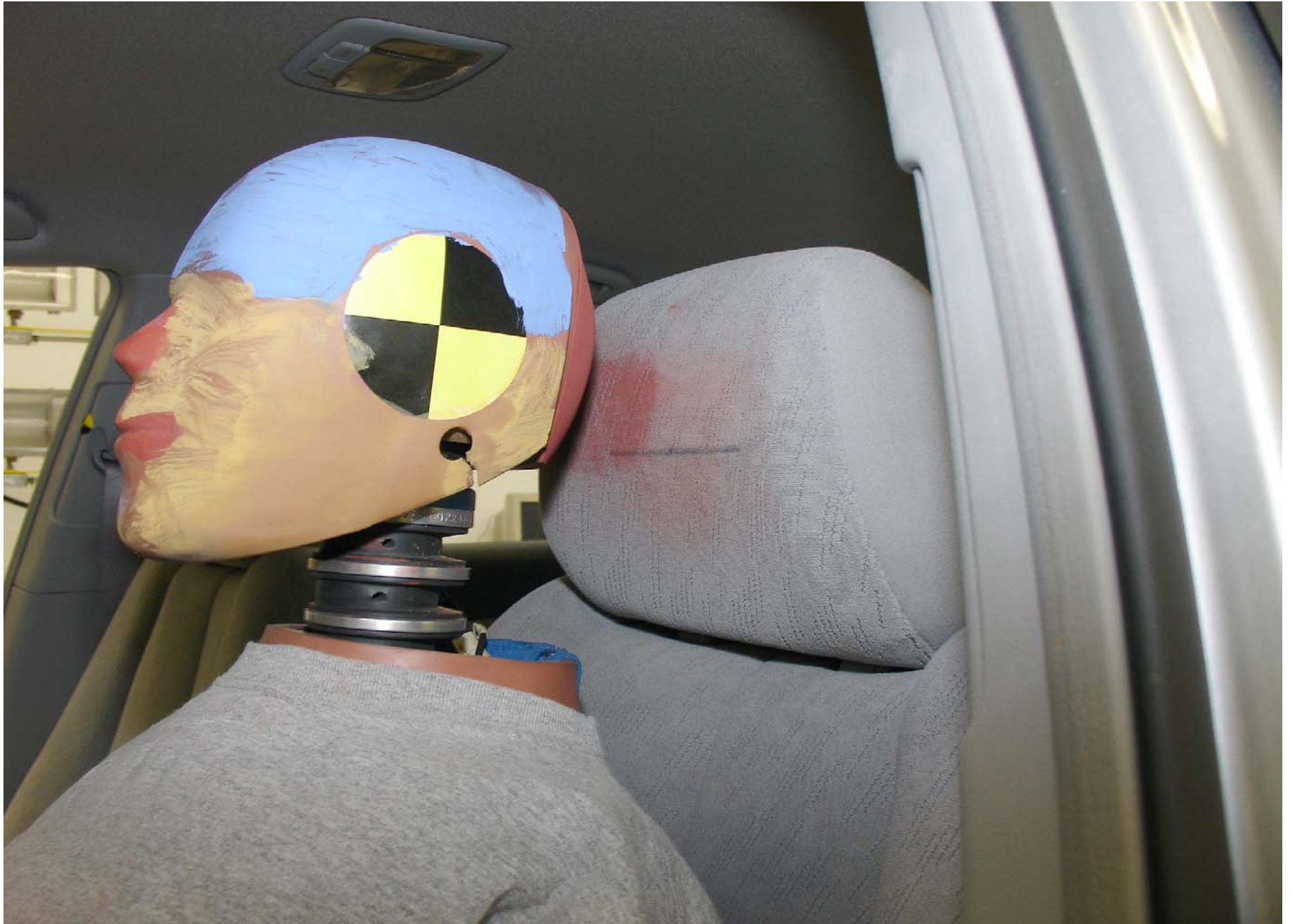
Post-Test 5th Fem. P2 Driver Dummy Left Side Head Position View Trial 3
