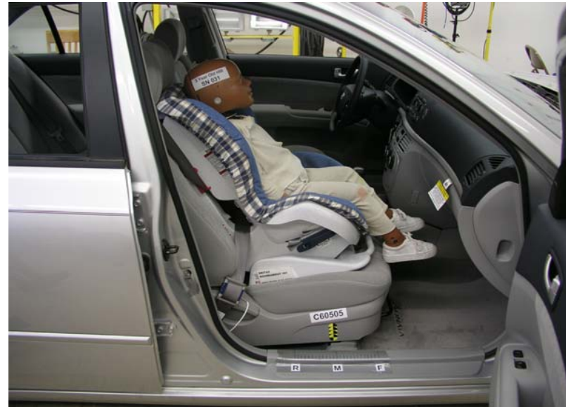
3-Year-Old Fwd Facing Britax Roundabout With Belt, Middle Seat Track
