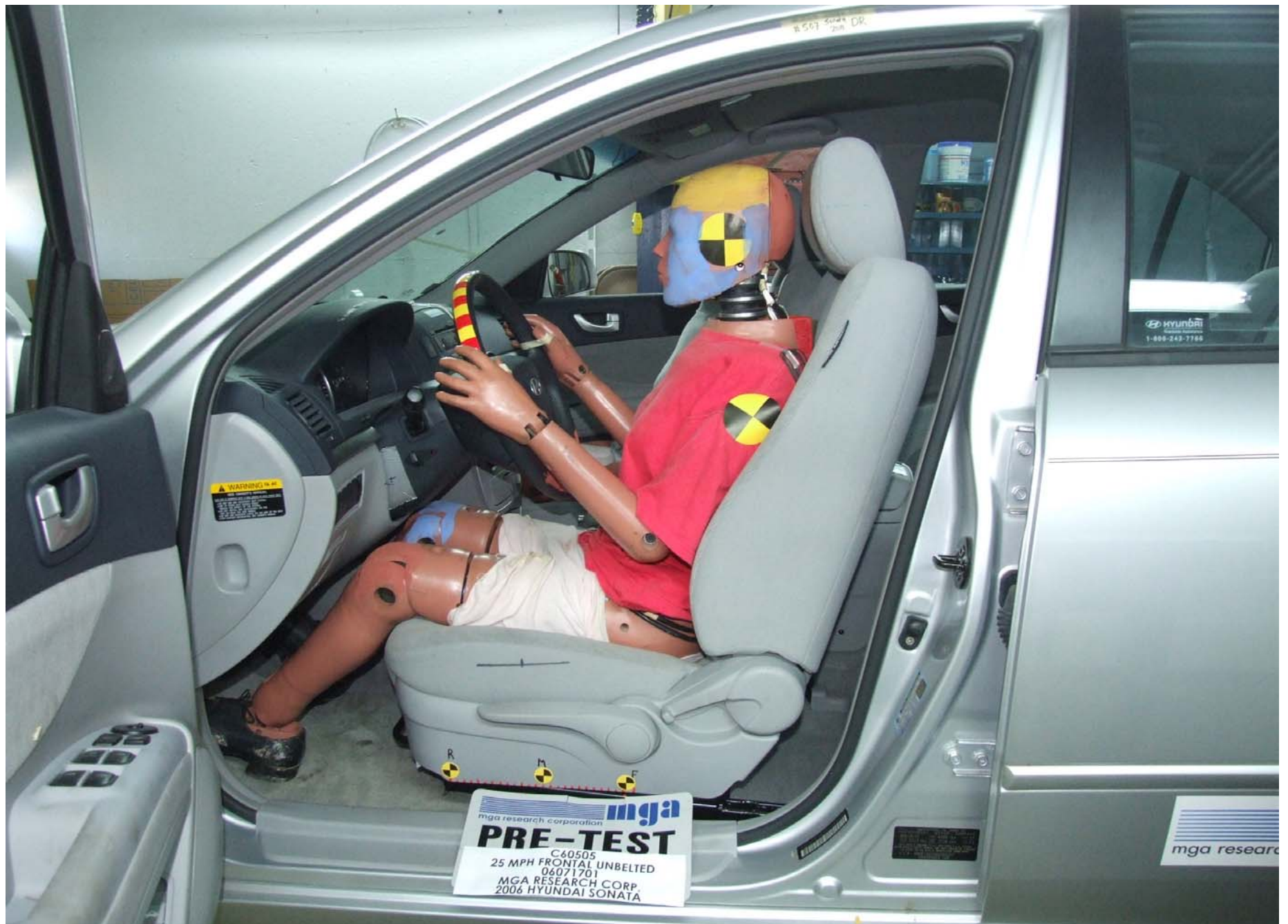
Pre-Test Driver Dummy Position Left Side View (Door Open)
