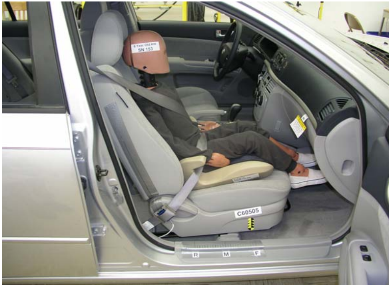
6-Year-Old Evenflo Right Fit With Belt, Forward Seat Track
