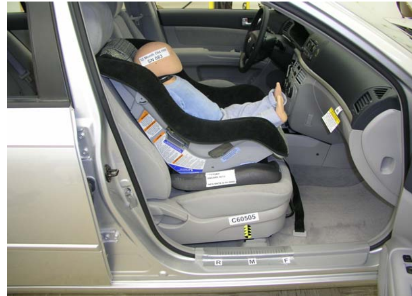
Century Encore Fwd Facing Unbelted, Middle Seat Track
