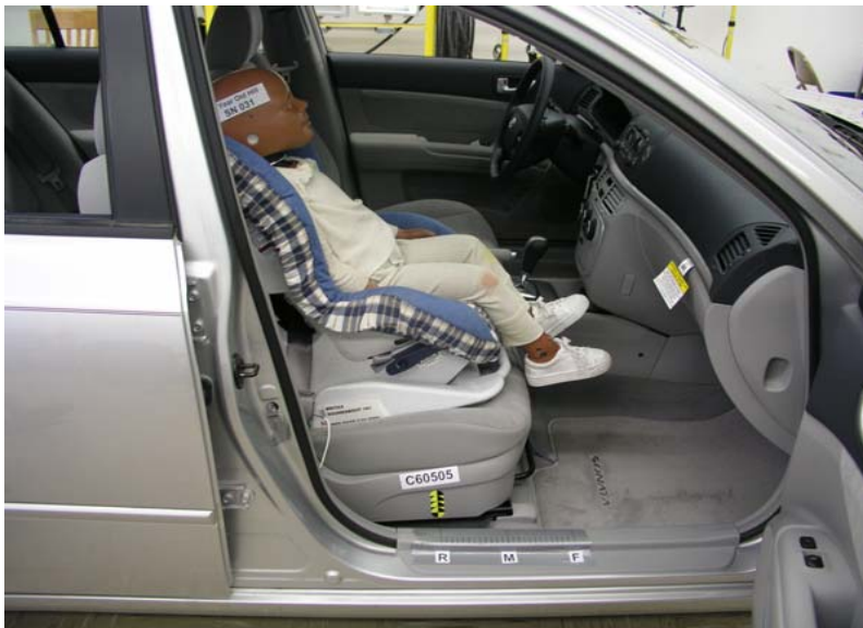
3-Year-Old Fwd Facing Britax Roundabout With Belt, Rearward Seat Track
