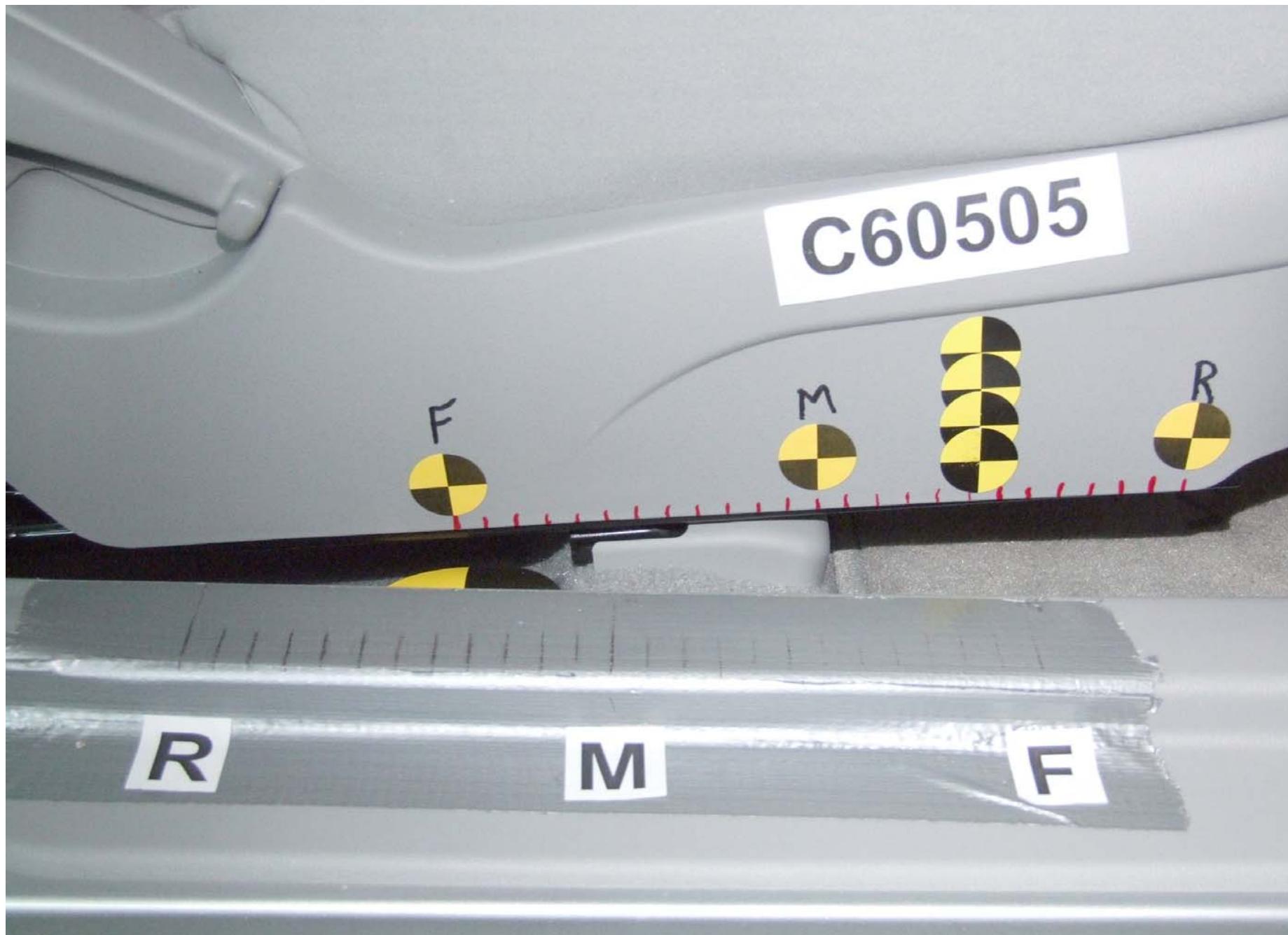
Pre-Test Passenger Dummy Seat Position
