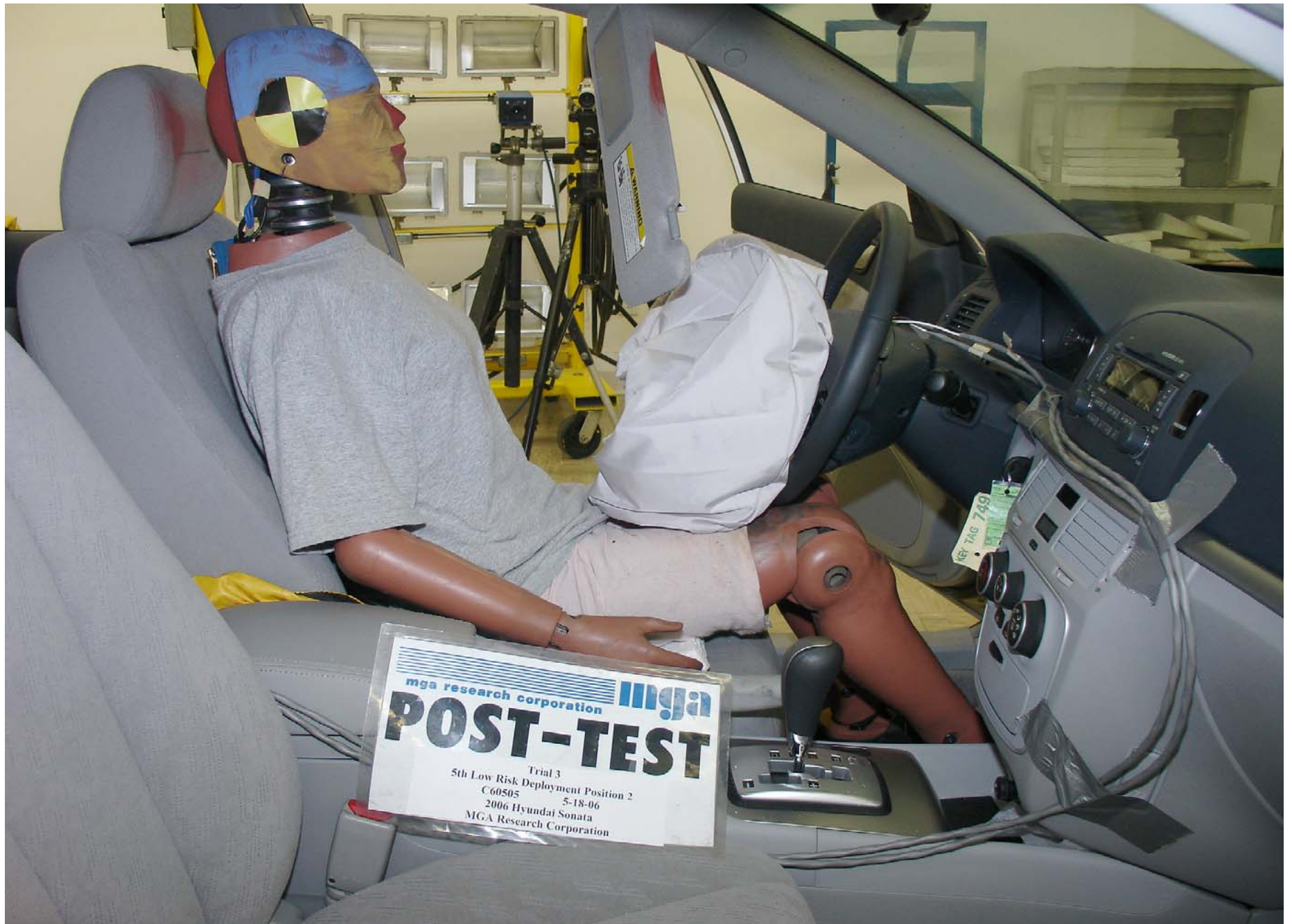
Post-Test 5th Fem. P2 Driver Dummy Right Side View (Door Open) Trial 3
