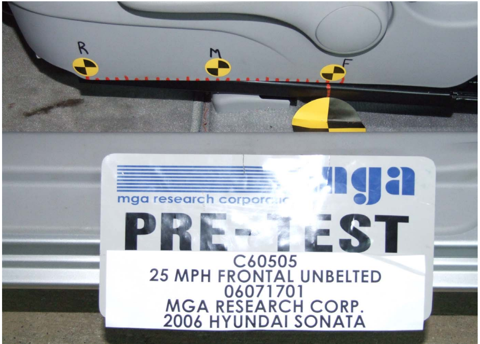
Pre-Test Driver Dummy Seat Position
