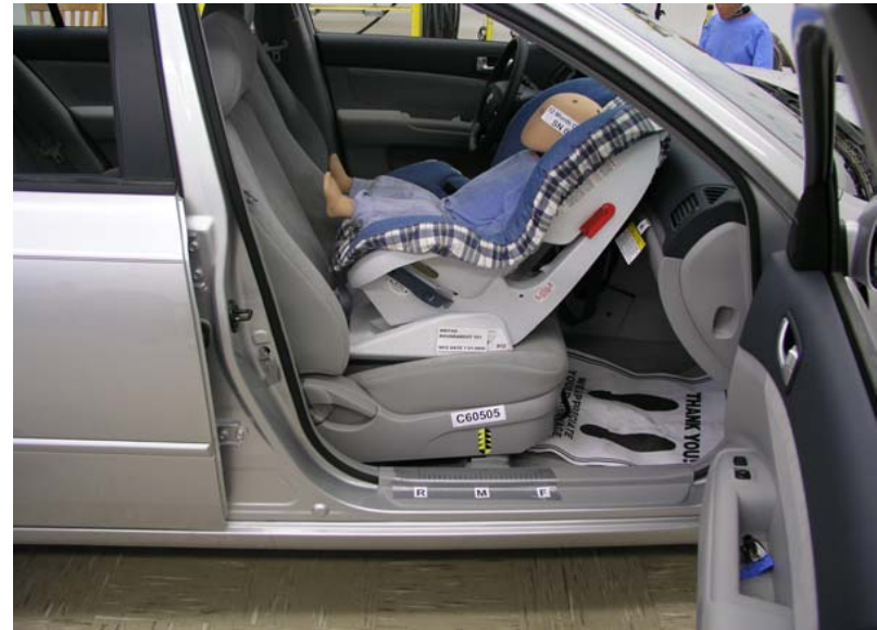
Britax Roundabout 161 Rear Facing Unbuckled, Forward Seat Track
