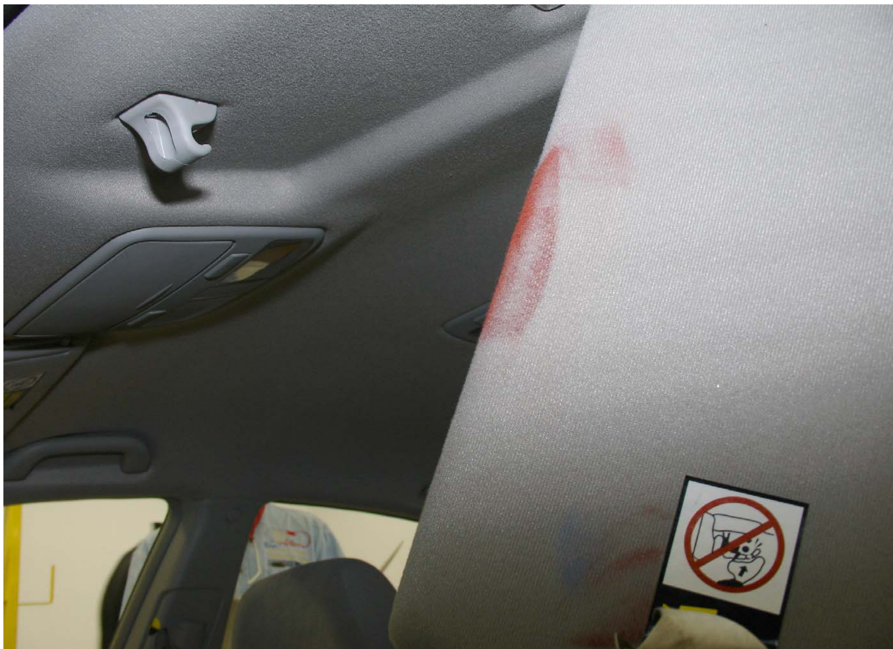
Post-Test 5th Fem. P2 Driver Dummy Head Contact View Trial 3
