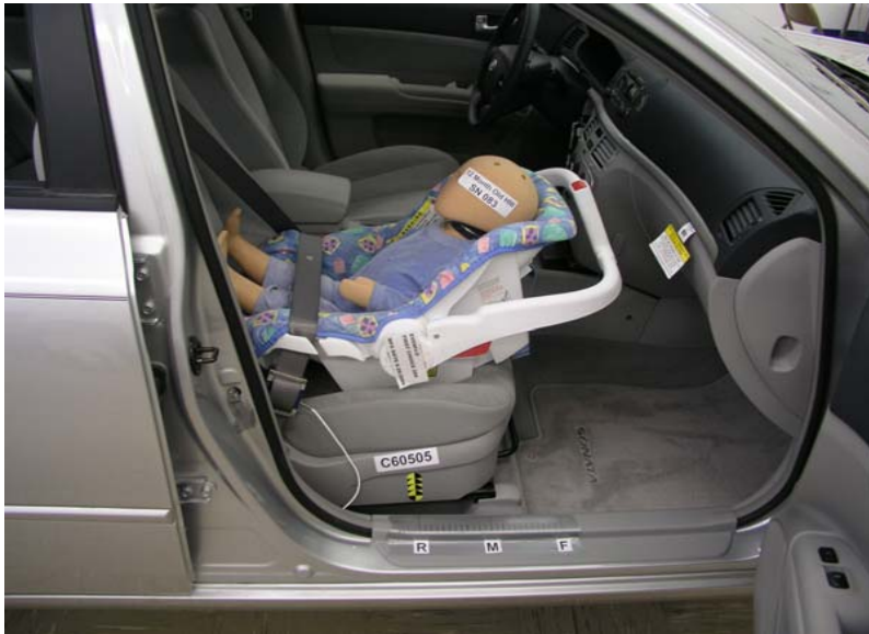
Evenflo First Choice 204 With Belt, Rearward Seat Track, Handle Down
