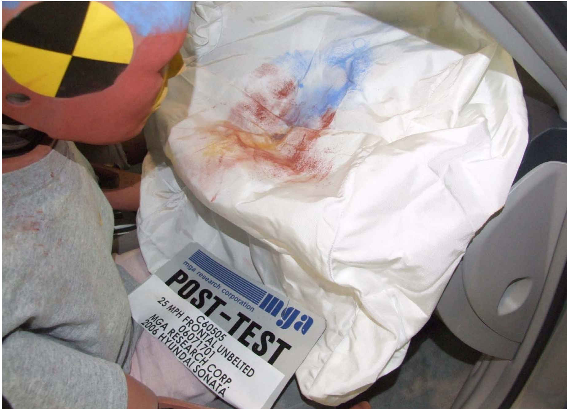
Post-Test Passenger Dummy Airbag Contact
