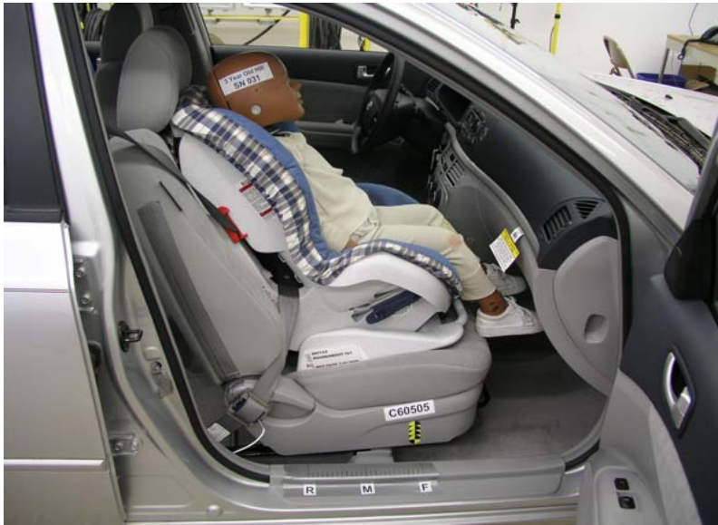
3-Year-Old Fwd Facing Britax Roundabout With Belt, Forward Seat Track
