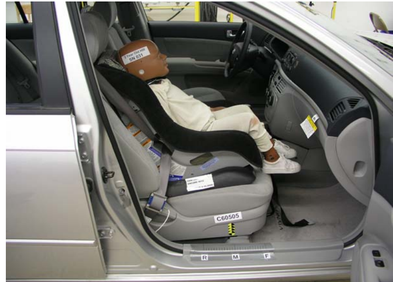
3-Year-Old Fwd Facing Century Encore With Belt, Middle Seat Track
