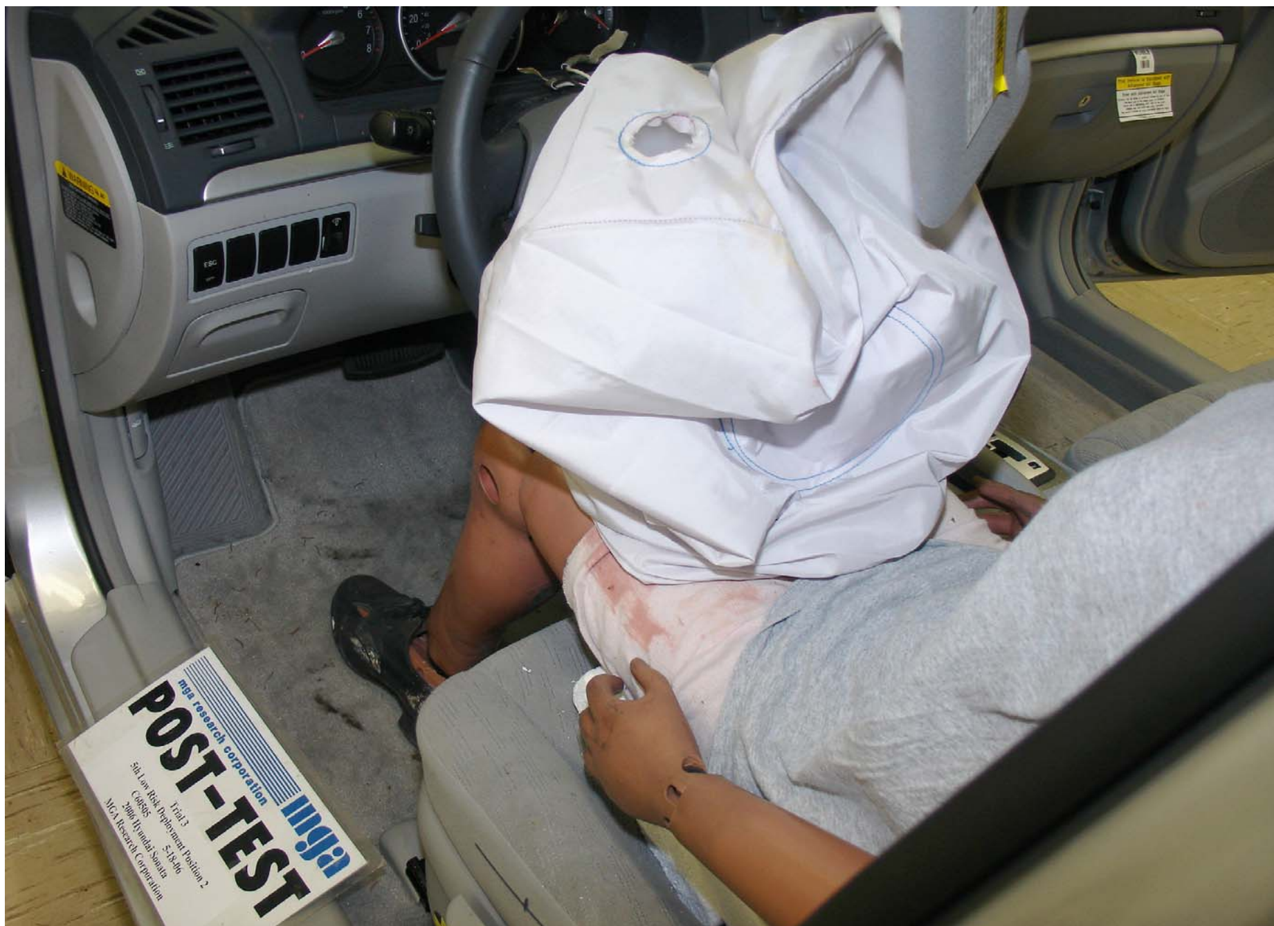
Post-Test 5th Fem. P2 Driver Dummy Airbag Left View Trial 3
