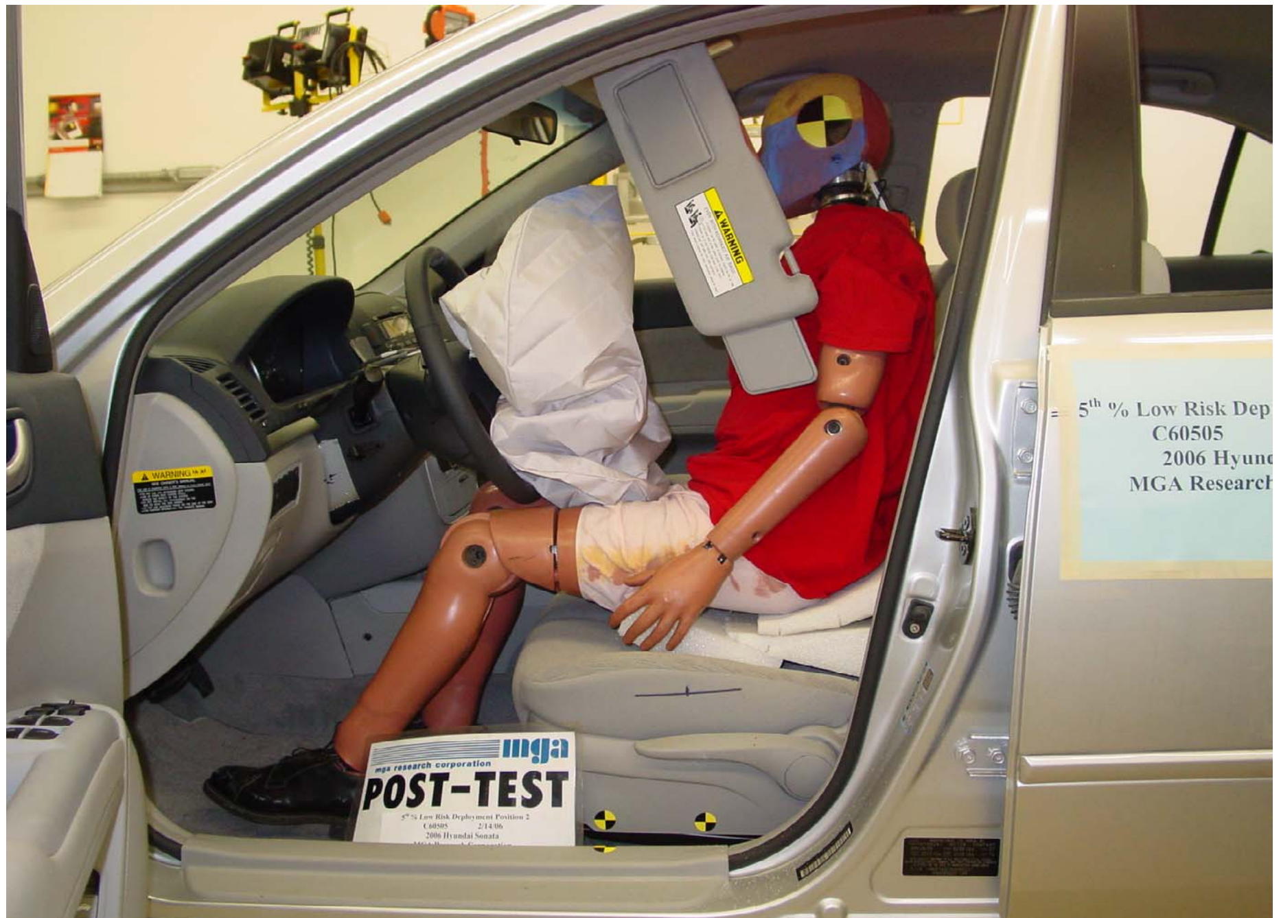
Post-Test 5th Fem. P2 Driver Dummy Left Side View (Door Open) Trial 1
