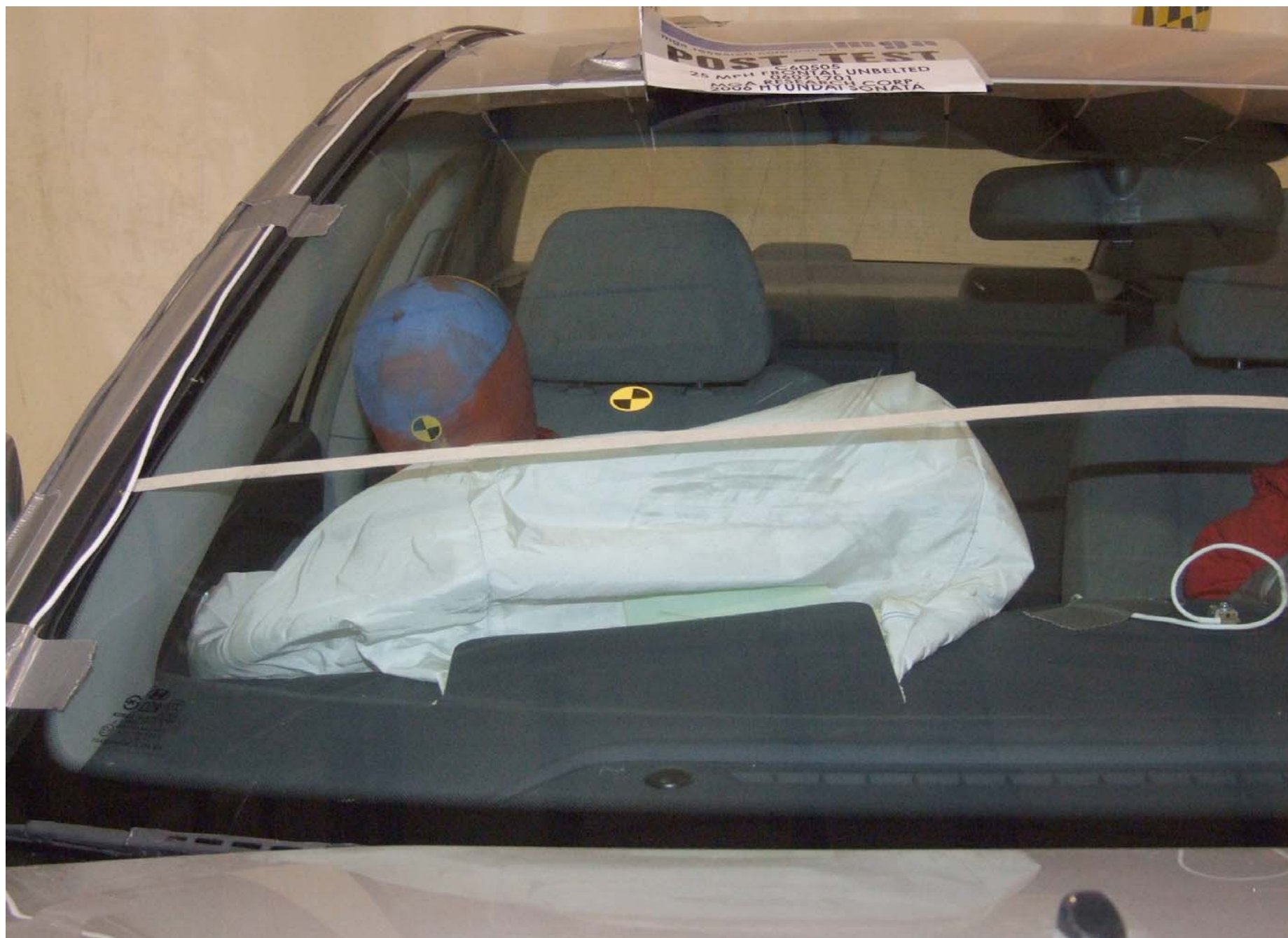
Post-Test Passenger Dummy Front View (head position)
