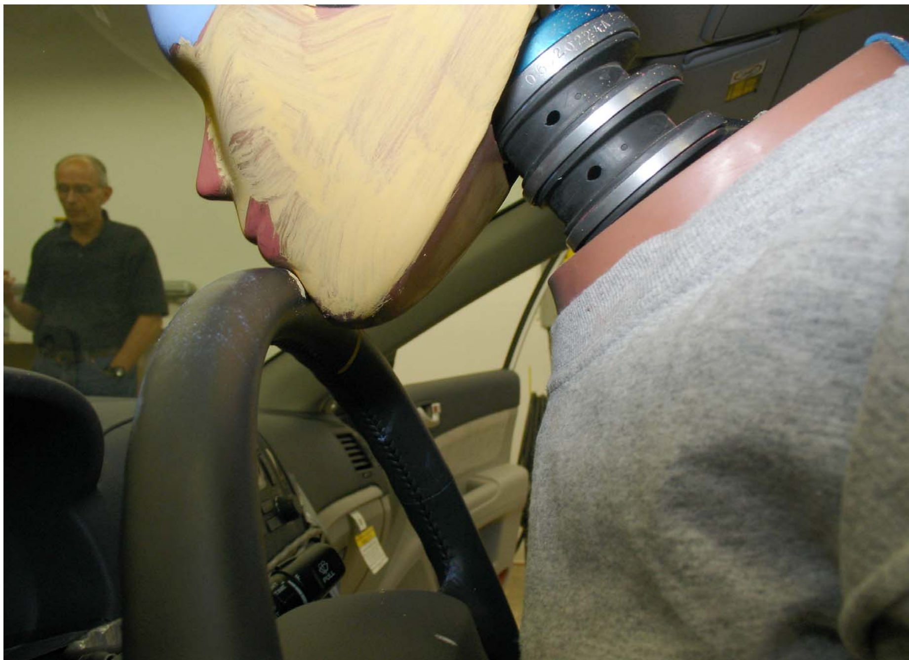
Pre-Test 5th Fem. P2 Driver Dummy Left Side Head Position View Trial 2
