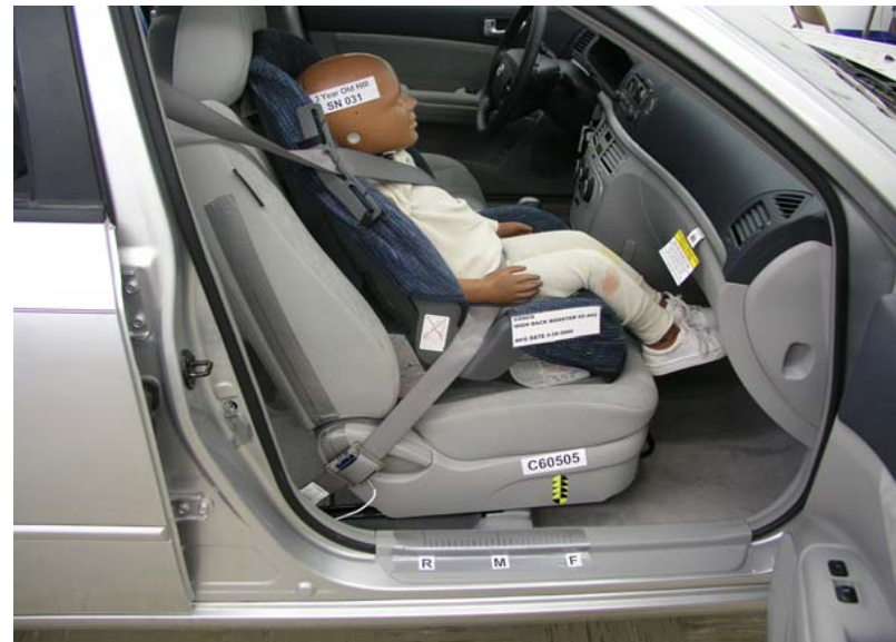
3-Year-Old Cosco High Back Booster With Belt, Forward Seat Track
