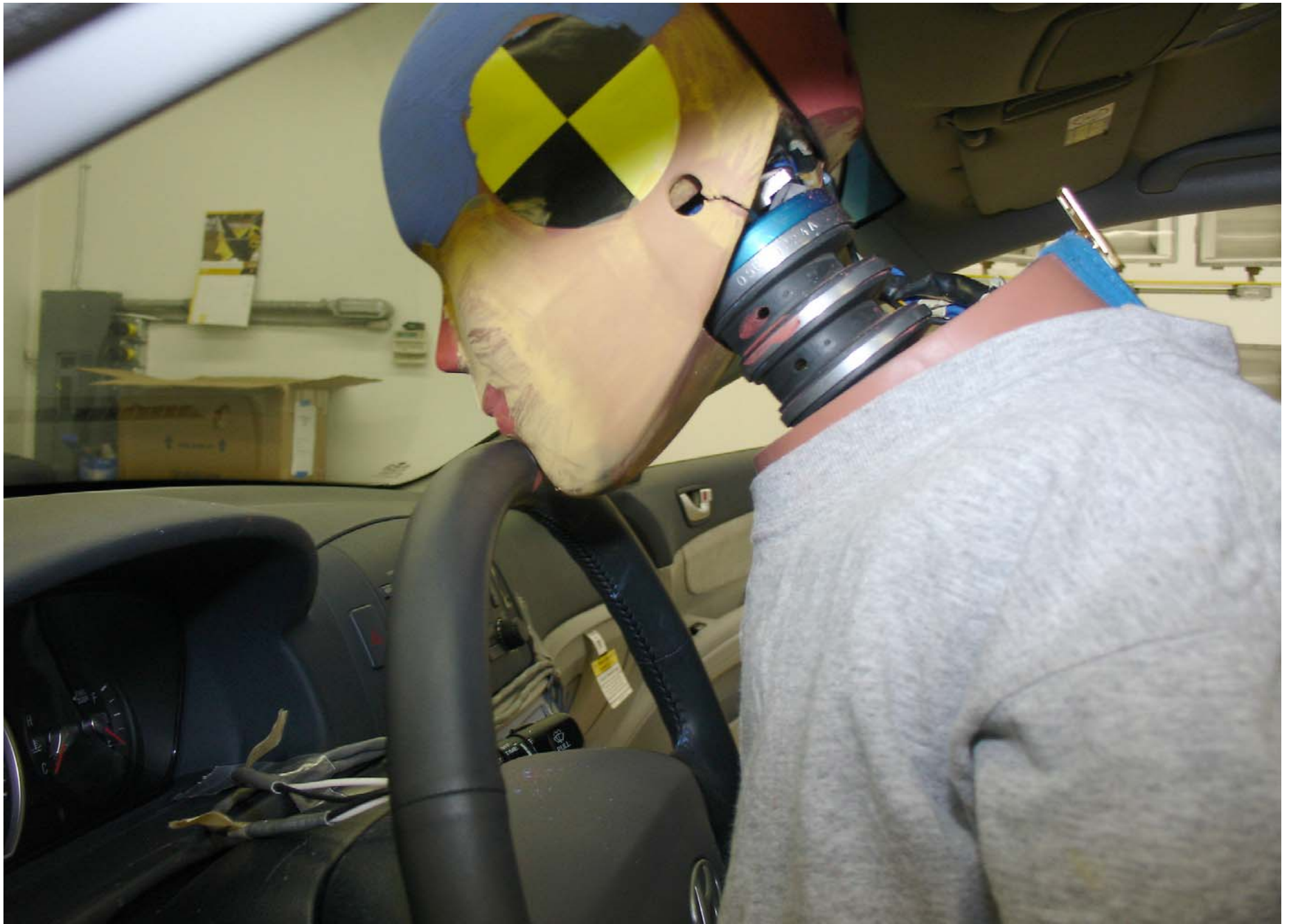
Pre-Test 5th Fem. P2 Driver Dummy Left Side Head Position View Trial 3
