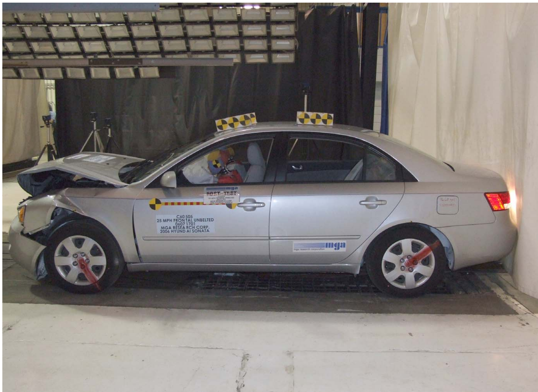
Post-Test Left Side View of Test Vehicle
