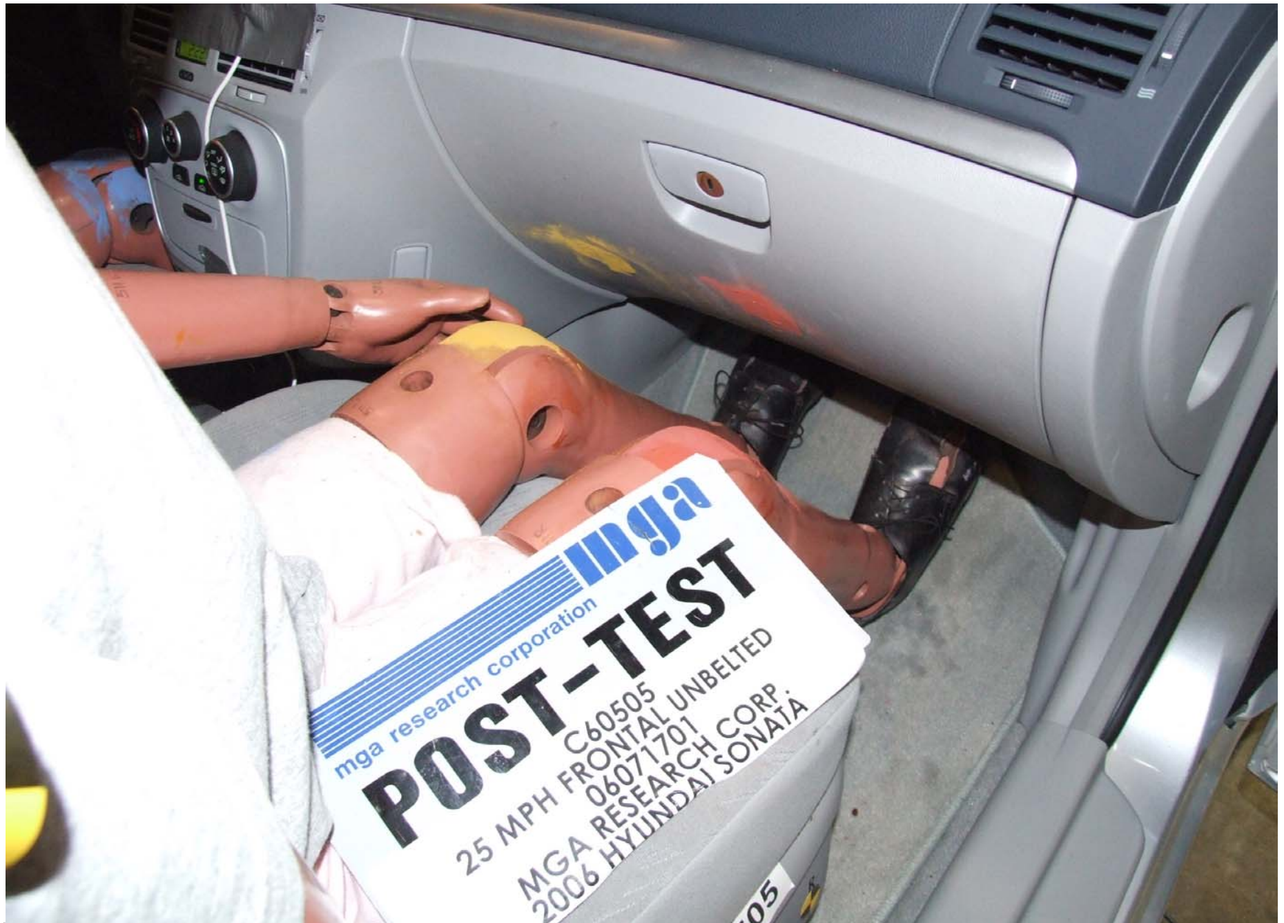
Post-Test Passenger Dummy Feet Position
