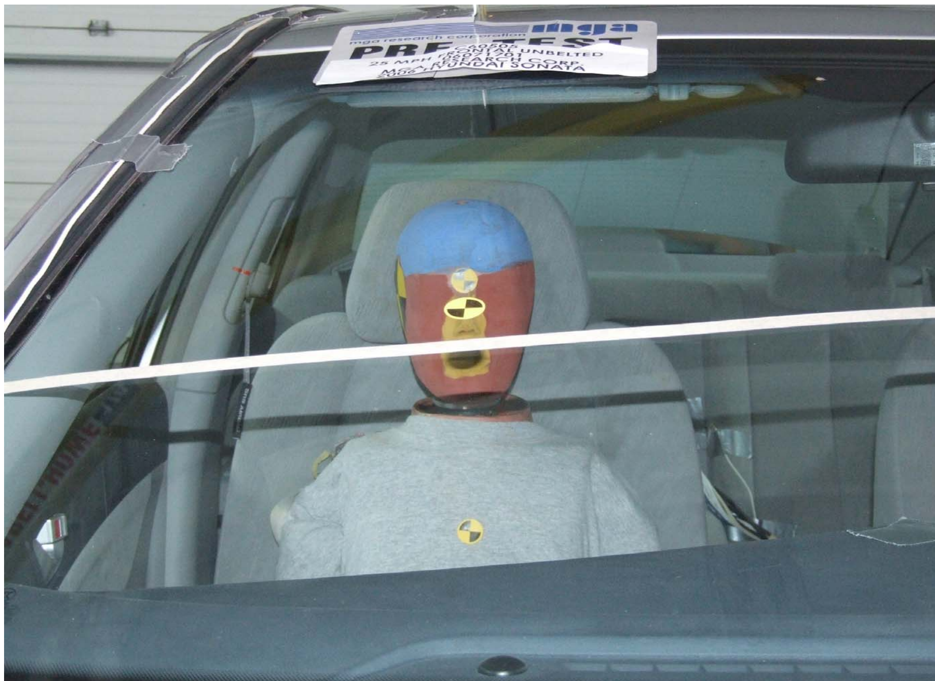
Pre-Test Passenger Dummy Front View (head position)
