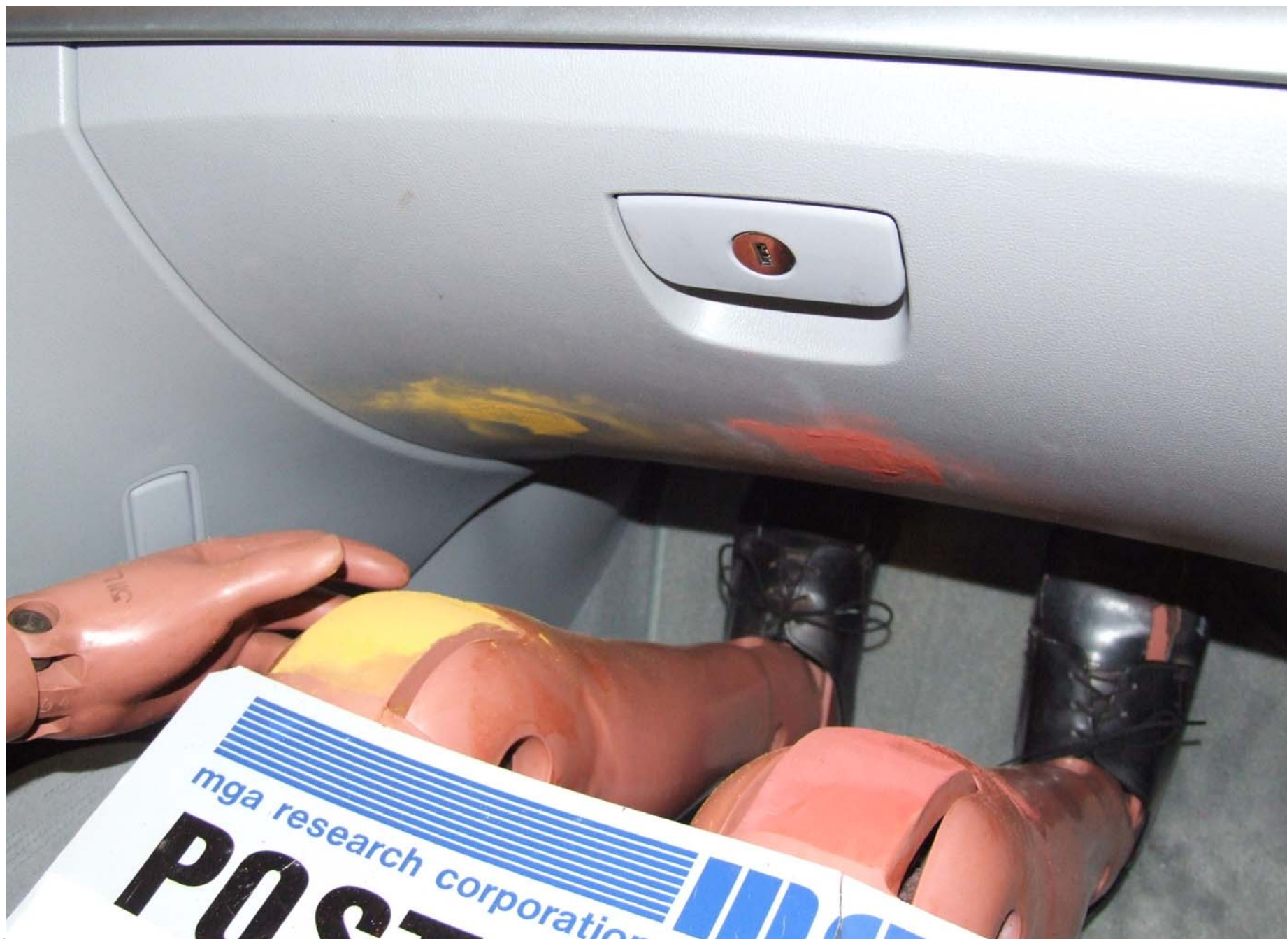
Post-Test Passenger Dummy Knee Contact
