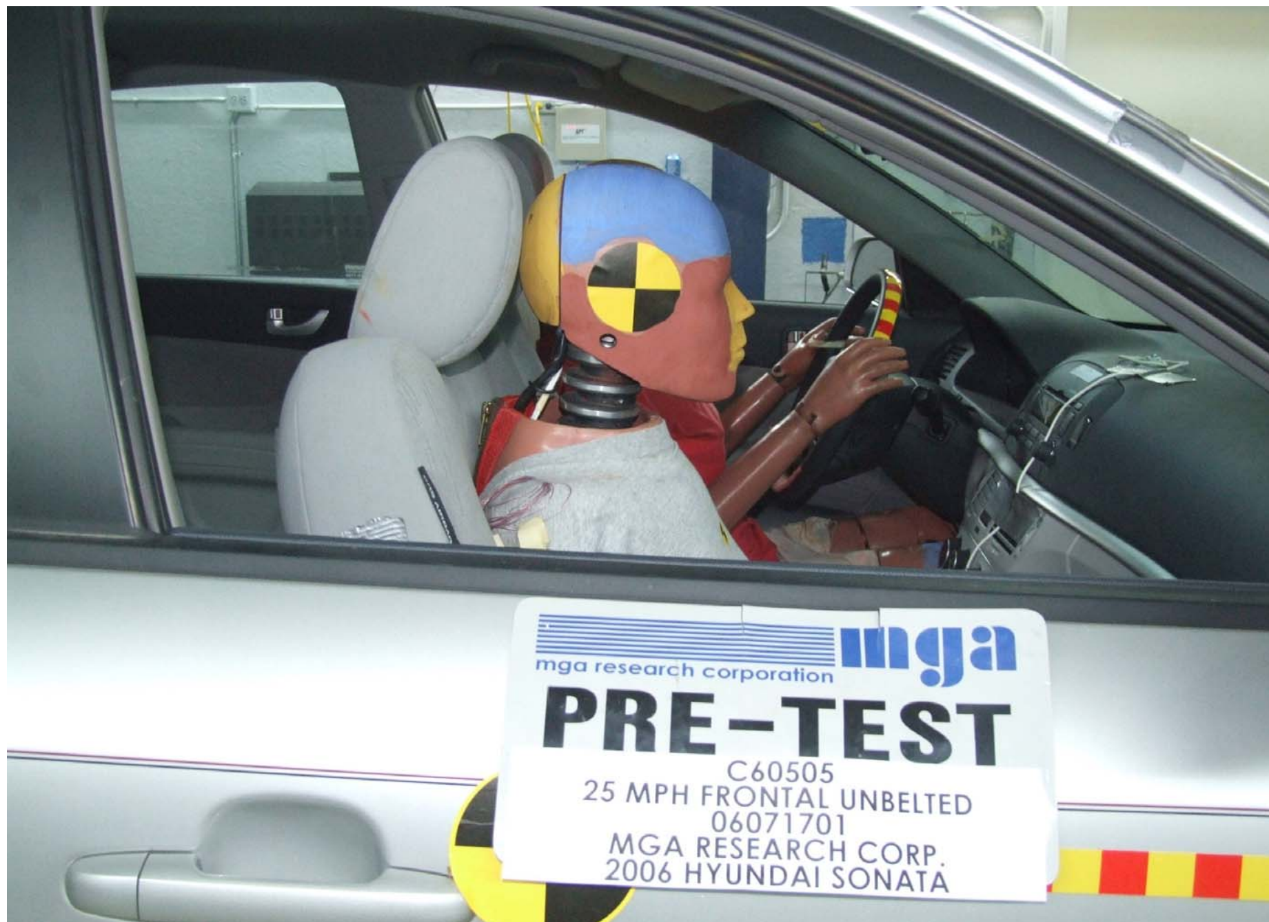
Pre-Test Passenger Dummy Position Right Side View
