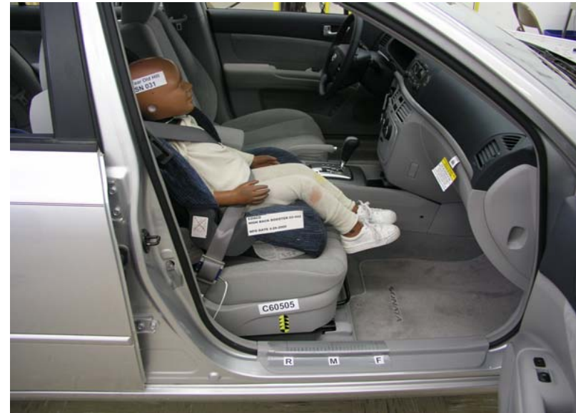
3-Year-Old Cosco High Back Booster With Belt, Rearward Seat Track
