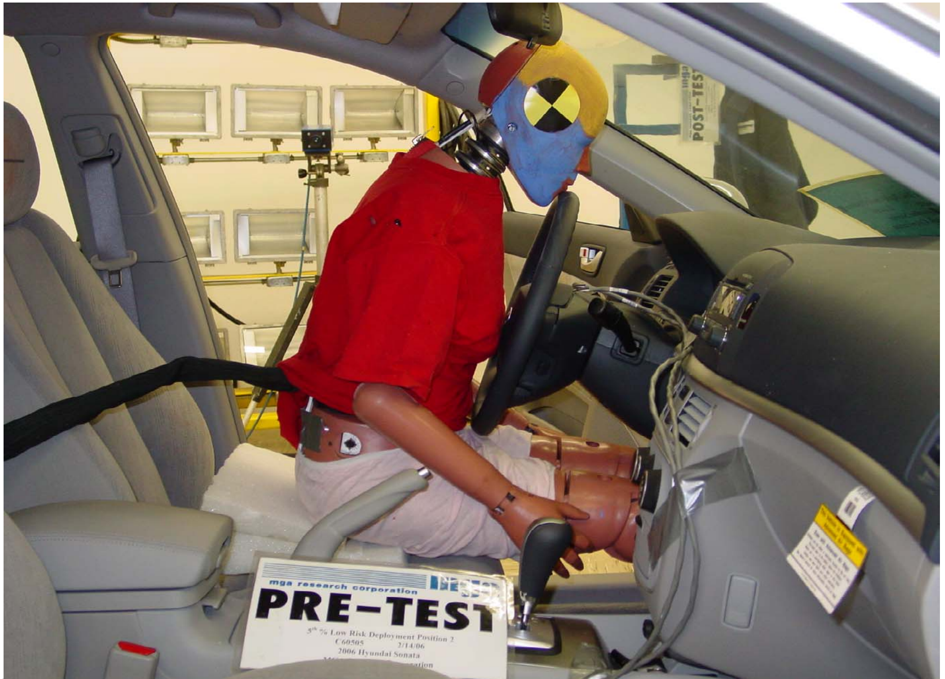
Pre-Test 5th Fem. P2 Driver Dummy Right Side View (Door Open) Trial 1
