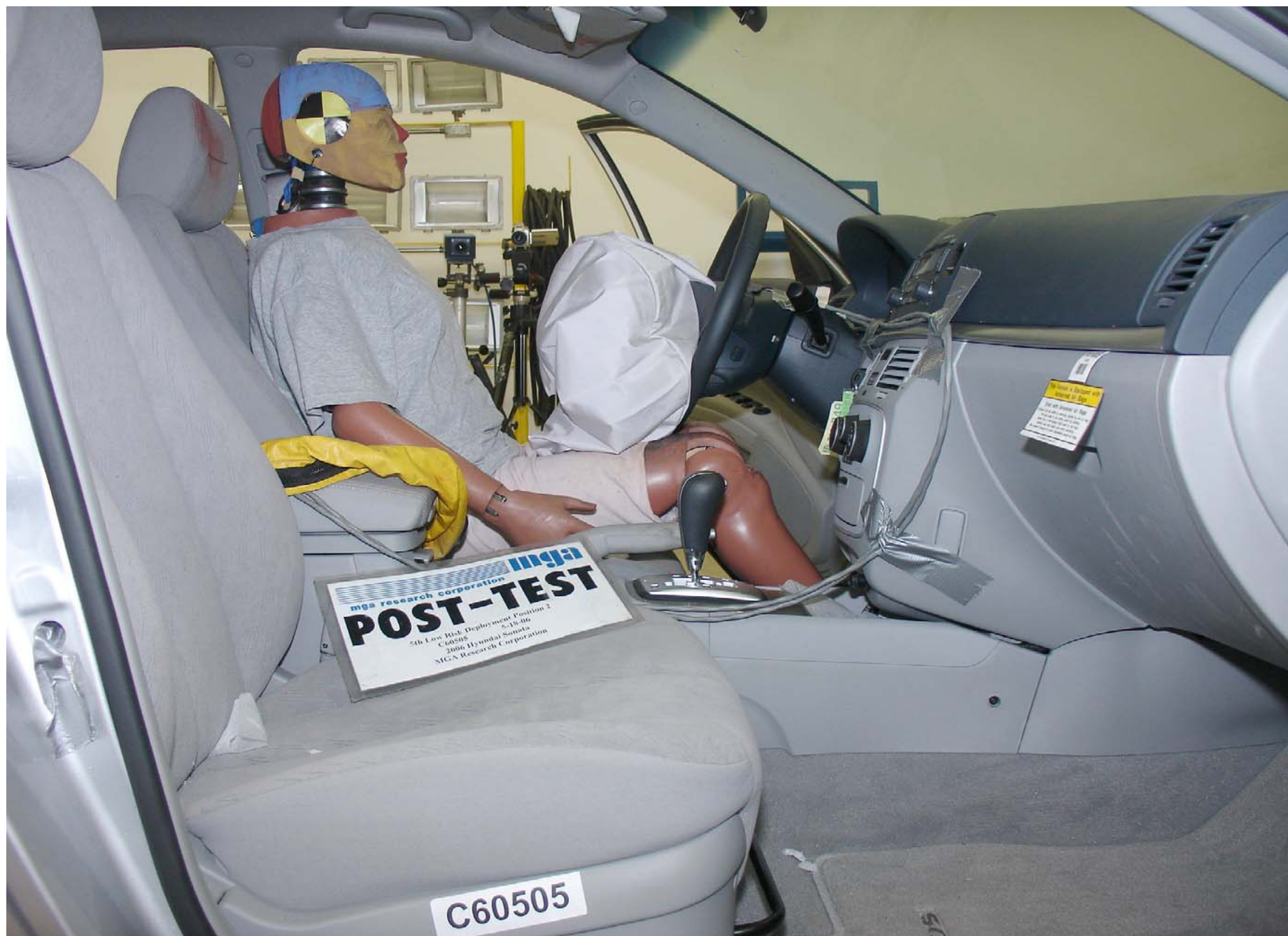
Post-Test 5th Fem. P2 Driver Dummy Right Side View (Door Open) Trial 2
