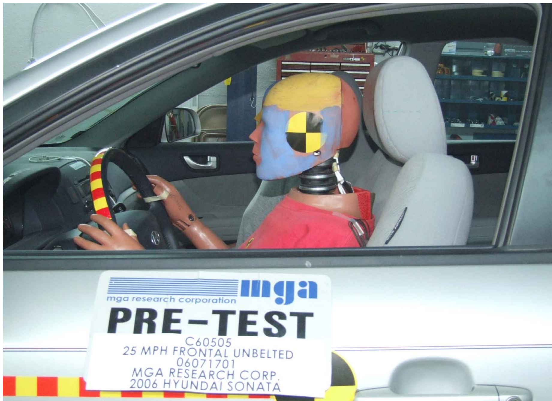
Pre-Test Driver Dummy Position Left Side View
