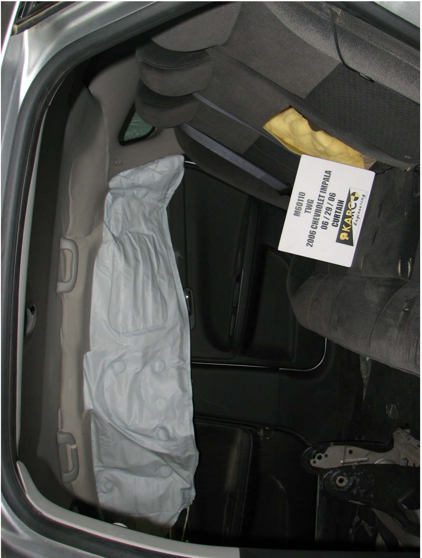
Figure A-9: Post-Test Airbags, Left Side View
