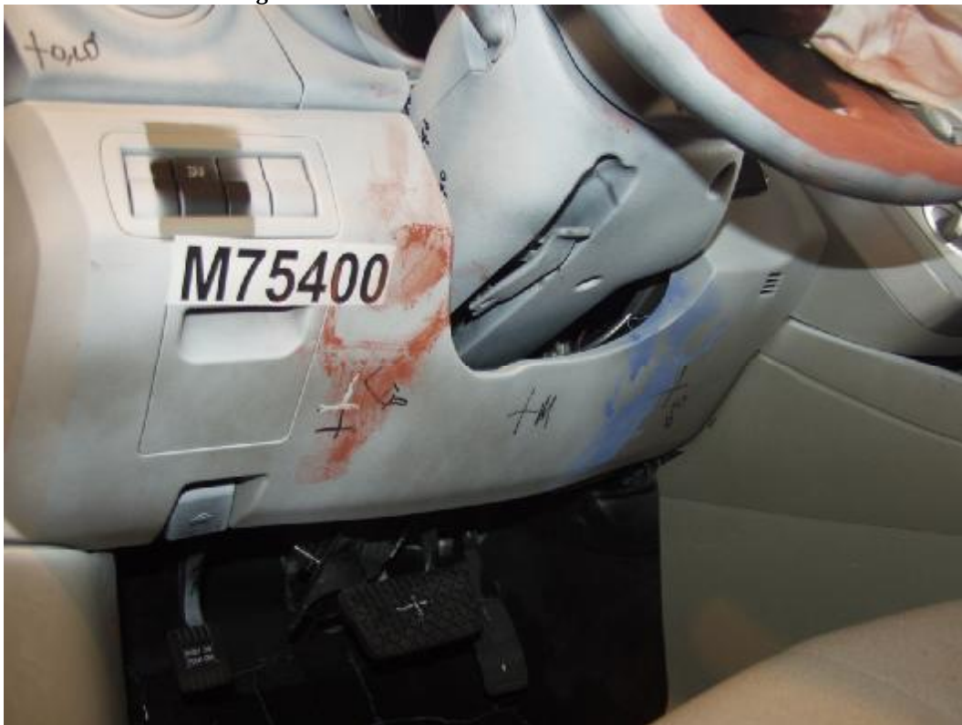
Figure A-39: Post-Test Driver Knee Bolster View
