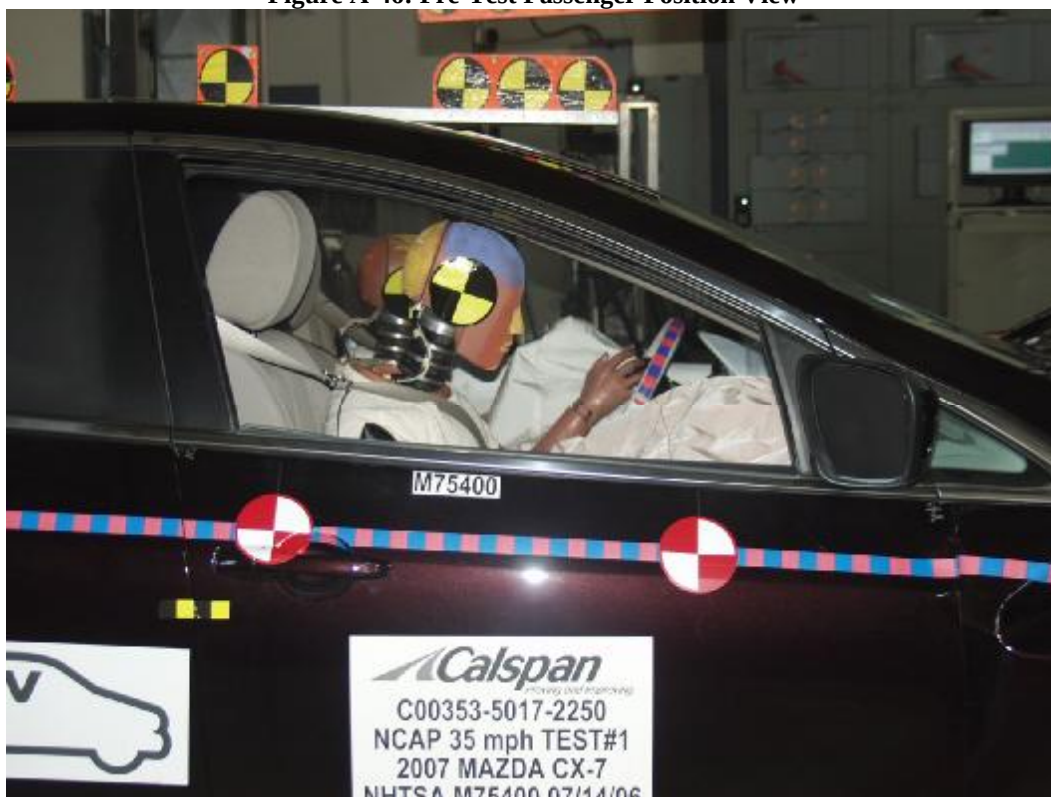
Figure A-47: Post-Test Passenger Position View
