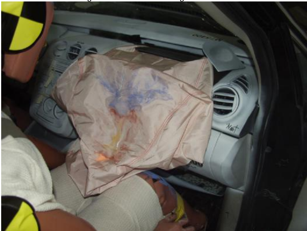
Figure A-57: Post-Test Passenger Contact to Airbag
