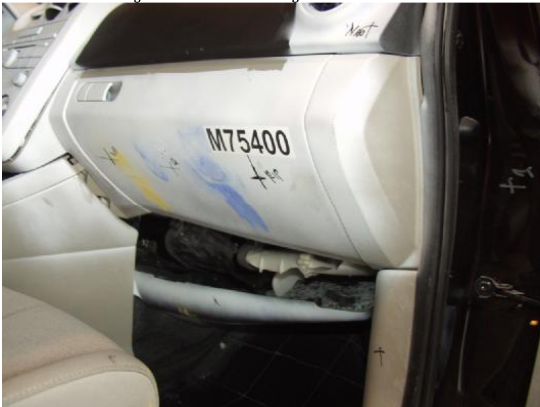
Figure A-53: Post-Test Passenger Knee Bolster View
