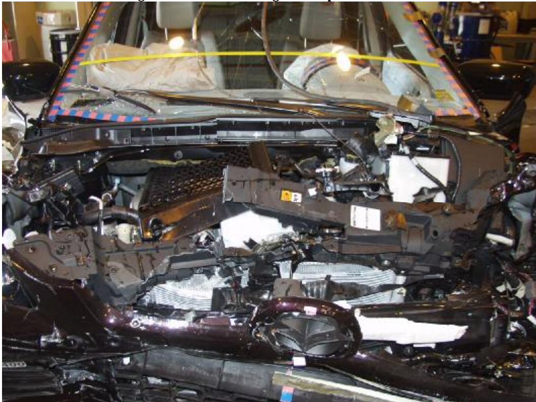
Figure A-21: Post-Test Engine Compartment View
