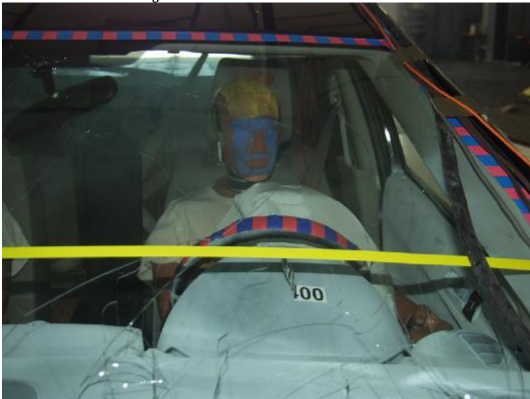
Figure A-31: Post-Test Driver Head Location
