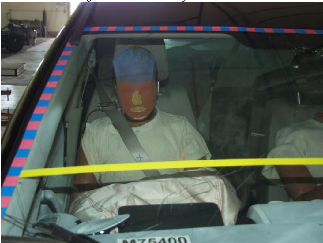
Figure A-45: Post-Test Passenger Head Location
