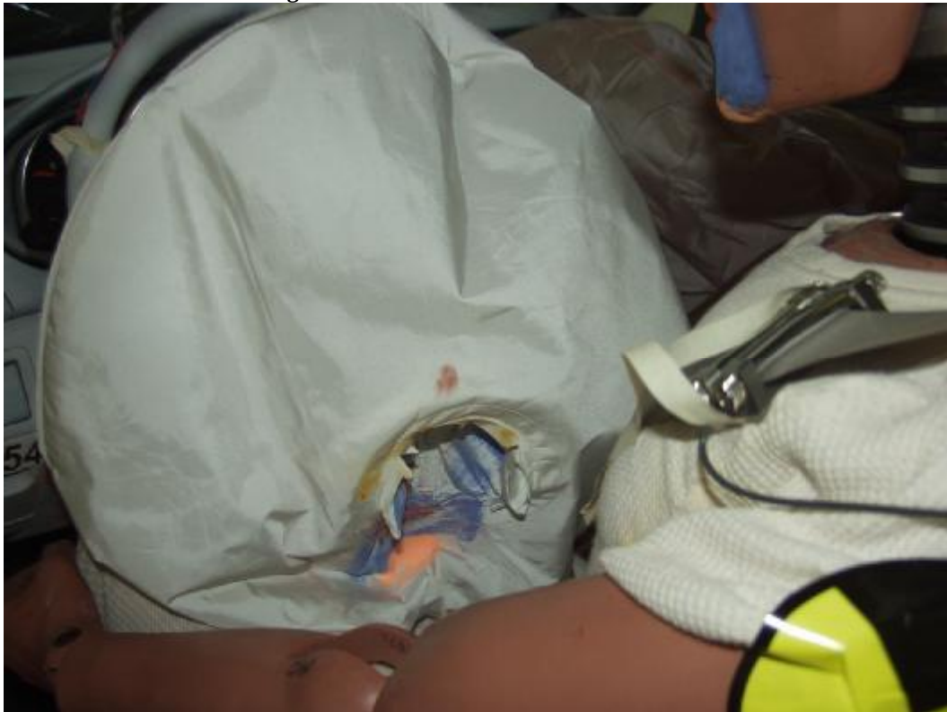
Figure A-43: Post-Test Driver Contact to Airbag
