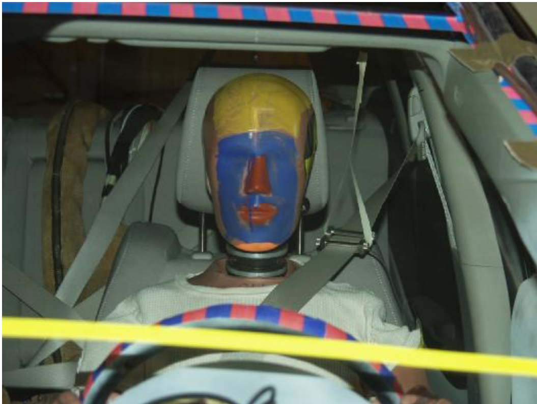
Figure A-30: Pre-Test Driver Head Location
