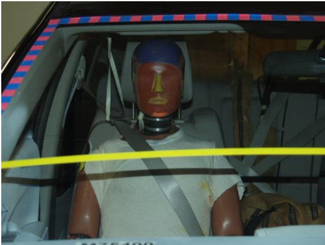
Figure A-44: Pre-Test Passenger Head Location
