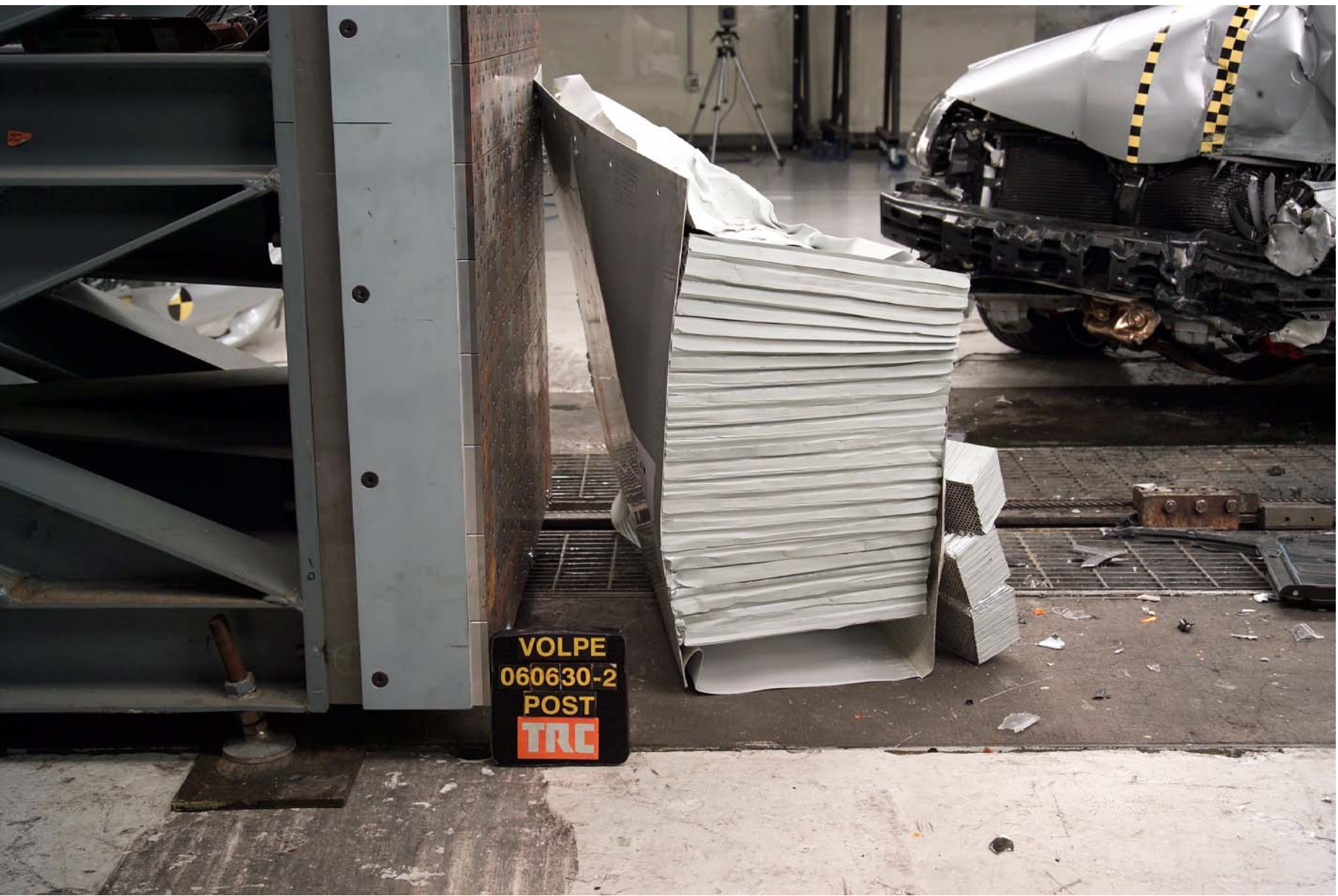
Figure A-64 Post-Test Barrier Left Side View
