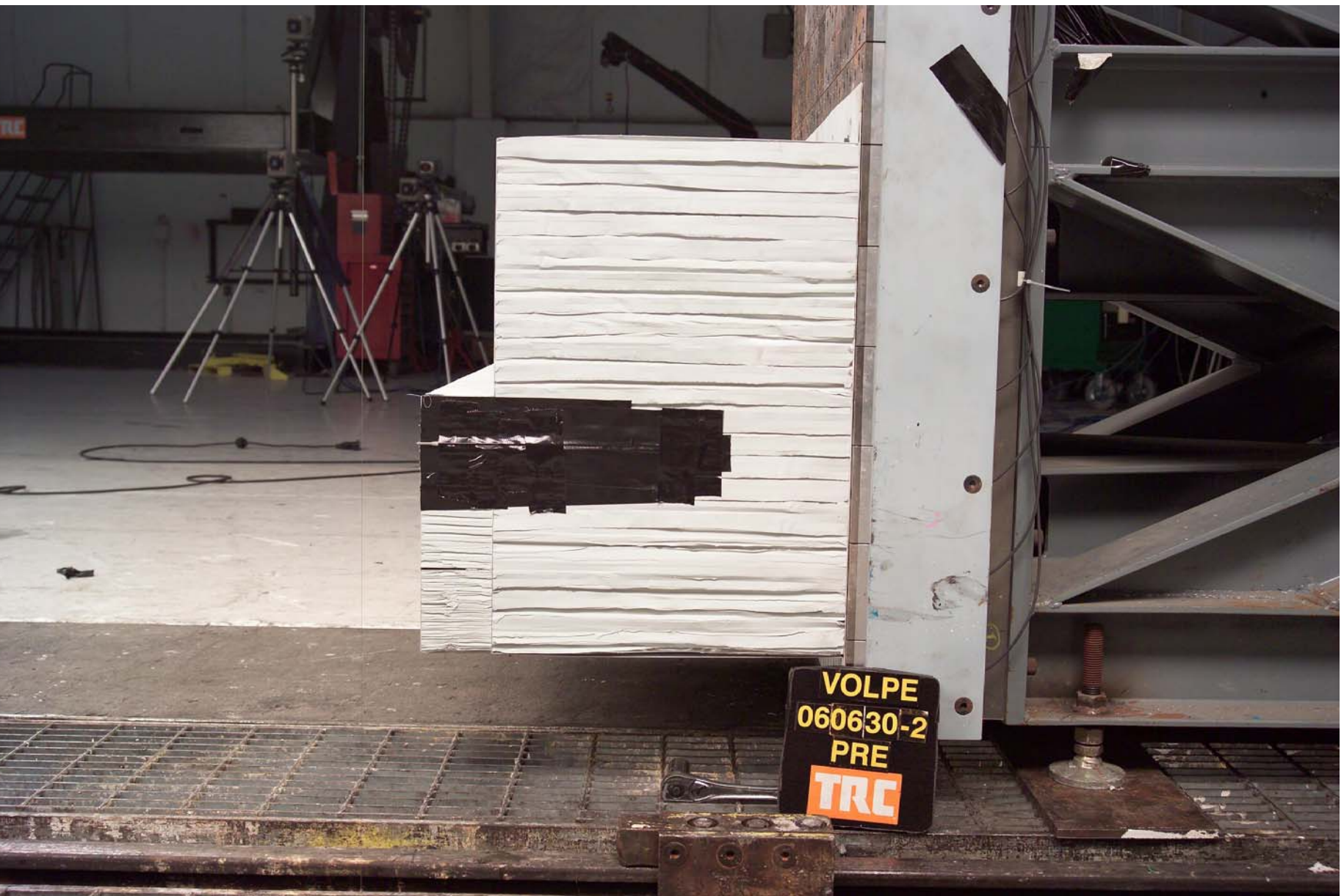
Figure A-65 Pre-Test Barrier Right Side View
