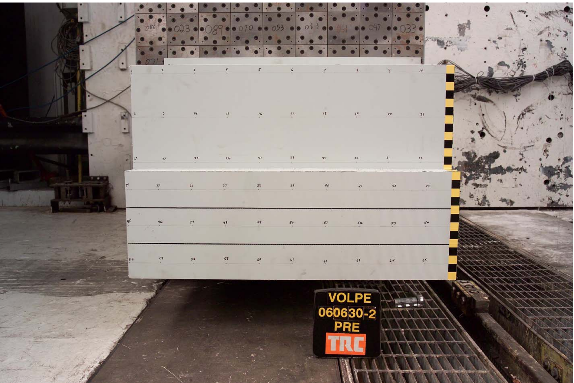
Figure A-61 Pre-Test Barrier Front View
