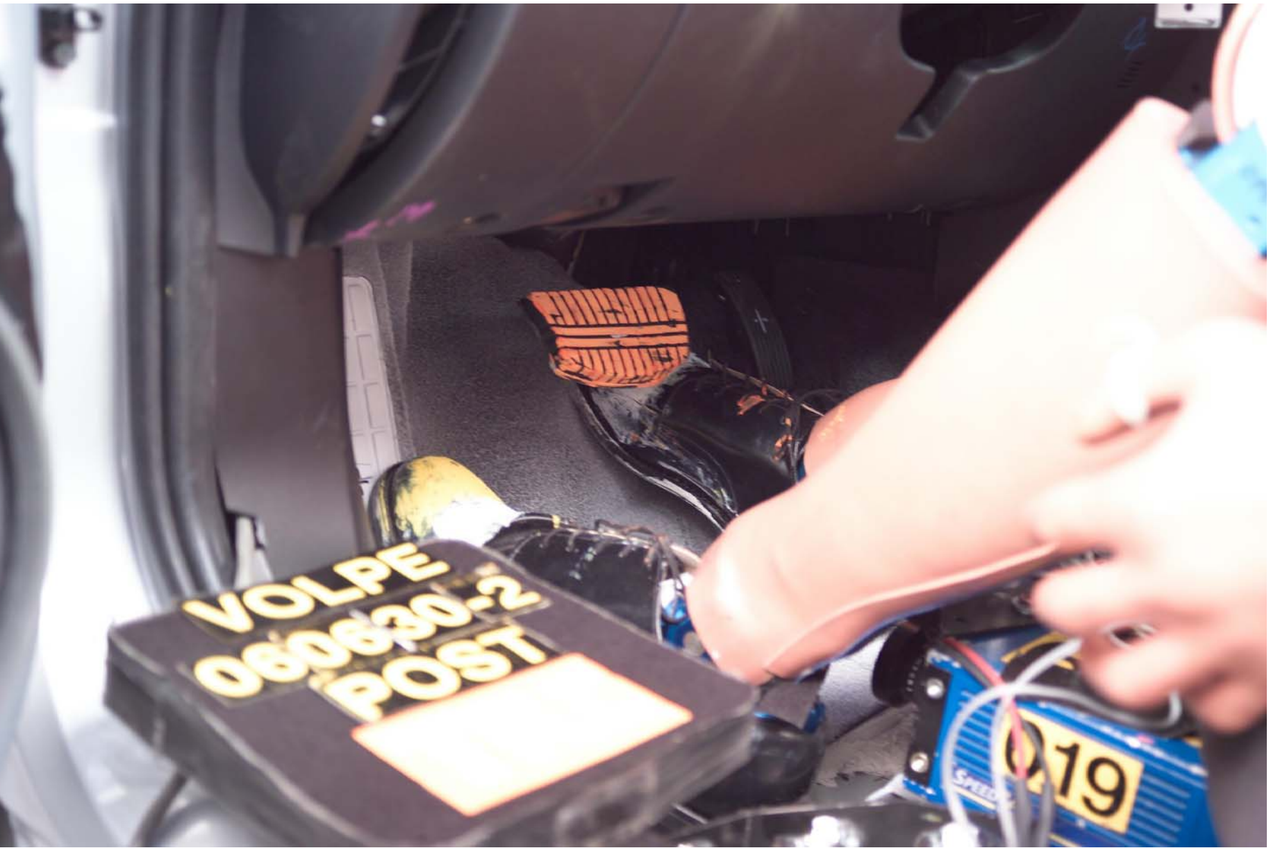
Figure A-54 Post-Test Driver Floorboard Deformation - View 1
