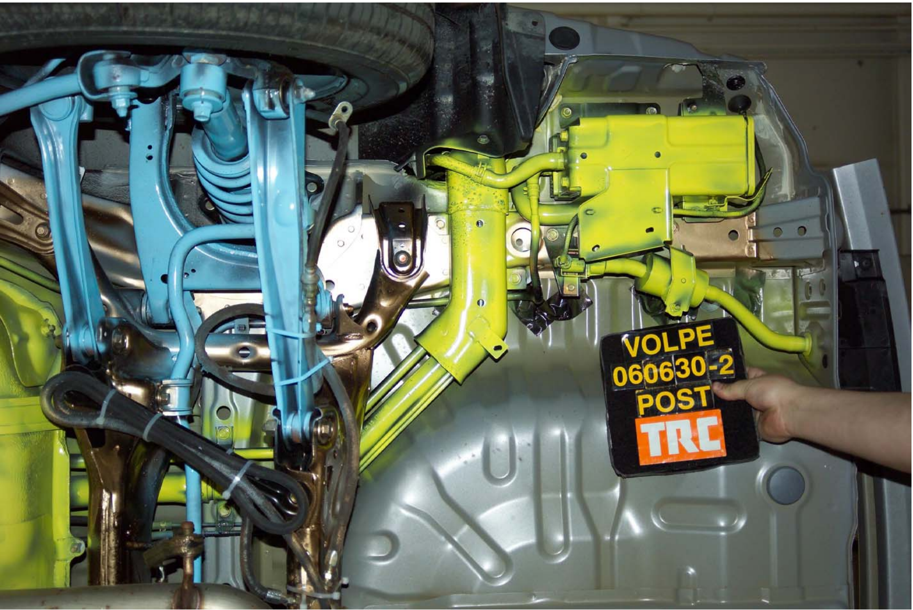
Figure A-32 Post-Test Fuel Filler Neck View
