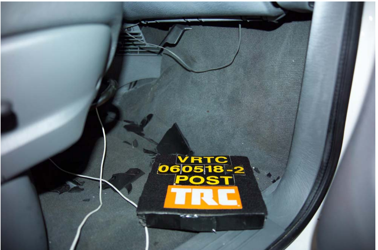
Figure A-74 Post-Test Right Front Passenger Toeboard Deformation View
