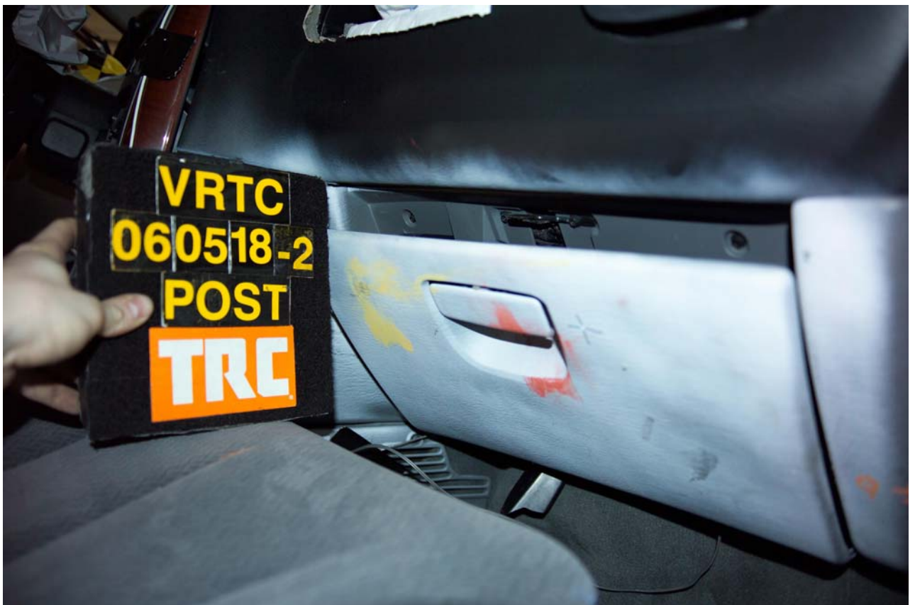
Figure A-72 Post-Test Right Front Passenger Dummy Knee Contact View
