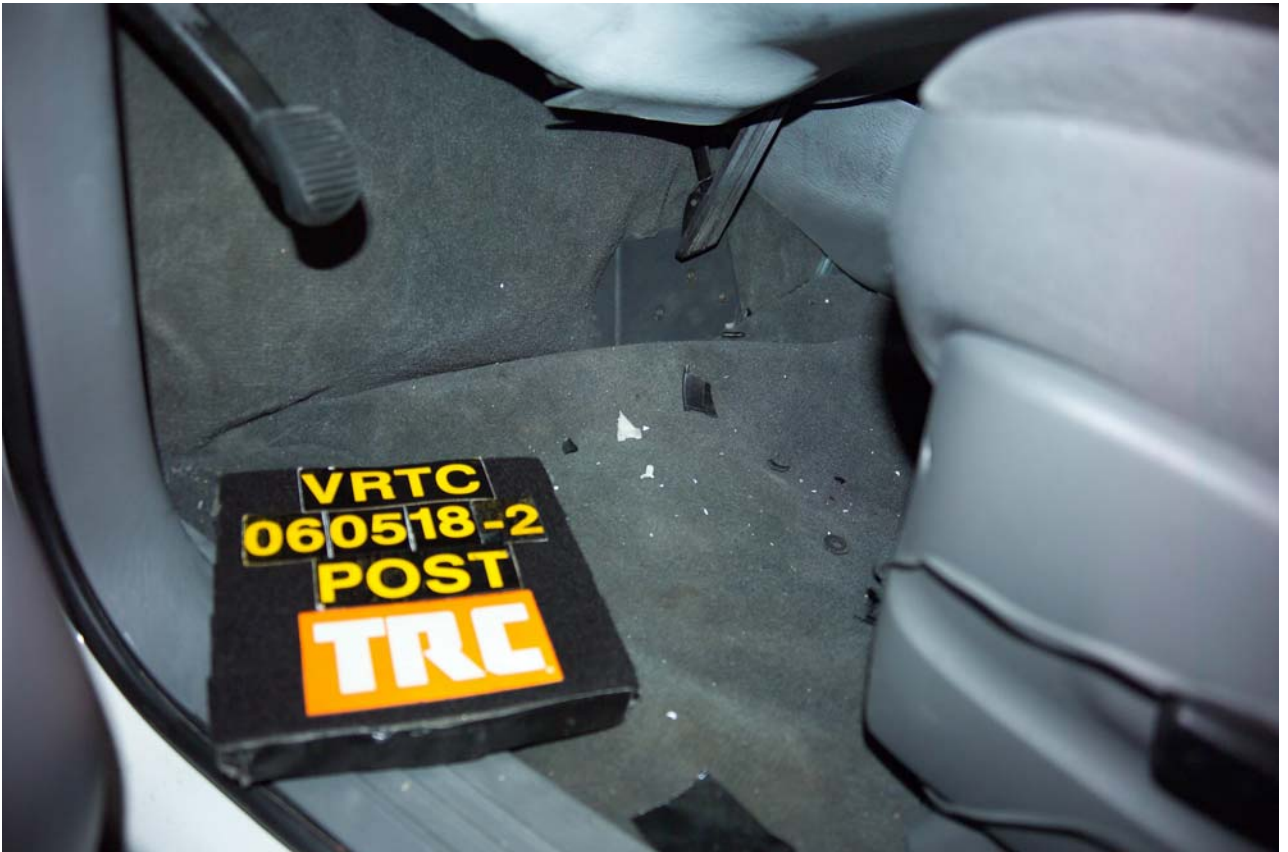
Figure A-66 Post-Test Driver Floorboard Deformation View
