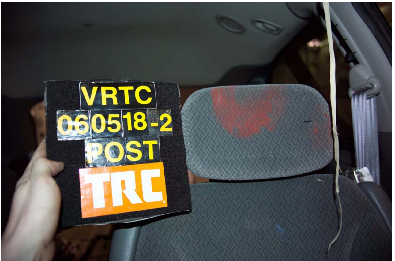
Figure A-76 Post-Test Left Rear Passenger Dummy Head Contact View
