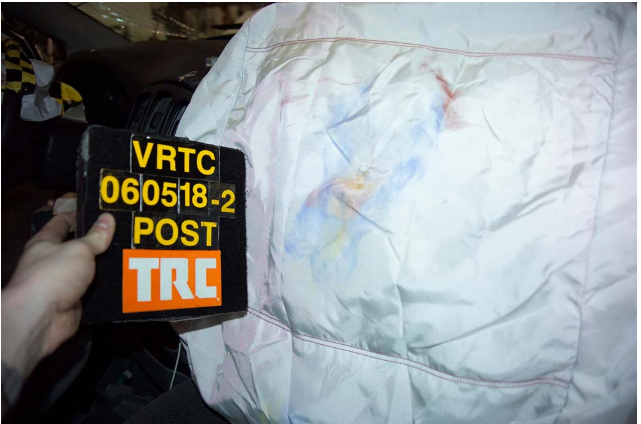
Figure A-70 Post-Test Right Front Passenger Dummy Head Contact - View 1
