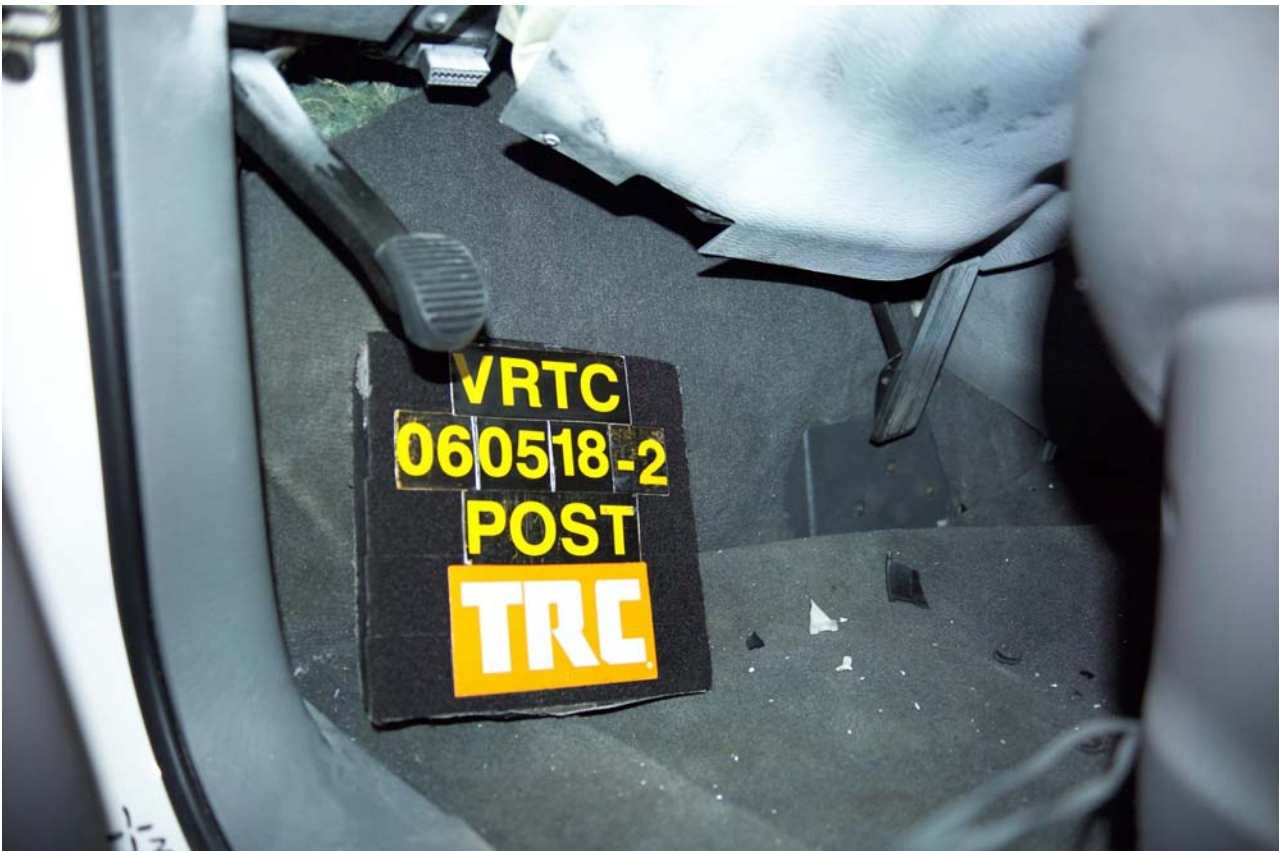
Figure A-67 Post-Test Driver Toeboard Deformation View
