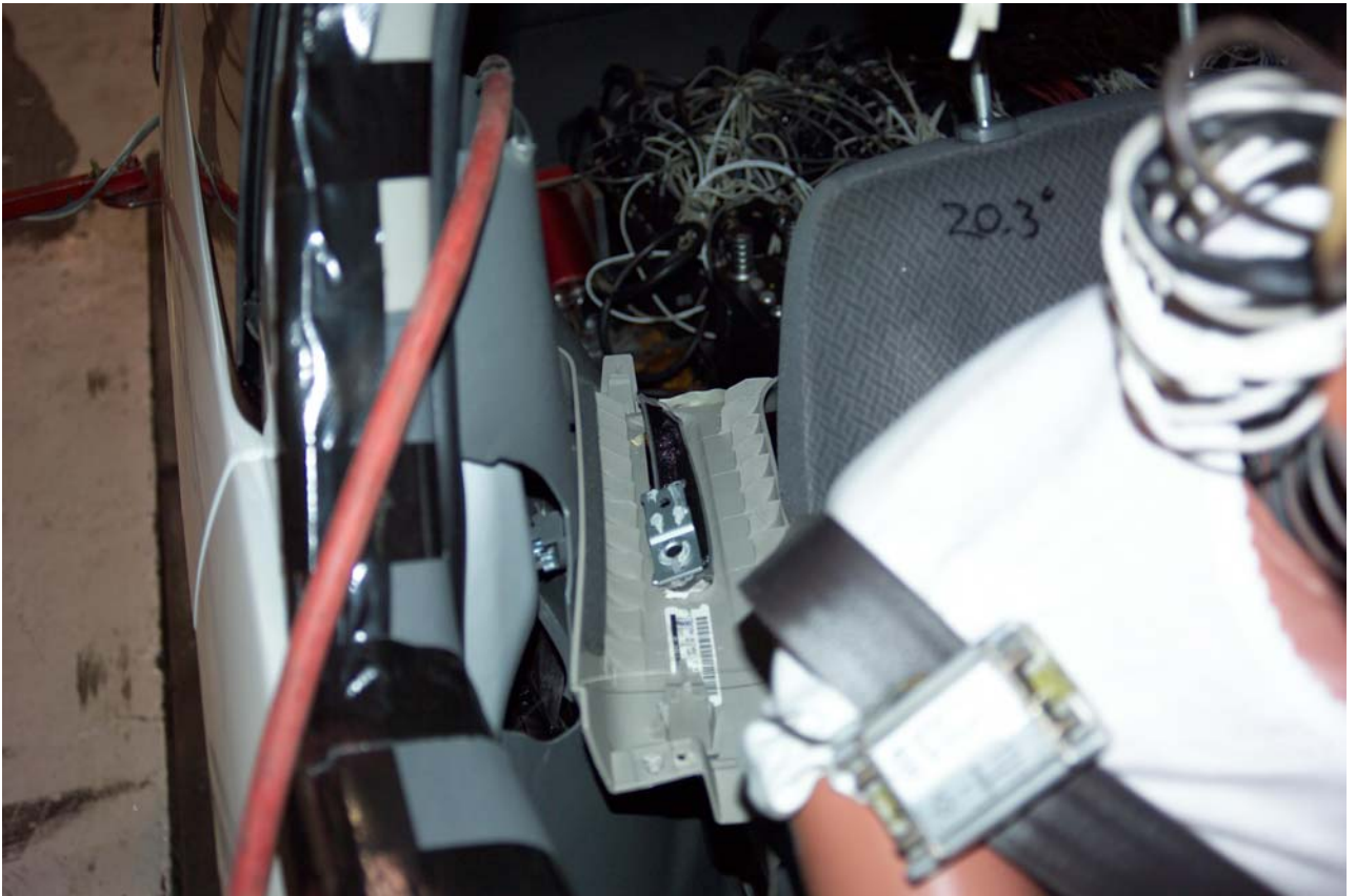
Figure A-79 Post-Test Right Rear Passenger D-Ring Damage - View 1
