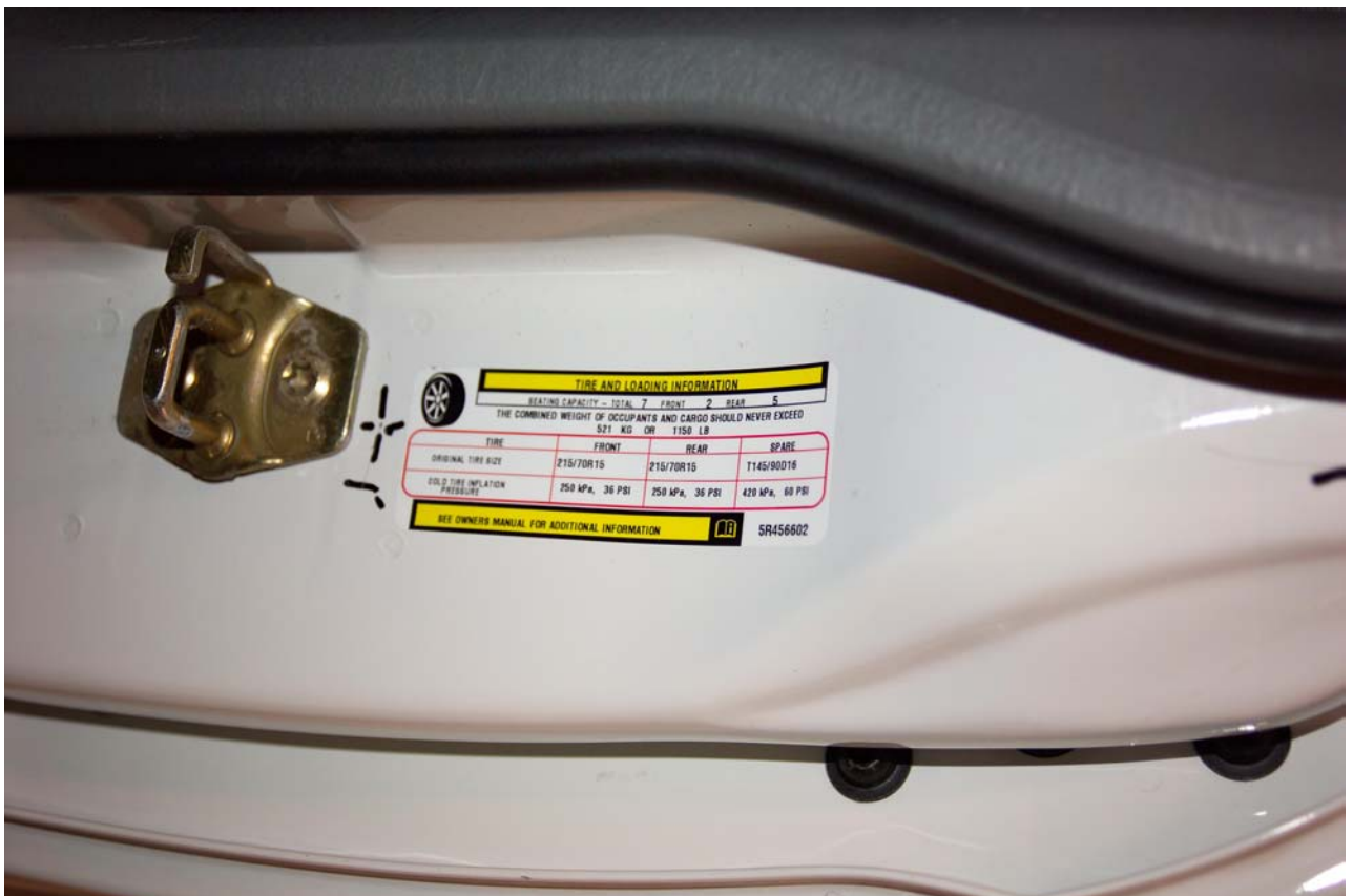
Figure A-84 Recommended Tire Pressure Label View
