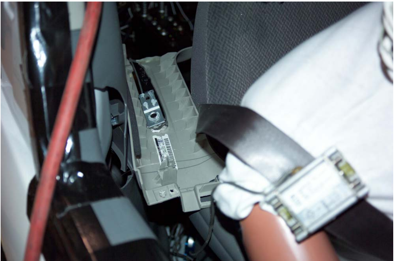
Figure A-80 Post-Test Right Rear Passenger D-Ring Damage - View 2
