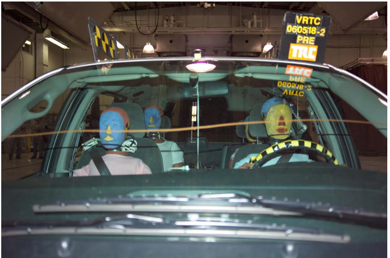
Figure A-32 Pre-Test Driver and Passenger Dummies through Windshield View
