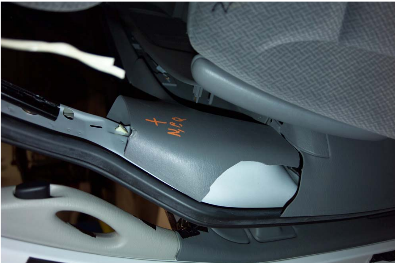
Figure A-82 Post-Test Right Rear Passenger Side Panel Damage View
