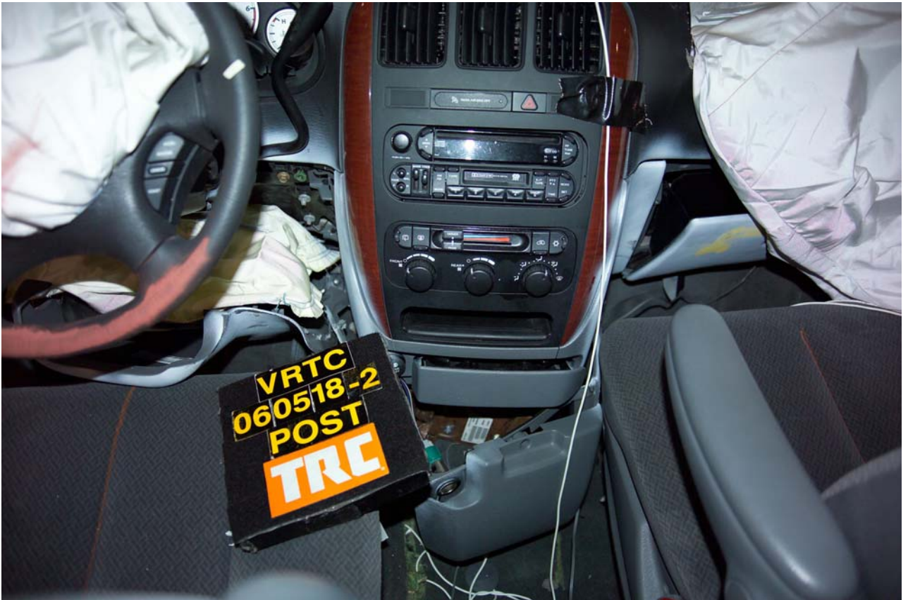
Figure A-68 Post-Test Center Dash Panel Deformation View
