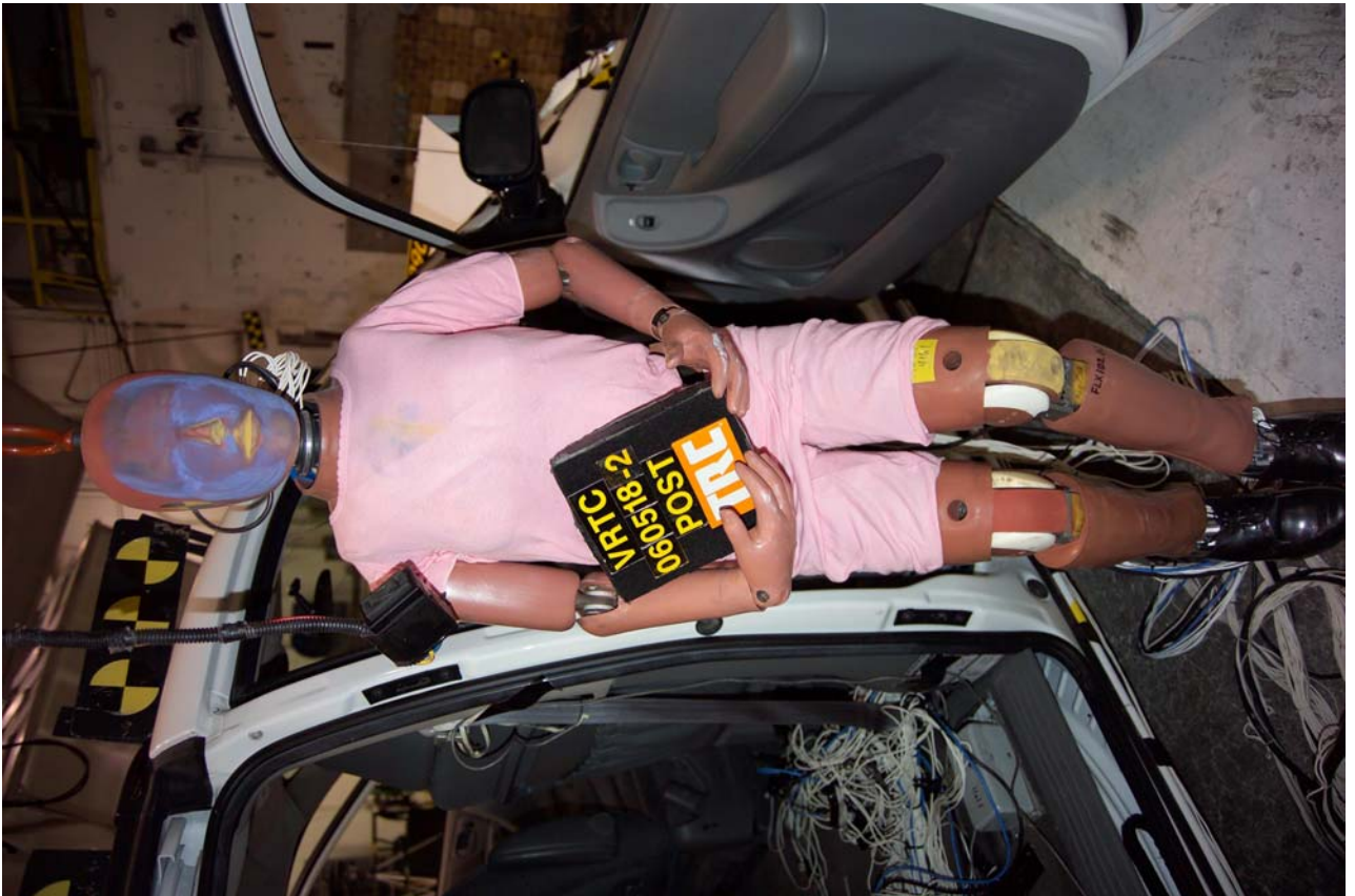
Figure A-69 Post-Test Right Front Passenger Dummy Overall Contact View
