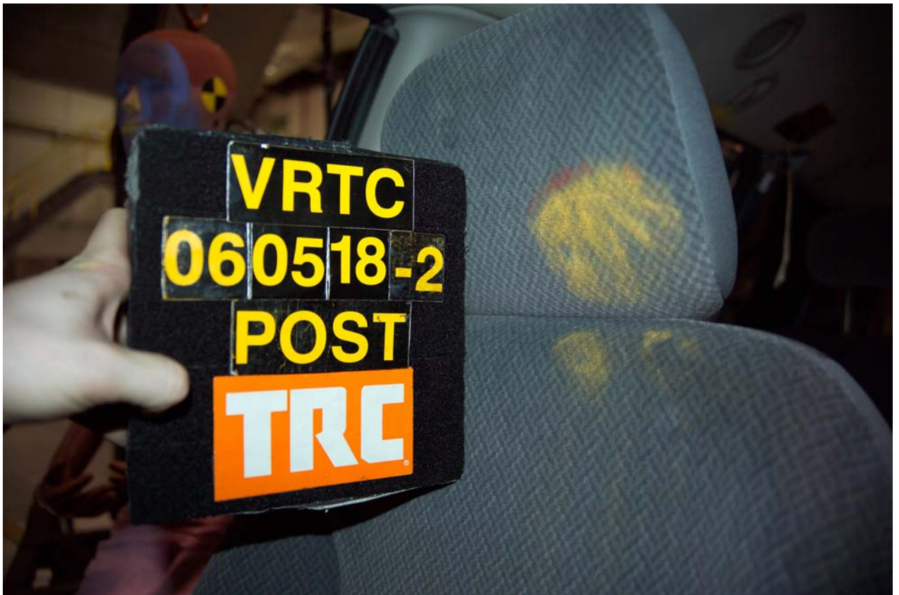
Figure A-71 Post-Test Right Front Passenger Dummy Head Contact - View 2
