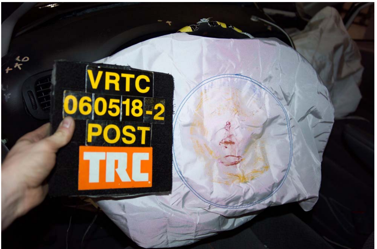
Figure A-63 Post-Test Driver Dummy Head Contact - View 1
