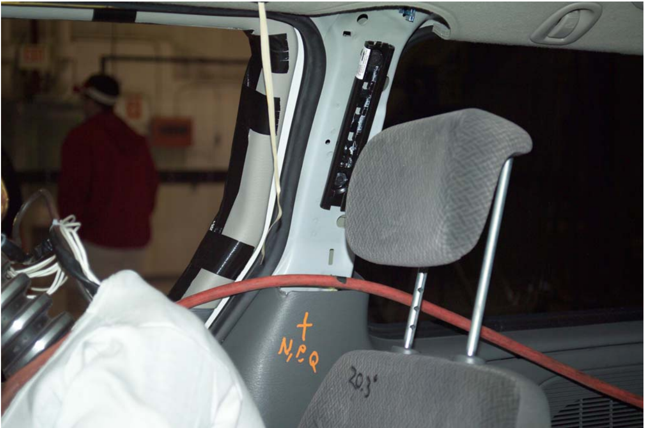
Figure A-81 Post-Test Right Rear Passenger D-Ring Damage - View 3
