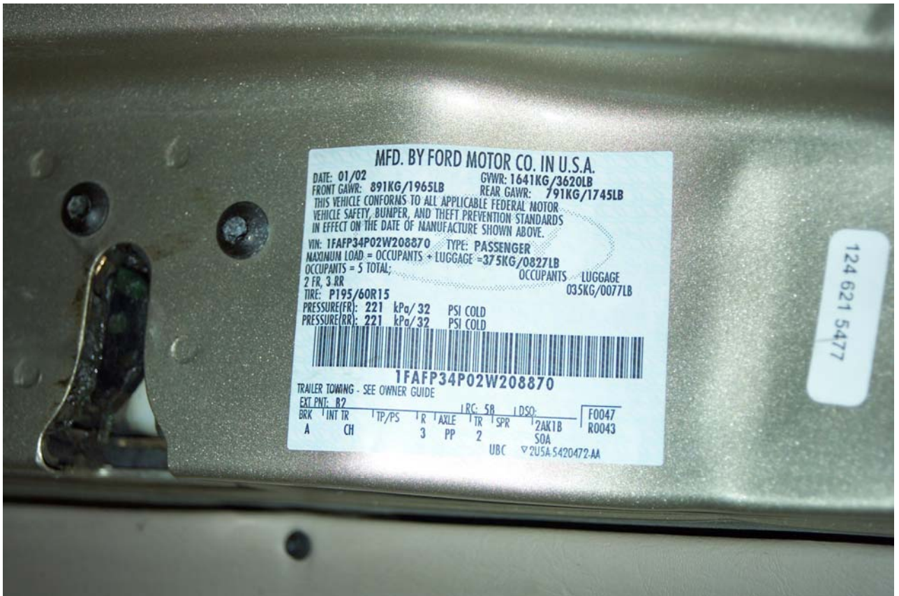
Figure A-65 Vehicle Certification and Tire Information Label View
