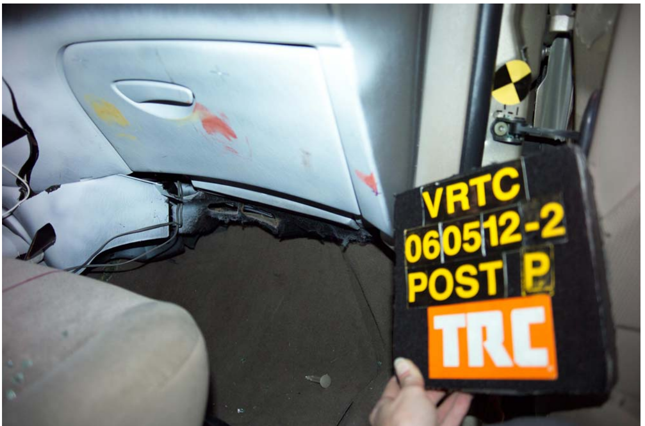
Figure A-64 Post-Test Passenger Toeboard Deformation View
