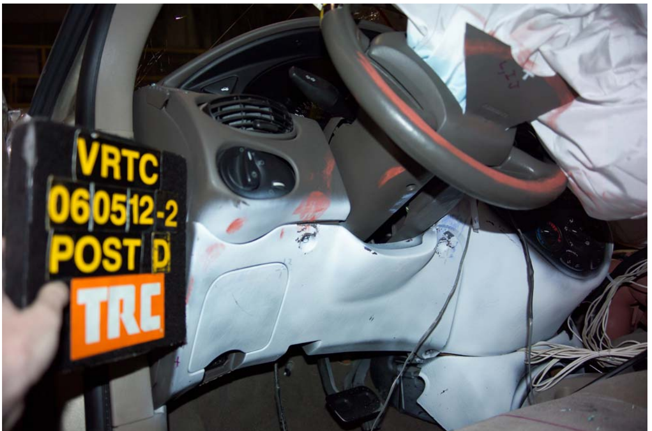
Figure A-54 Post-Test Driver Dummy Knee Contact View
