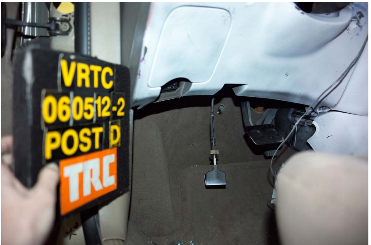
Figure A-57 Post-Test Driver Toeboard Deformation View
