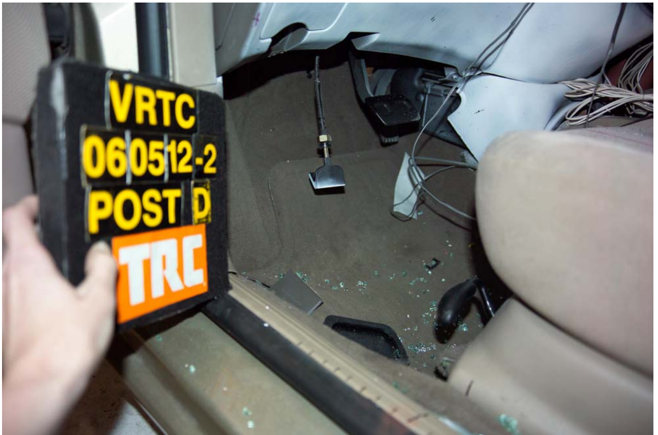
Figure A-56 Post-Test Driver Floorboard Deformation View
