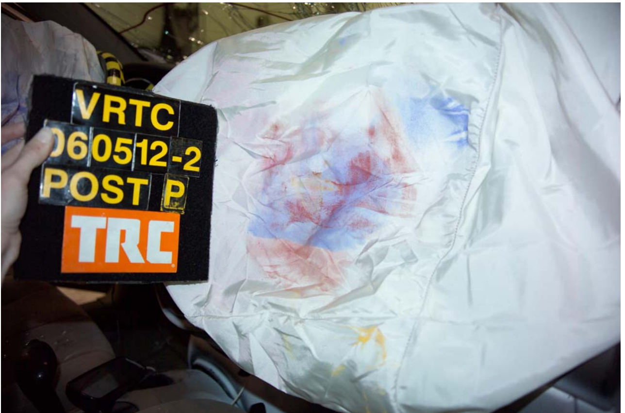
Figure A-59 Post-Test Passenger Dummy Head Contact - View 1
