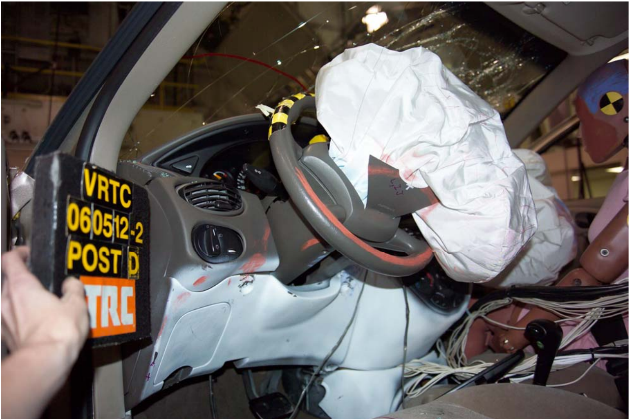
Figure A-55 Post-Test Driver Dash Panel Deformation View
