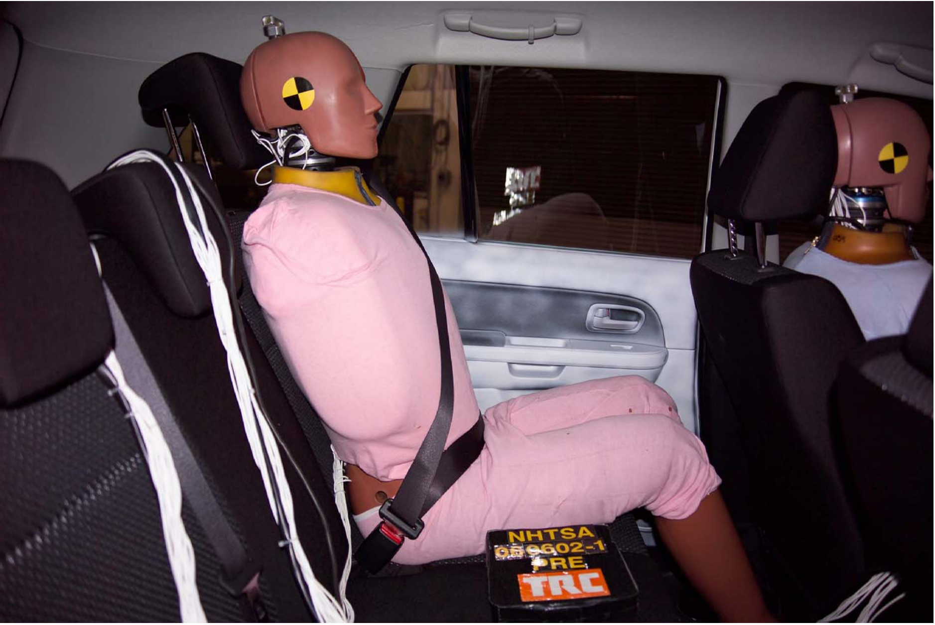
Figure A-43 Pre-Test Right Occupant Compartment View of Rear SID HIII
