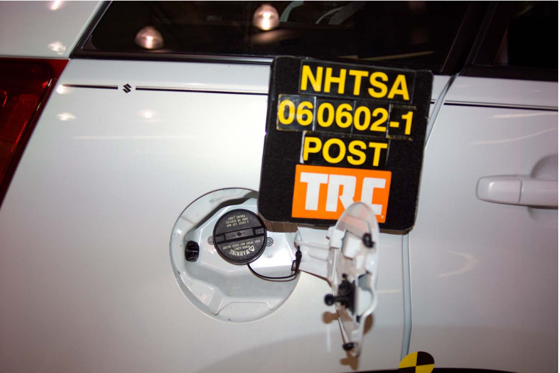
Figure A-80 Post-Test Fuel Cap
