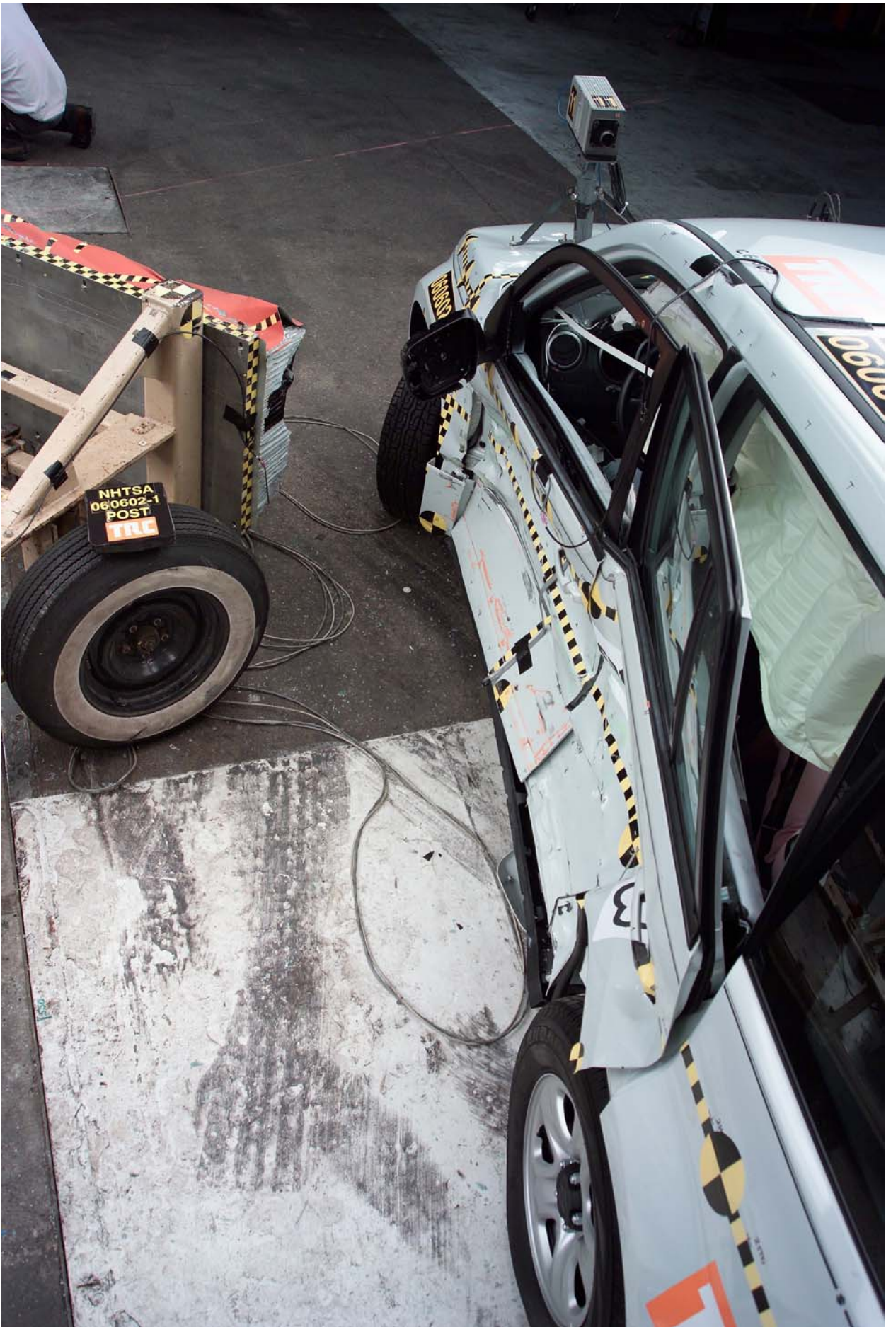
Figure A-40 Post-Test Overhead View of MDB and Vehicle
