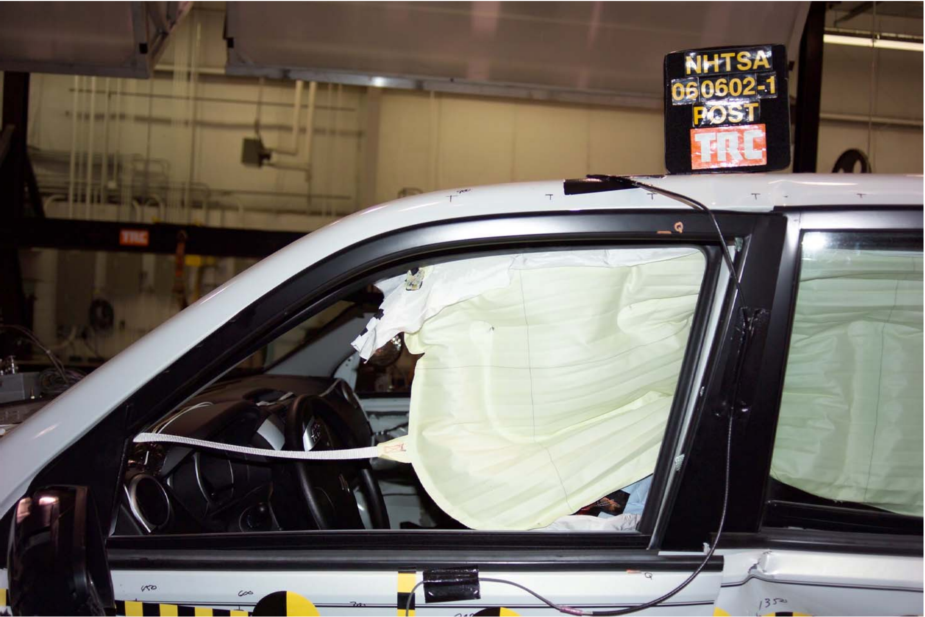
Figure A-46 Post-Test Left View of Front SID HIII
