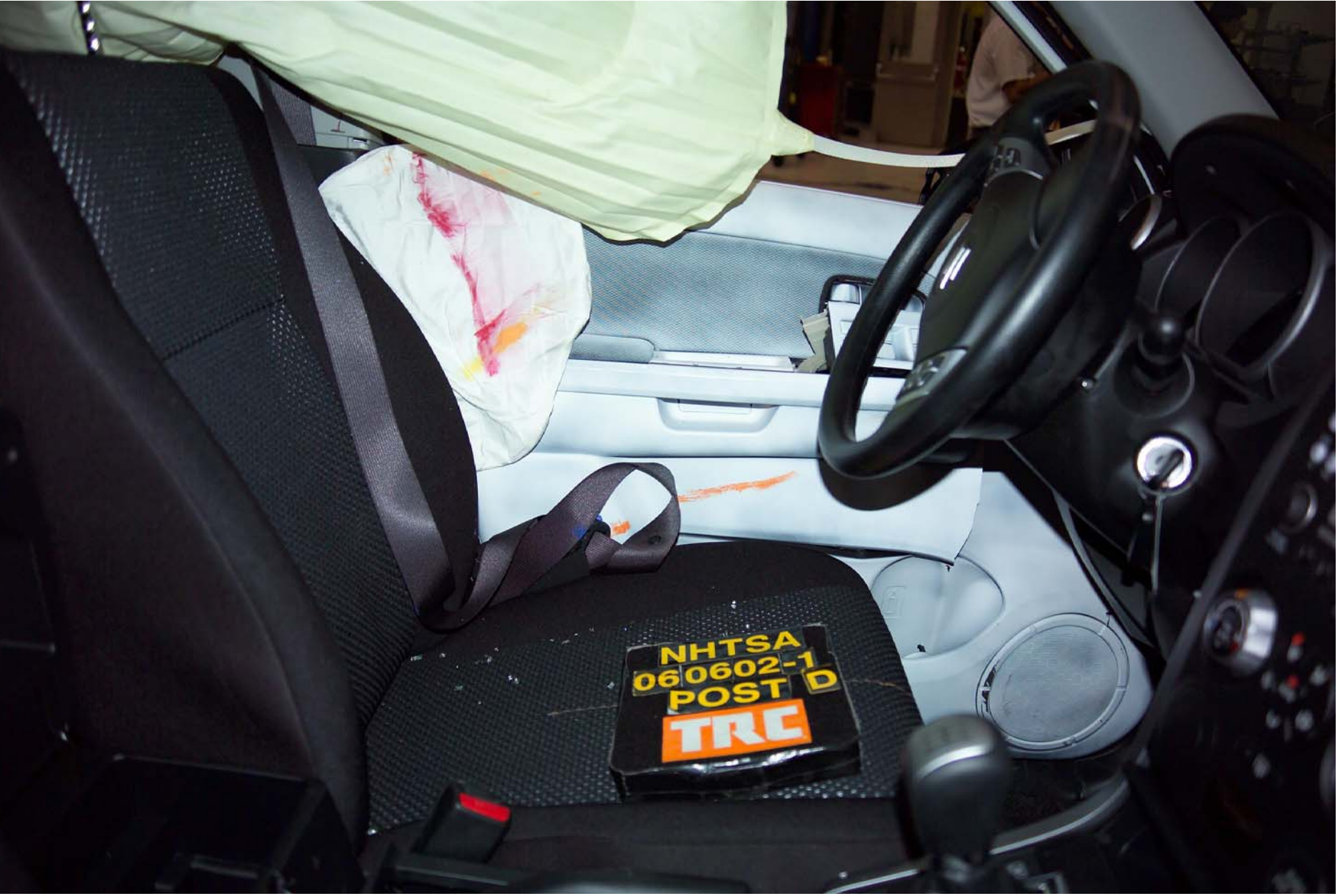
Figure A-56 Post-Test Interior of Front Door Showing SID HIII Impact Locations
