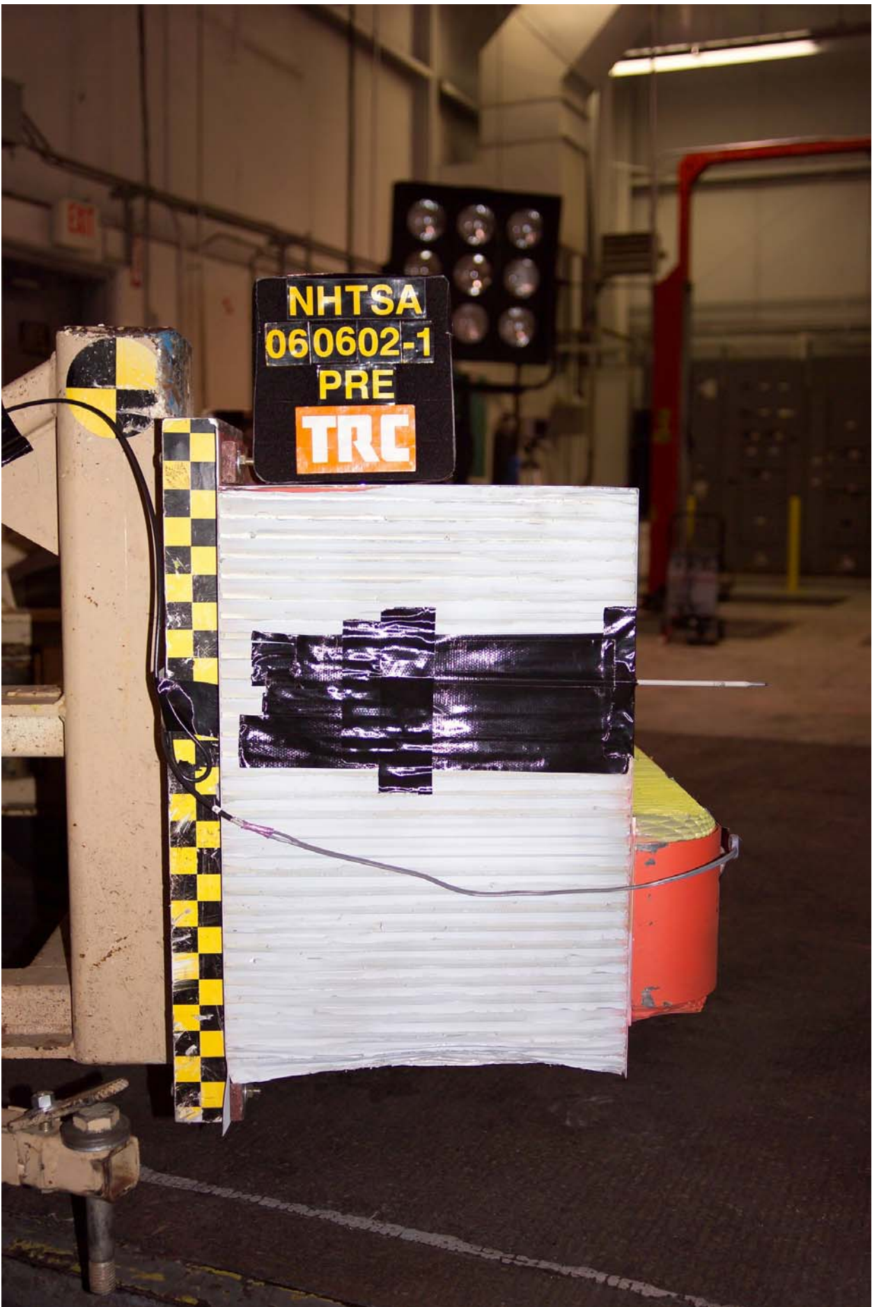
Figure A-29 Pre-Test Right Side View of Impactor
