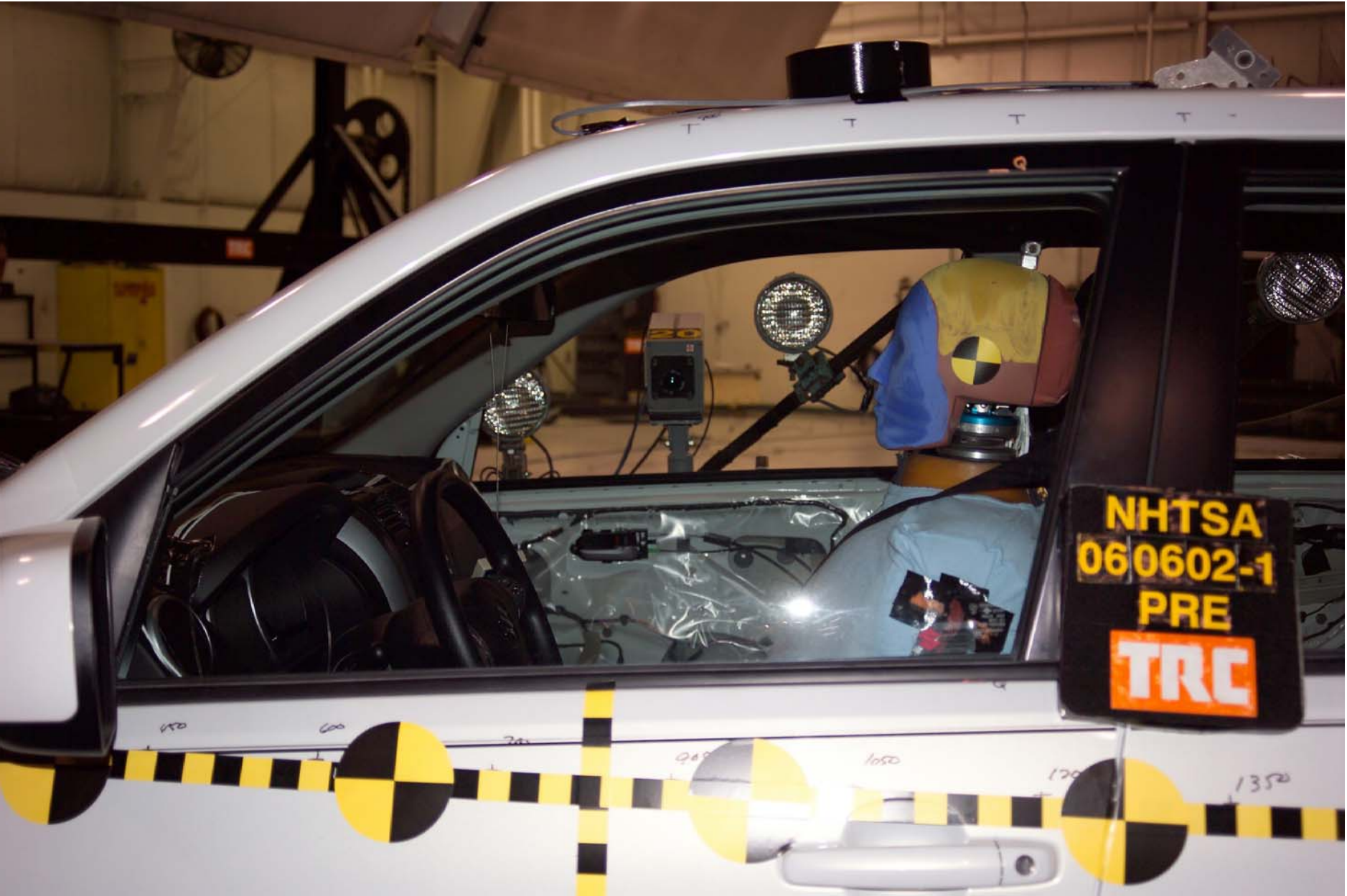
Figure A-45 Pre-Test Left View of Front SID HIII
