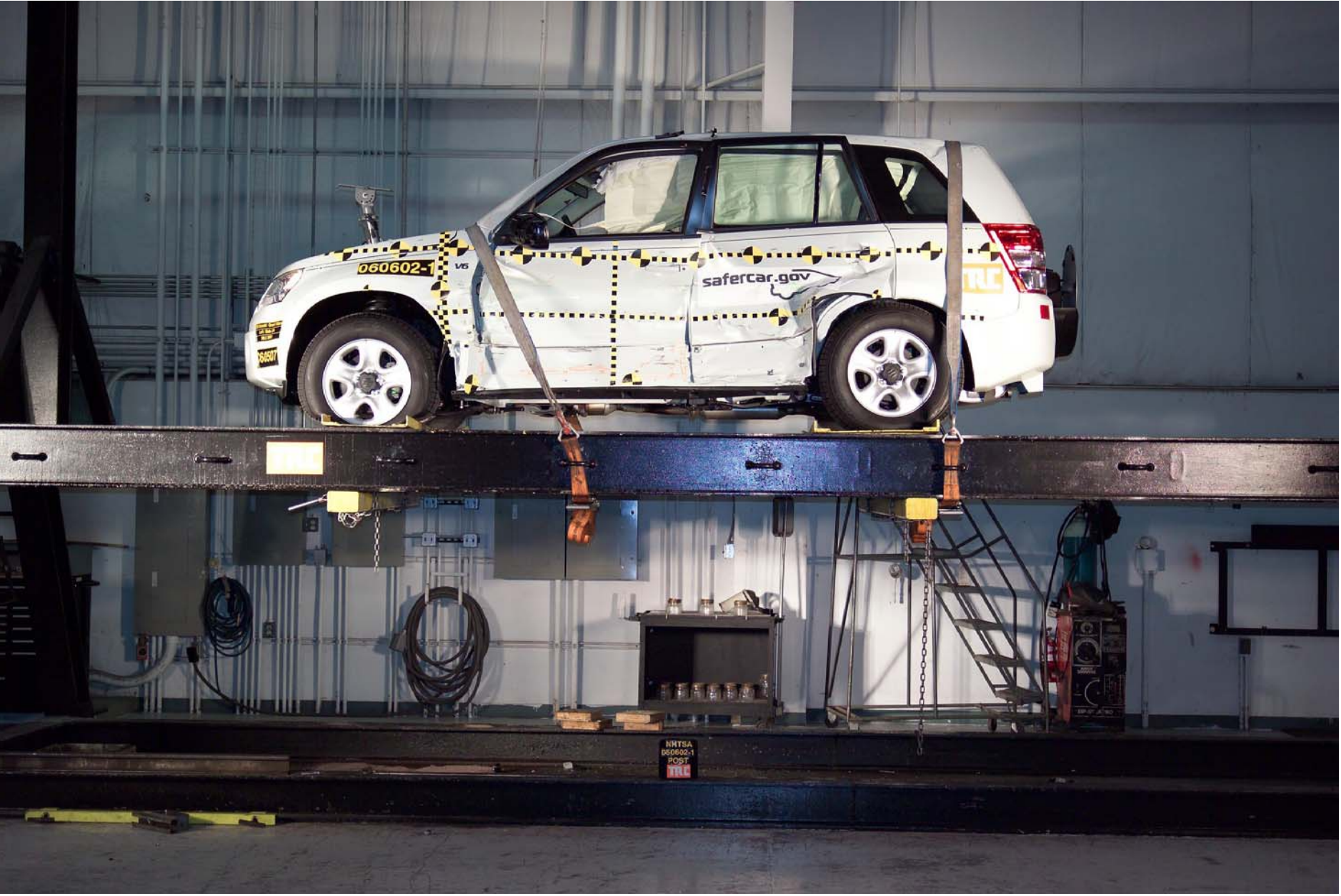
Figure A-84 FMVSS 301 Rollover View at 360°
