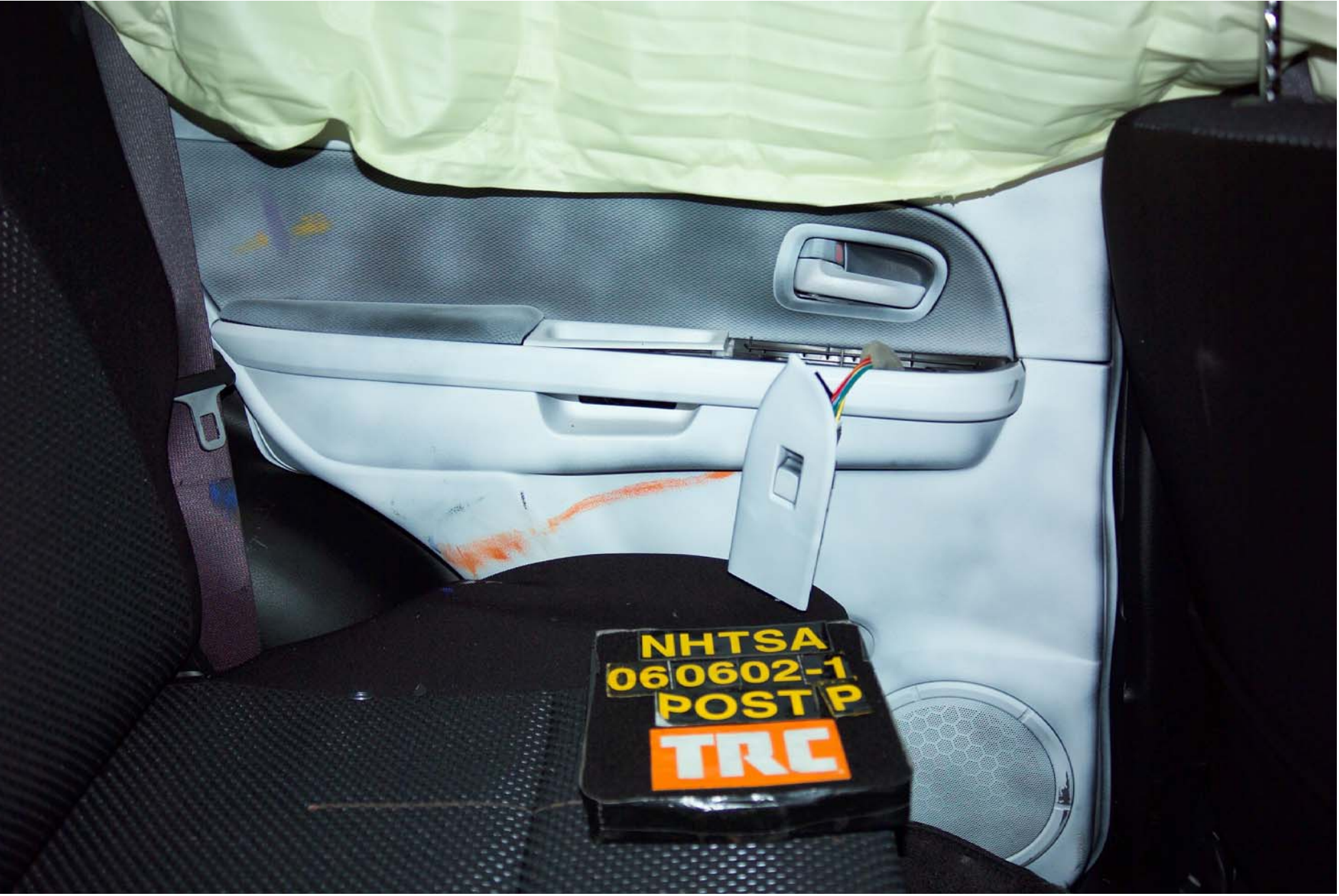
Figure A-61 Post-Test Interior of Rear Panel Showing SID HIII Impact Locations
