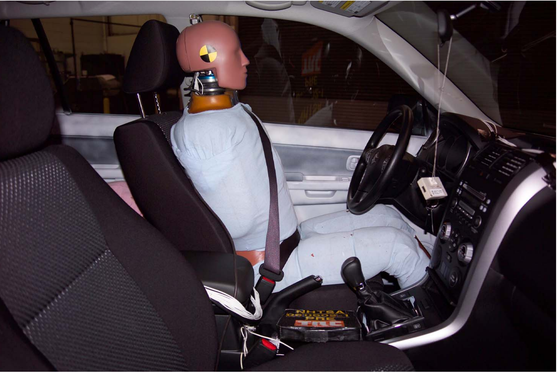
Figure A-41 Pre-Test Right Occupant Compartment View of Front SID HIII
