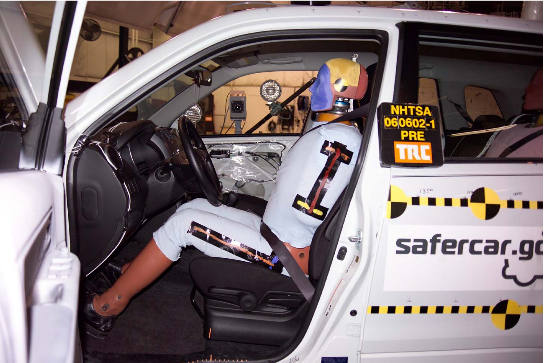
Figure A-47 Pre-Test Left View of Front SID HIII and Belt Position
