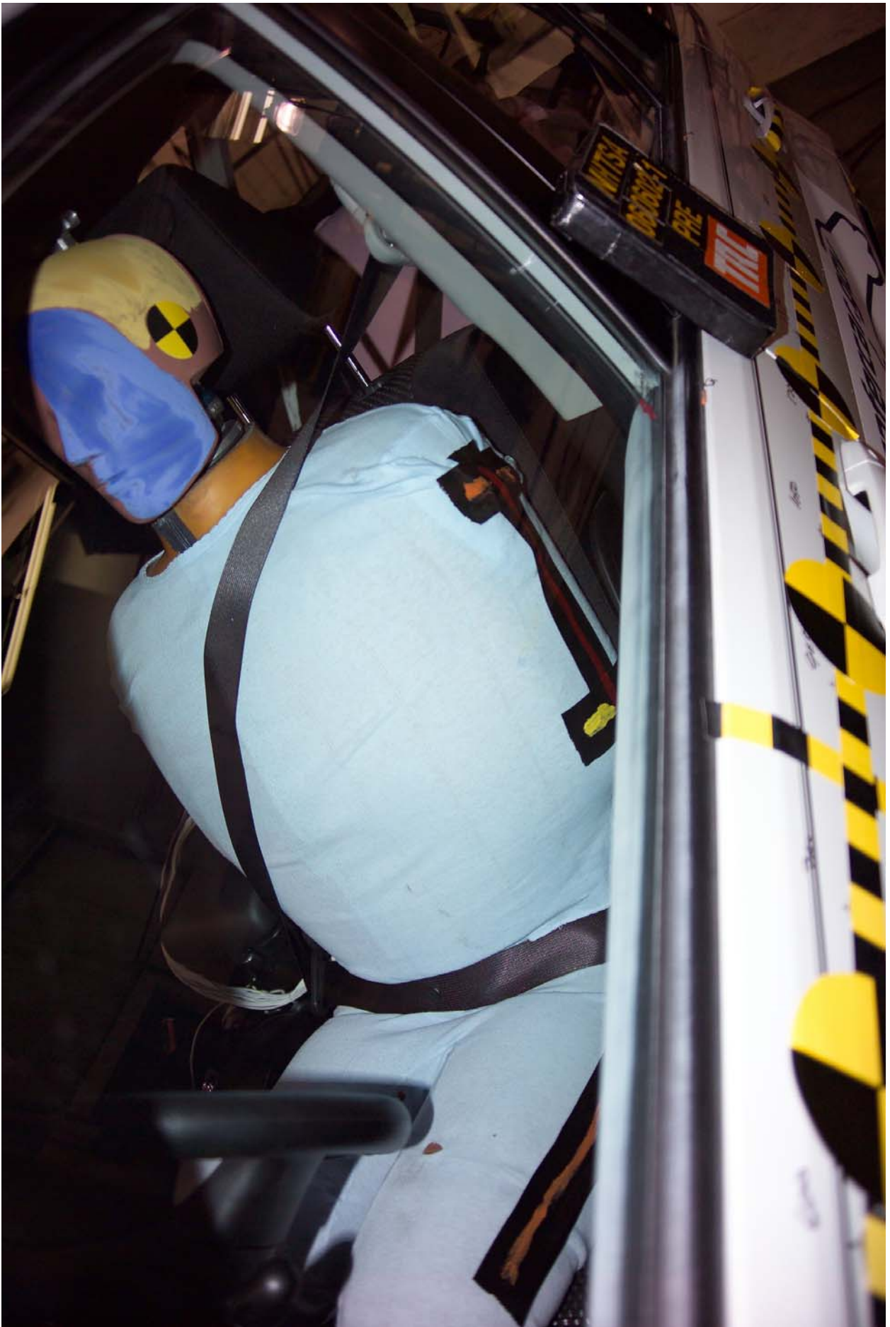
Figure A-48 Pre-Test Left View of Front SID HIII and Door Clearance
