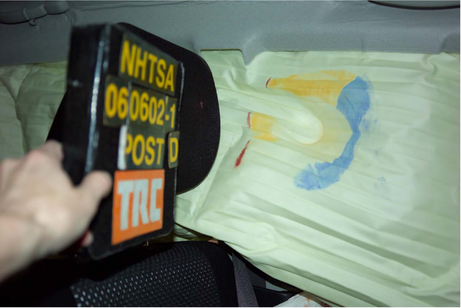
Figure A-57 Post-Test Front SID HIII Contact - View 1
