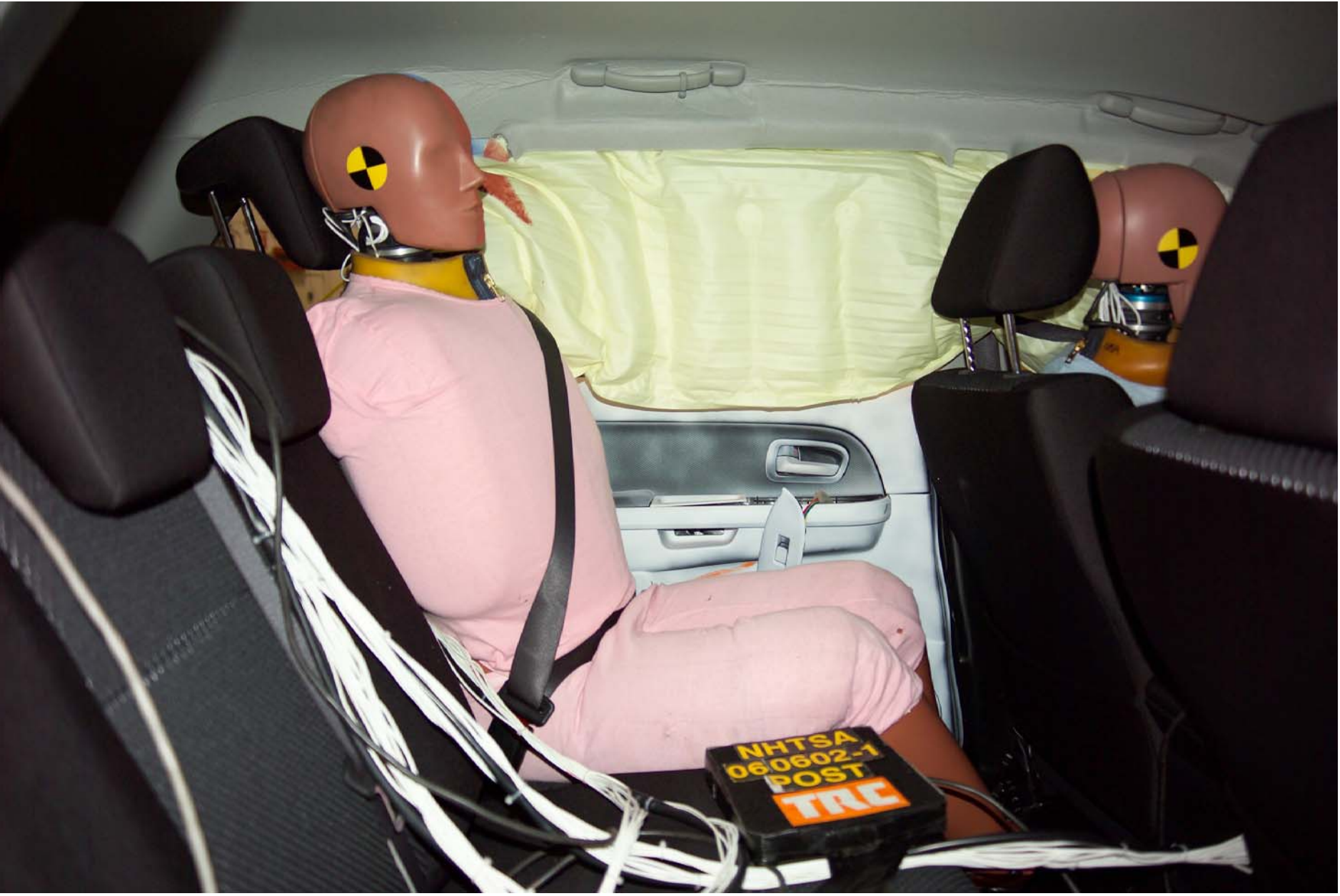
Figure A-44 Post-Test Right Occupant Compartment View of Rear SID HIII
