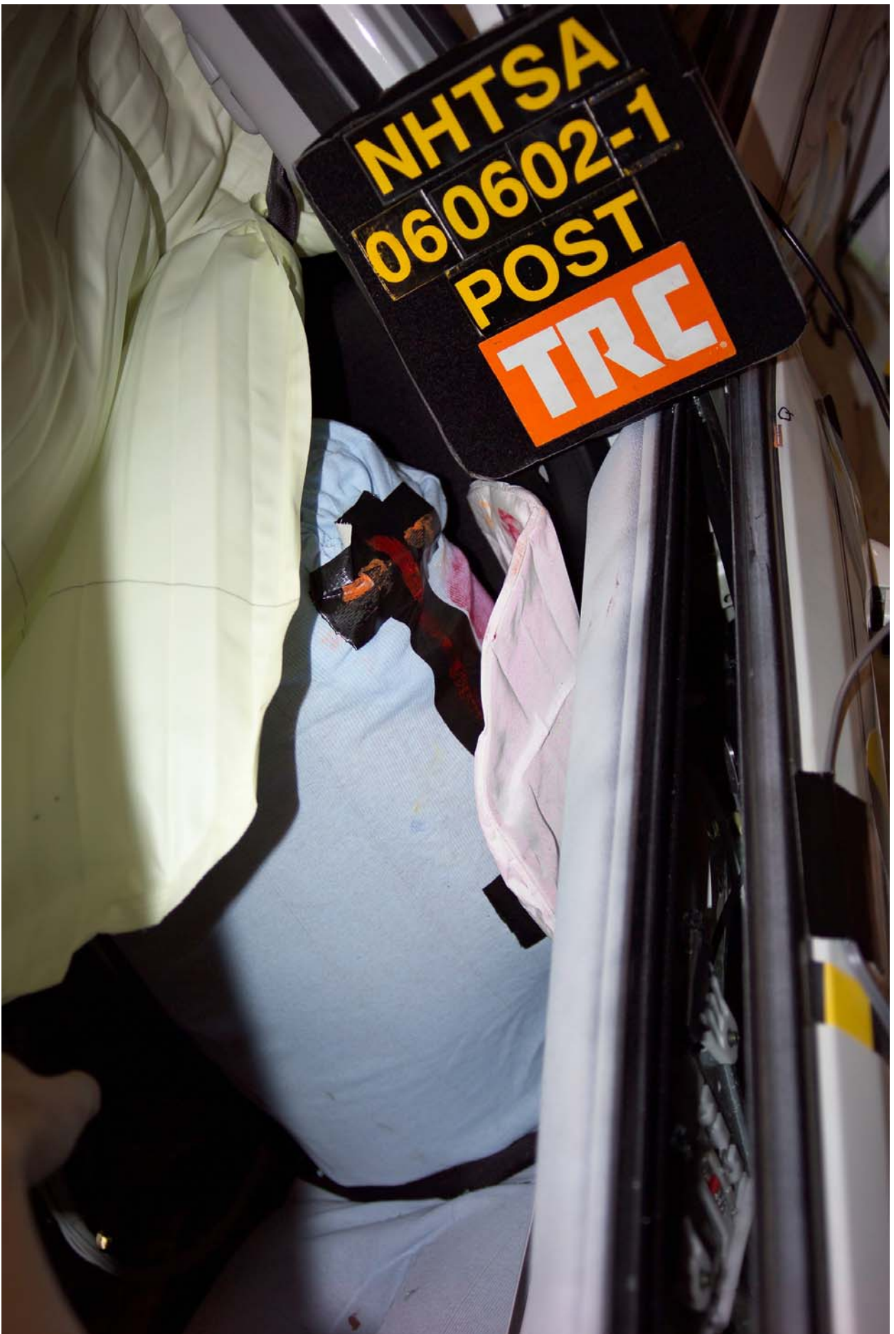
Figure A-49 Post-Test Left View of Front SID HIII and Door Clearance
