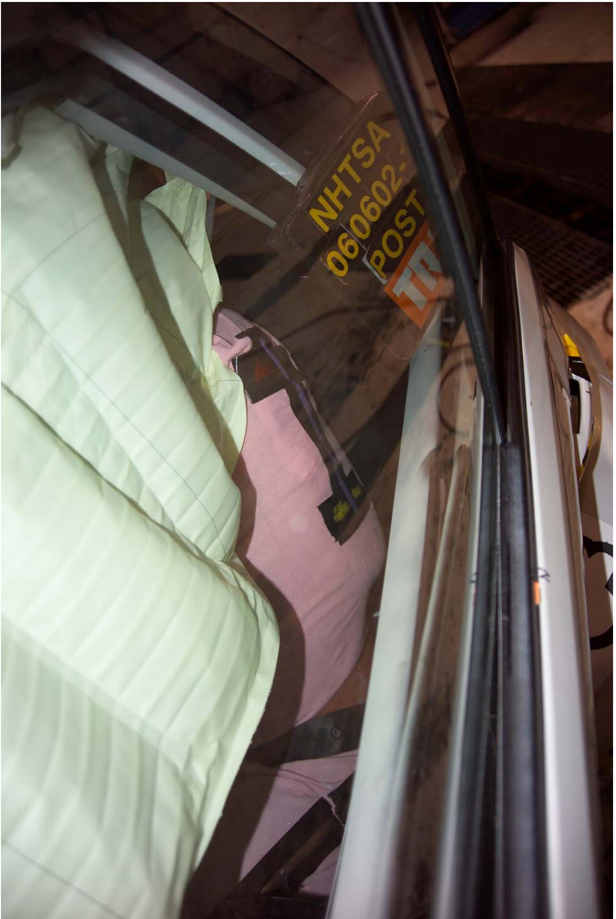
Figure A-54 Post-Test Left View of Rear SID HIII and Door Clearance
