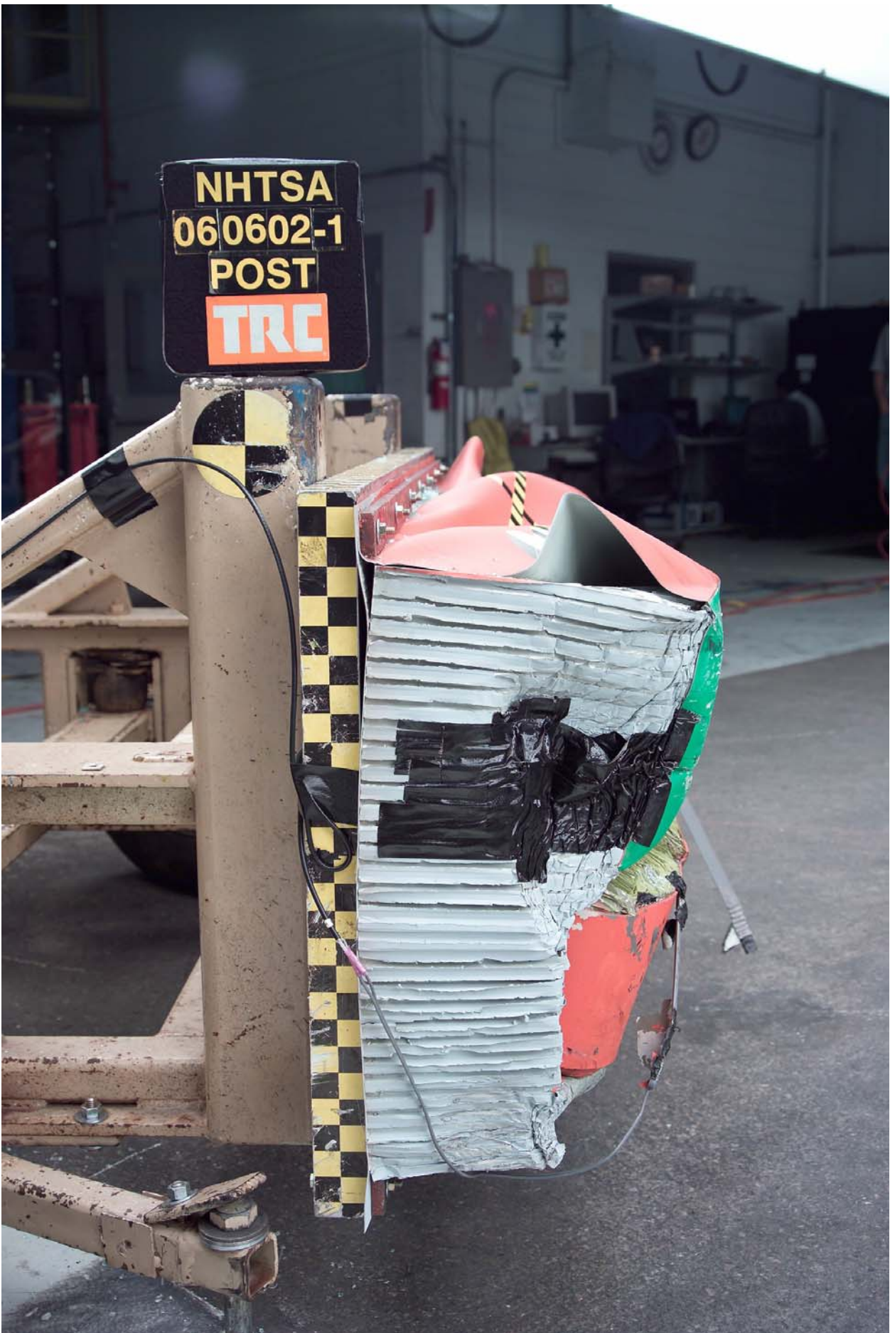
Figure A-30 Post-Test Right Side View of Impactor
