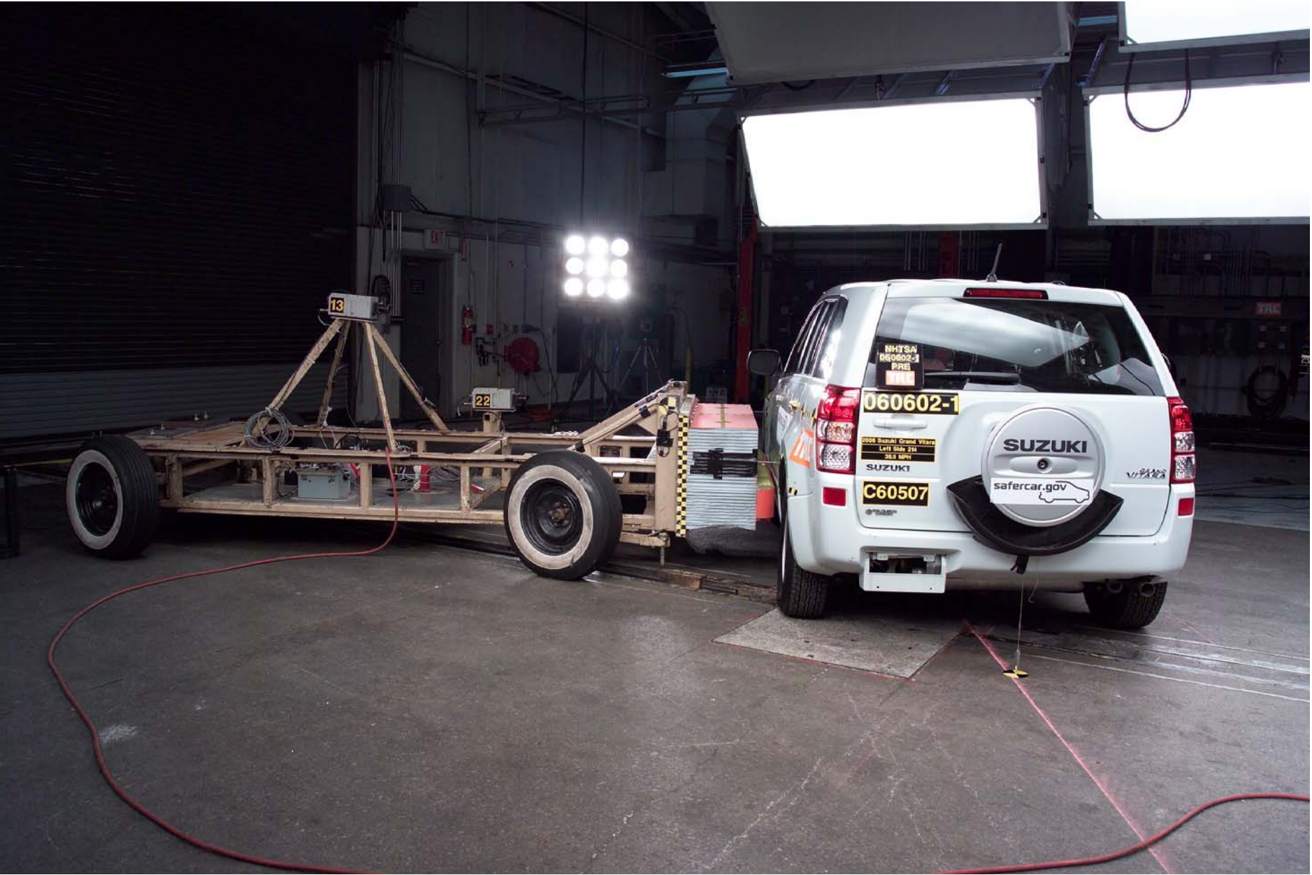
Figure A-69 Pre-Test Right Side View of MDB With Impactor Face in Position
