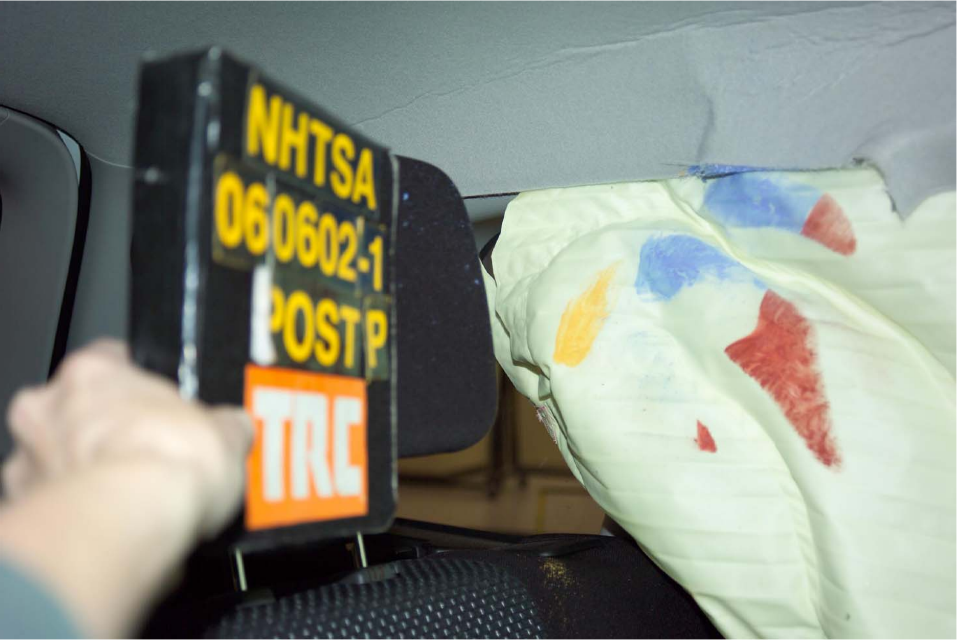
Figure A-62 Post-Test Rear SID HIII Contact - View 1
