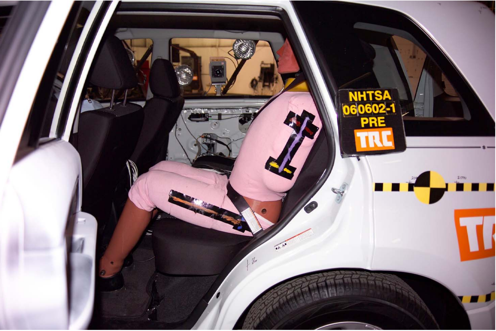
Figure A-52 Pre-Test Left of Rear SID HIII and Belt Position
