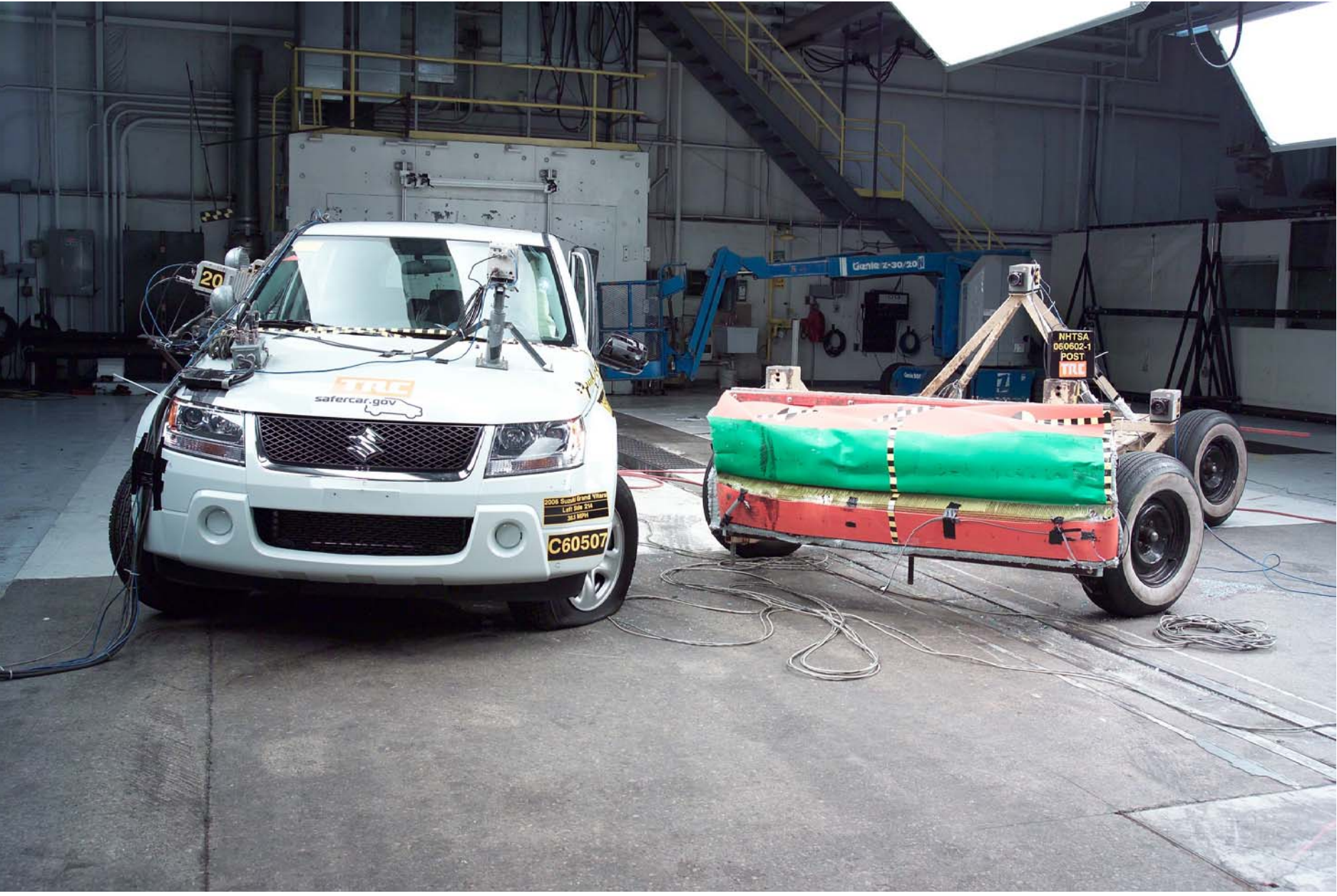
Figure A-66 Post-Test Left Side View of MDB With Impactor Face in Position
