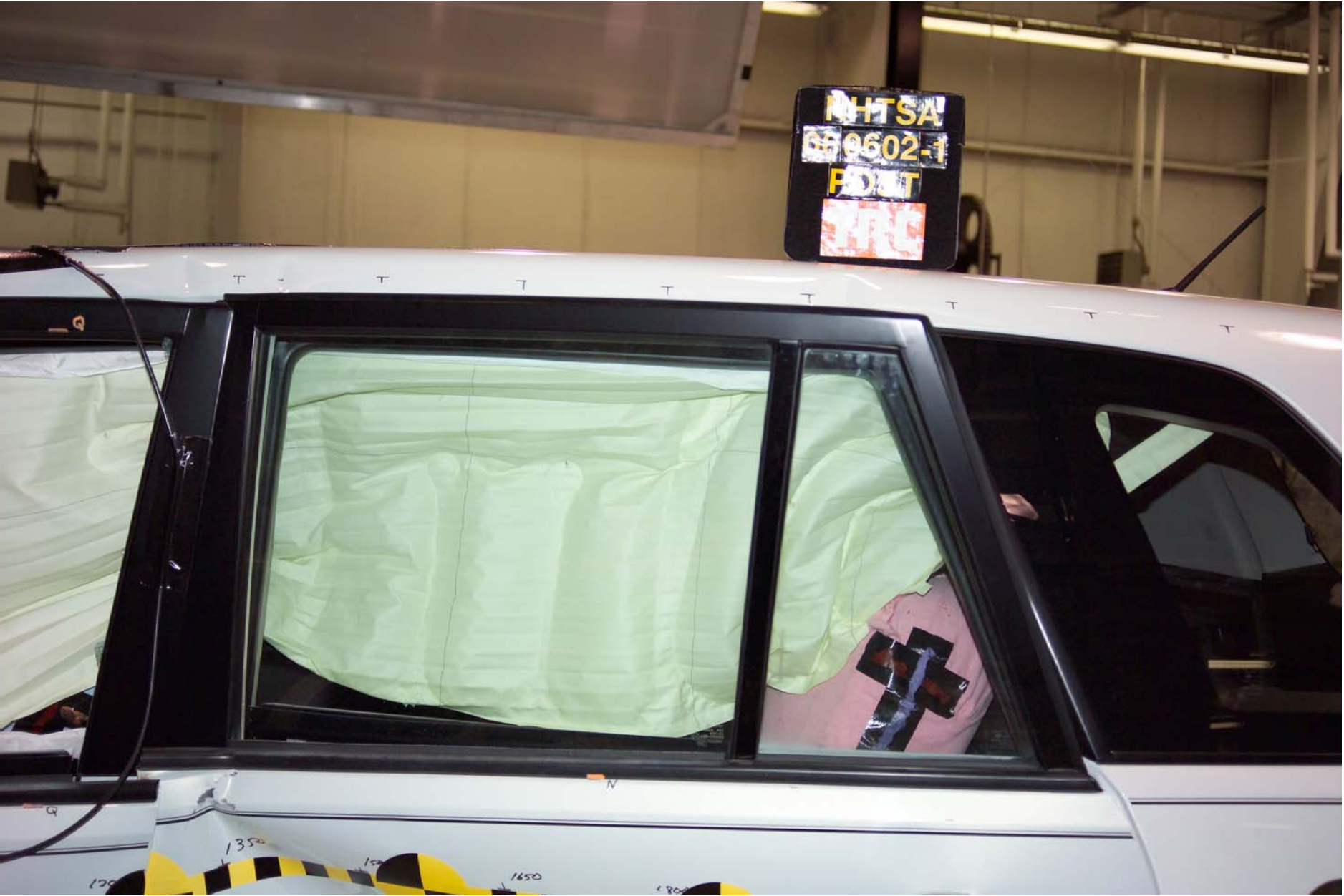
Figure A-51 Post-Test Left View of Rear SID HIII
