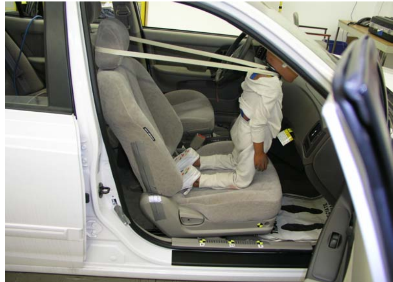
3-Year-Old Unbelted, Forward Seat Track, Position 6
