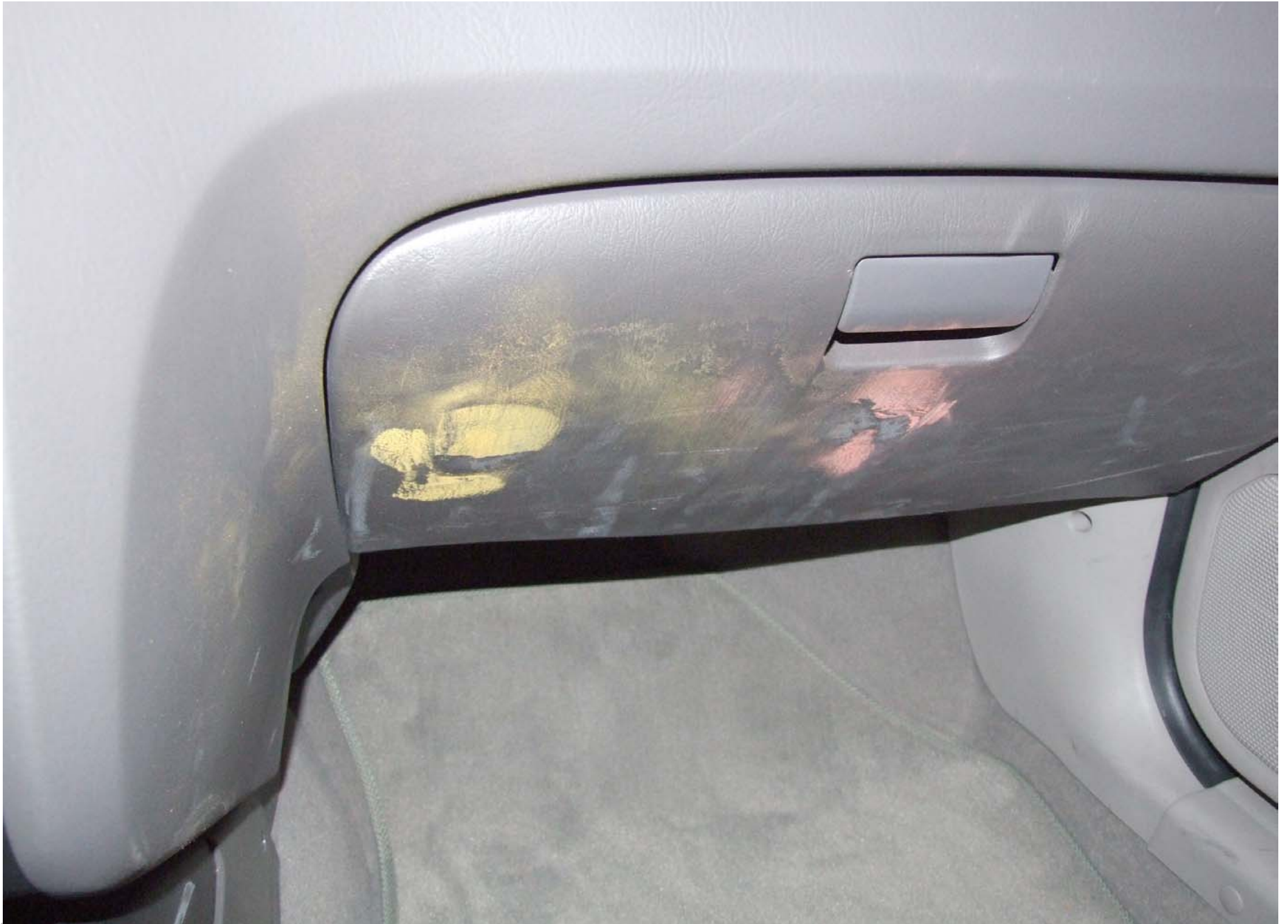
Post-Test Passenger Dummy Knee Contact
