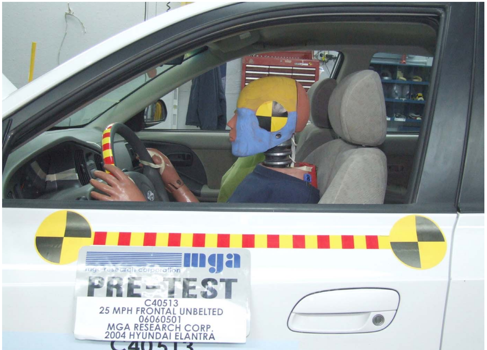
Pre-Test Driver Dummy Position Left Side View
