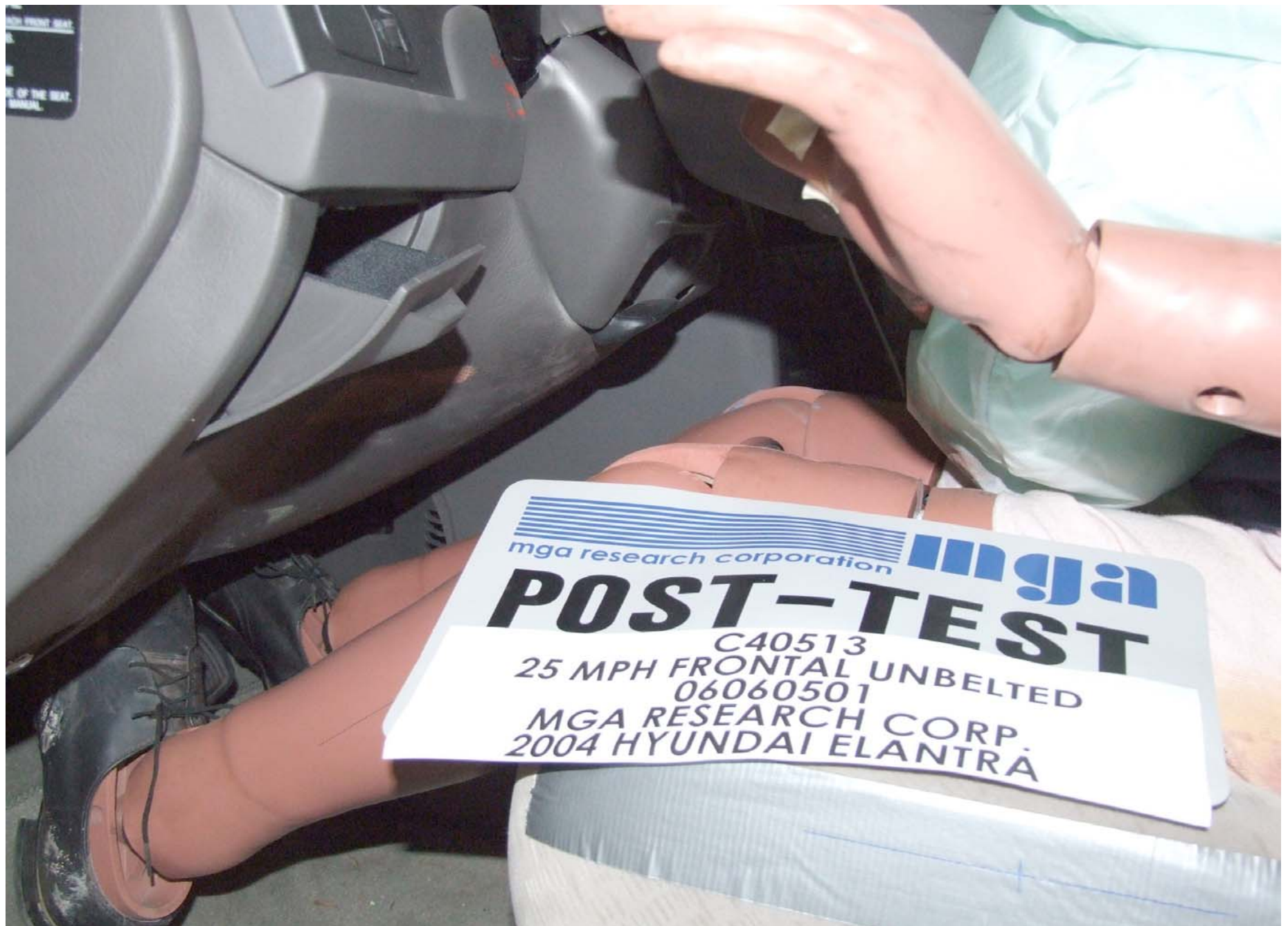
Post-Test Driver Side Knee Bolster View
