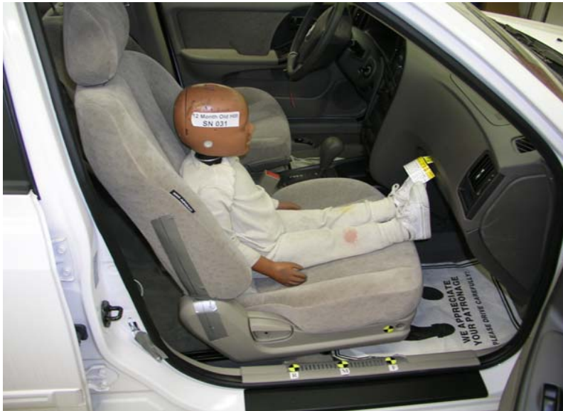
3-Year-Old Unbelted, Forward Seat Track, Position 1
