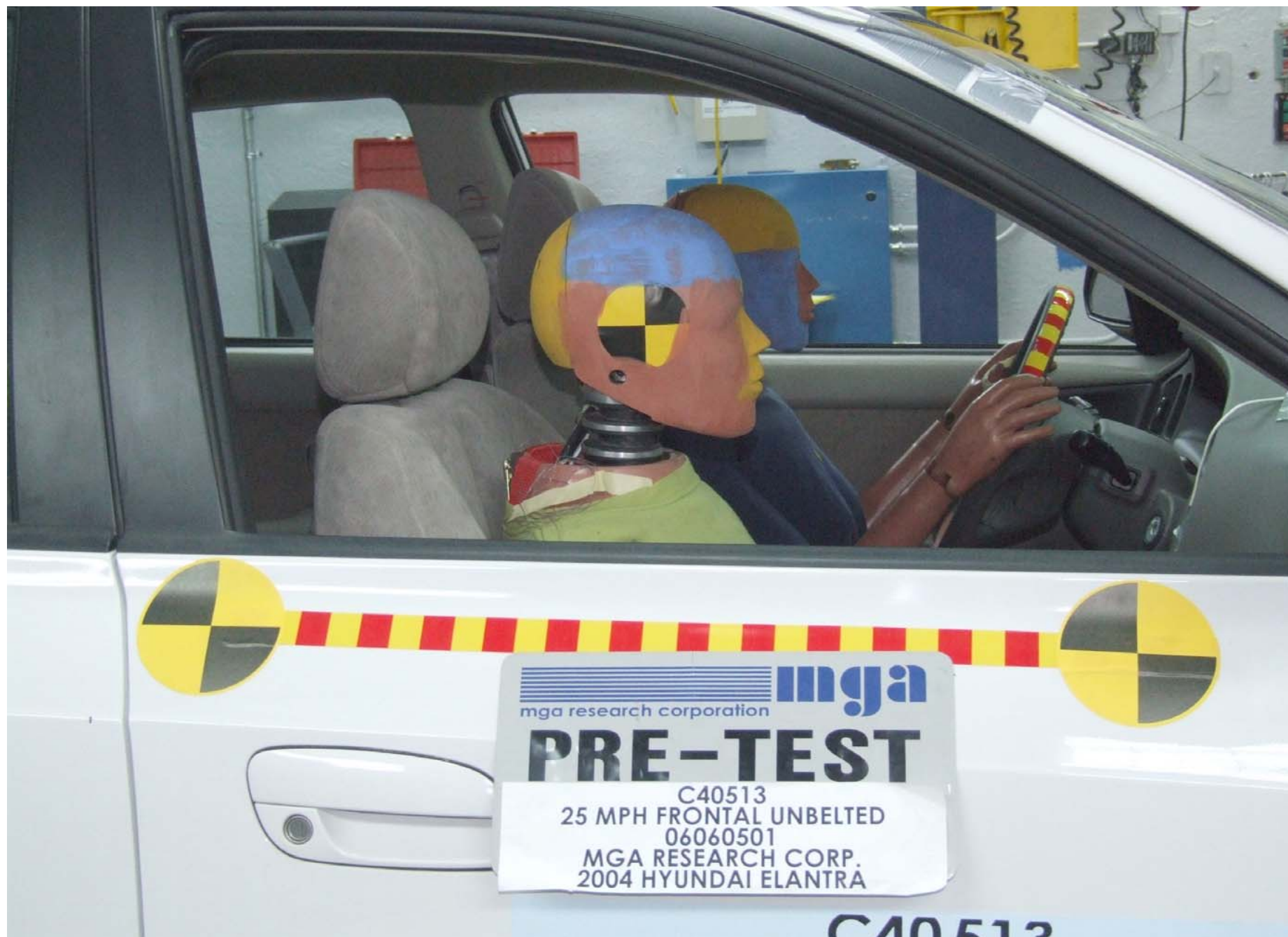
Pre-Test Passenger Dummy Position Right Side View
