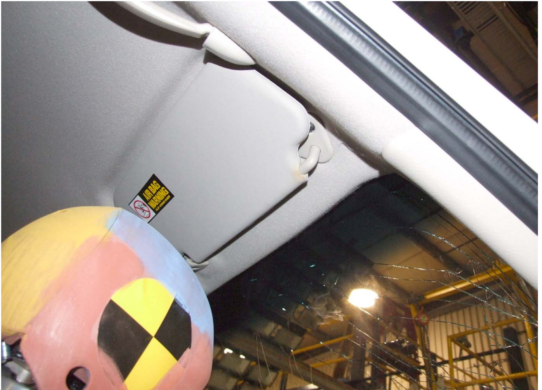
Post-Test Passenger Dummy Head Contact View (visor)
