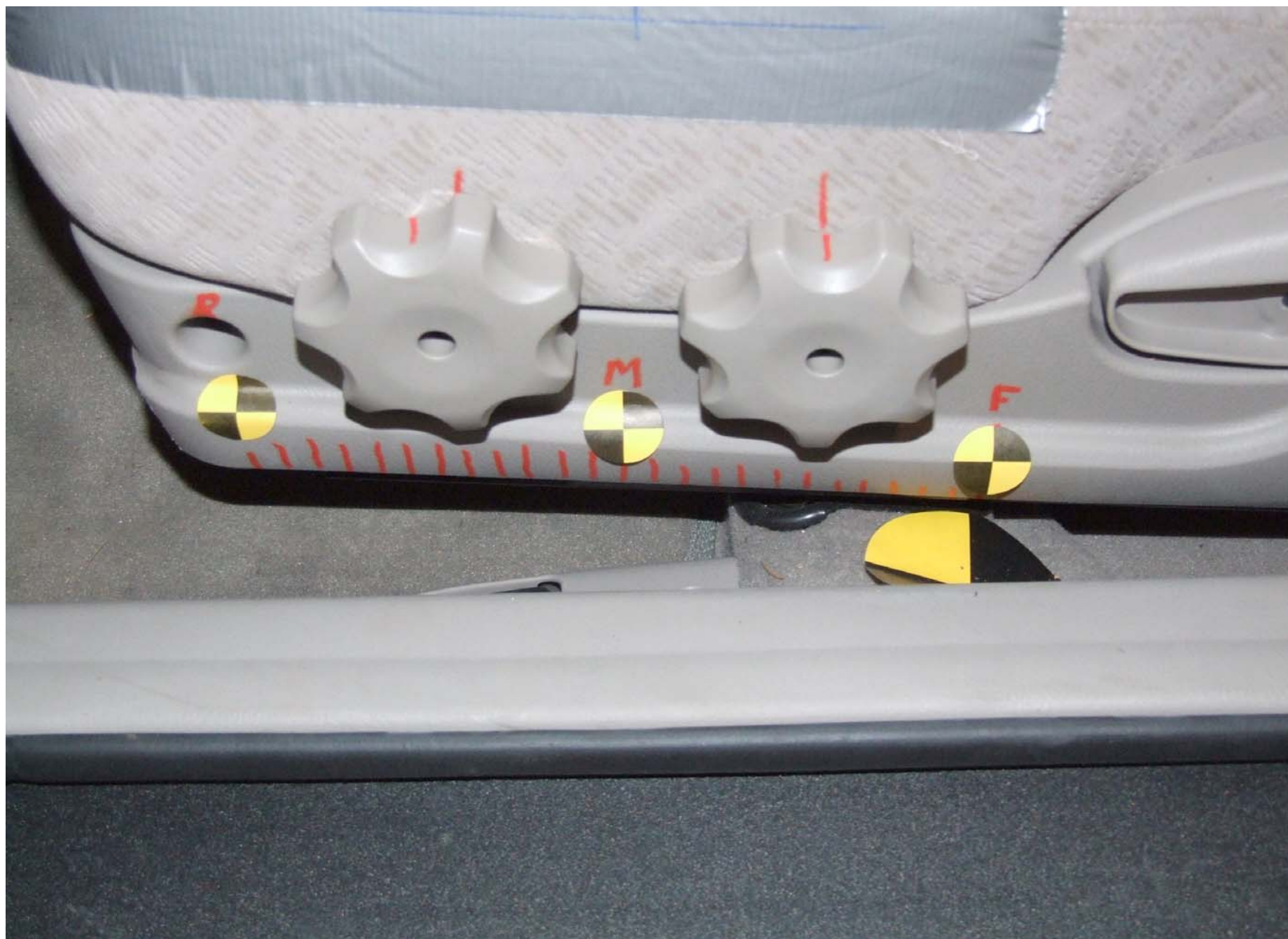
Post-Test Driver Dummy Seat Position
