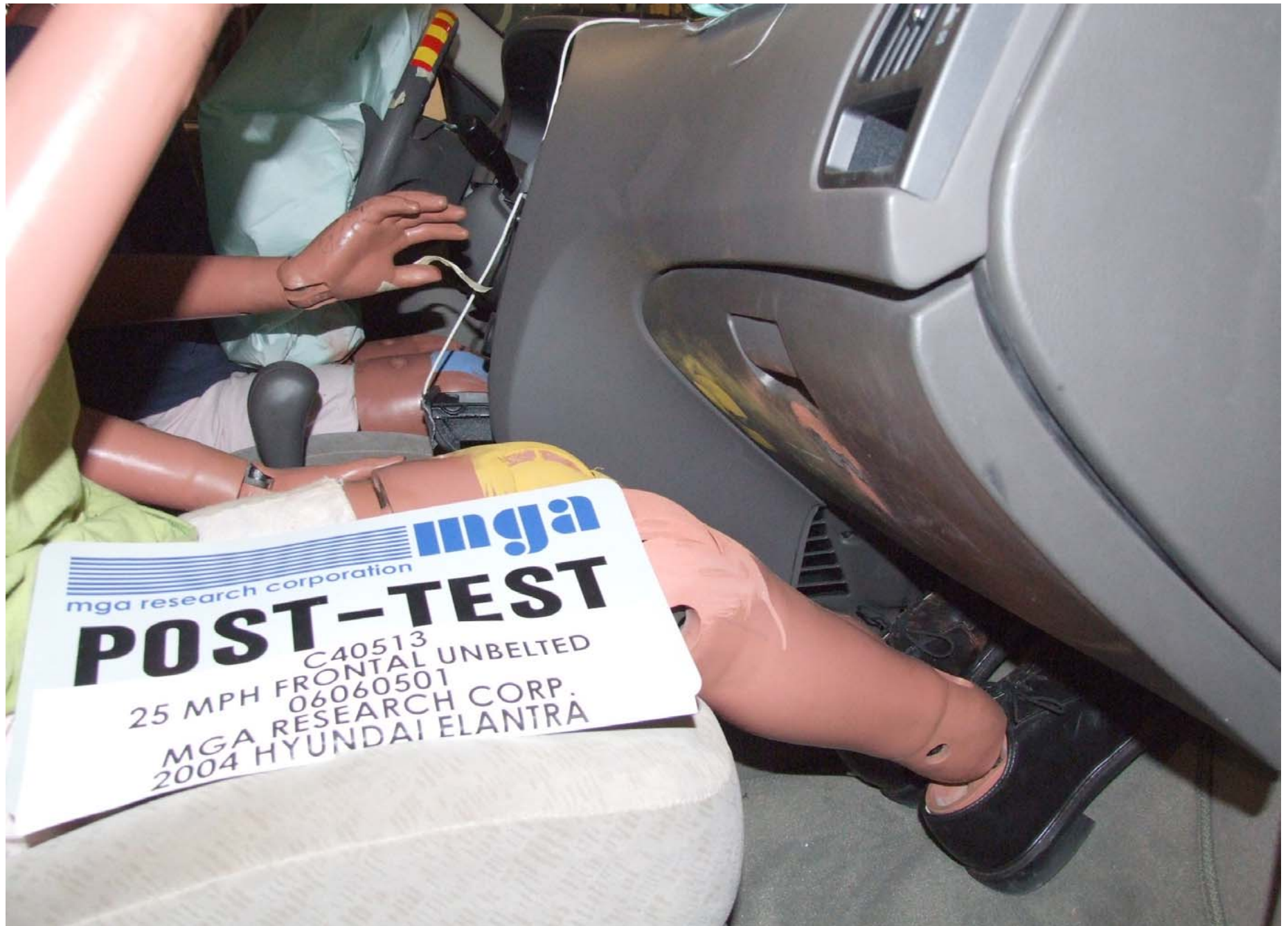
Post-Test Passenger Side Knee Bolster View
