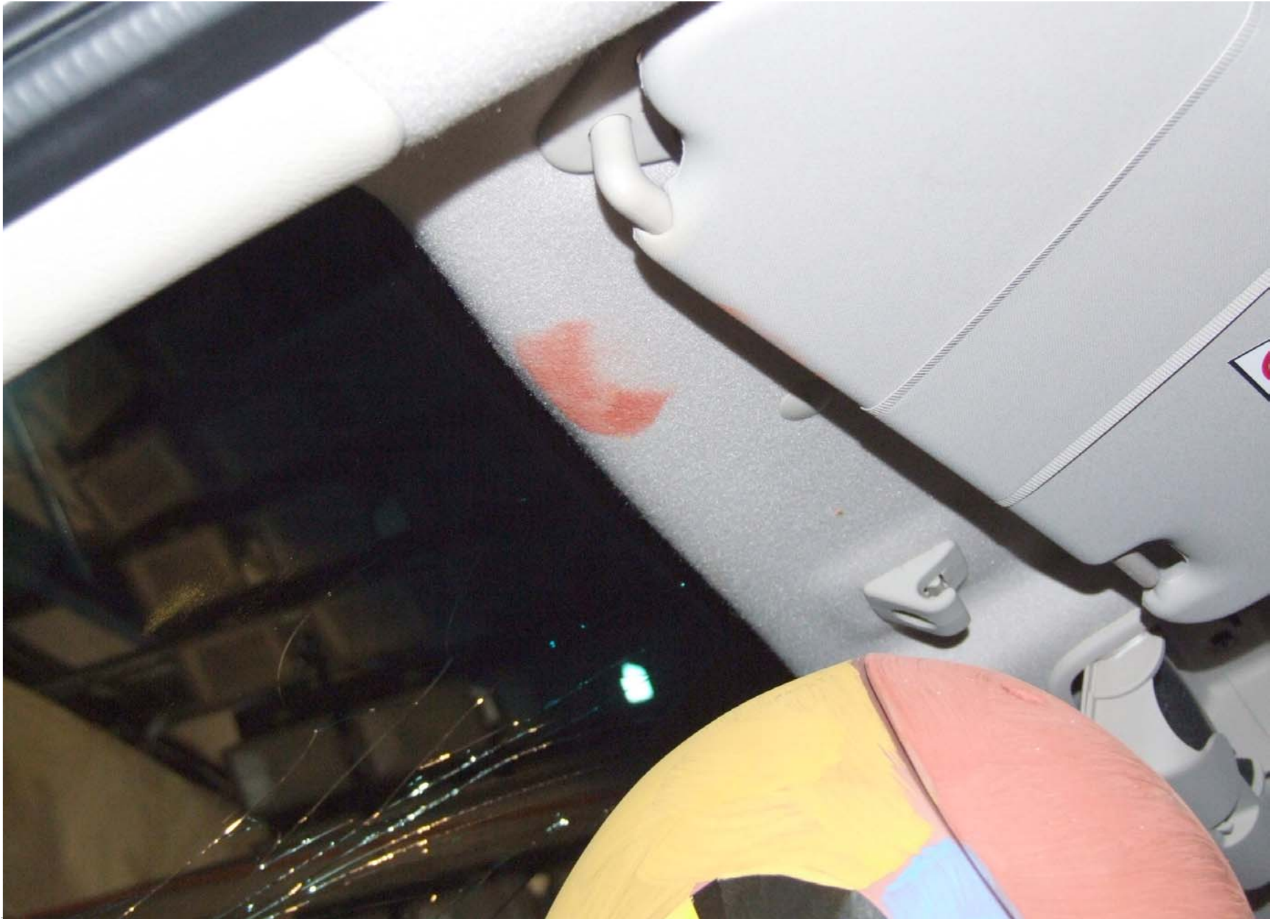
Post-Test Driver Dummy Head Contact (header)
