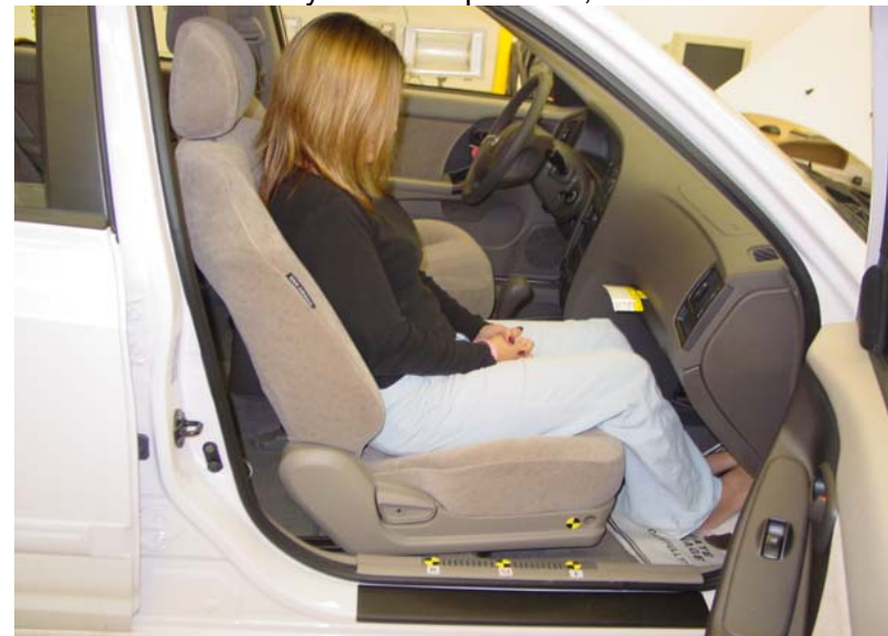
Unbelted 5th Percentile Female Reactivation, Forward Seat Track, Human Subject 013
