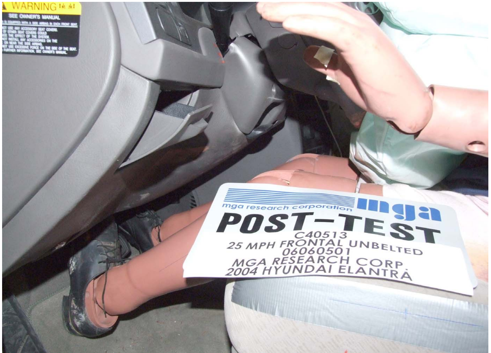
Post-Test Driver Dummy Feet Position
