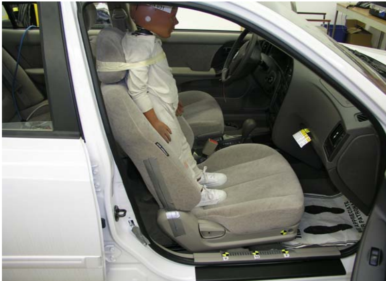
3-Year-Old Unbelted, Forward Seat Track, Position 5
