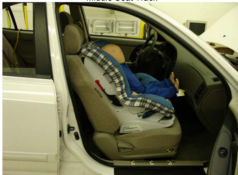
Britax Roundabout 161 Fwd Facing Unbelted, Forward Seat Track
