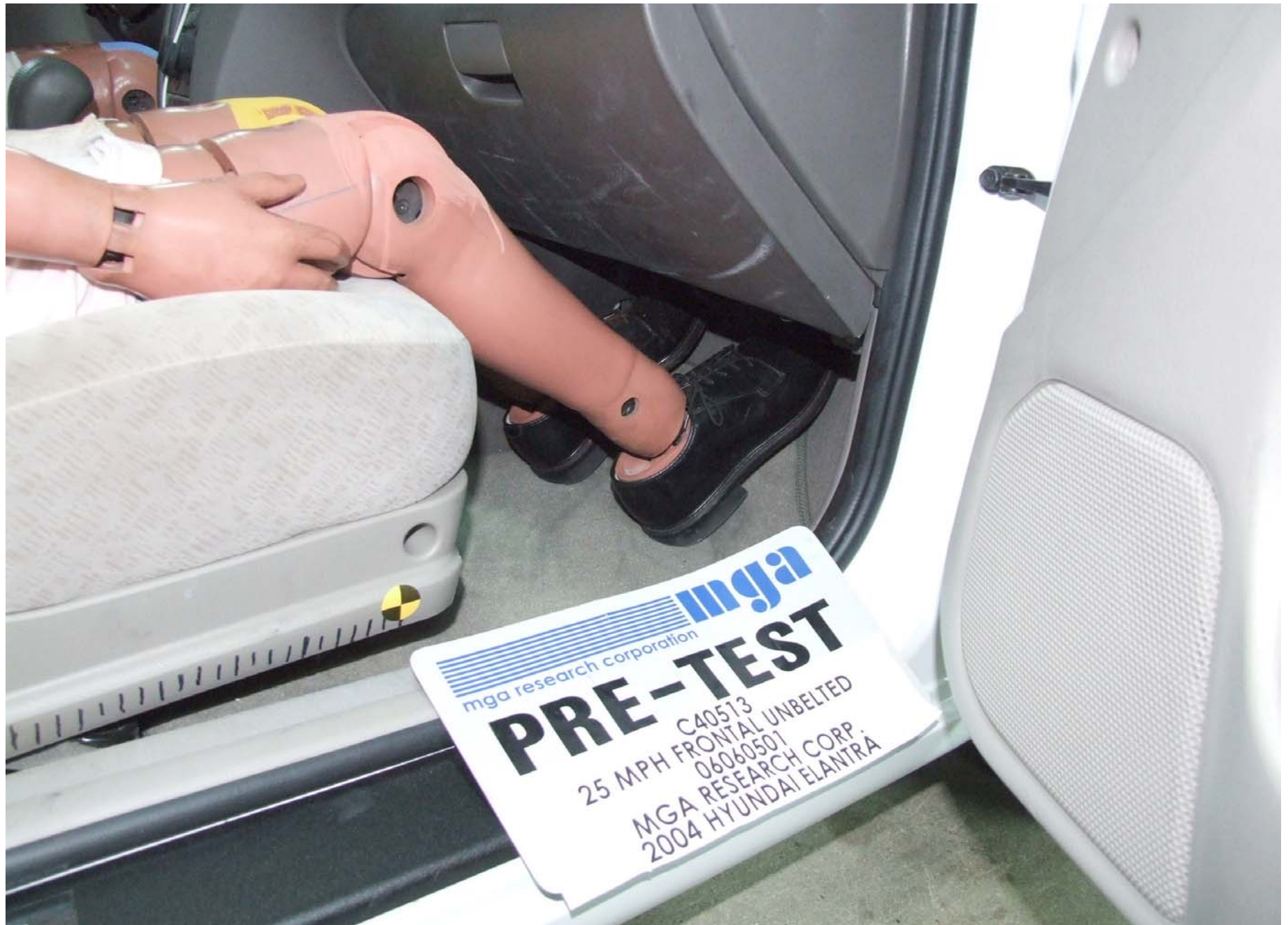
Pre-Test Passenger Dummy Feet Position
