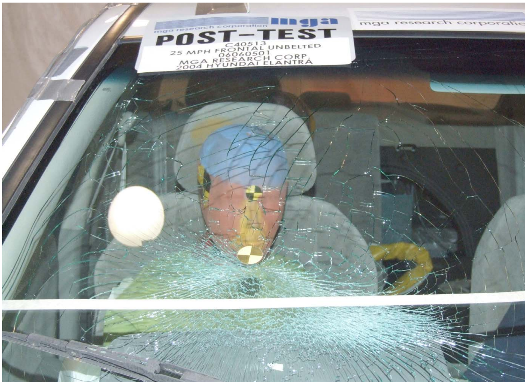
Post-Test Passenger Dummy Front View (head position)
