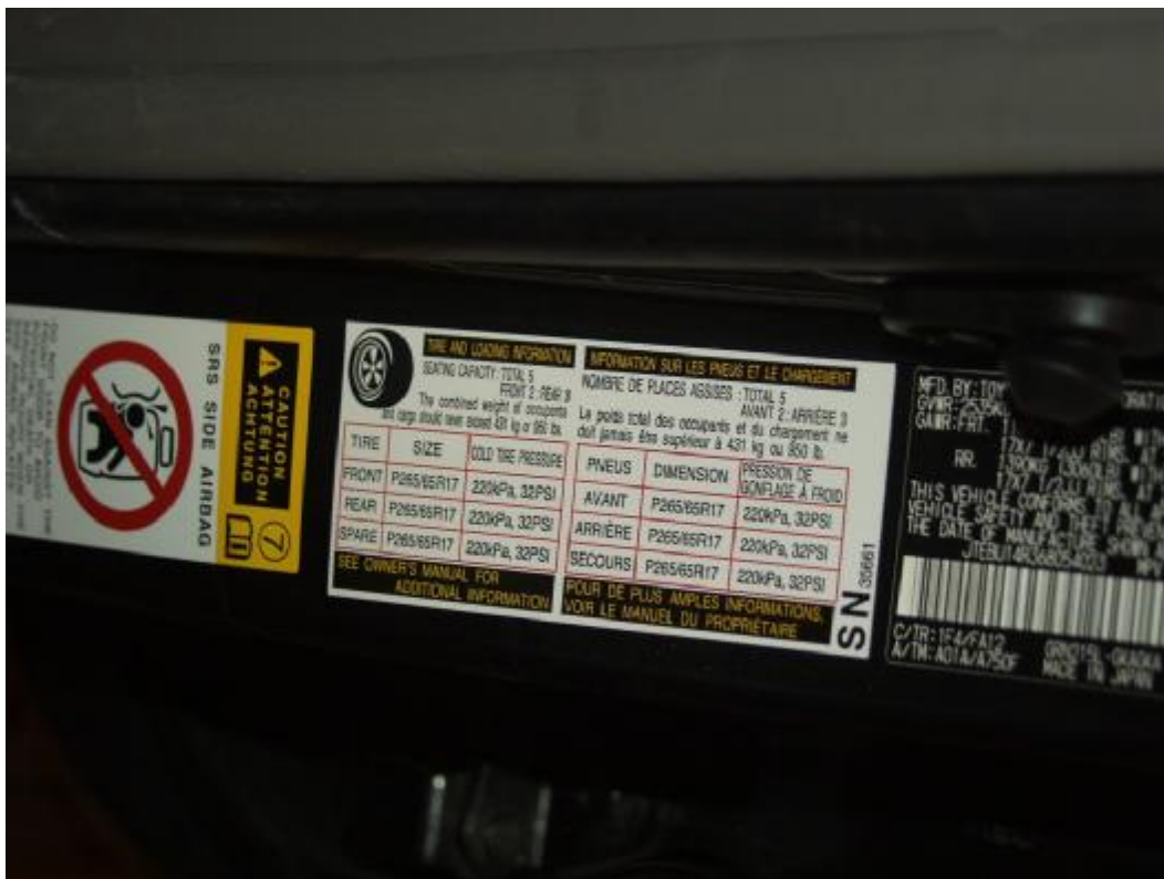
Figure A-4: Vehicle Tire Placard
