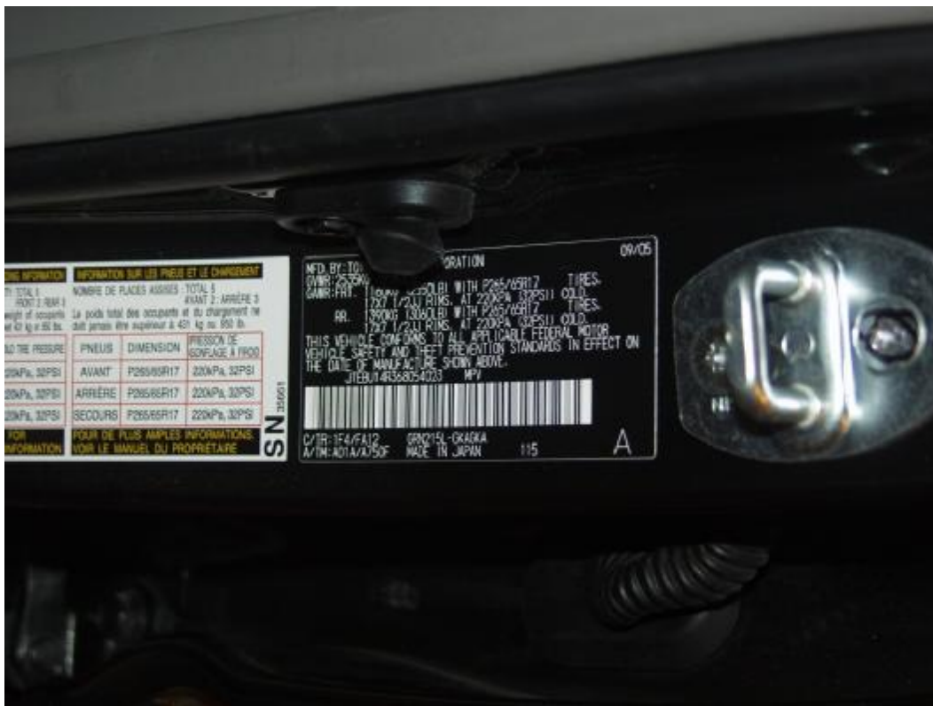
Figure A-3: Vehicle Certification Placard
