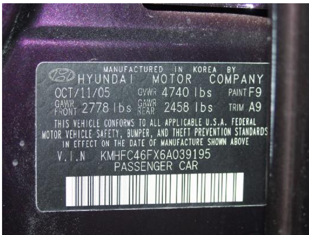
Figure A-3: Vehicle Certification Placard
