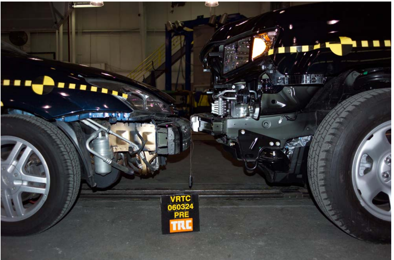
Figure A-6 Pre-Test Impact Alignment - View 2
