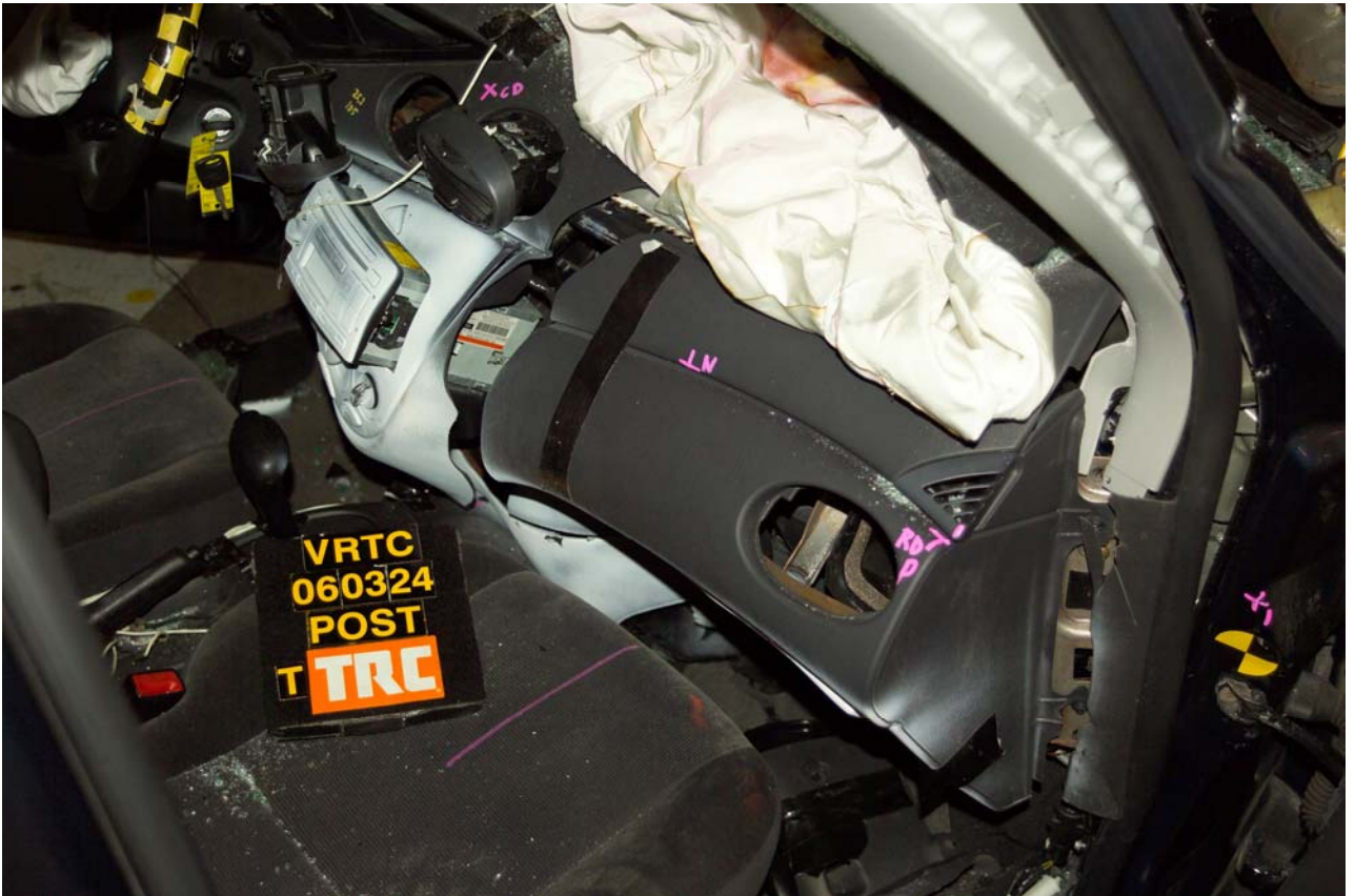
Figure A-128 Post-Test Target Vehicle Passenger Dash Panel Deformation View
