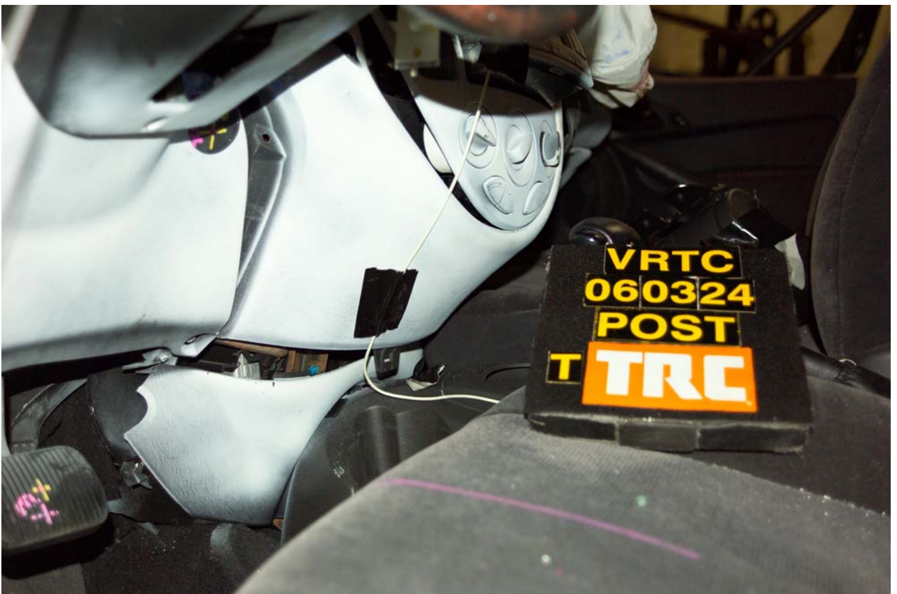
Figure A-121 Post-Test Target Vehicle Driver Console Deformation View
