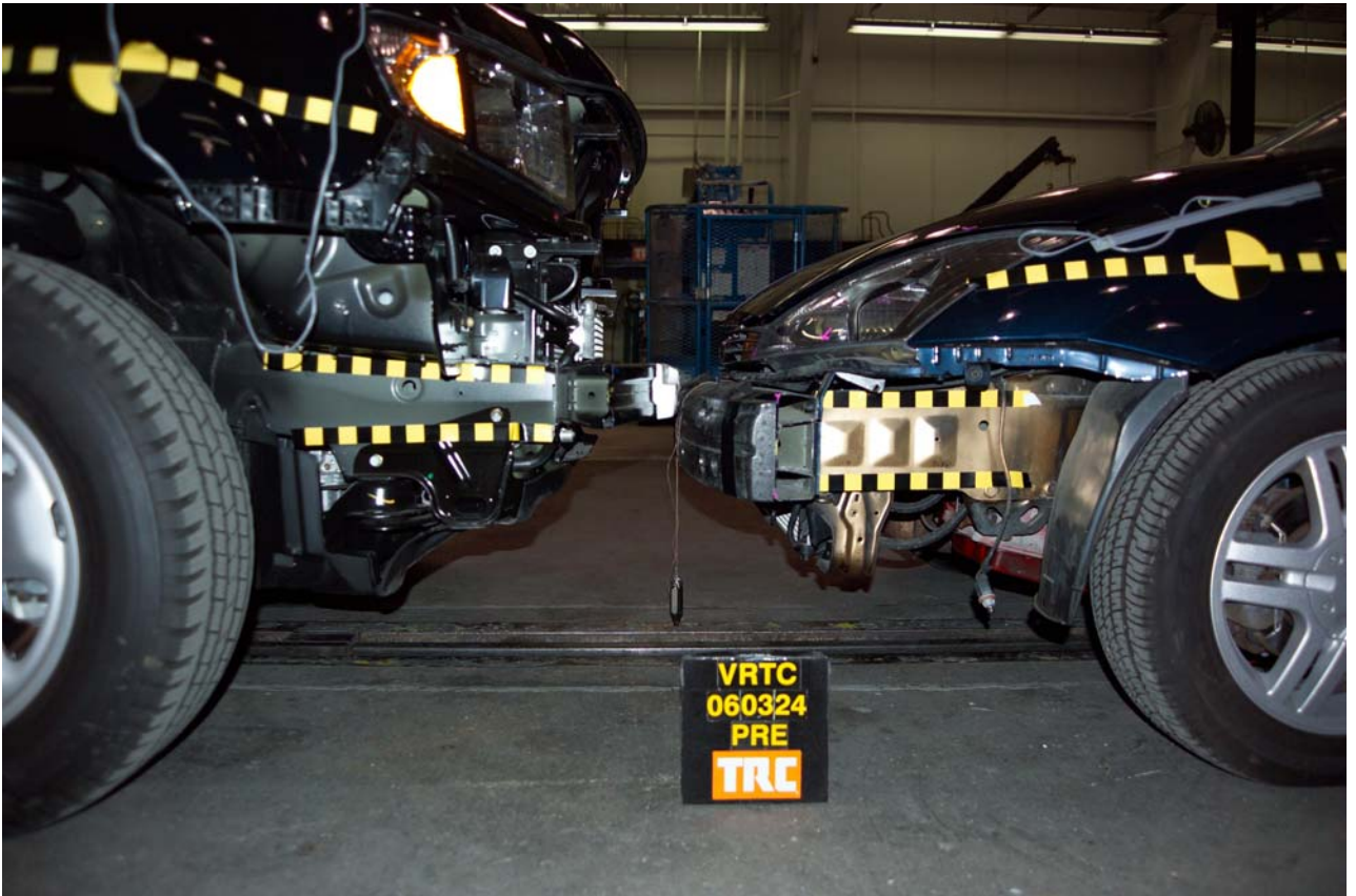
Figure A-5 Pre-Test Impact Alignment - View 1
