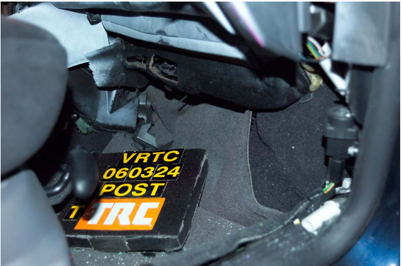
Figure A-130 Post-Test Target Vehicle Passenger Toeboard Deformation View
