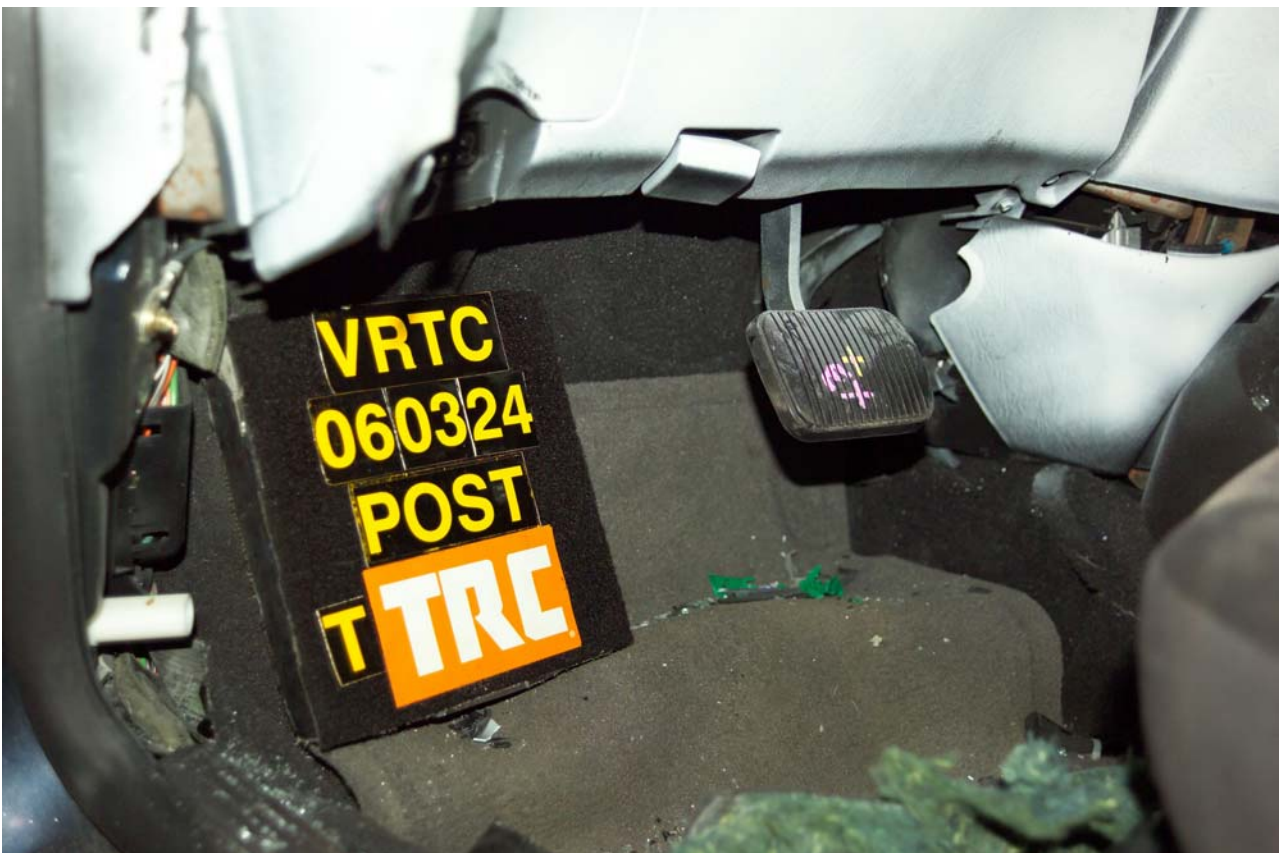
Figure A-123 Post-Test Target Vehicle Driver Toeboard Deformation View
