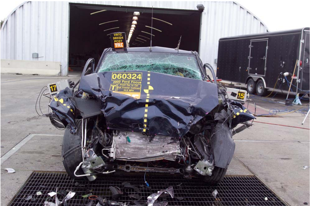
Figure A-16 Post-Test Target Vehicle Front View
