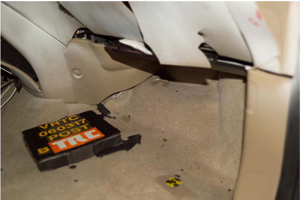
Figure A-133 Post-Test Bullet Vehicle Passenger Toeboard Deformation View
