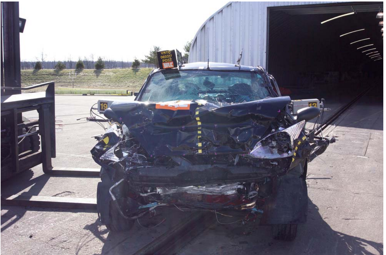
Figure A-16 Post-Test Target Vehicle Front View
