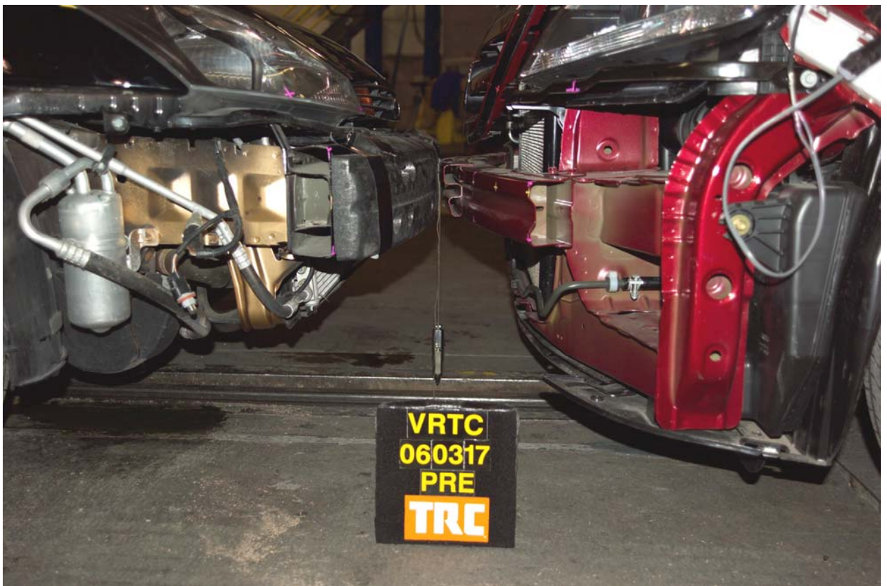
Figure A-6 Pre-Test Impact Alignment - View 2
