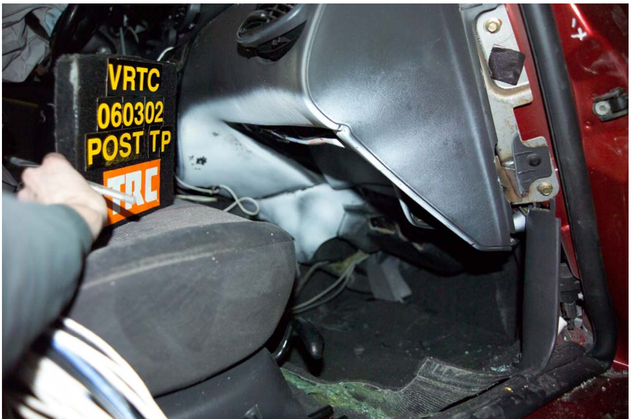
Figure A-118 Post-Test Target Vehicle Passenger Toeboard Deformation View
