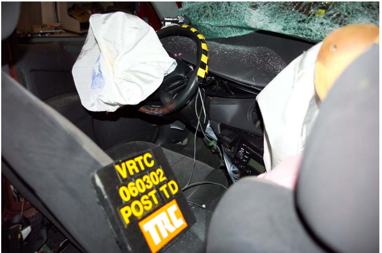
Figure A-119 Post-Test Target Vehicle Interior Damage - View 1
