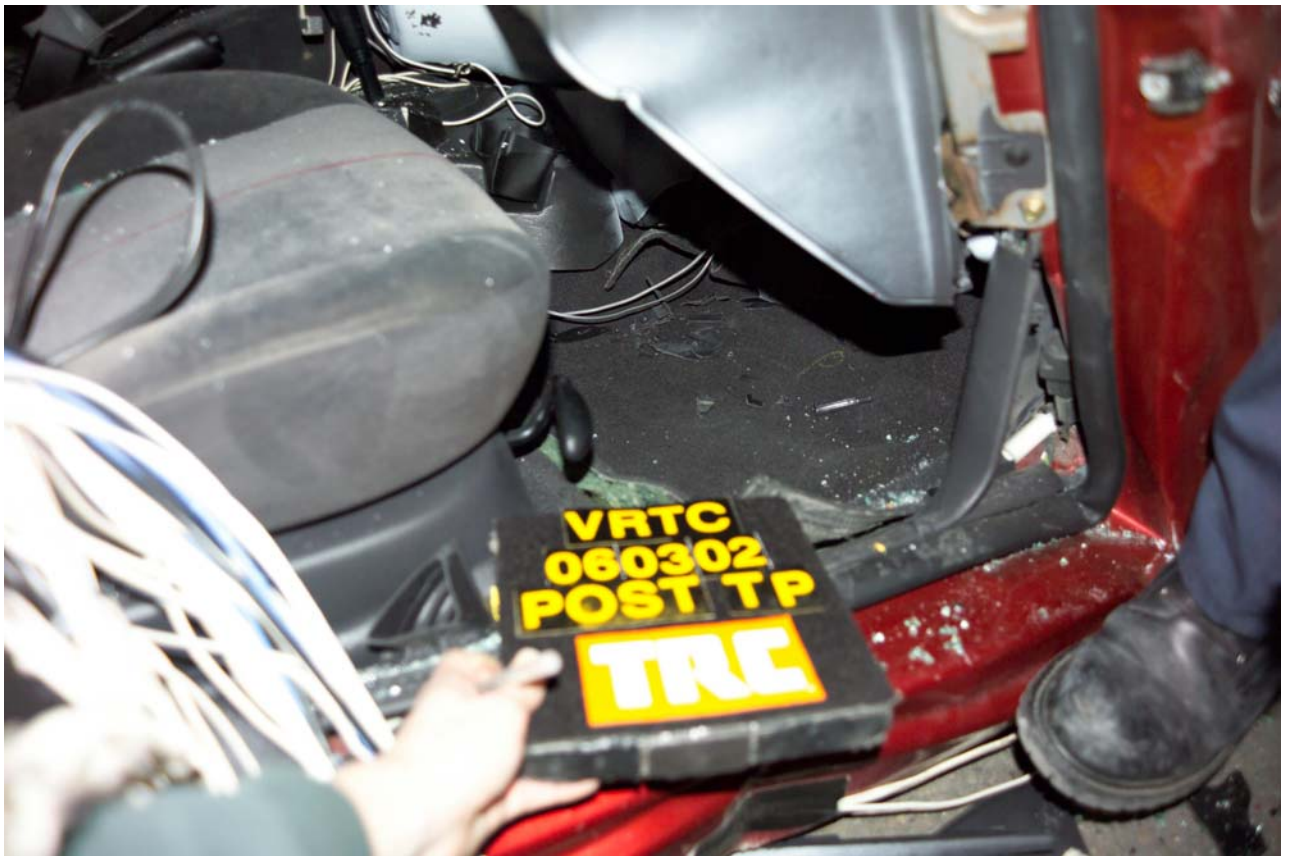
Figure A-117 Post-Test Target Vehicle Passenger Floorboard Deformation View
