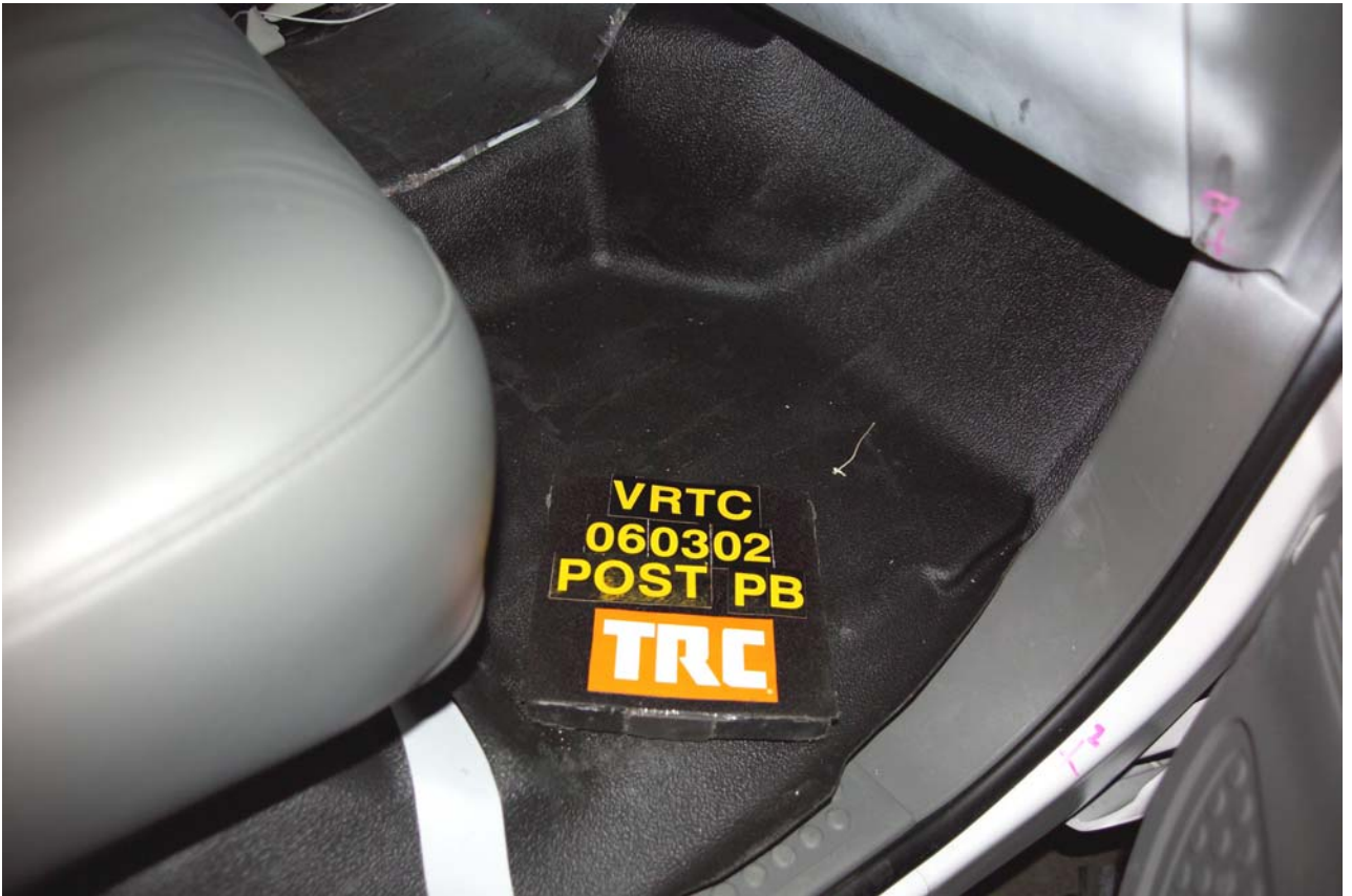
Figure A-131 Post-Test Bullet Vehicle Passenger Floorboard Deformation View
