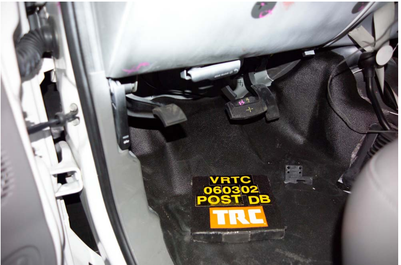
Figure A-126 Post-Test Bullet Vehicle Driver Toeboard Deformation View
