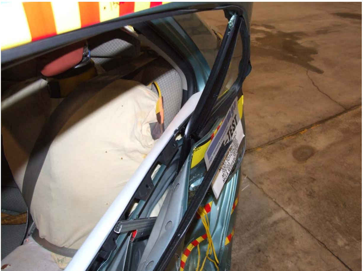
Post-Test Passenger Dummy Clearance From Door
