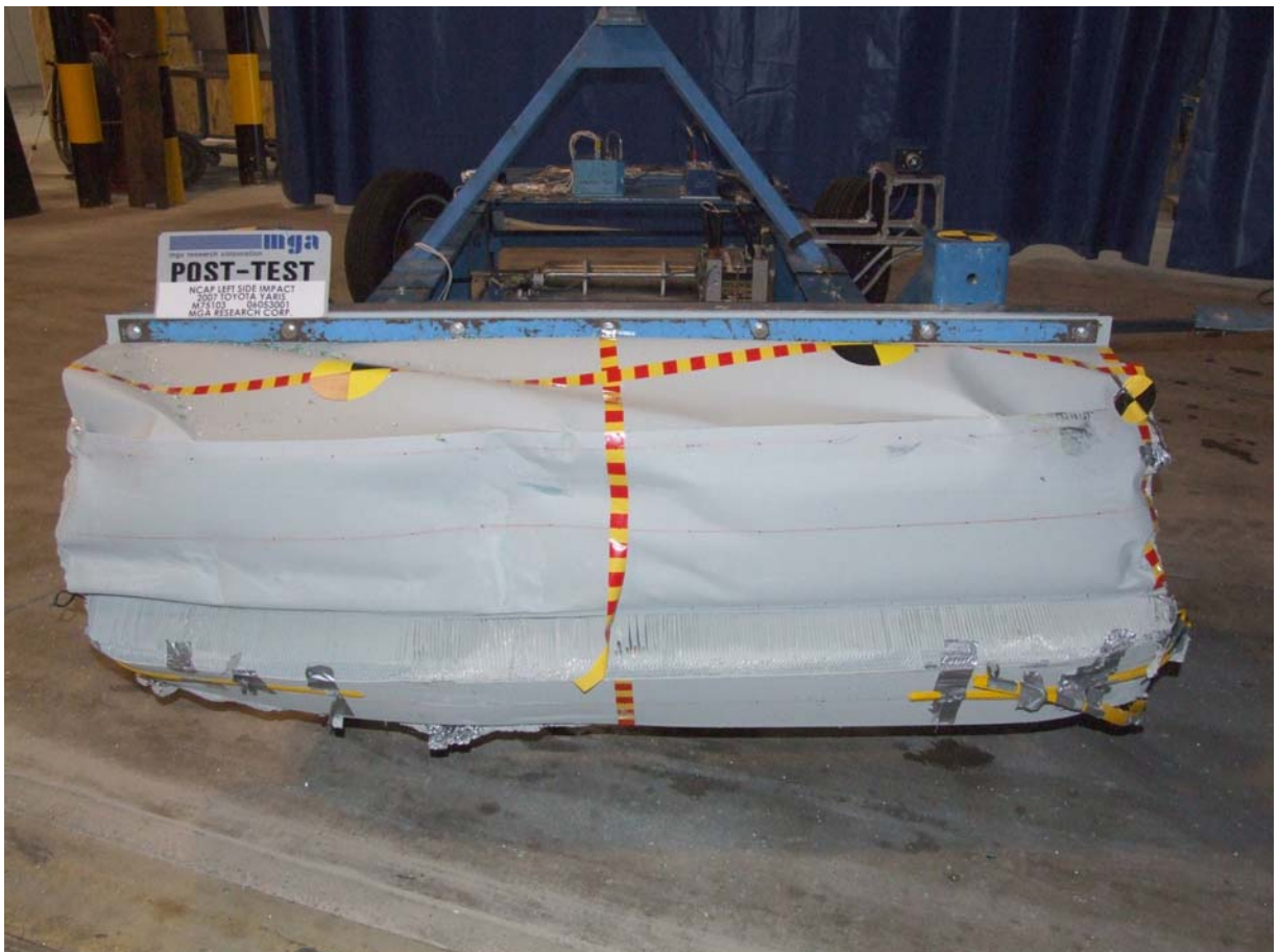
Post-Test Front View of Deformable Barrier
