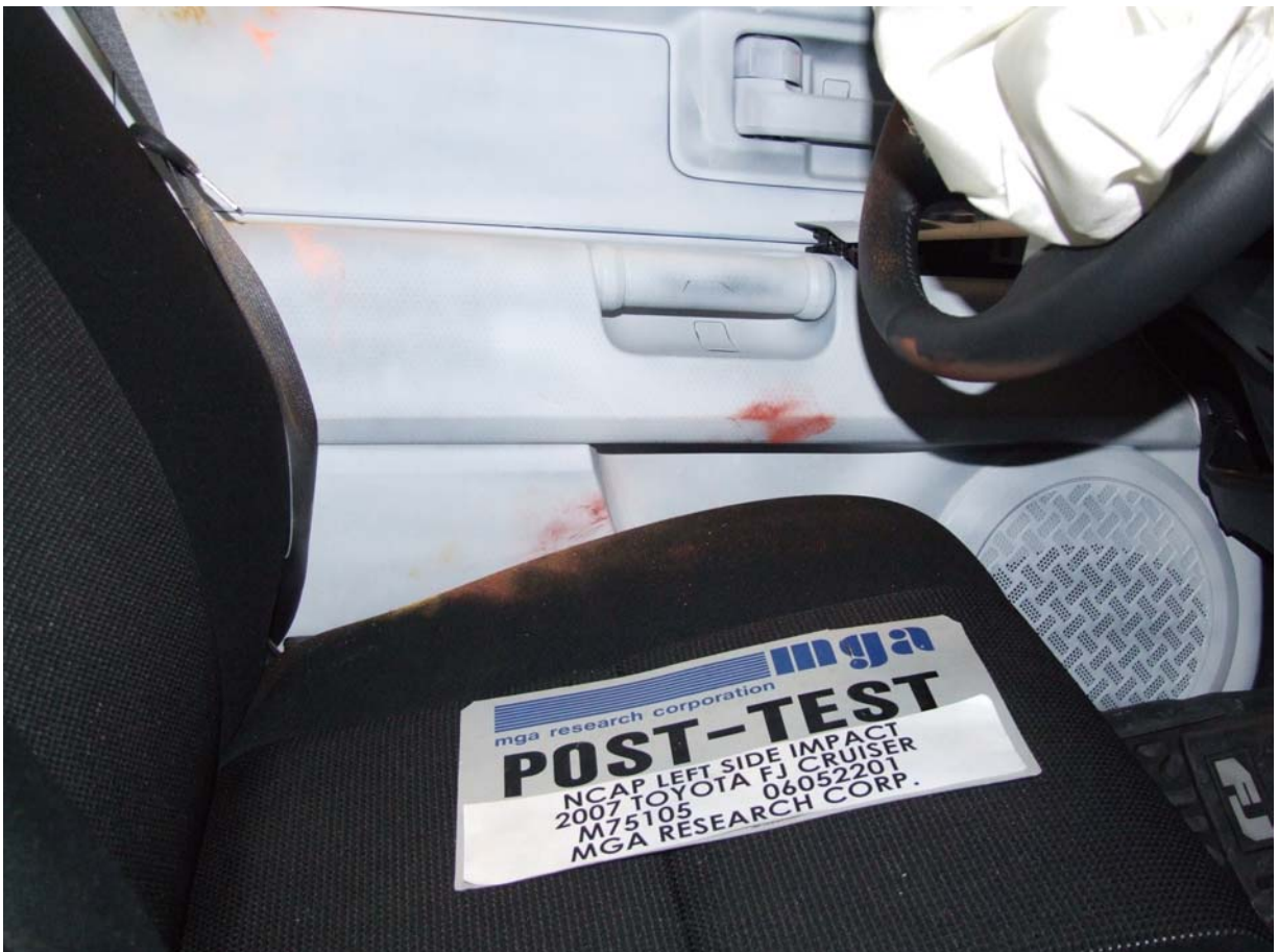
Post-Test Driver Dummy Torso Contact
