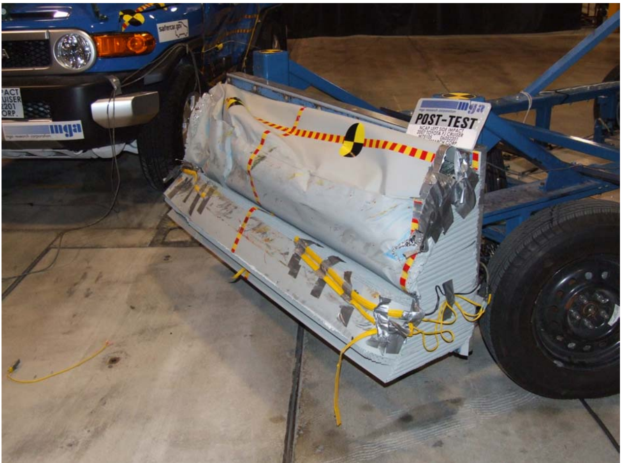
Post-Test Left Side View of Deformable Barrier
