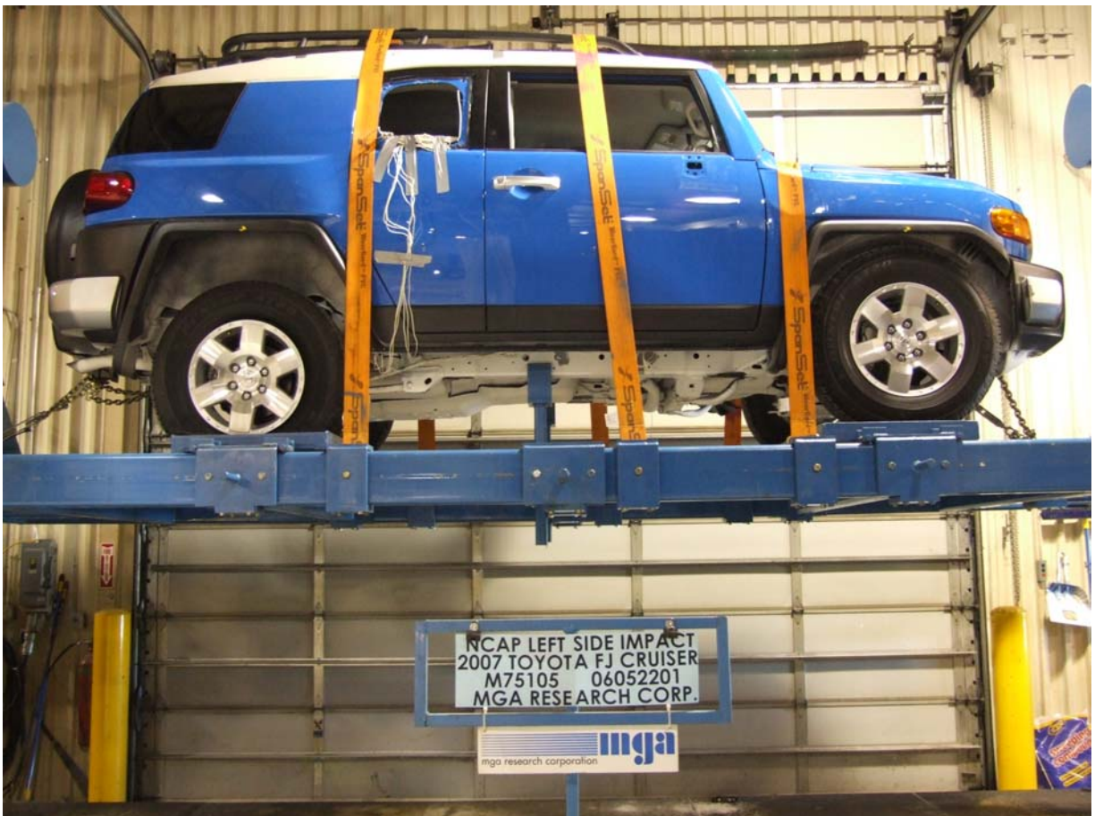
Vehicle on Rollover Device (360 Degrees)
