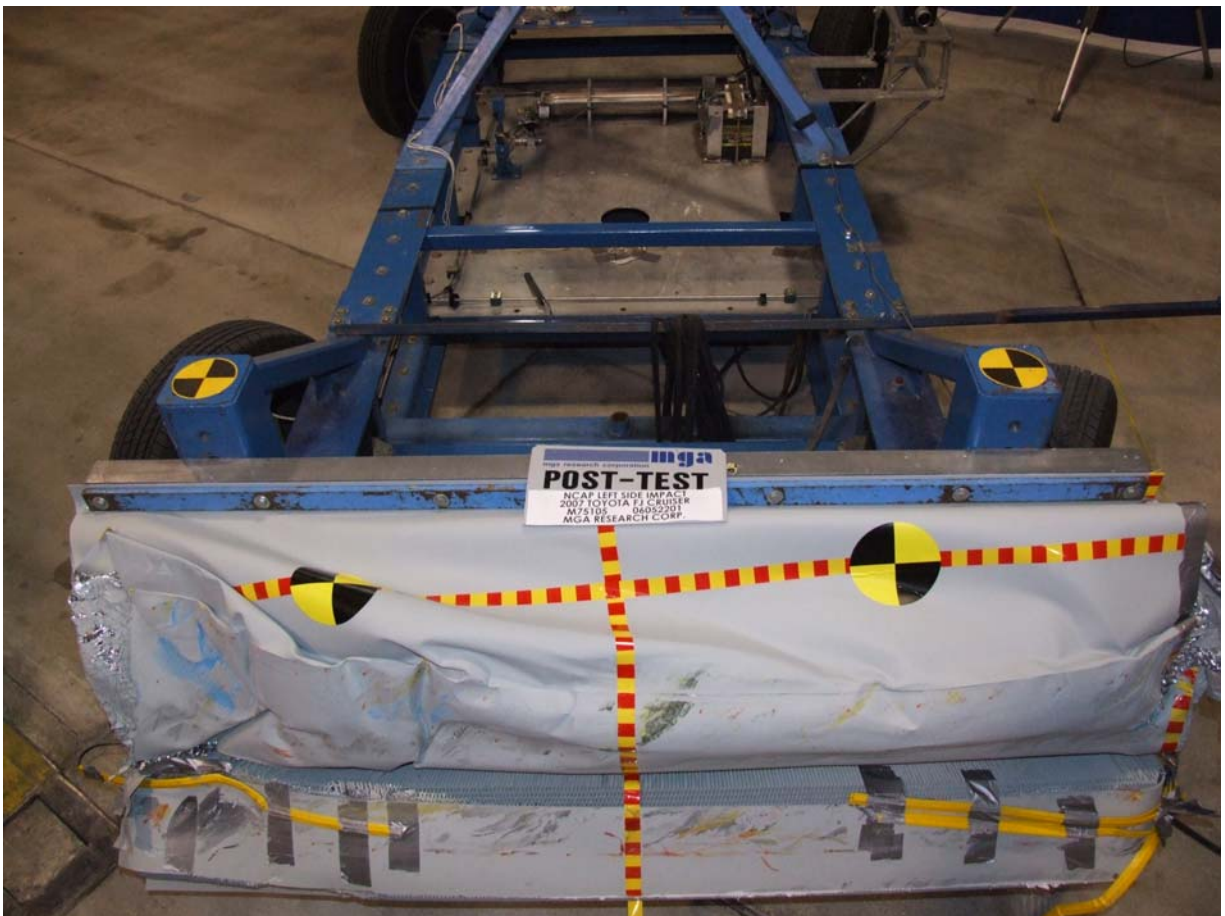
Post-Test Top View of Deformable Barrier
