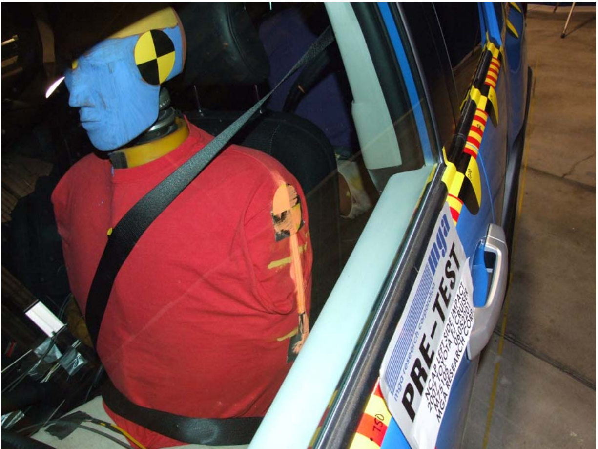
Pre-Test Driver Dummy Clearance From Door
