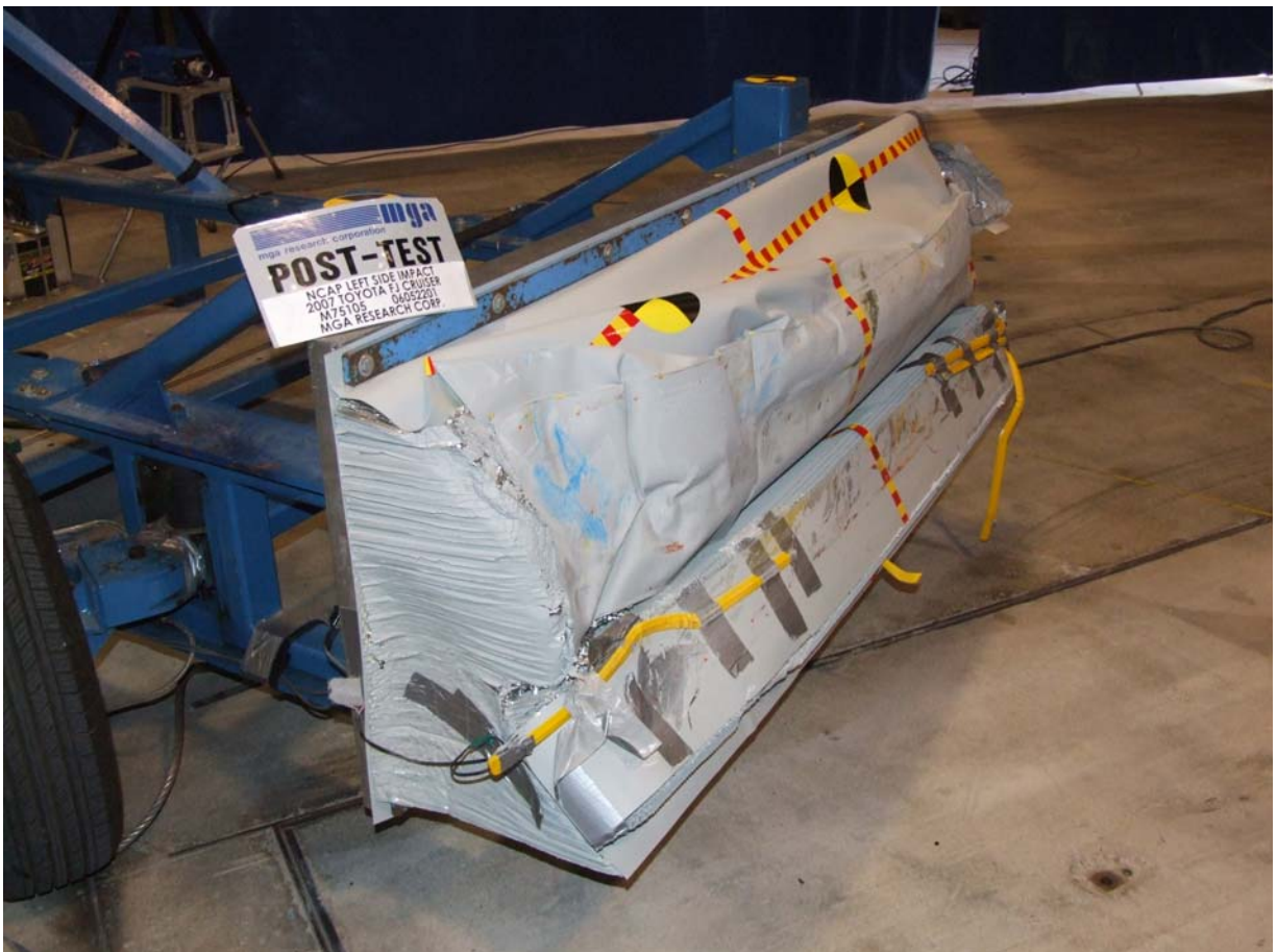
Post-Test Right Side View of Deformable Barrier
