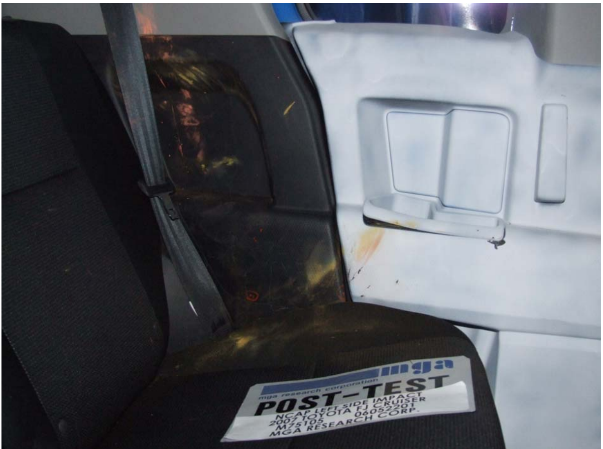
Post-Test Passenger Dummy Torso Contact
