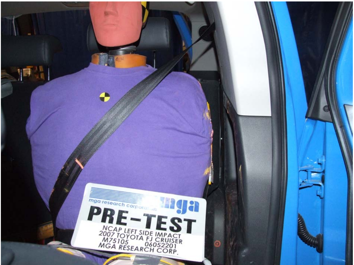
Pre-Test Passenger Dummy Clearance From Door
