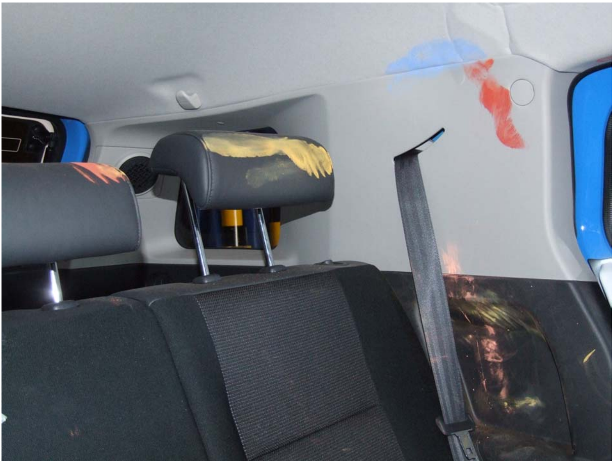
Post-Test Passenger Dummy Head Contact
