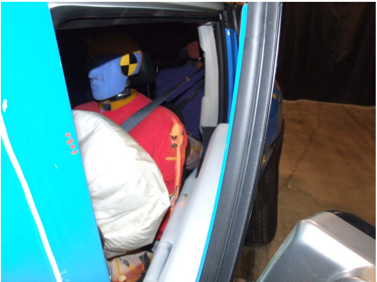
Post-Test Driver Dummy Clearance From Door
