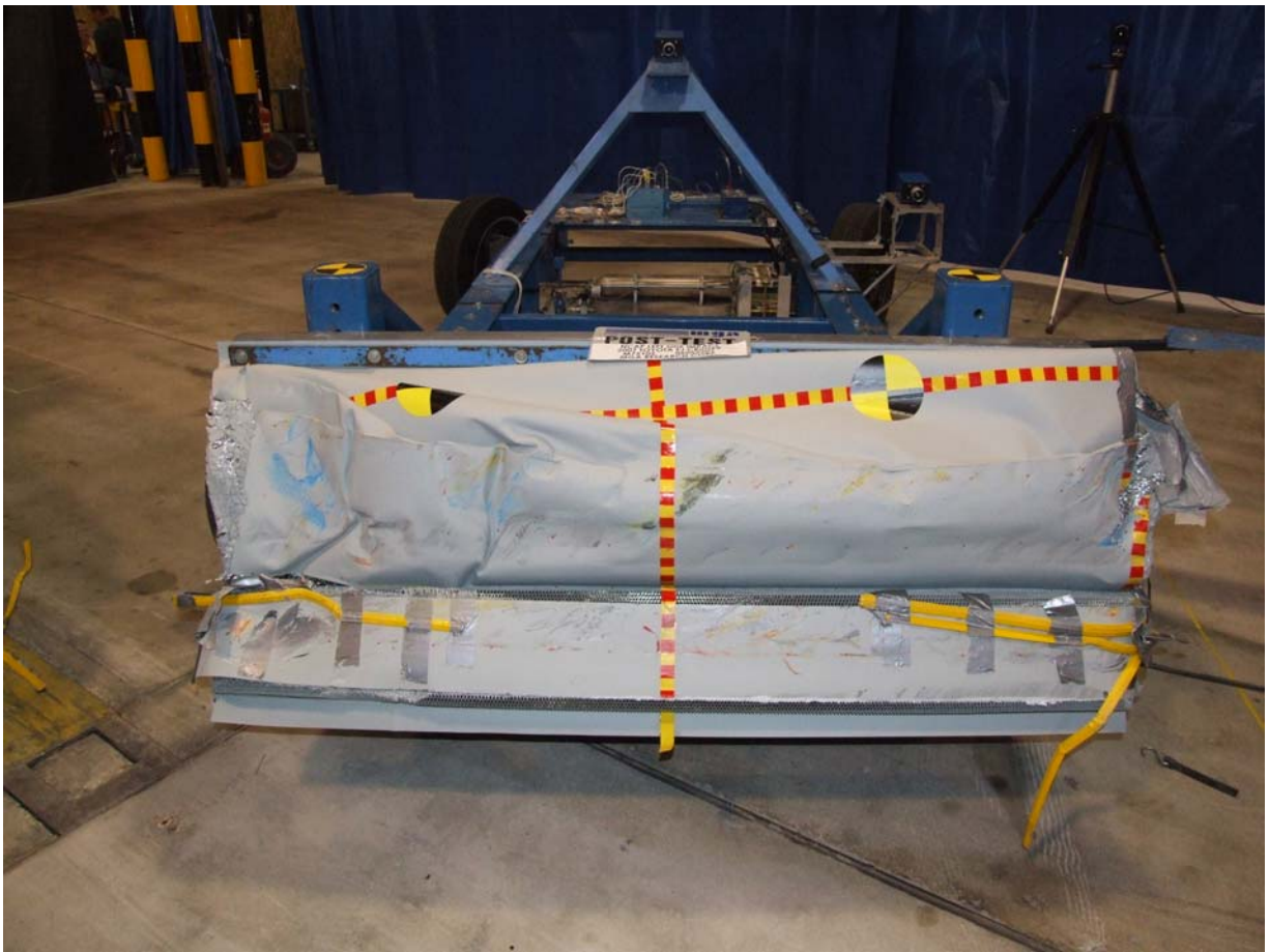
Post-Test Front View of Deformable Barrier
