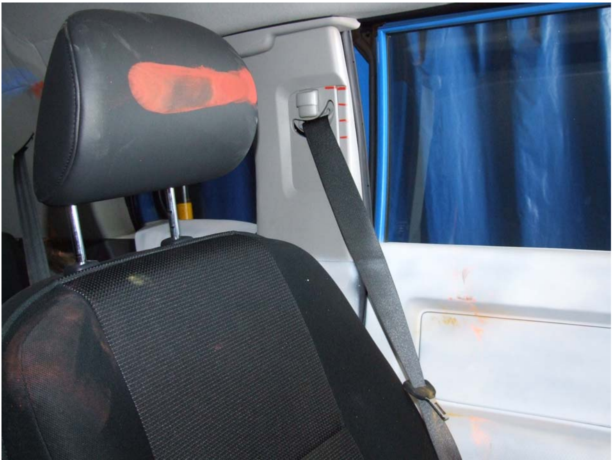
Post-Test Driver Dummy Head Contact
