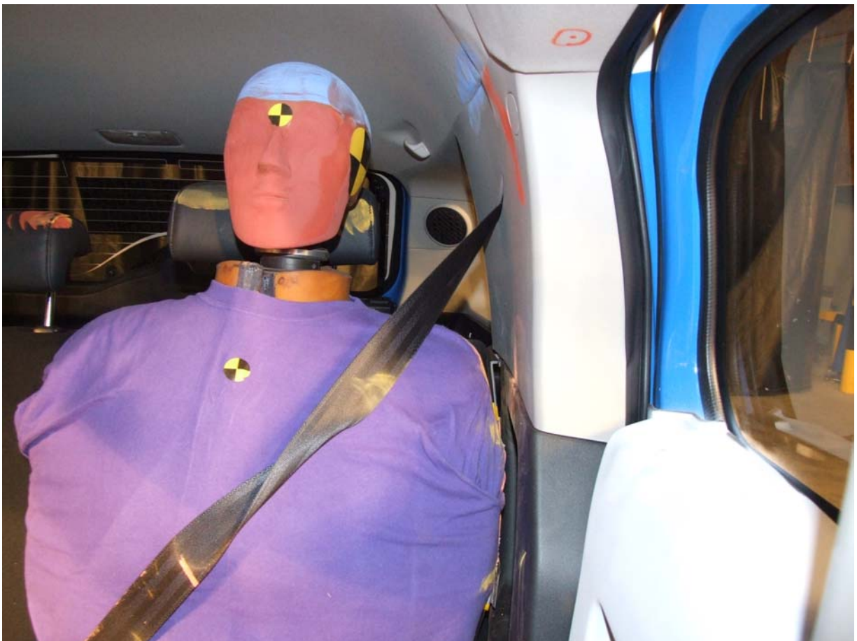
Post-Test Passenger Dummy Clearance From Door
