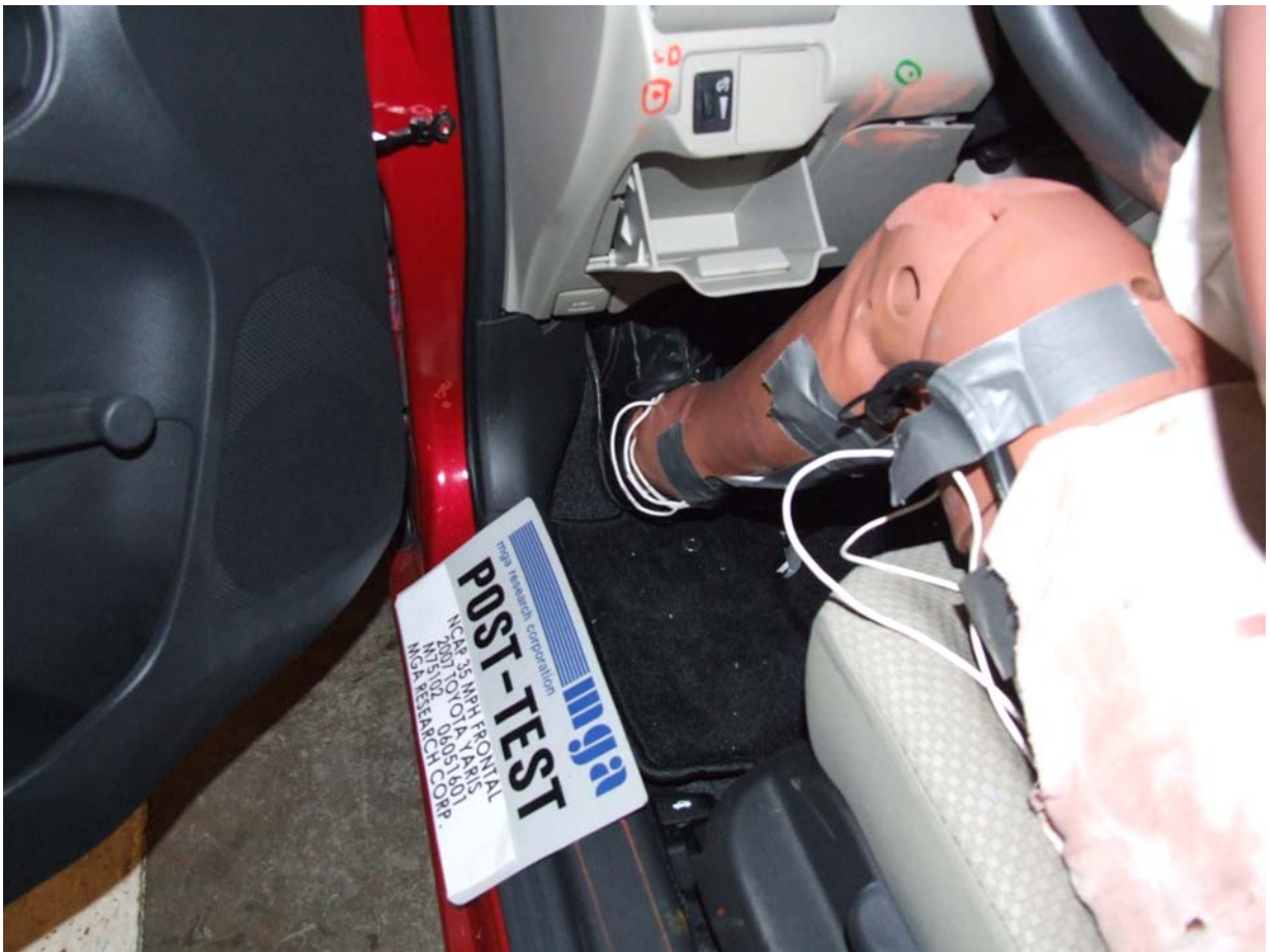
Post-Test Driver Dummy Left Knee Contact
