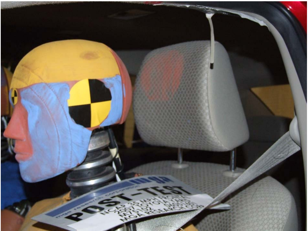
Post-Test Driver Dummy Head Contact
