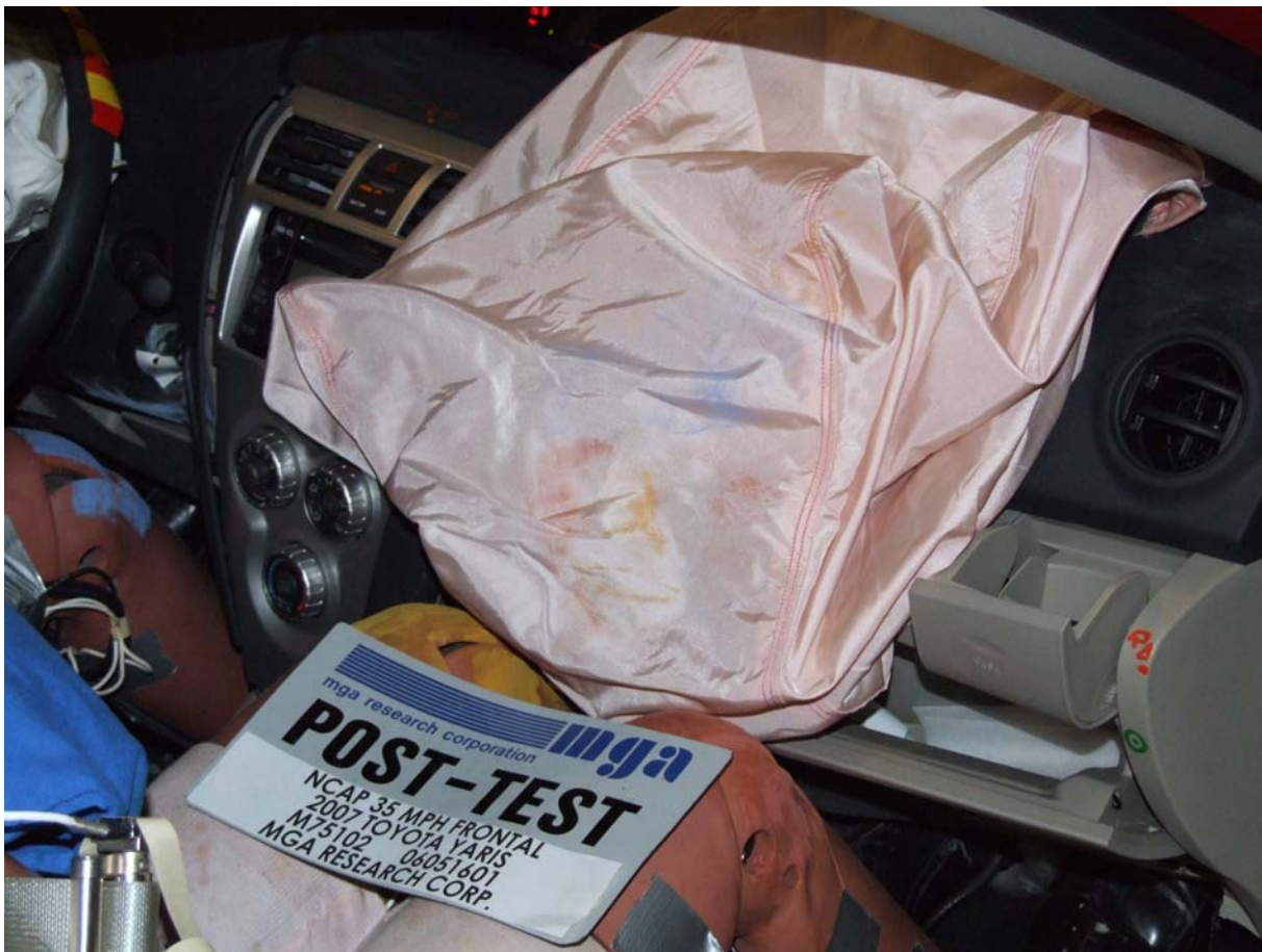
Post-Test Passenger Dummy Airbag Contact
