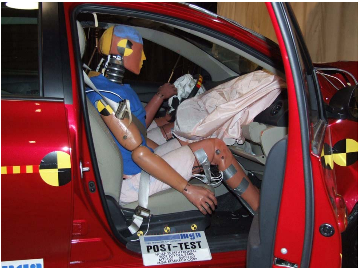
Post-Test Passenger Dummy (Door Open)
