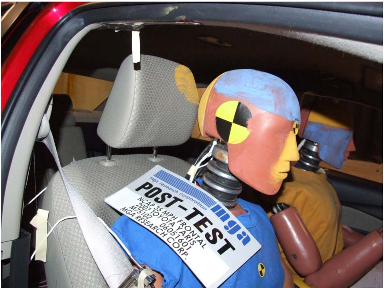
Post-Test Passenger Dummy Head Contact
