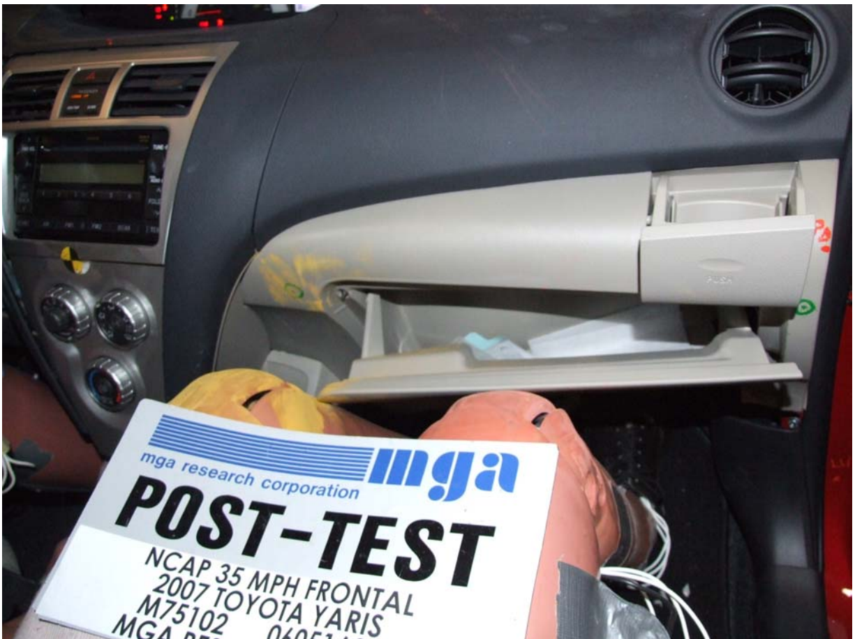
Post-Test Passenger Dummy Knee Contact
