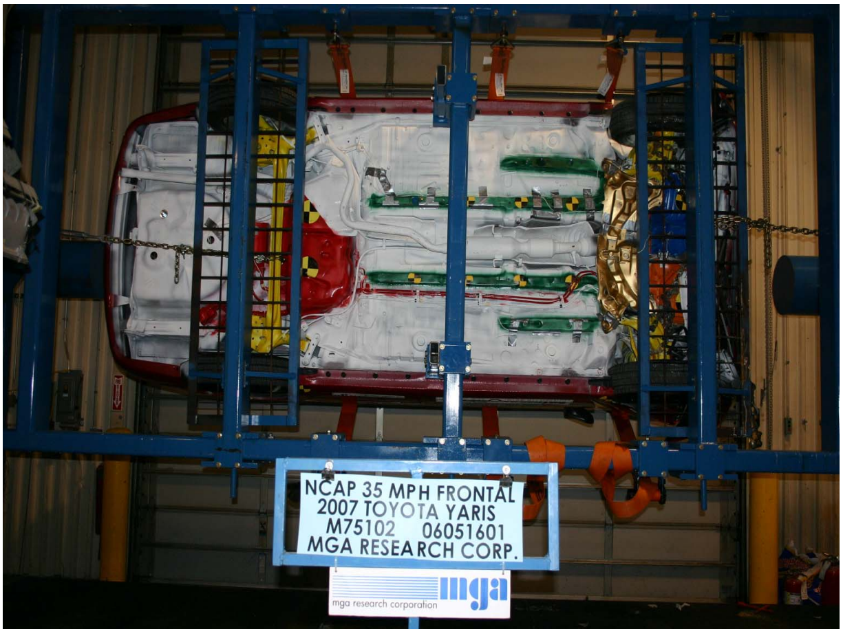
Vehicle on Rollover Device at 90 Degrees
