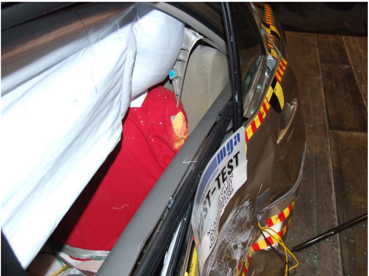
Post-Test Passenger Dummy Clearance From Door
