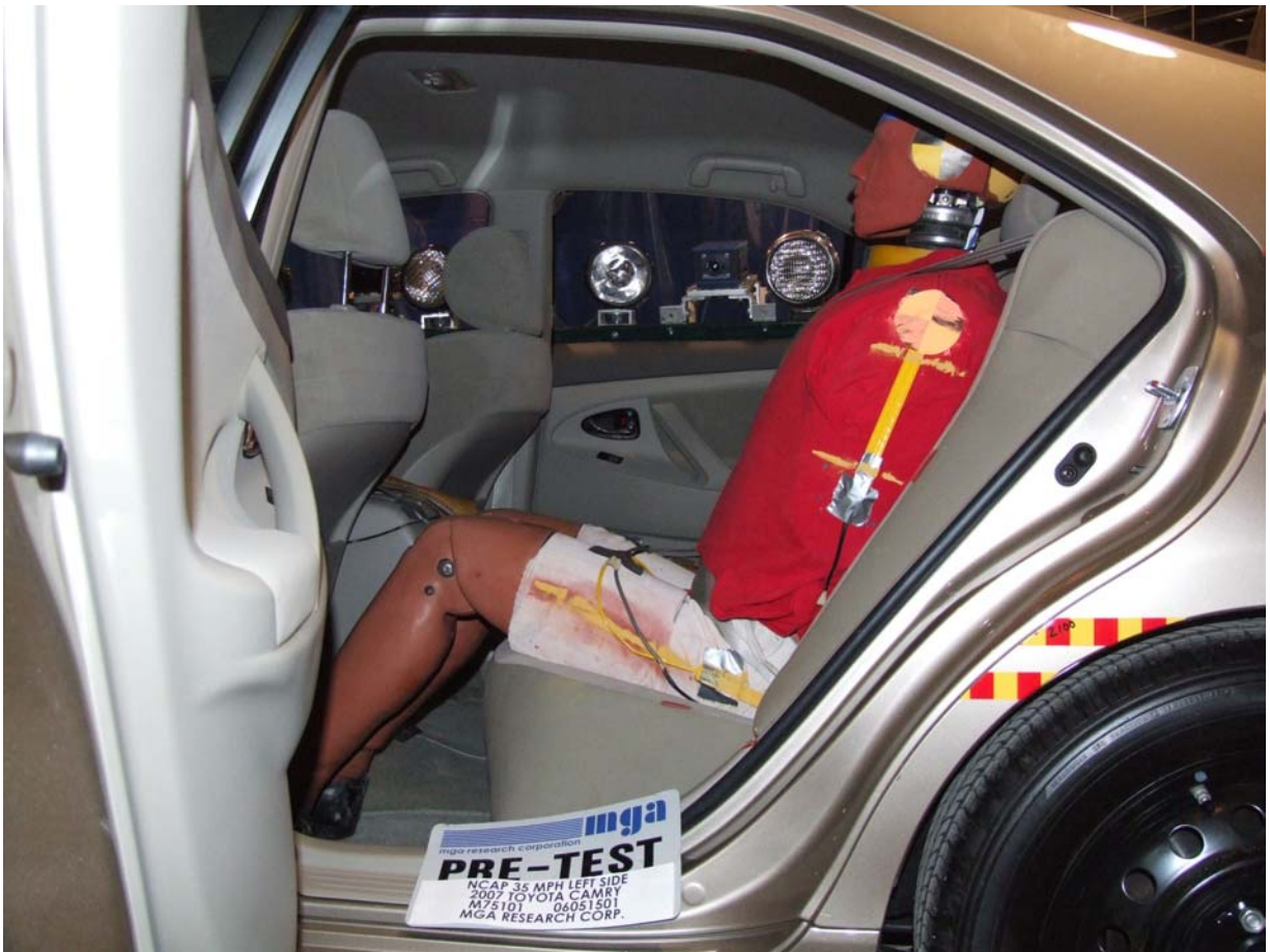
Pre-Test Passenger Dummy (Door Open)
