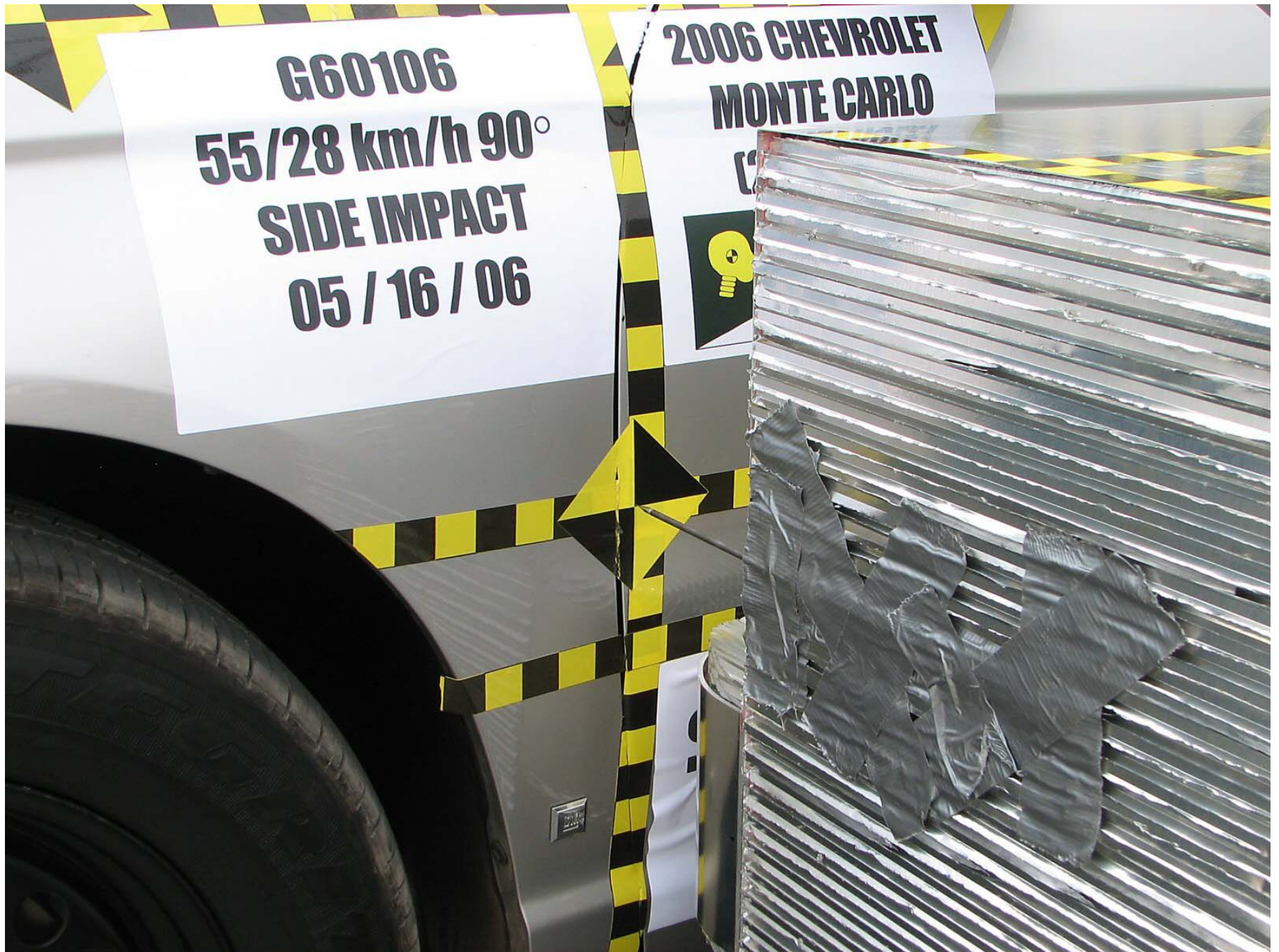
Figure A-25: Pre-Test Left Impact Point
