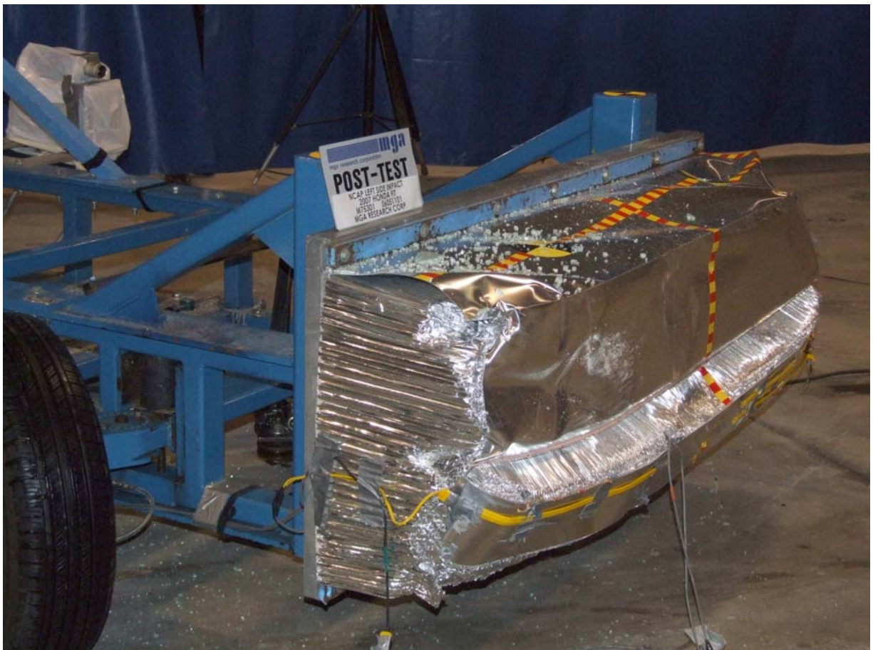
Post-Test Right Side View of Deformable Barrier
