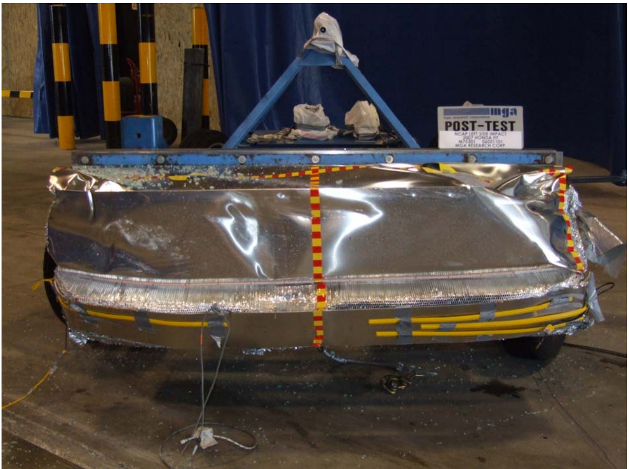
Post-Test Front View of Deformable Barrier
