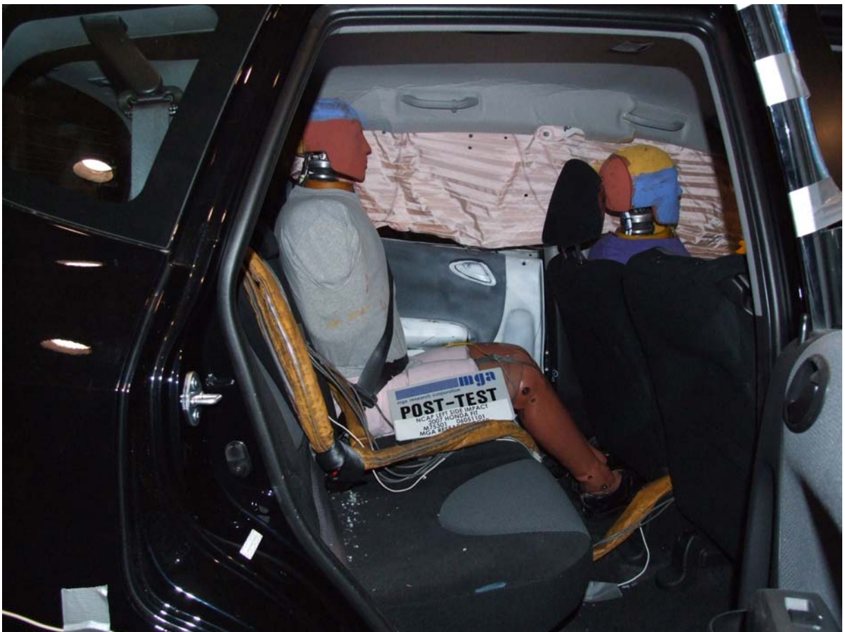
Post-Test Passenger Dummy Right Side View
