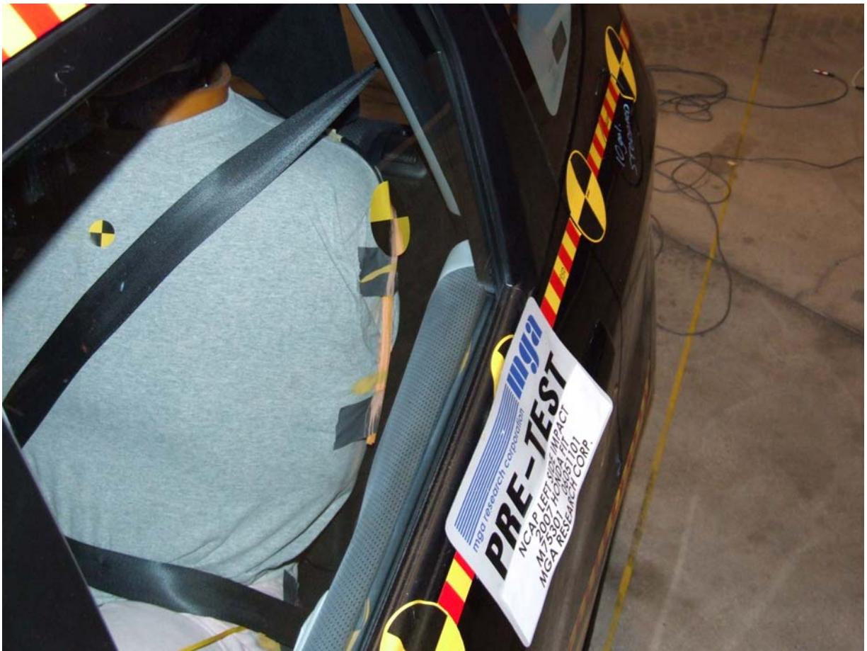
Pre-Test Passenger Dummy Clearance From Door
