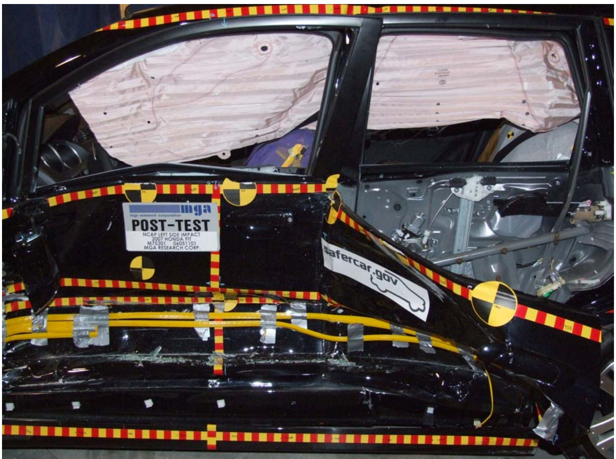
Post-Test Left Impact Zone
