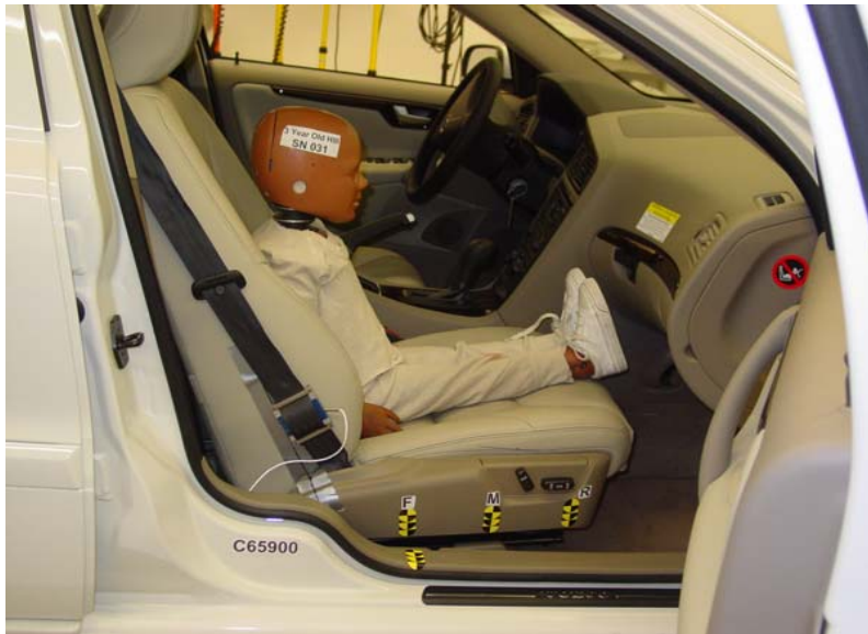
3-Year-Old Unbelted, Forward Seat Track, Position 1
