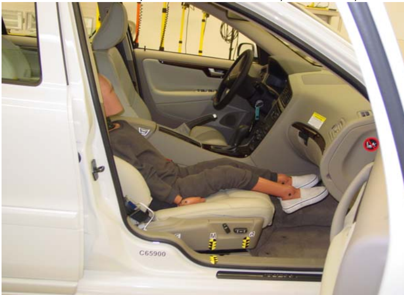
6-Year-Old Unbelted, Middle Seat Track, Position 2
