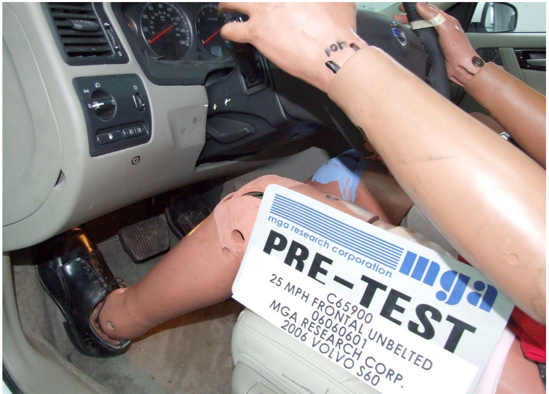
Pre-Test Driver Side Knee Bolster View
