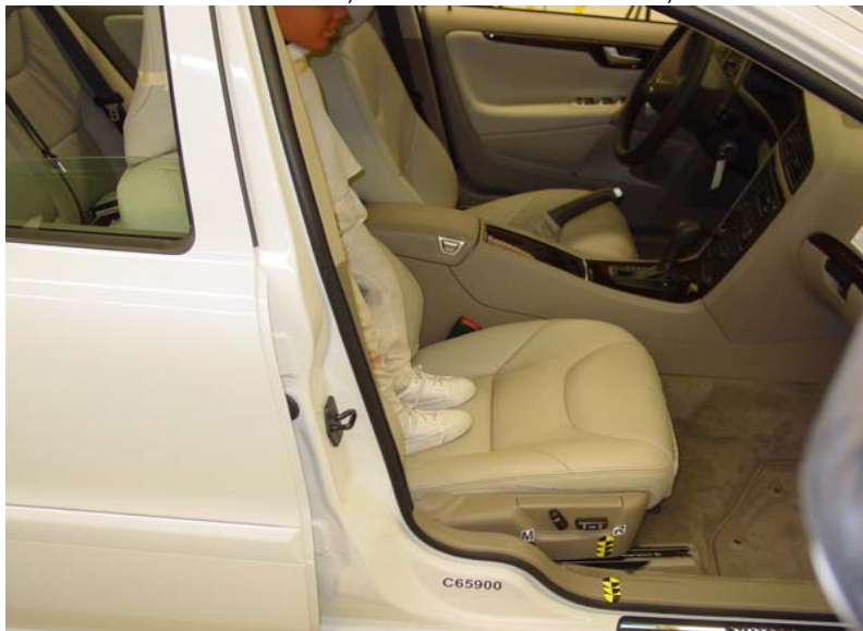
3-Year-Old Unbelted, Rearward Seat Track, Position 5
