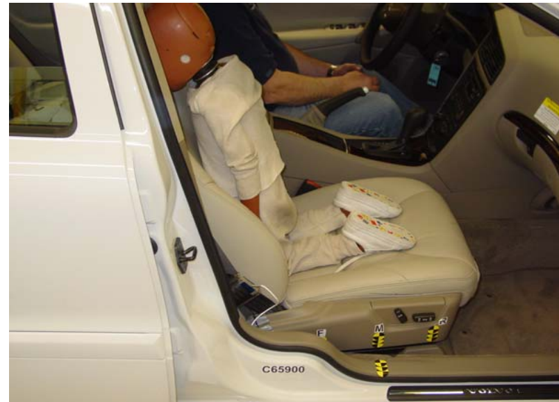
3-Year-Old Unbelted, Middle Seat Track, Position 7
