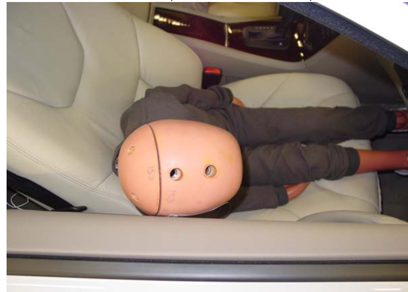
6-Year-Old Unbelted, Forward Seat Track, Position 4
