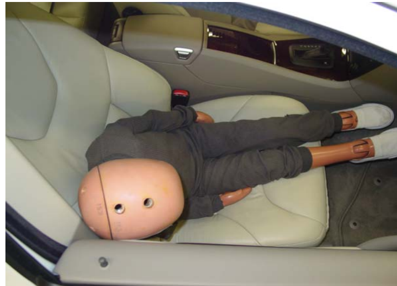
6-Year-Old Unbelted, Rearward Seat Track, Position 4
