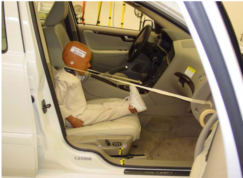
3-Year-Old Unbelted, Rearward Seat Track, Position 3
