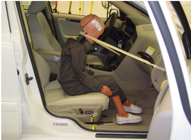
6-Year-Old Unbelted, Rearward Seat Track, Position 3
