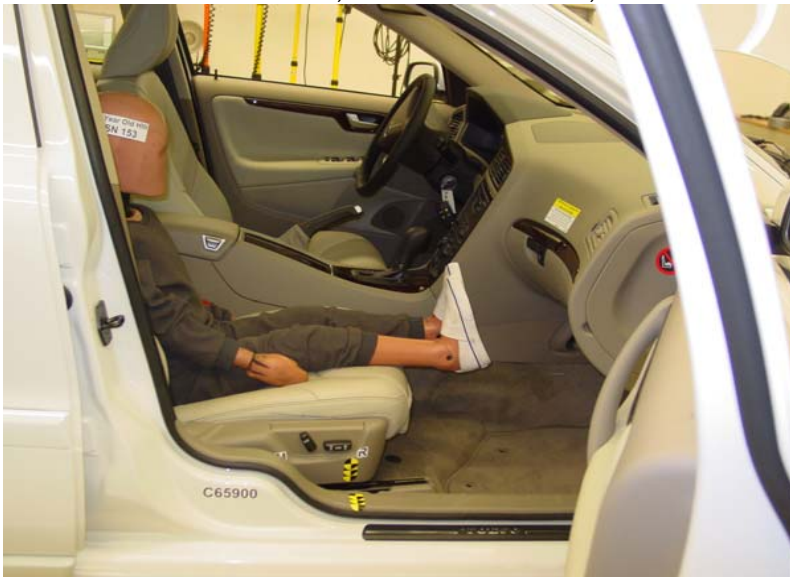
6-Year-Old Unbelted, Rearward Seat Track, Position 1
