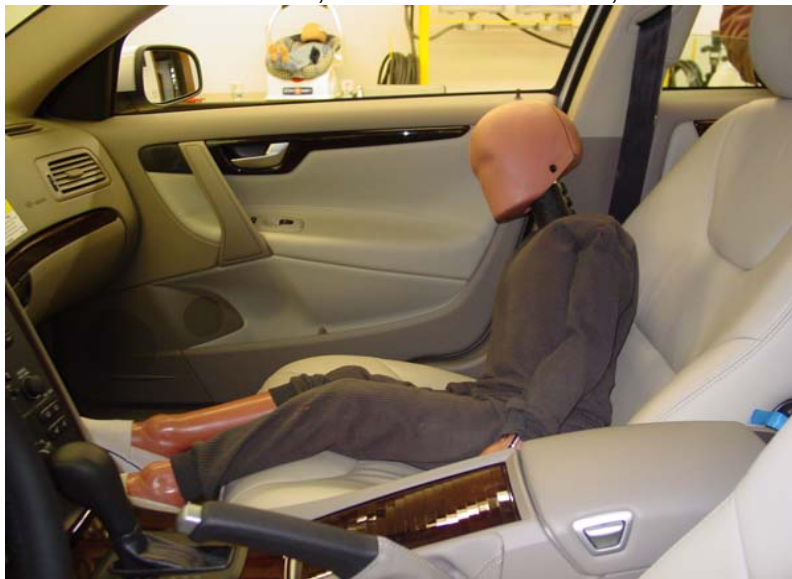
6-Year-Old Unbelted, Rearward Seat Track, Position 4, View 2
