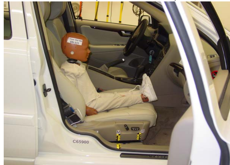
3-Year-Old Unbelted, Middle Seat Track, Position 1
