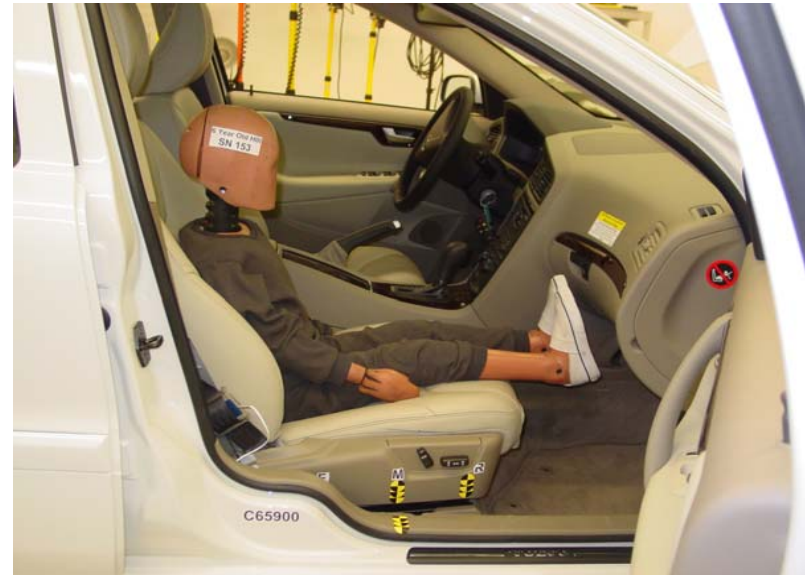
6-Year-Old Unbelted, Middle Seat Track, Position 1
