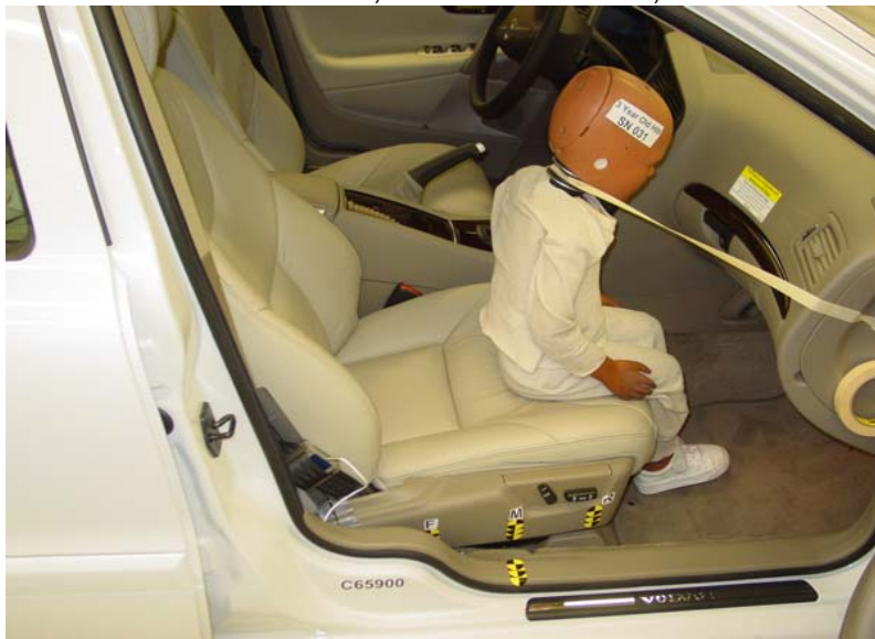
3-Year-Old Unbelted, Middle Seat Track, Position 4
