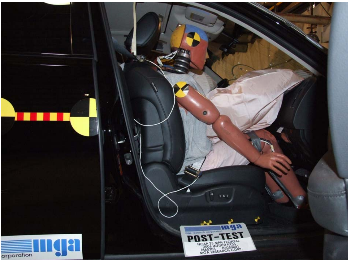
Post-Test Passenger Dummy (Door Open)
