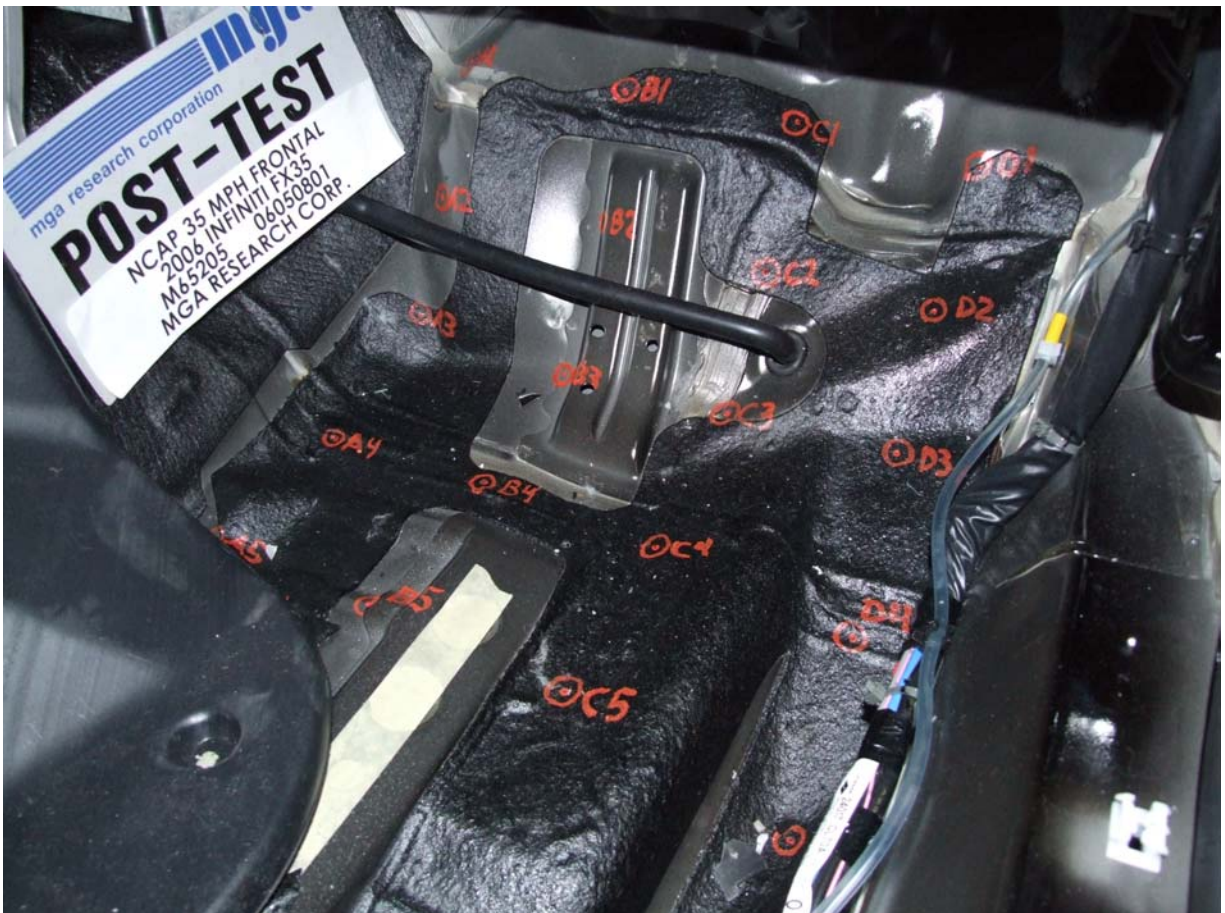
Post-Test Passenger Side Floor Pan
