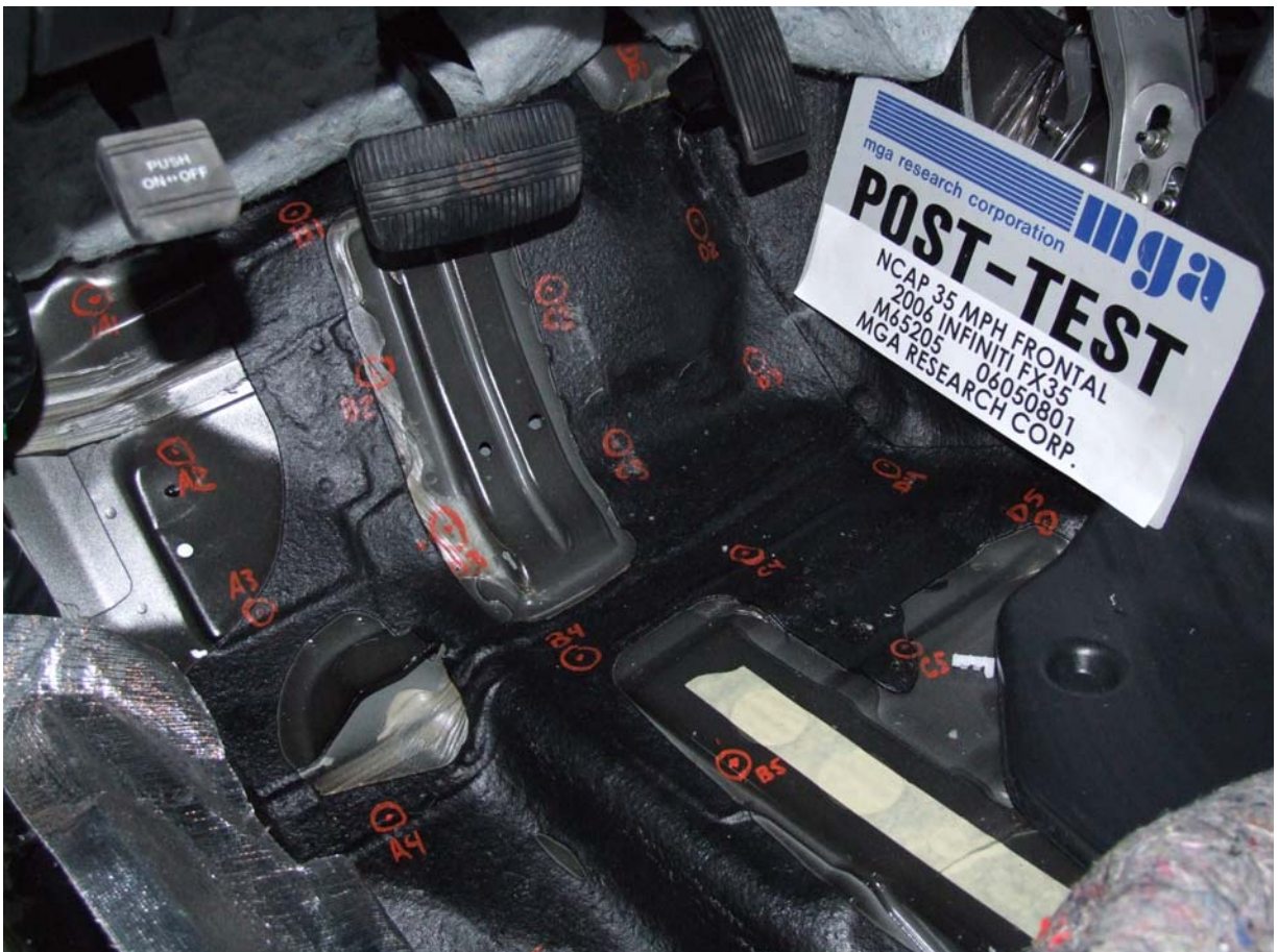
Post-Test Driver Side Floor Pan
