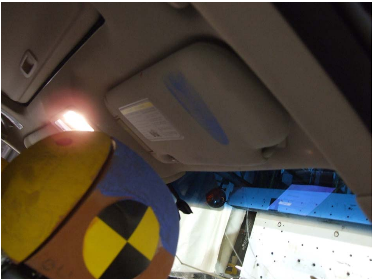
Post-Test Passenger Dummy Head Contact (visor)
