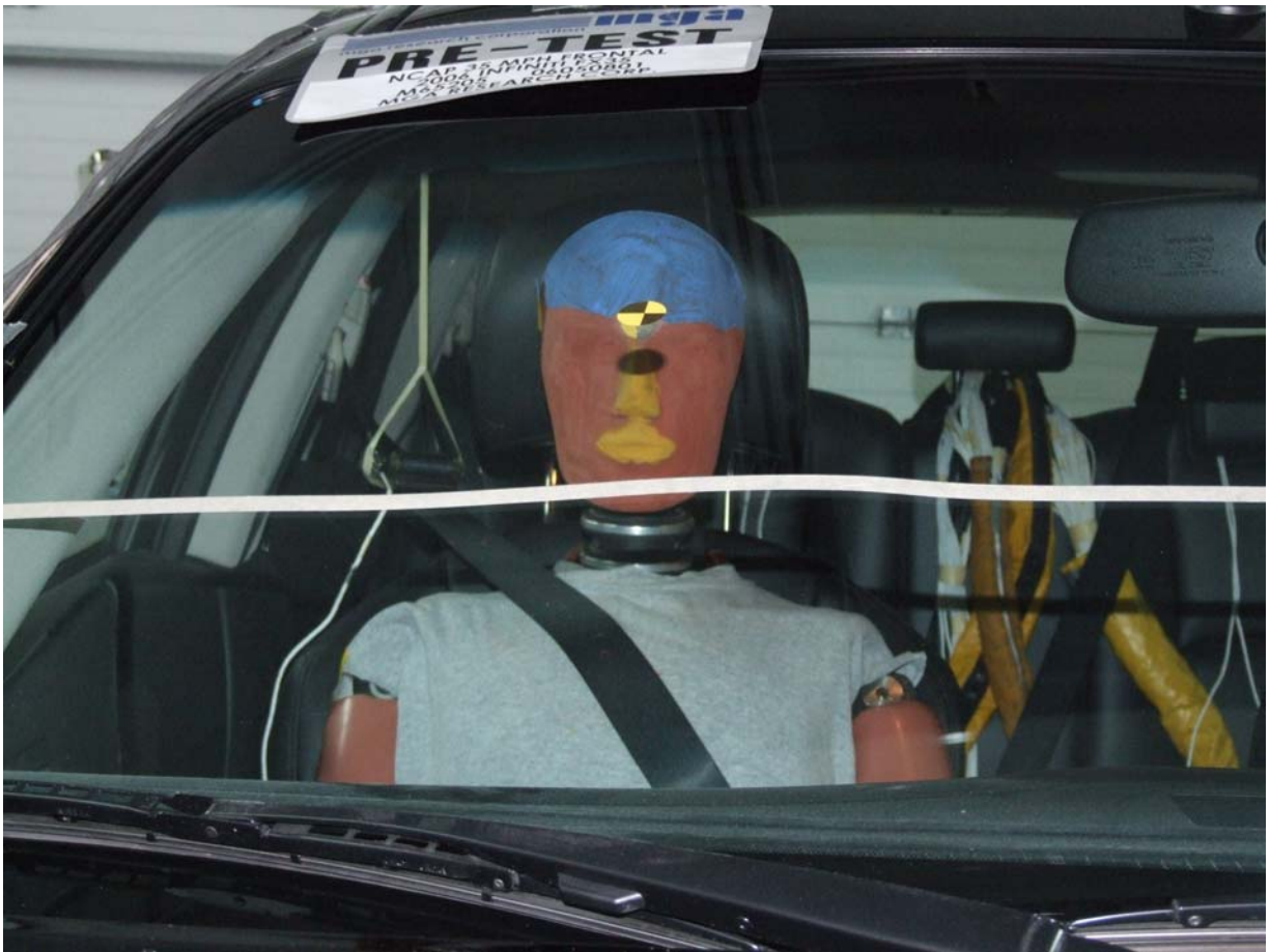
Pre-Test Passenger Dummy Front View (Head Position)
