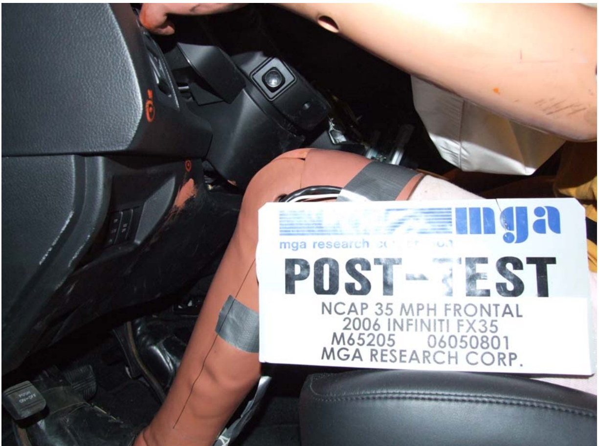
Post-Test Driver Side Knee Bolster
