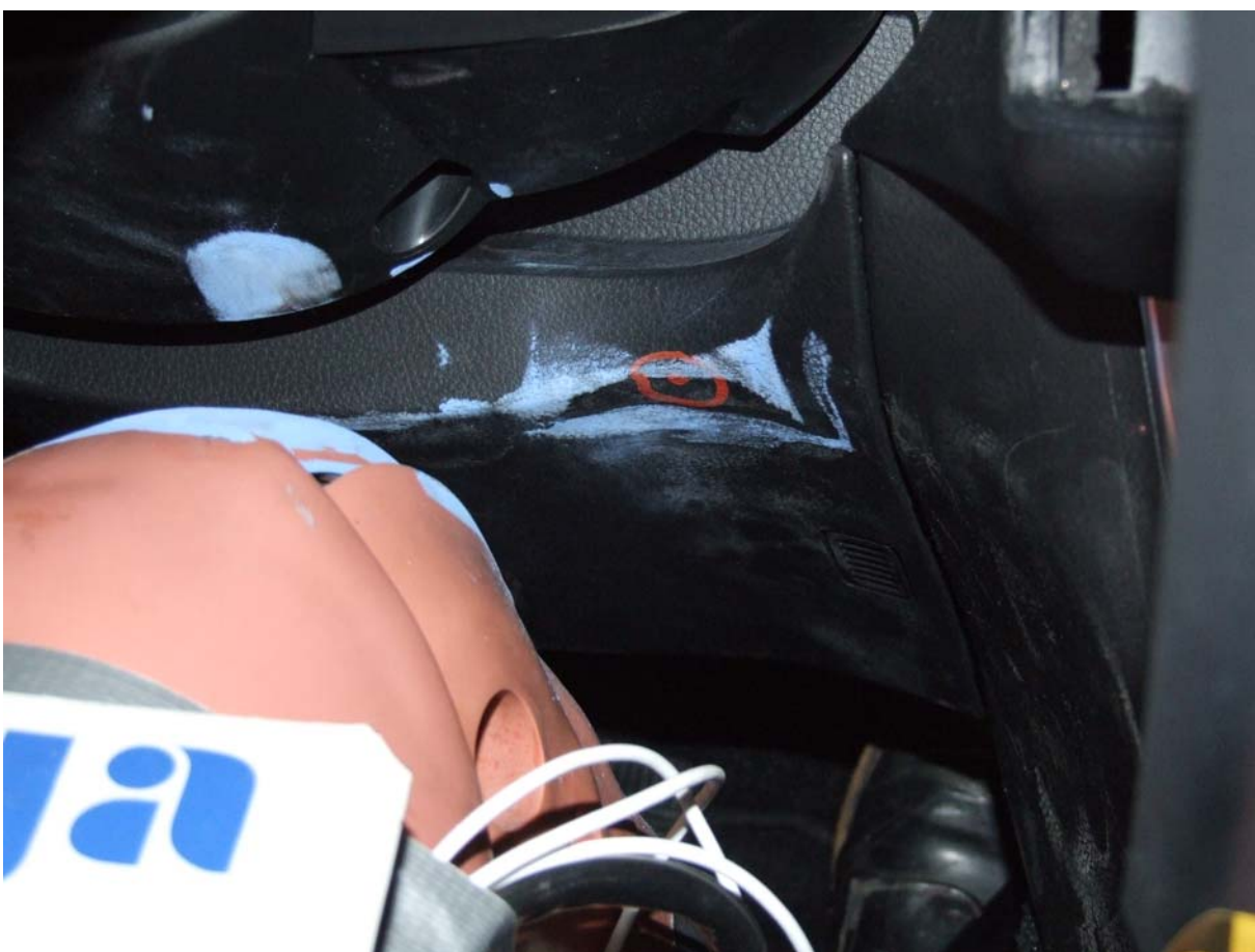
Post-Test Driver Dummy Right Knee Contact
