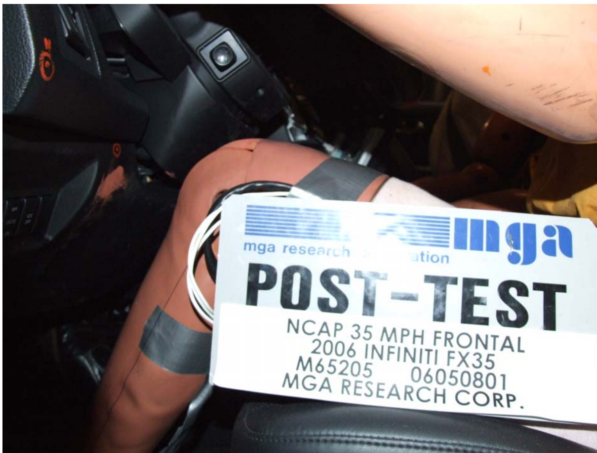
Post-Test Driver Dummy Left Knee Contact
