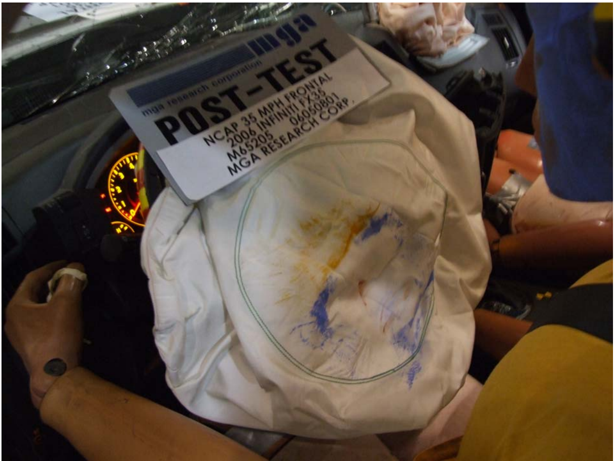
Post-Test Driver Dummy Airbag Contact
