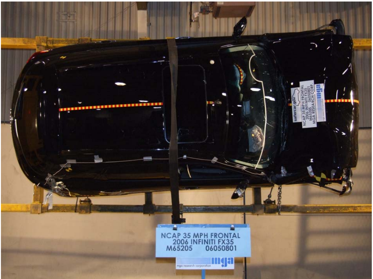
Vehicle on Rollover Device at 90 Degrees
