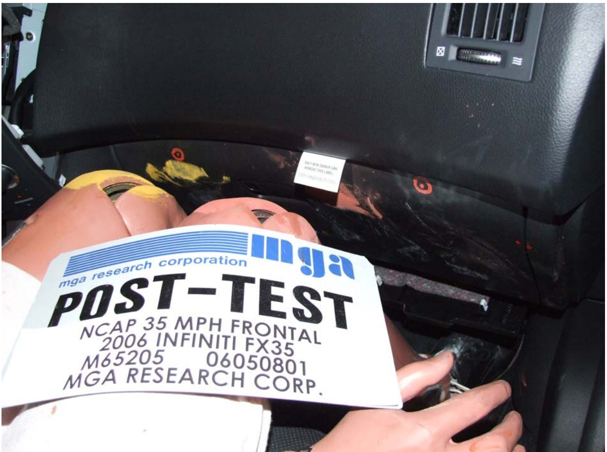
Post-Test Passenger Side Glove Box
