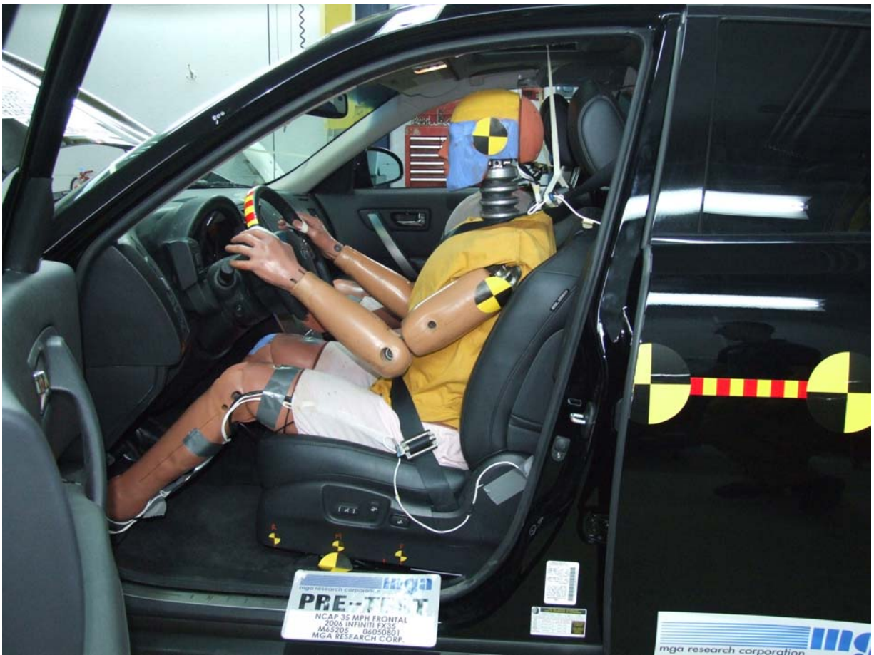
Pre-Test Driver Dummy (Door Open)
