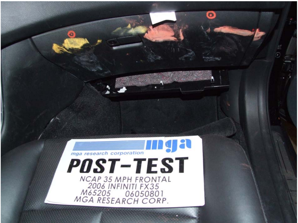
Post-Test Passenger Dummy Knee Contact
