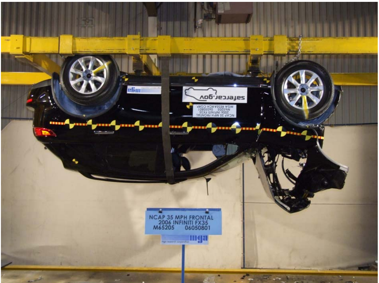
Vehicle on Rollover Device at 180 Degrees
