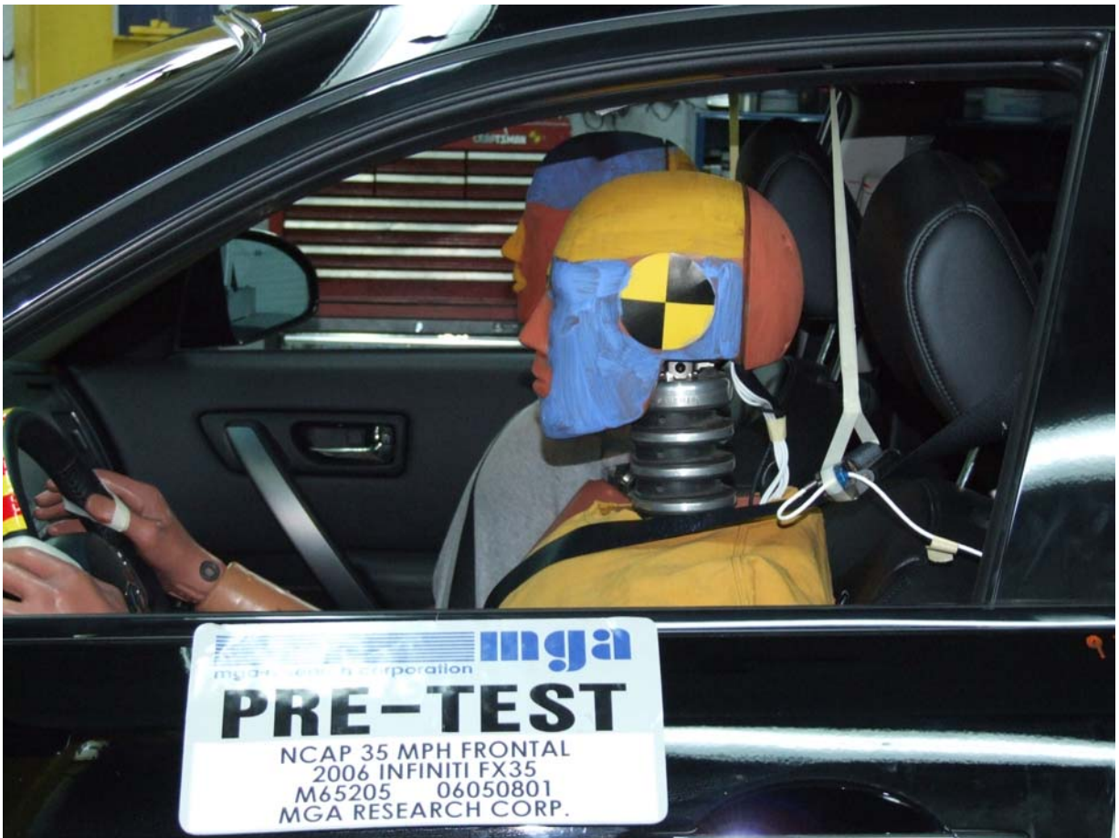
Pre-Test Driver Dummy (Through Window)
