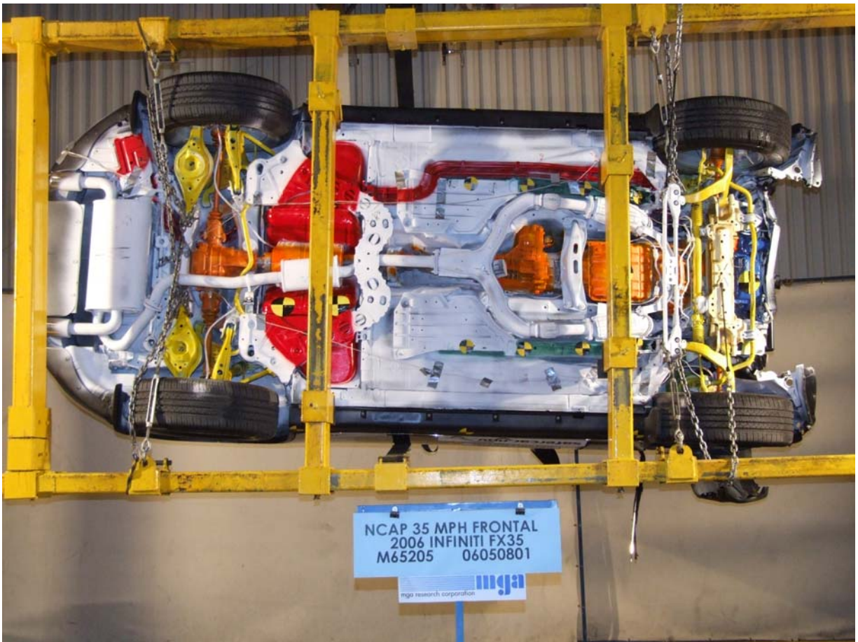
Vehicle on Rollover Device at 270 Degrees
