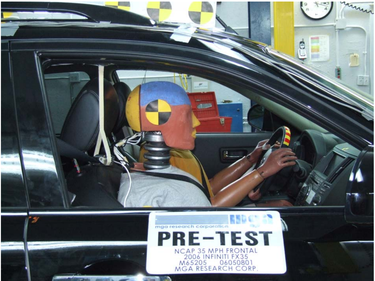
Pre-Test Passenger Dummy (Through Window)
