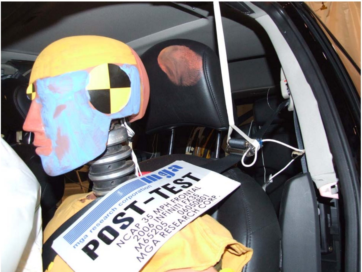
Post-Test Driver Dummy Head Contact
