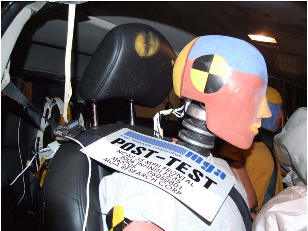
Post-Test Passenger Dummy Head Contact (headrest)
