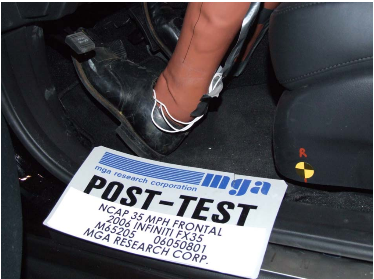
Post-Test Driver Dummy Feet
