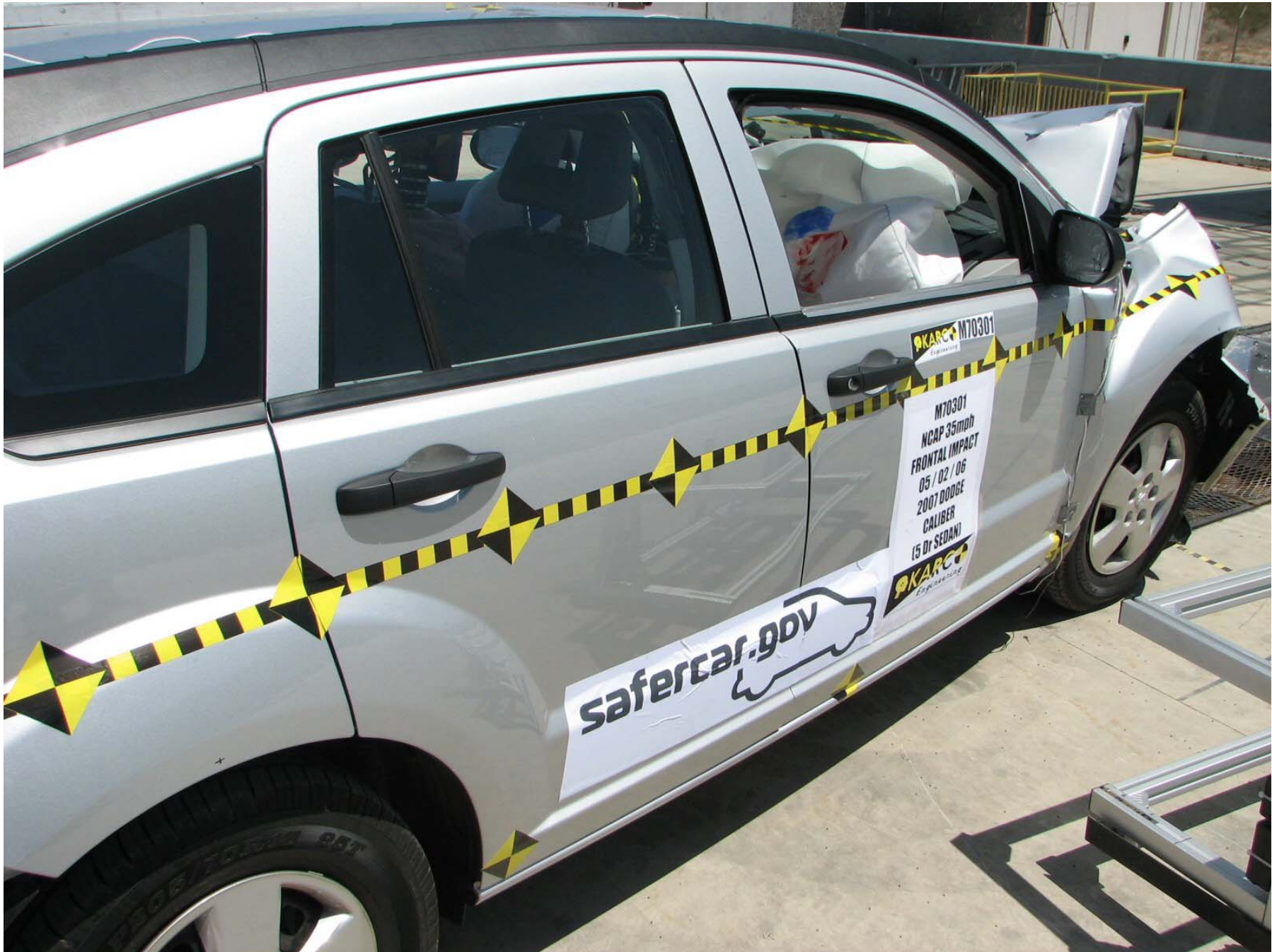
Figure A-17: Post-Test Right Side ¾ View of Doors After Impact
